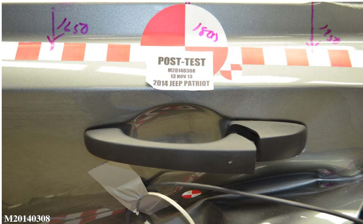
Figure A-24: Post-Test Left Rear Door Latch Close-Up
