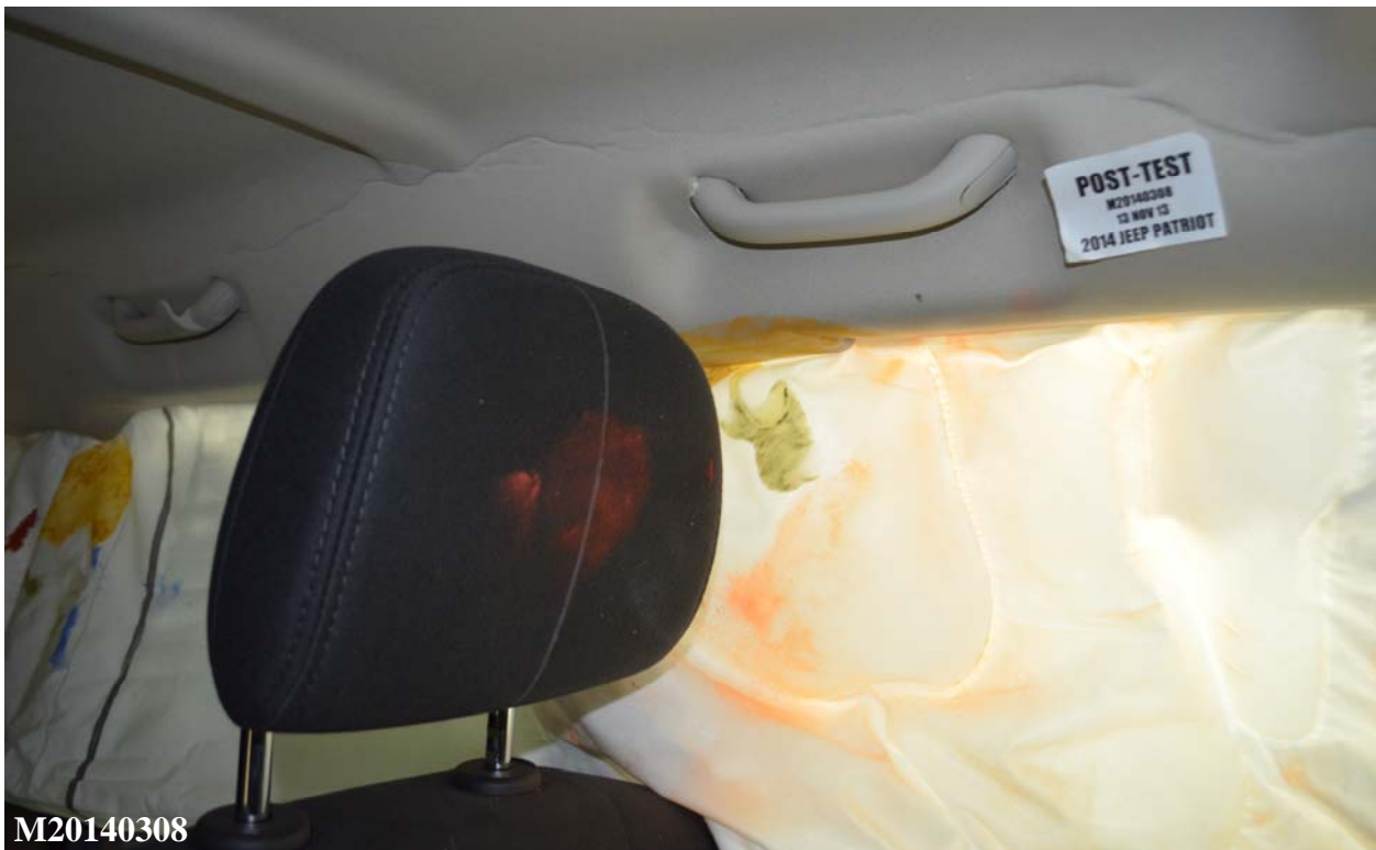
Figure A-48: Post-Test Driver Dummy Close-Up Head Contact With Vehicle Interior View
