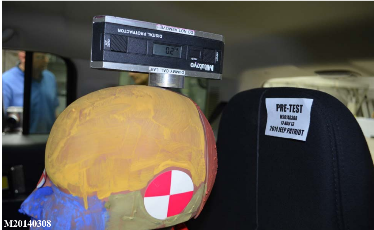
Figure A-63: Pre-Test View of Rear Passenger Dummy's Head Showing Dummy's Head is Level
