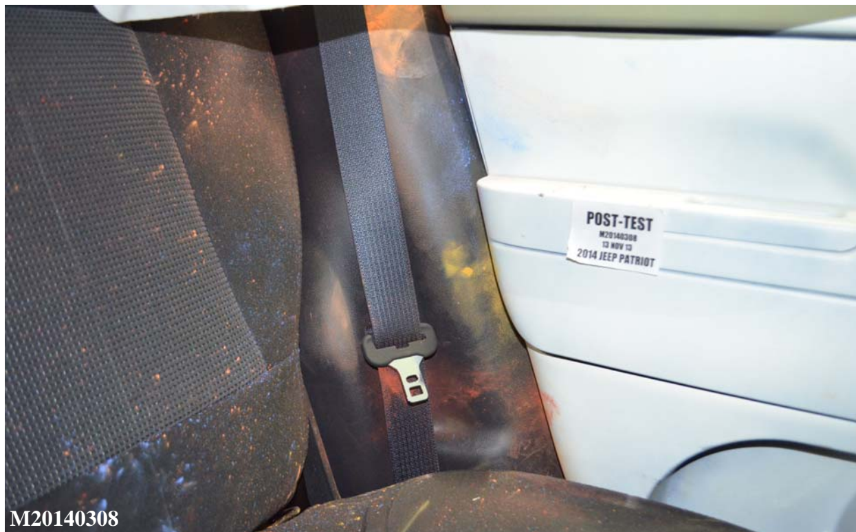
Figure A-79: Post-Test Rear Passenger Dummy Close-Up Pelvis Contact with Vehicle Interior View
