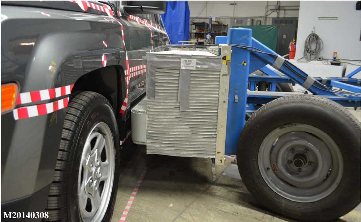
Figure A-17: Pre-Test Left Side View of MDB Positioned Against Side of Test Vehicle
