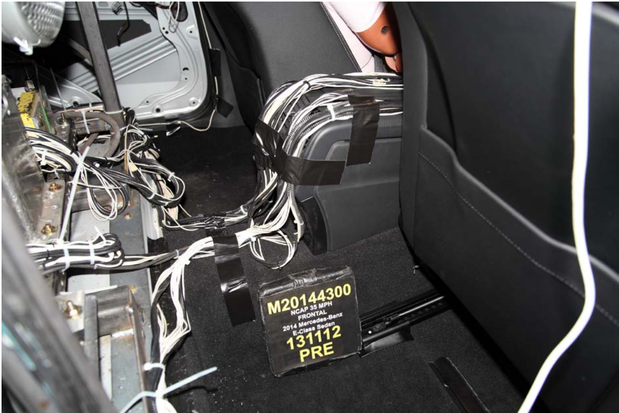
027 Pre-test Dummy Cable Routing
