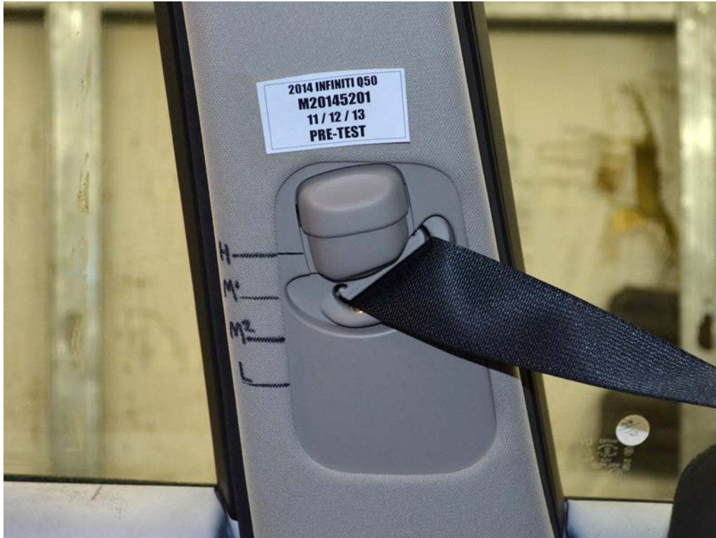
FIGURE 33. Pre-Test View of Belt Anchorage for Dummy
