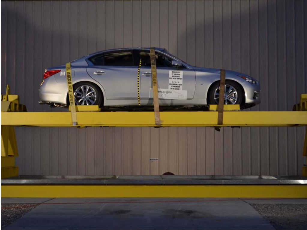
FIGURE 67. FMVSS No. 301 Static Rollover 360 Degrees
