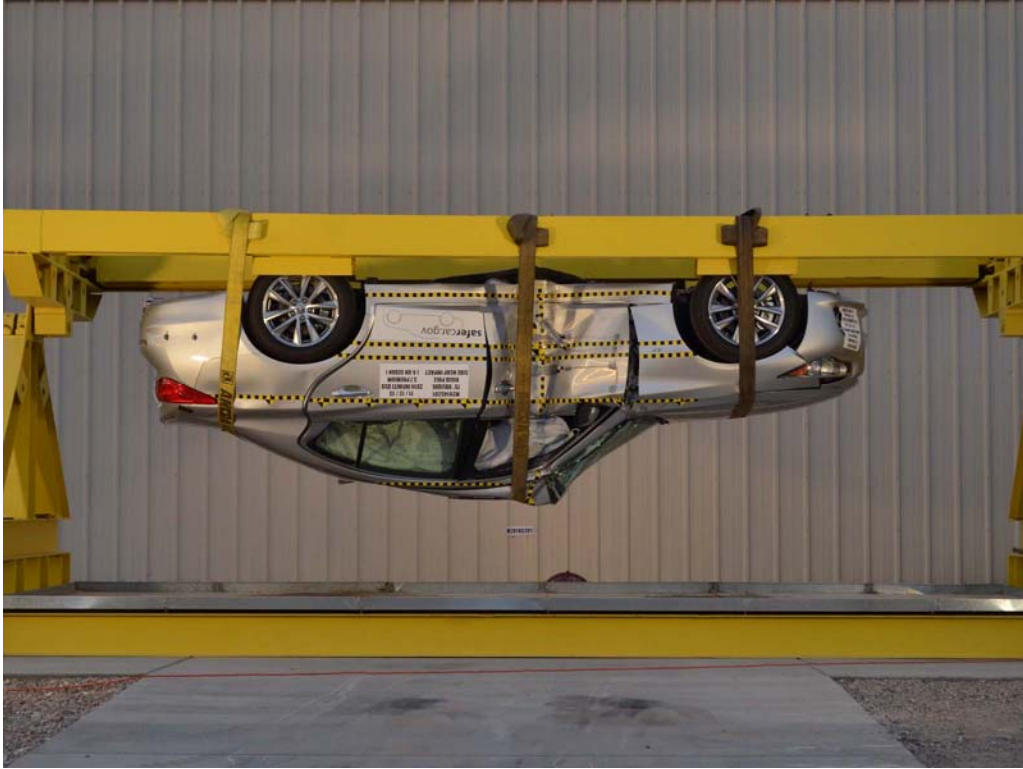
FIGURE 65. FMVSS No. 301 Static Rollover 180 Degrees
