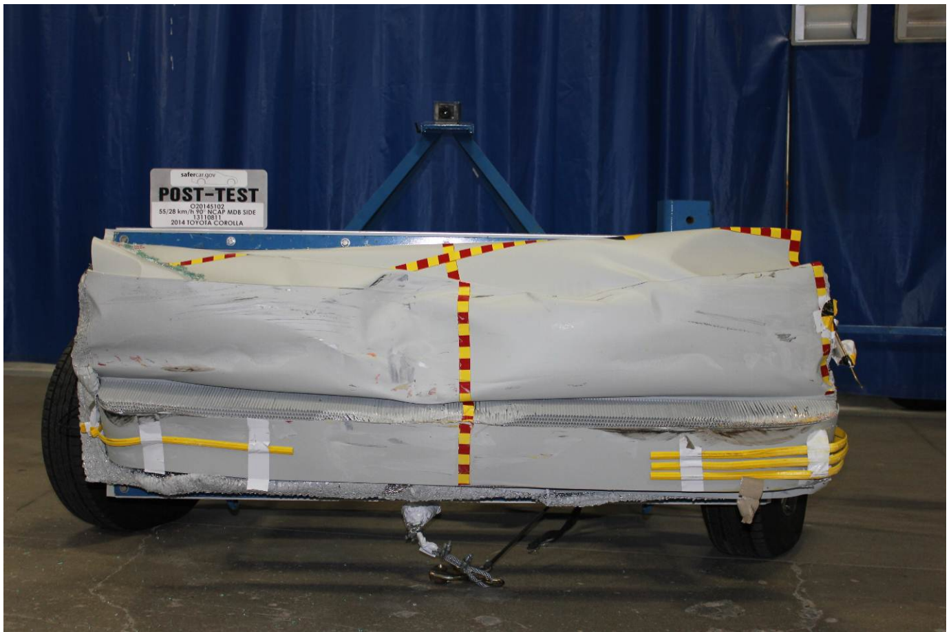
Post-Test Front View of MDB Impactor Face
