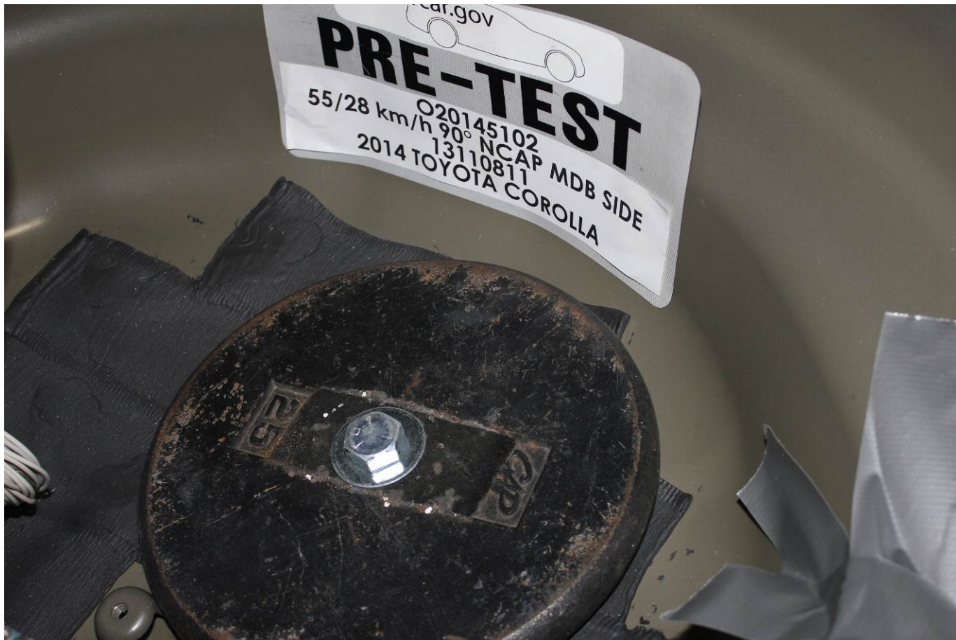
Pre-Test Ballast View
