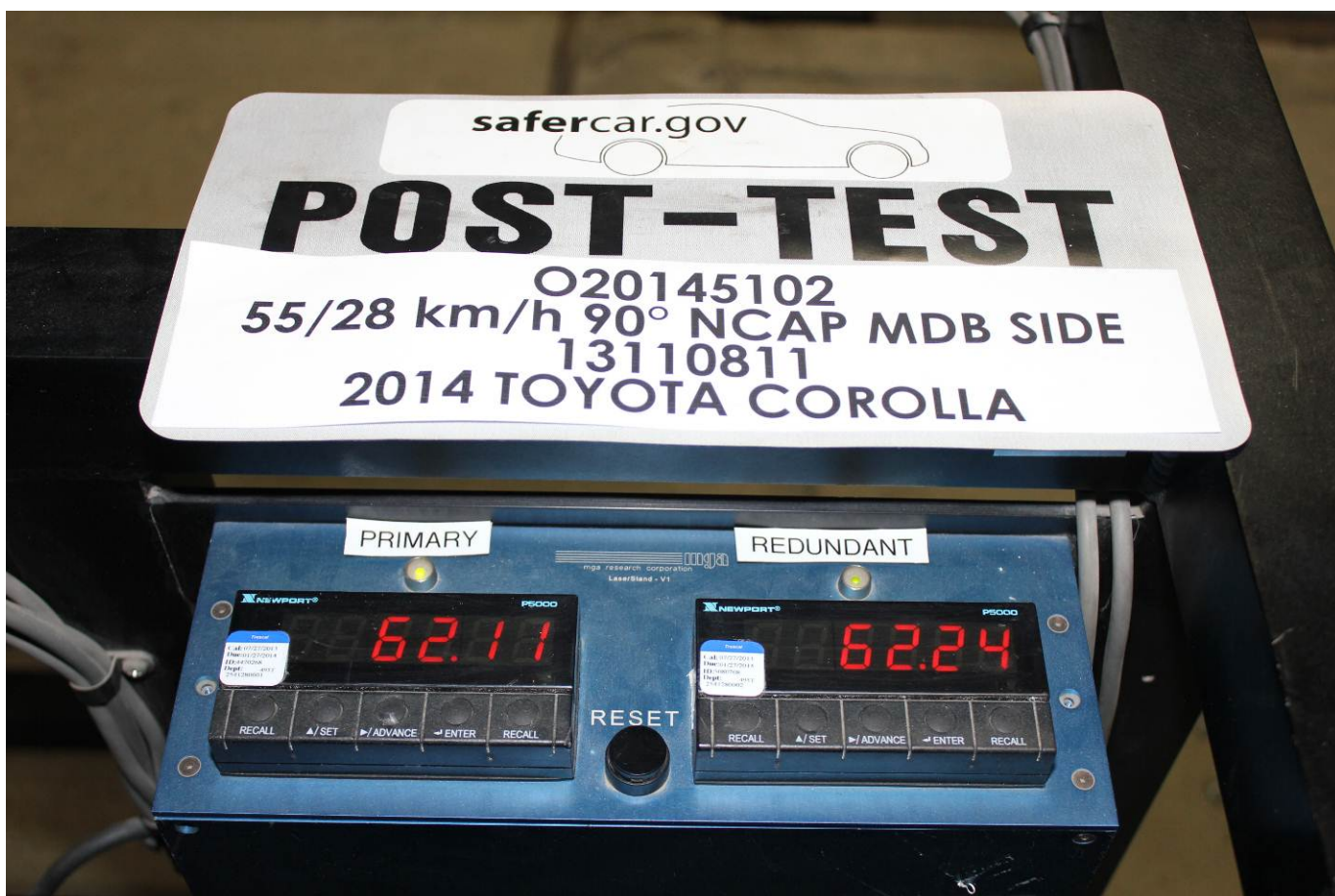
Post-Test Primary and Redundant Speed Trap Read-Out
