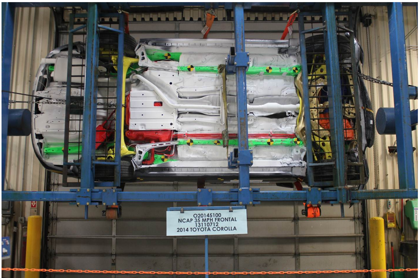
Vehicle at 90 Degrees on Static Rollover Device
