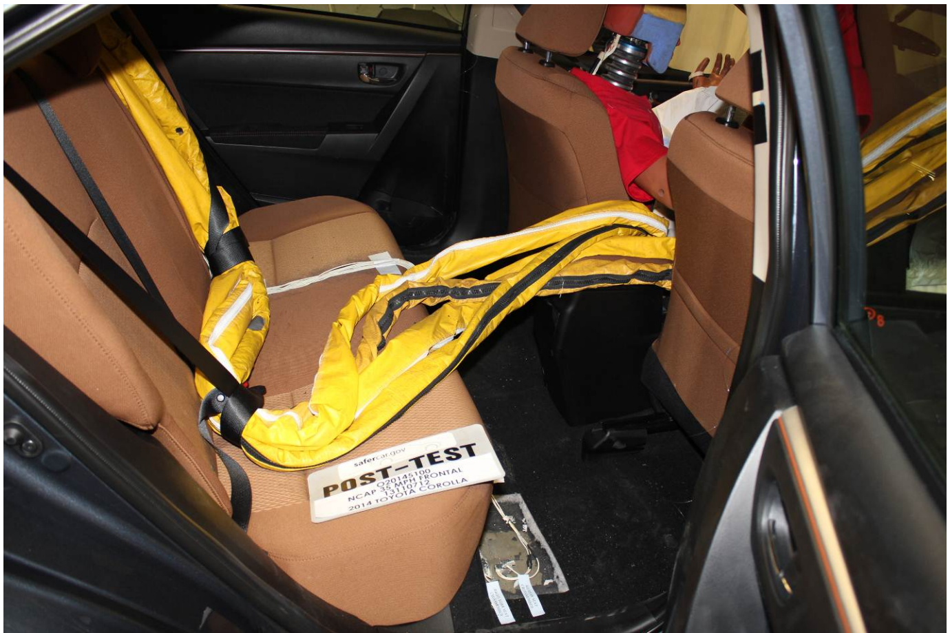
Post-Test Dummy Cable Routing
