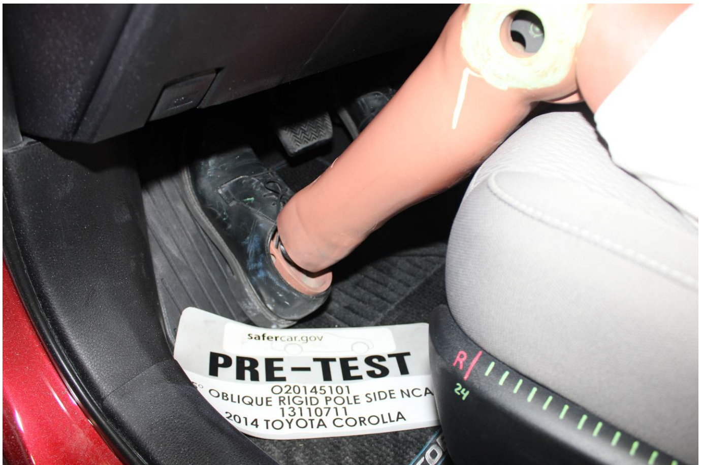
Pre-Test Placement of Dummy's Feet
