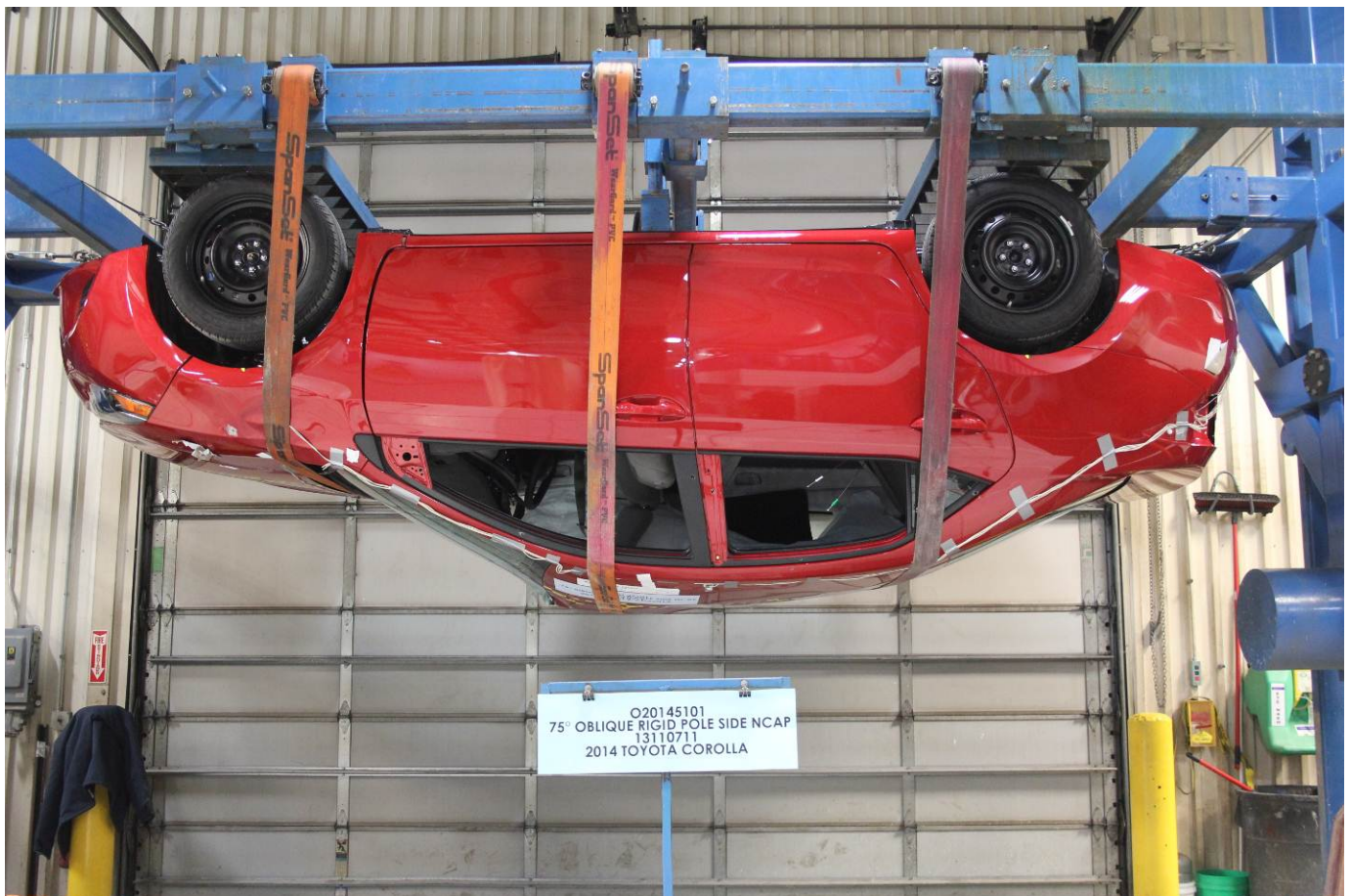
FMVSS No. 301 Static Rollover 180 Degrees
