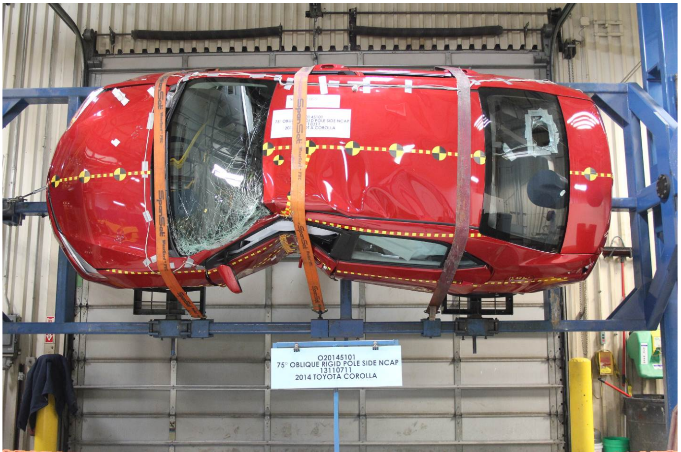
FMVSS No. 301 Static Rollover 90 Degrees
