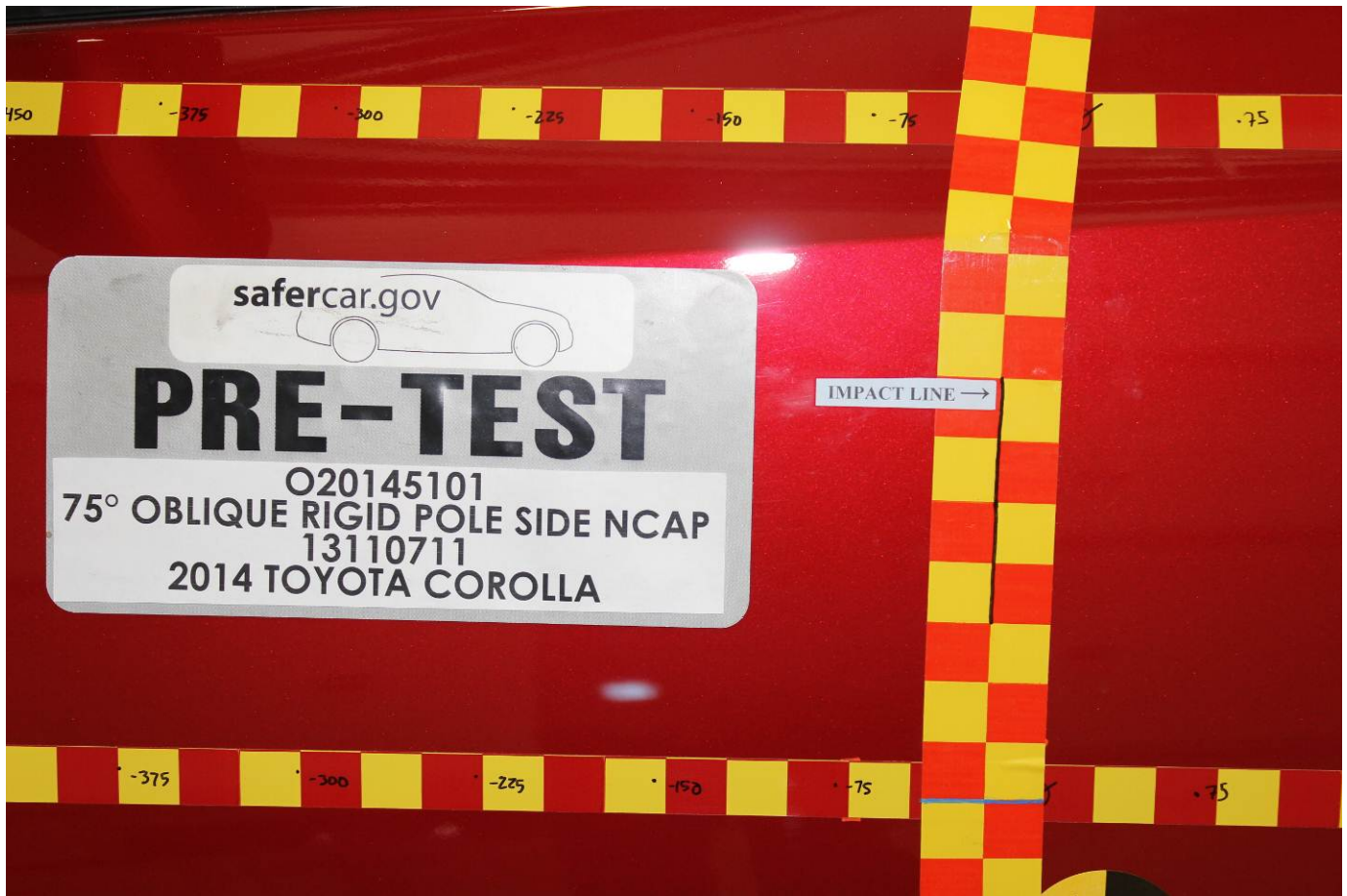
Pre-Test Close-Up View of Impact Point Target
