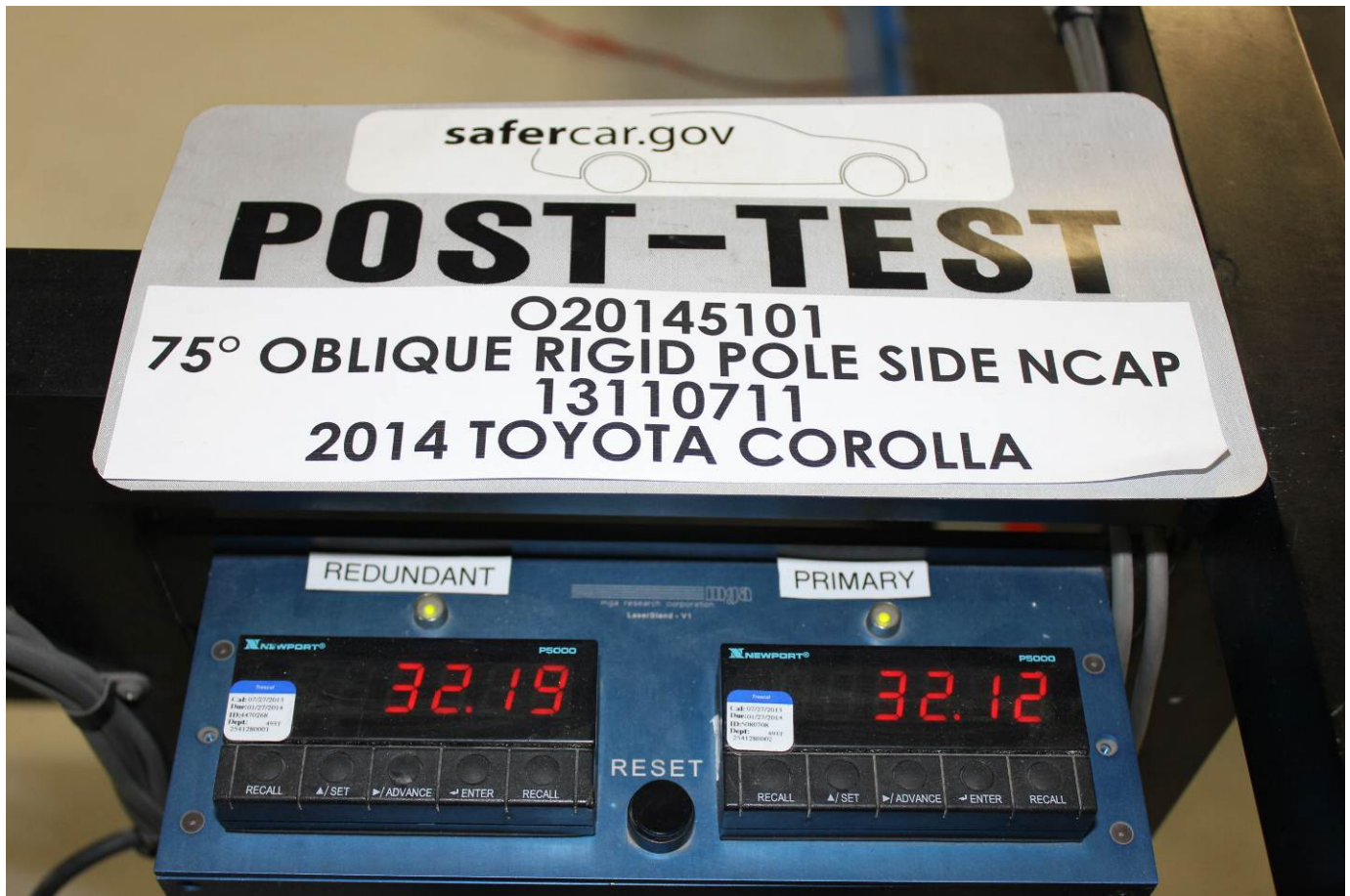
Post-Test Primary and Redundant Speed Trap Read-Out
