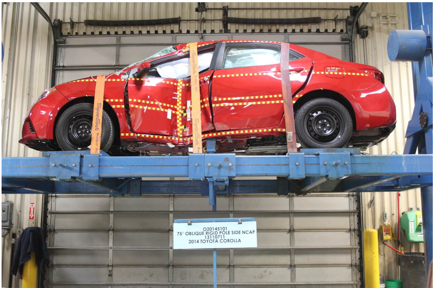
FMVSS No. 301 Static Rollover 0 Degrees
