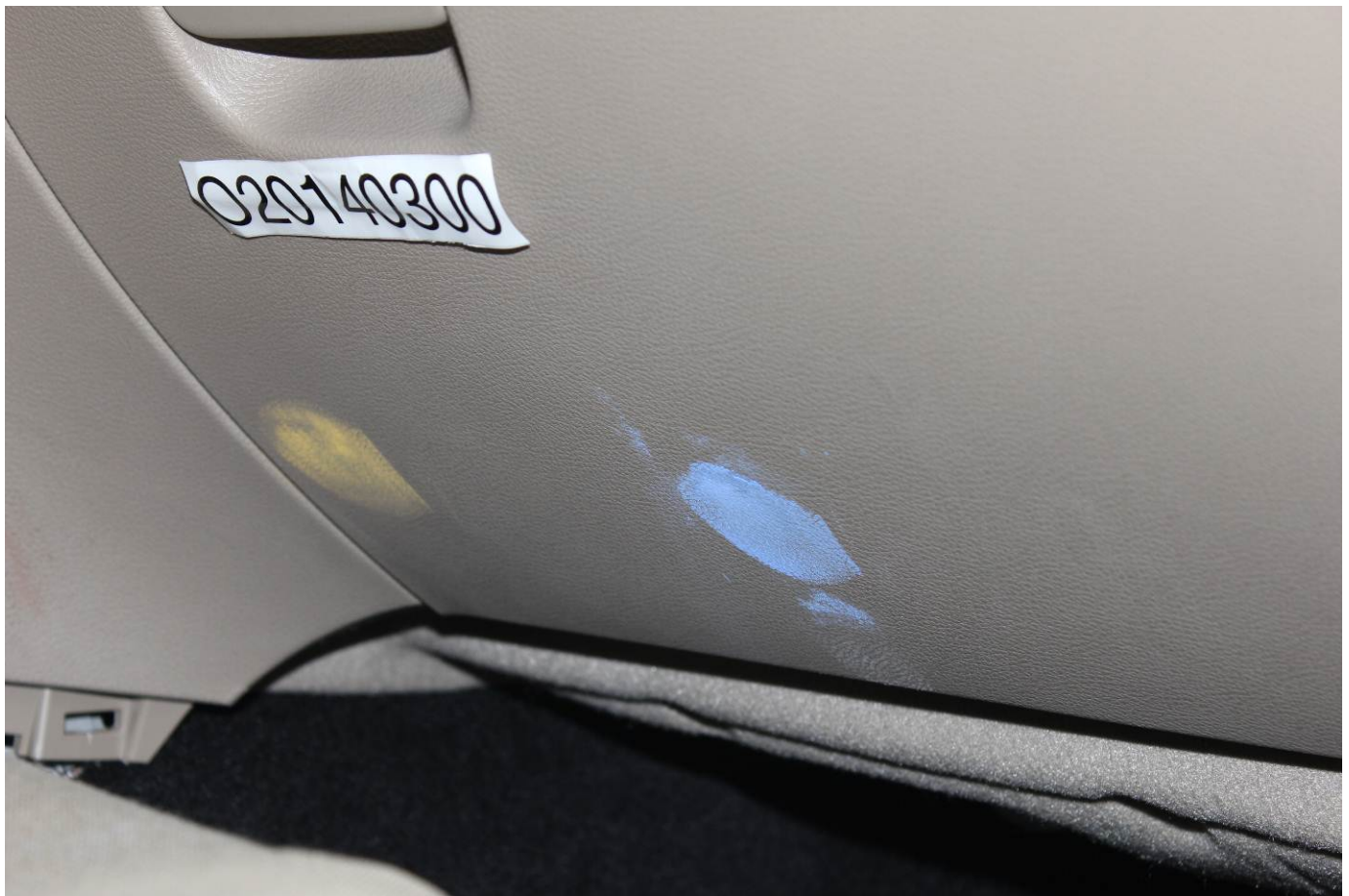
Post-Test Passenger Dummy Contact with Glovebox
