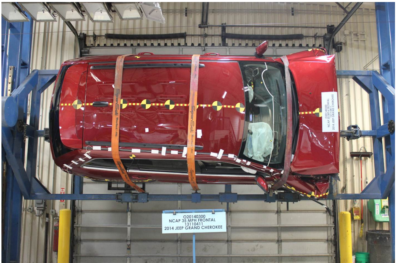
Vehicle at 270 Degree on Static Rollover Device
