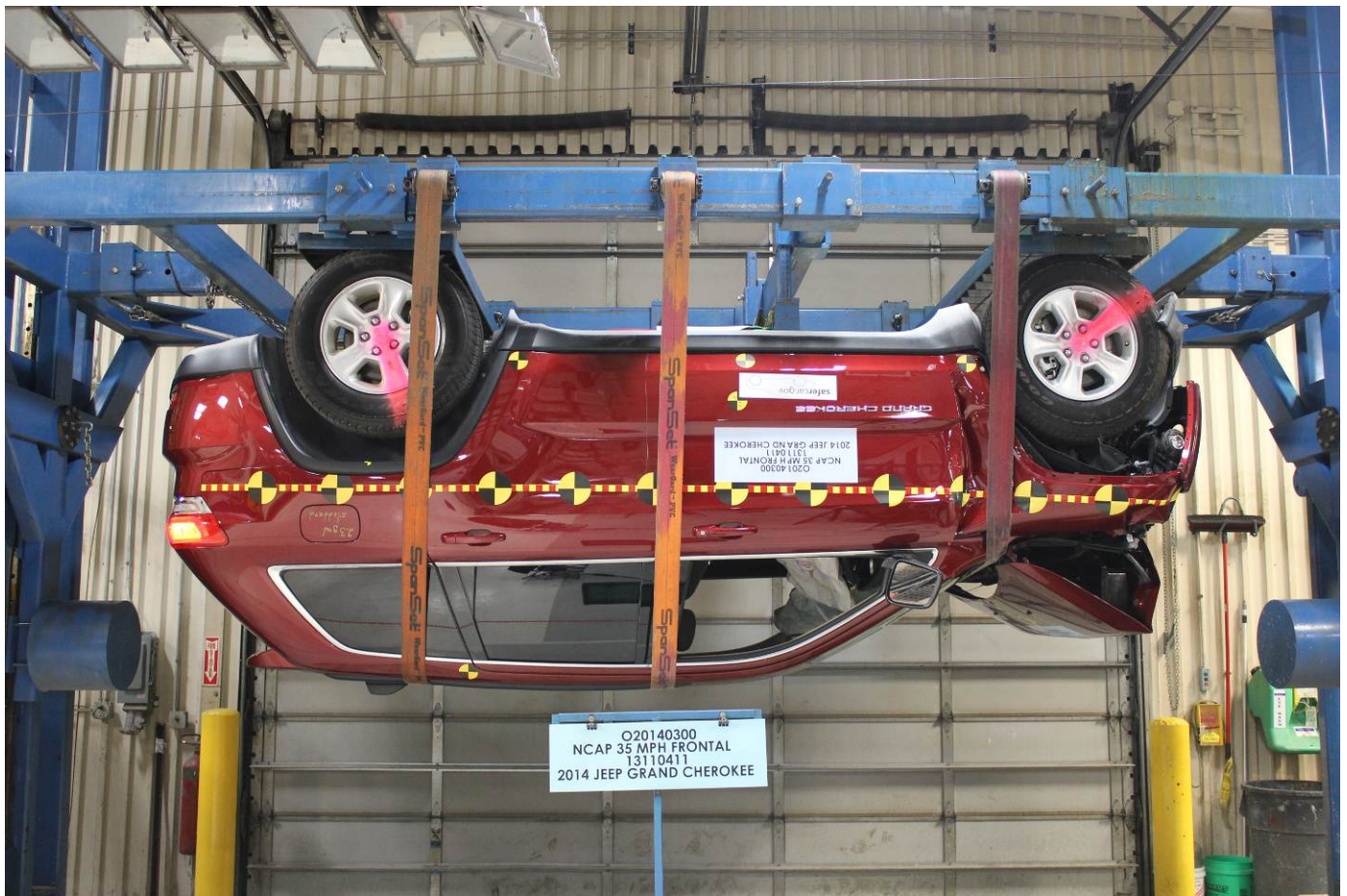
Vehicle at 180 Degrees on Static Rollover Device
