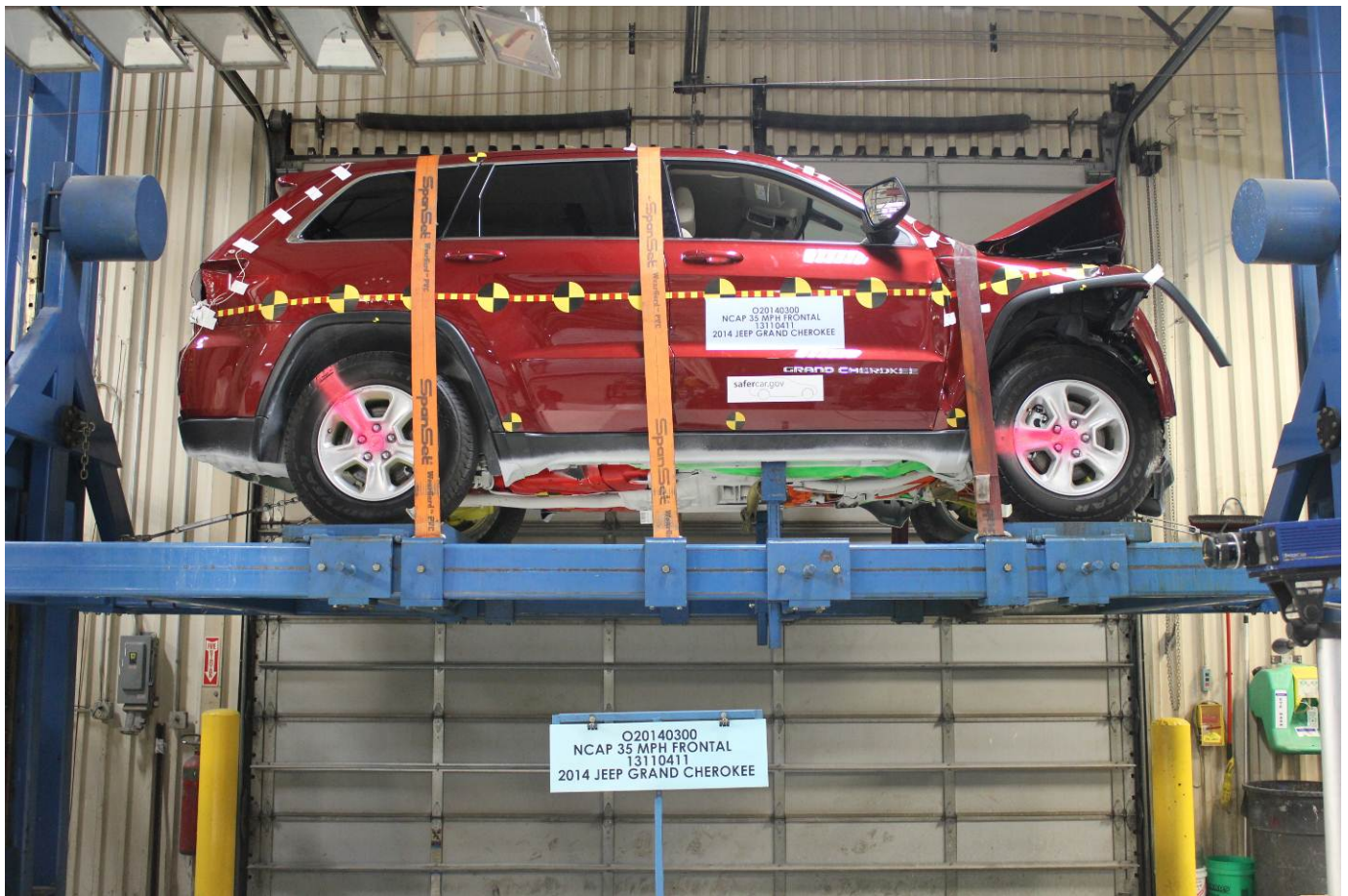
Vehicle at 0 Degree on Static Rollover Device
