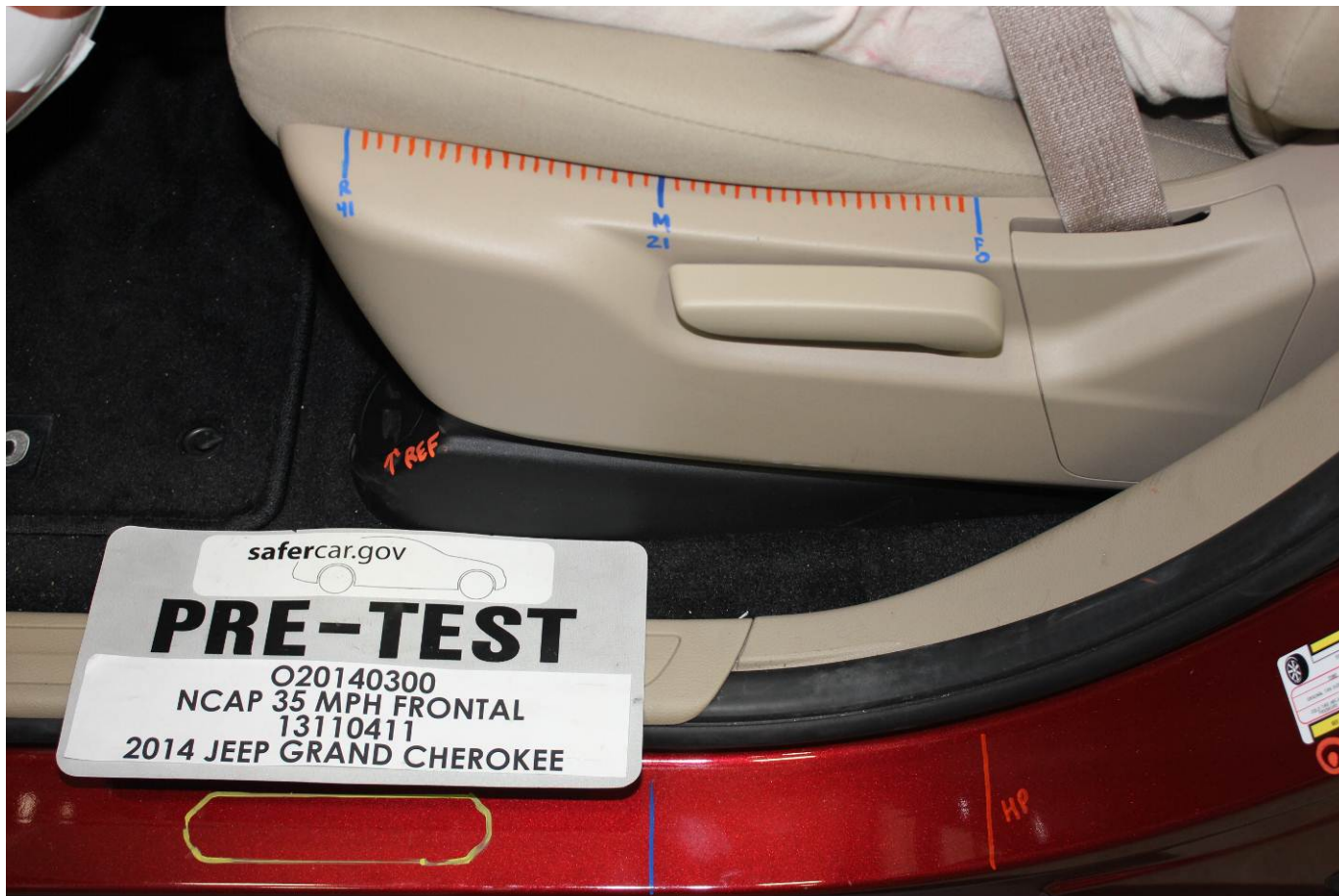
Pre-Test Driver's Seat Fore-Aft Markings
