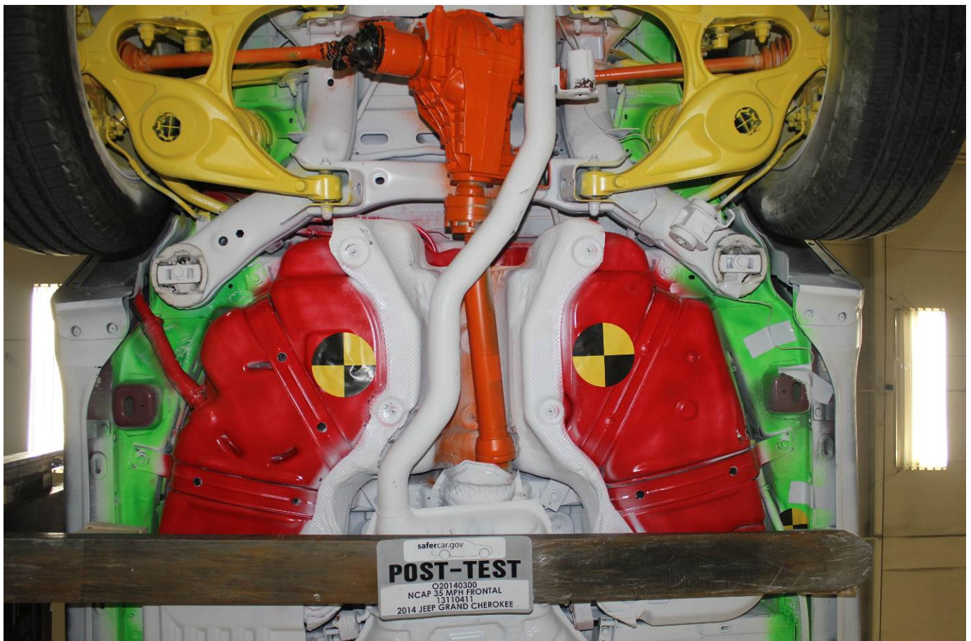
Post-Test Mid Rear Underbody View
