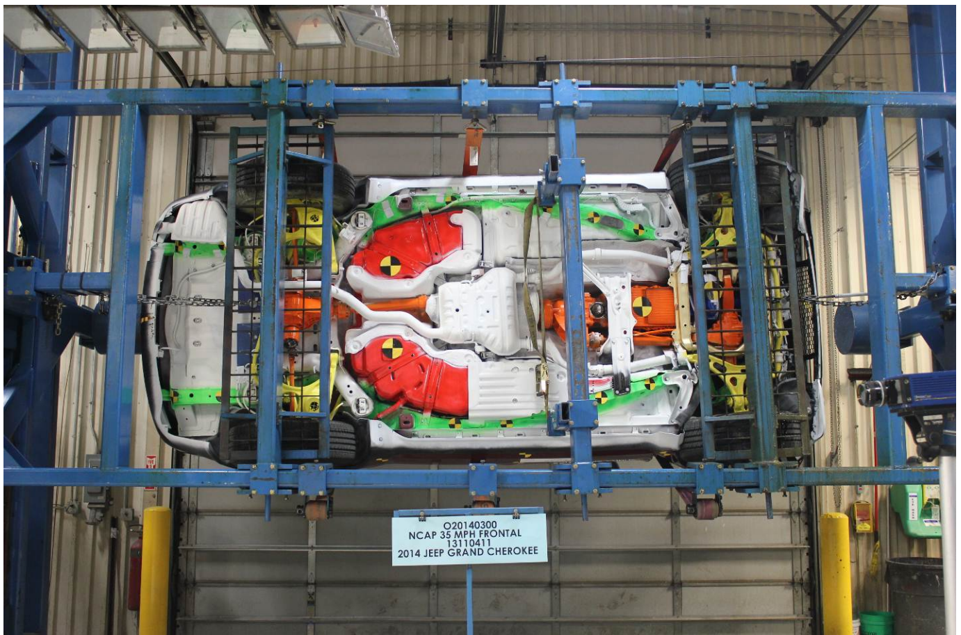
Vehicle at 90 Degrees on Static Rollover Device
