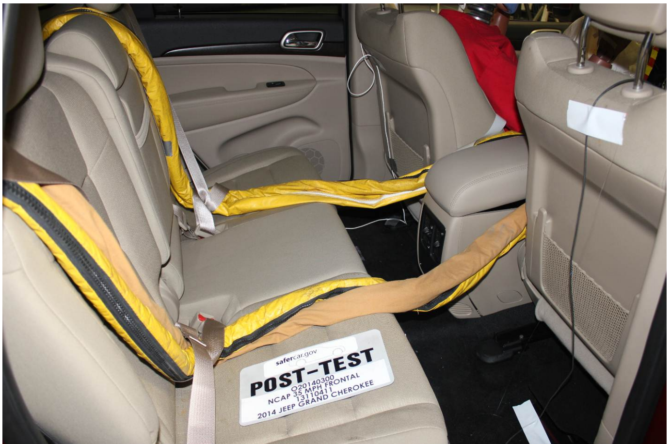
Post-Test Dummy Cable Routing
