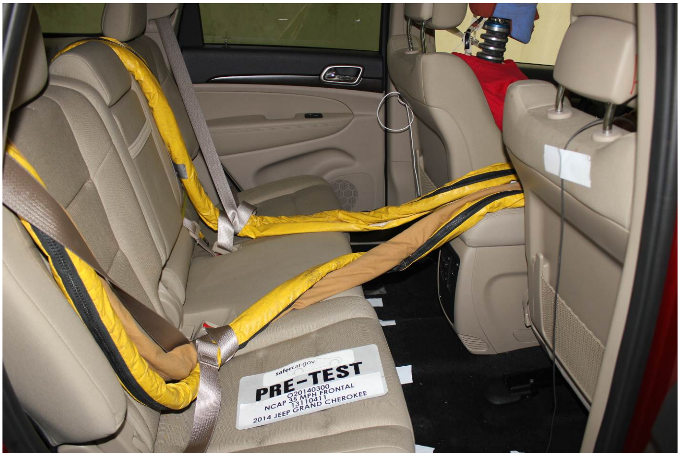
Pre-Test Dummy Cable Routing
