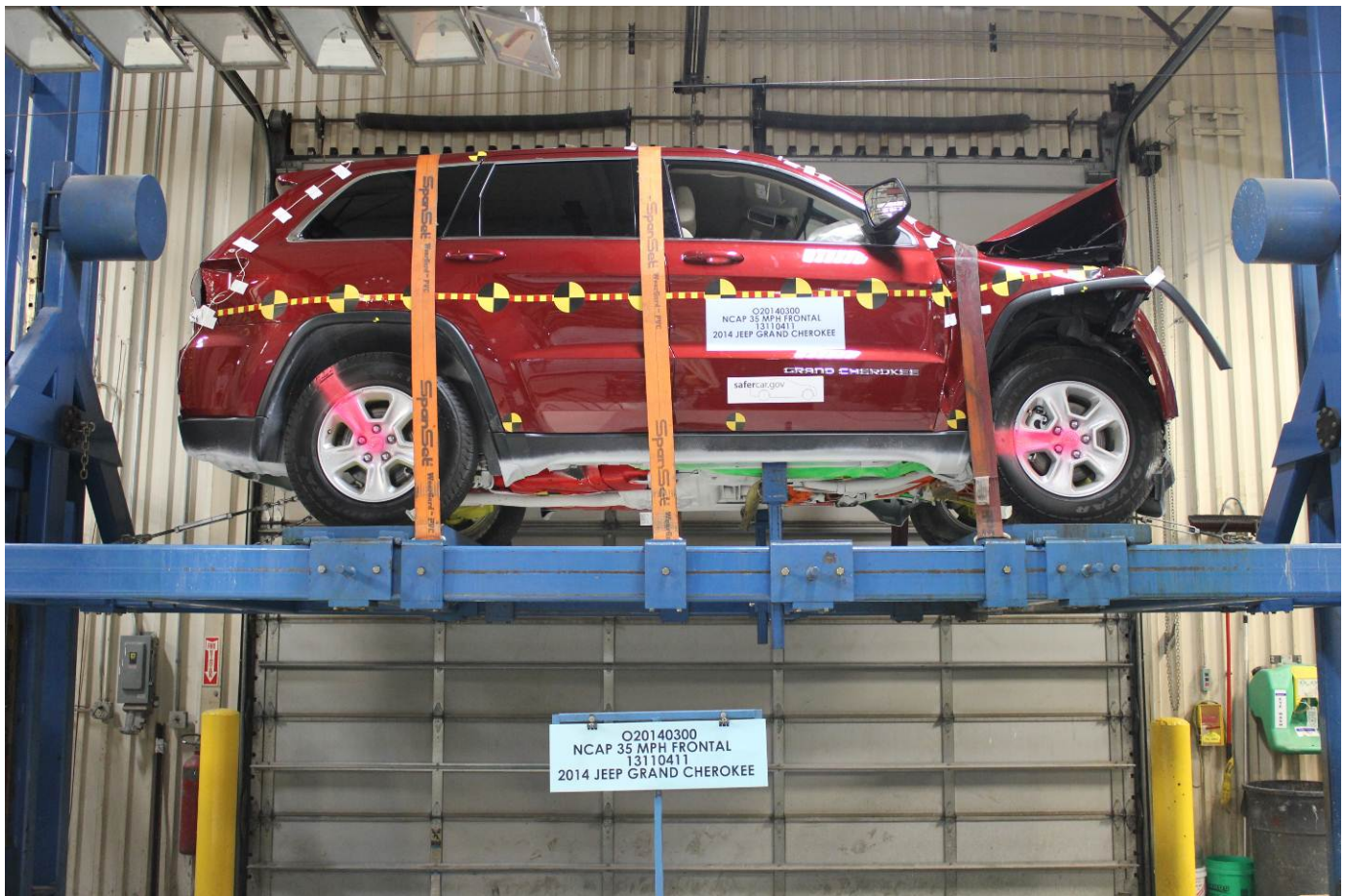
Vehicle at 360 Degrees on Static Rollover Device
