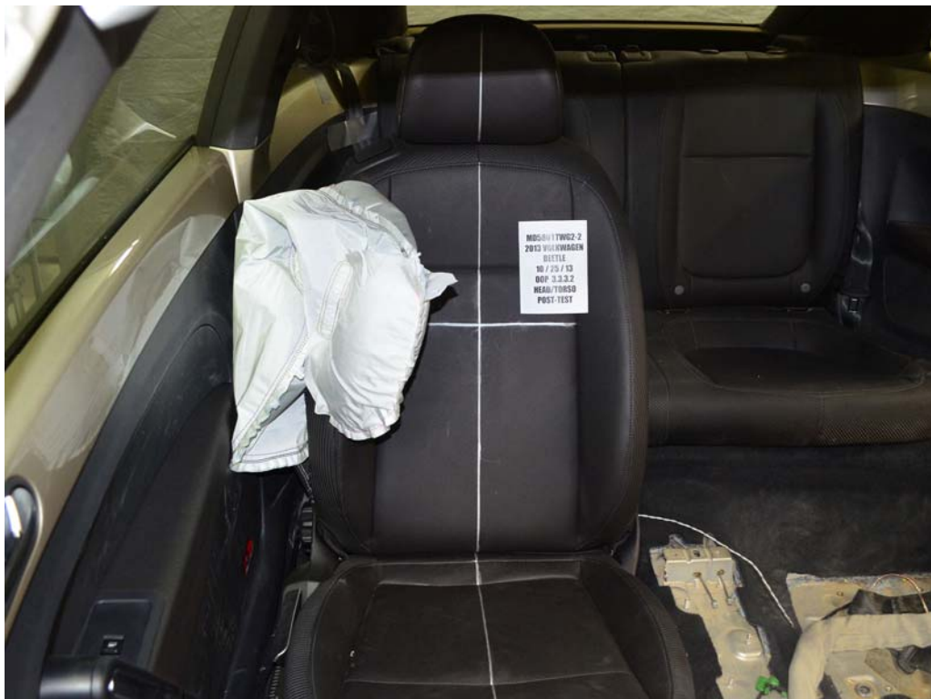
FIGURE 12. Post-Test Dummy Position, Front View
