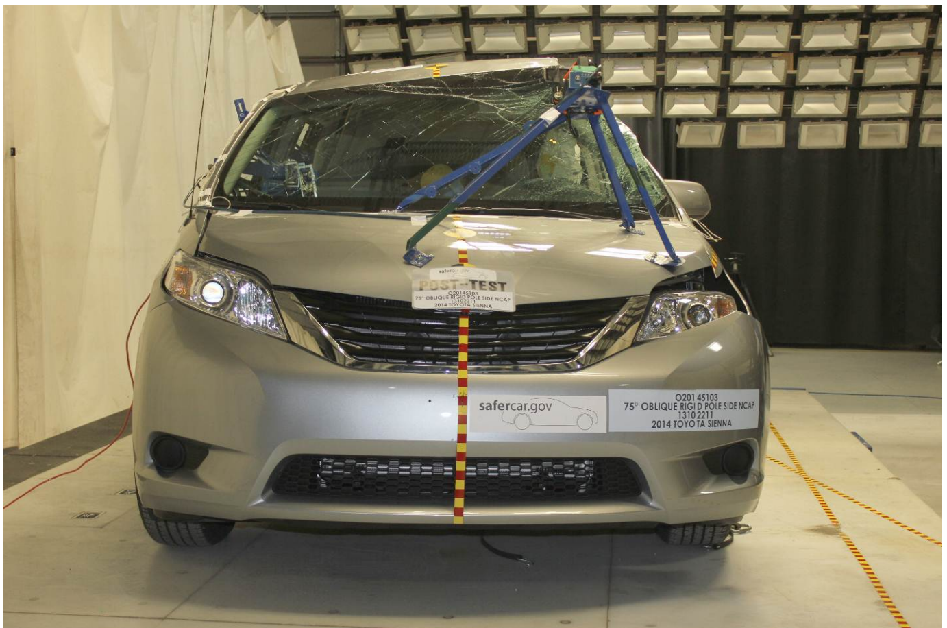
Post-Test Frontal View of Test Vehicle
