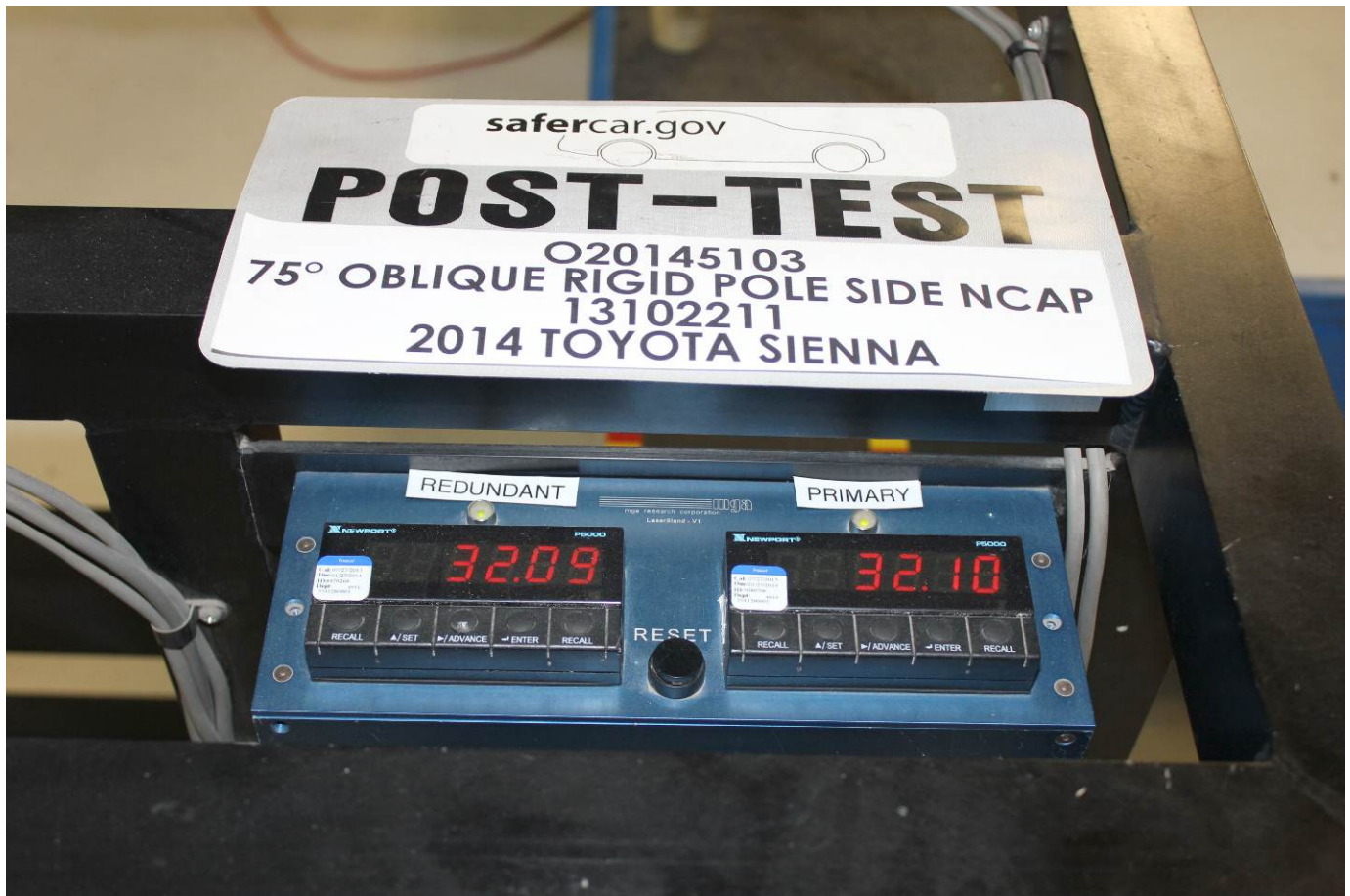
Post-Test Primary and Redundant Speed Trap Read-Out
