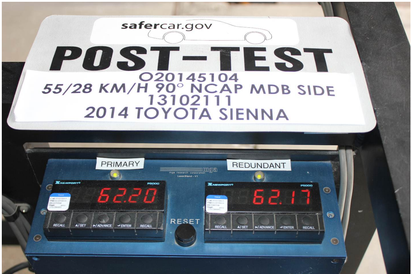
Post-Test Primary and Redundant Speed Trap Read-Out
