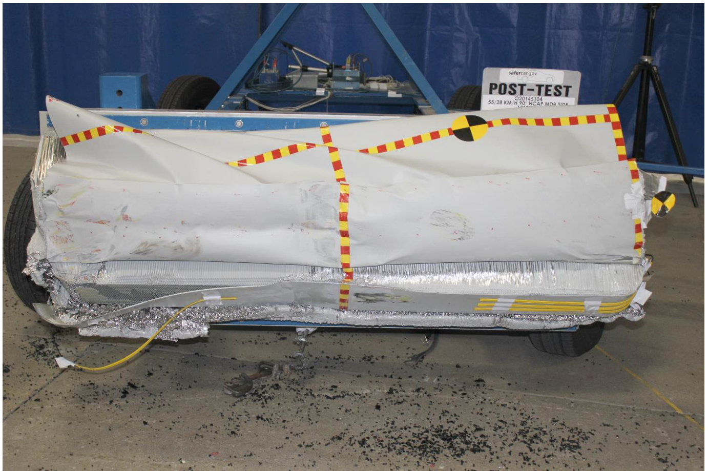
Post-Test Front View of MDB Impactor Face
