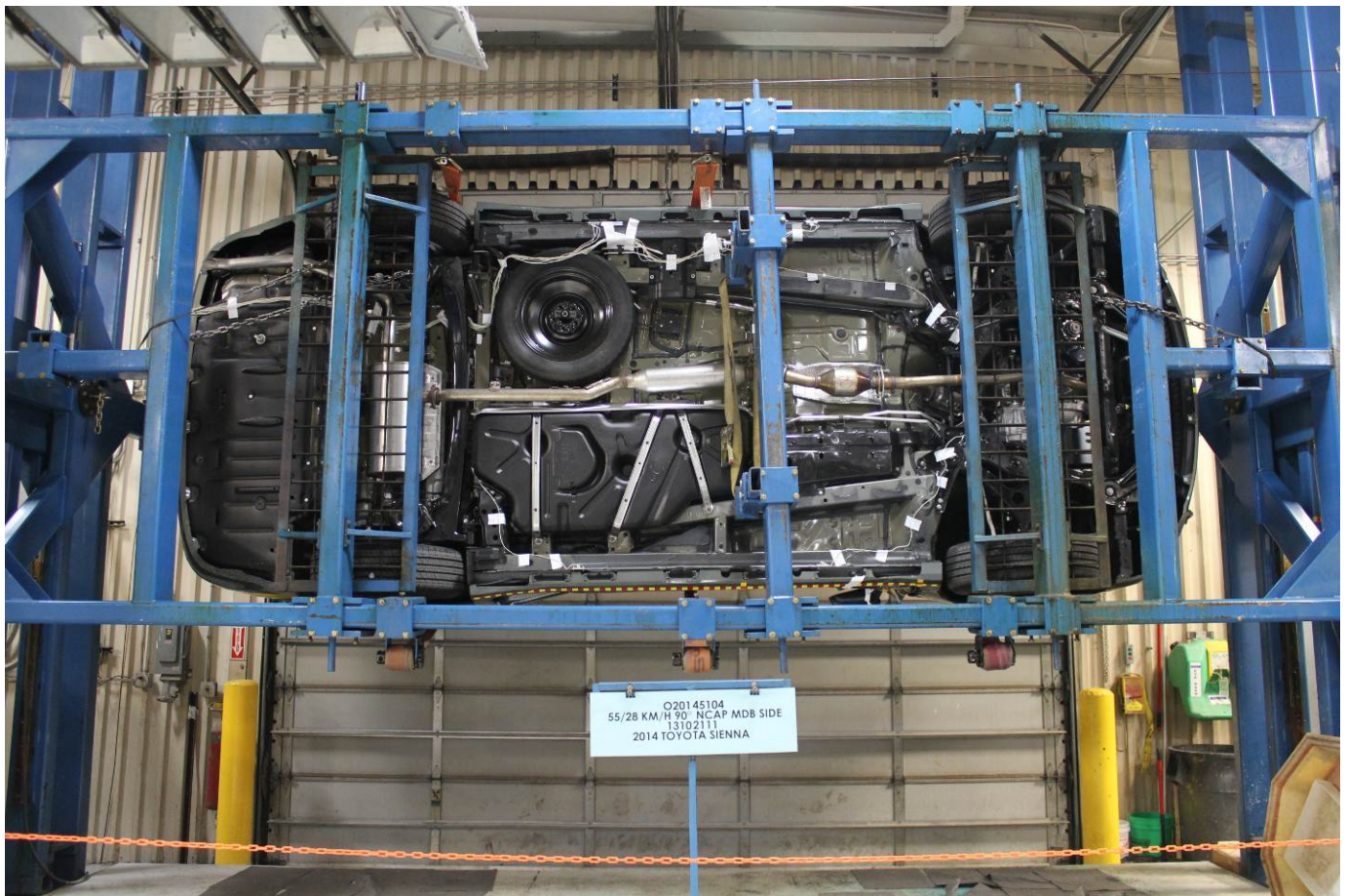
FMVSS No. 301 Static Rollover 90 Degrees
