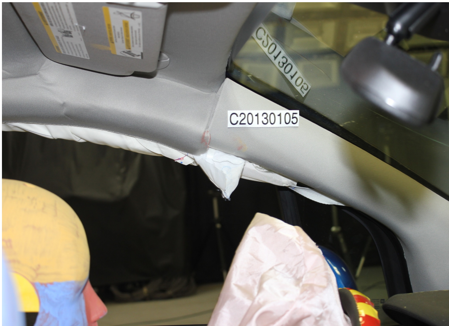
Post-Test Driver Dummy Head Contact (A-pillar)
