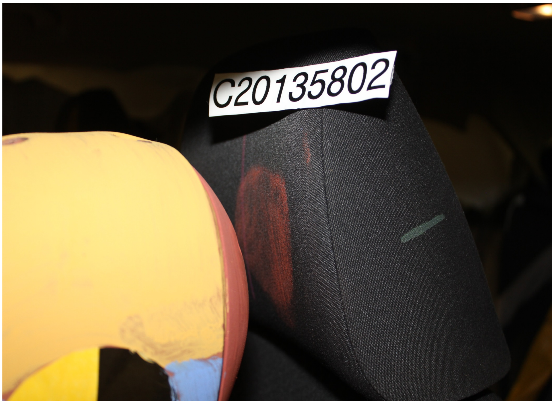
Post-Test Driver Dummy Head Contact (headrest)
