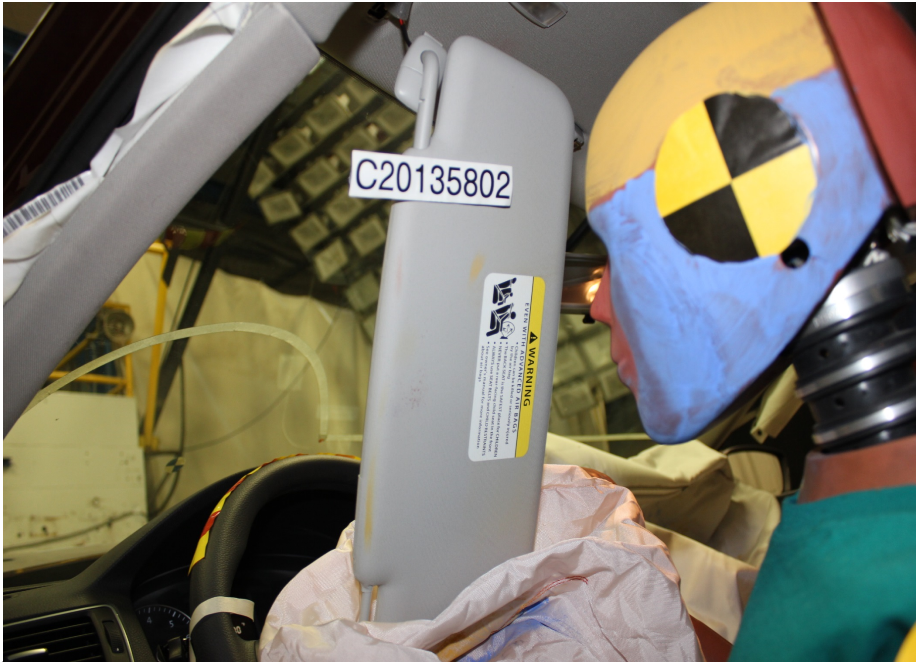
Post-Test Driver Dummy Head Contact (visor)
