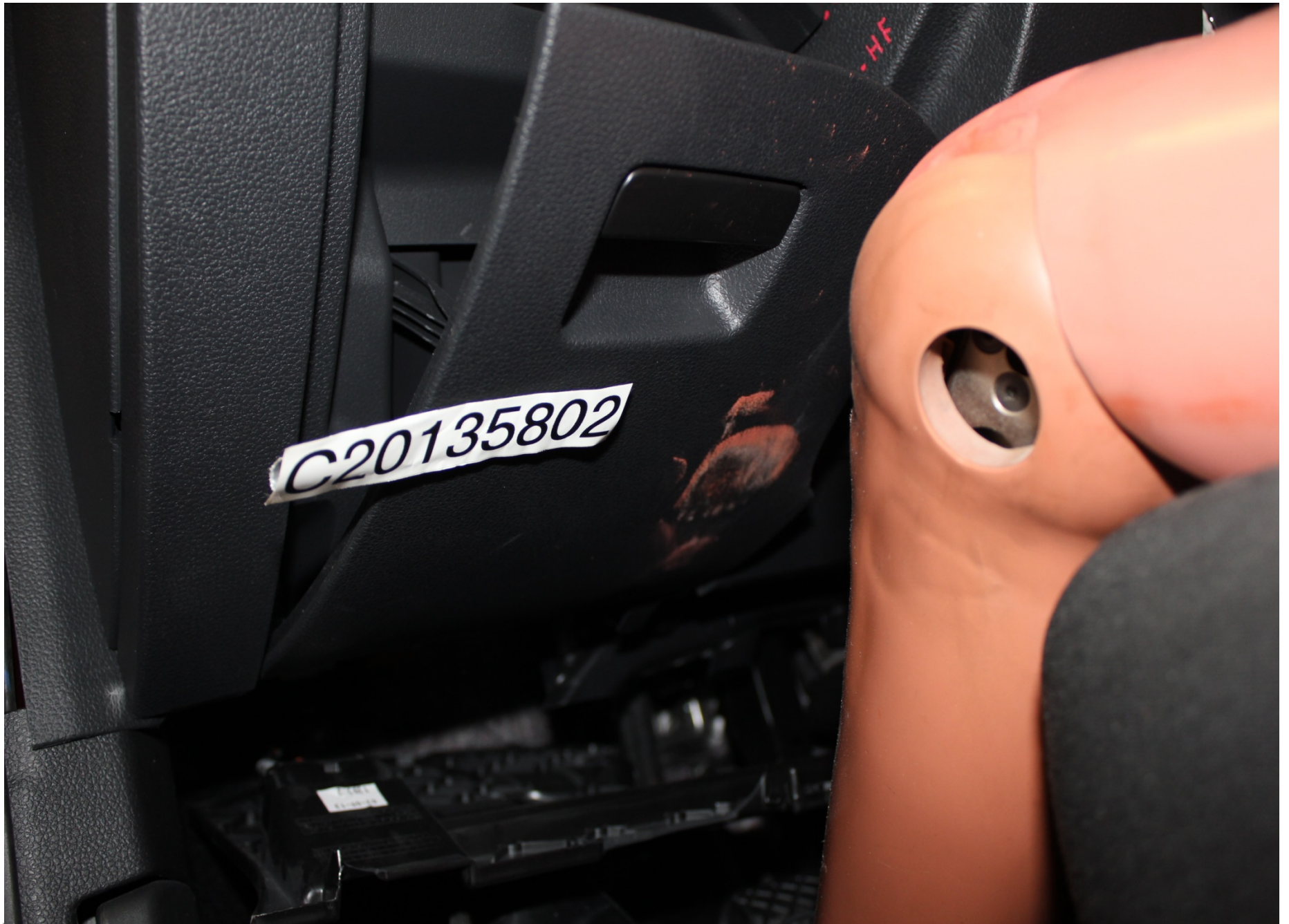
Post-Test Driver Dummy Knee Contact
