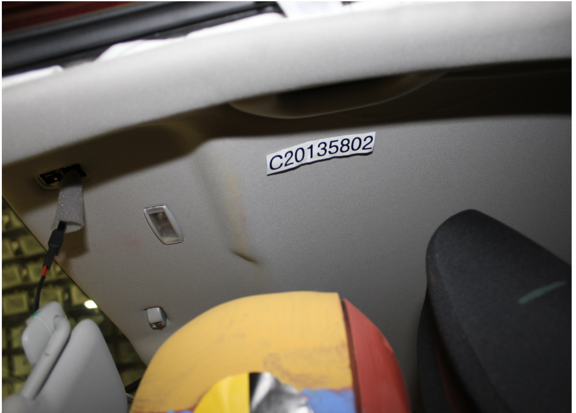
Post-Test Driver Dummy Head Contact (roof)
