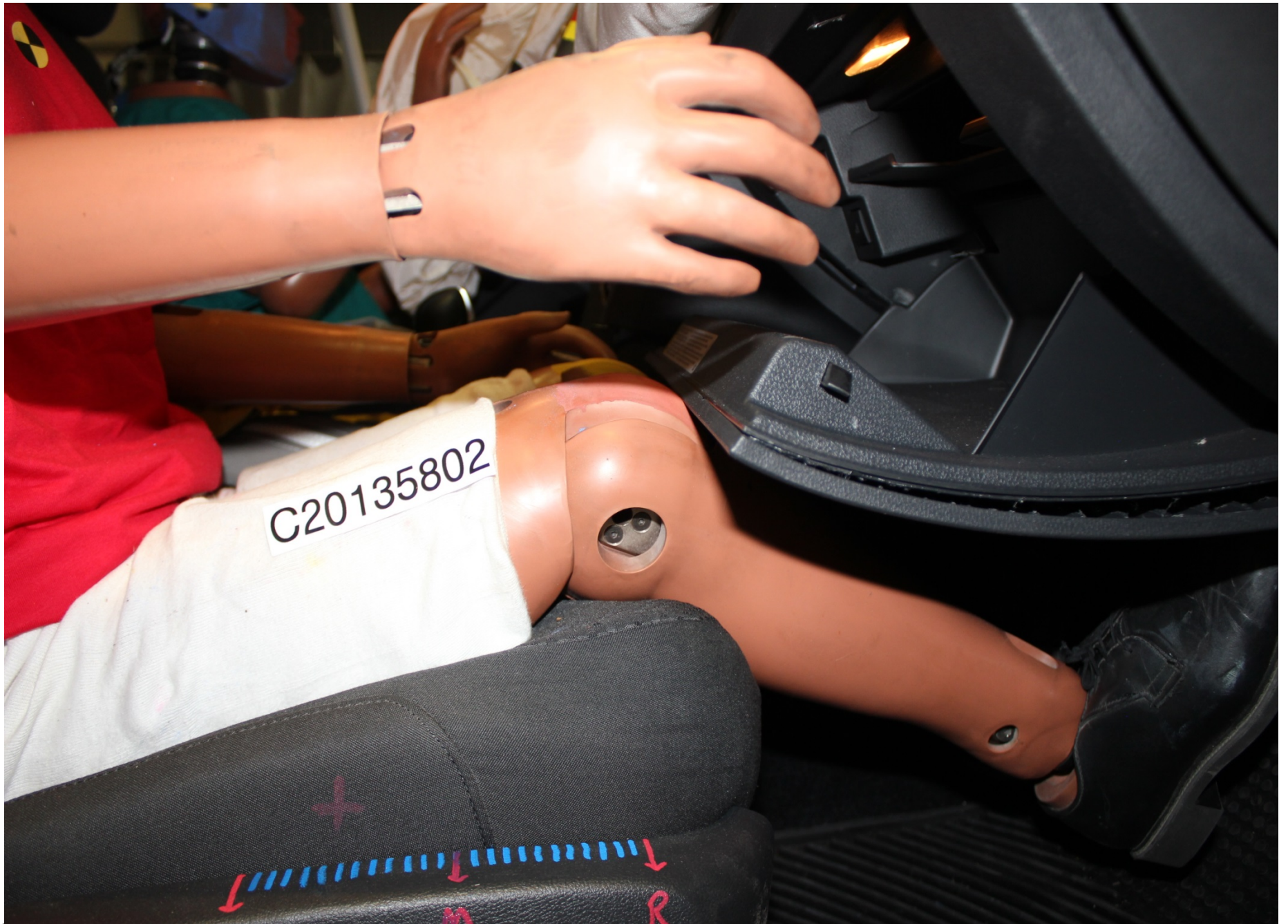
Post-Test Passenger Side Knee Bolster View
