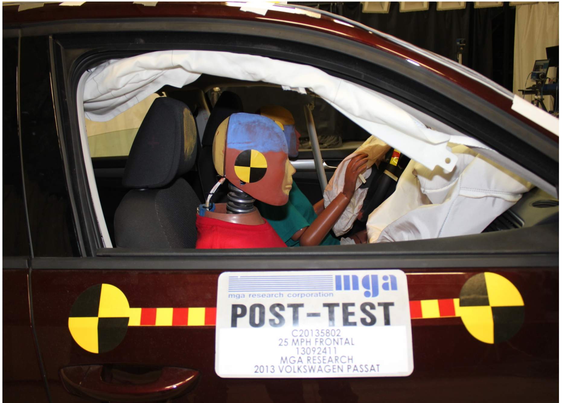
Post-Test Passenger Dummy Position Right Side View
