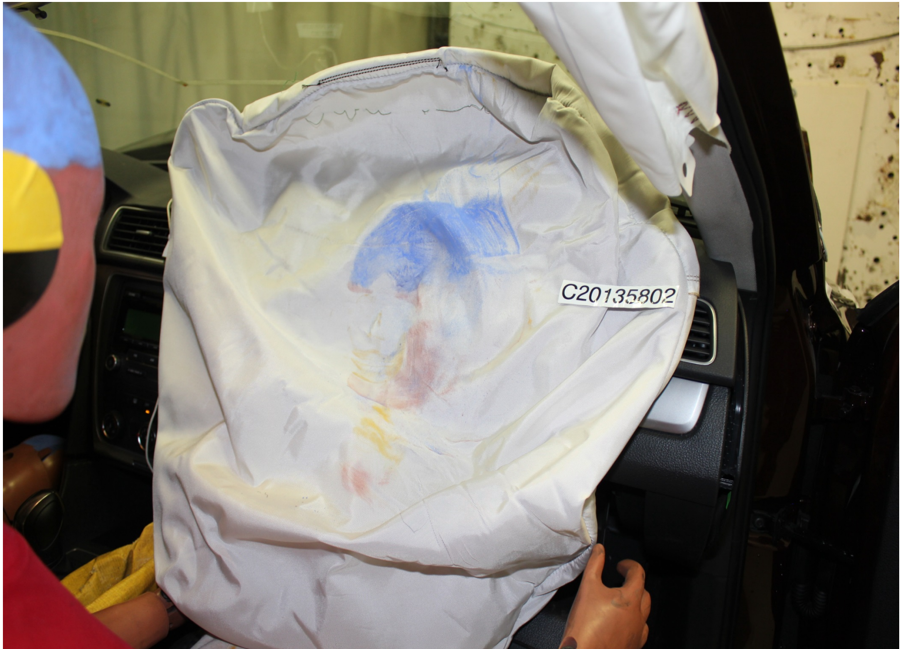
Post-Test Passenger Dummy Airbag Contact
