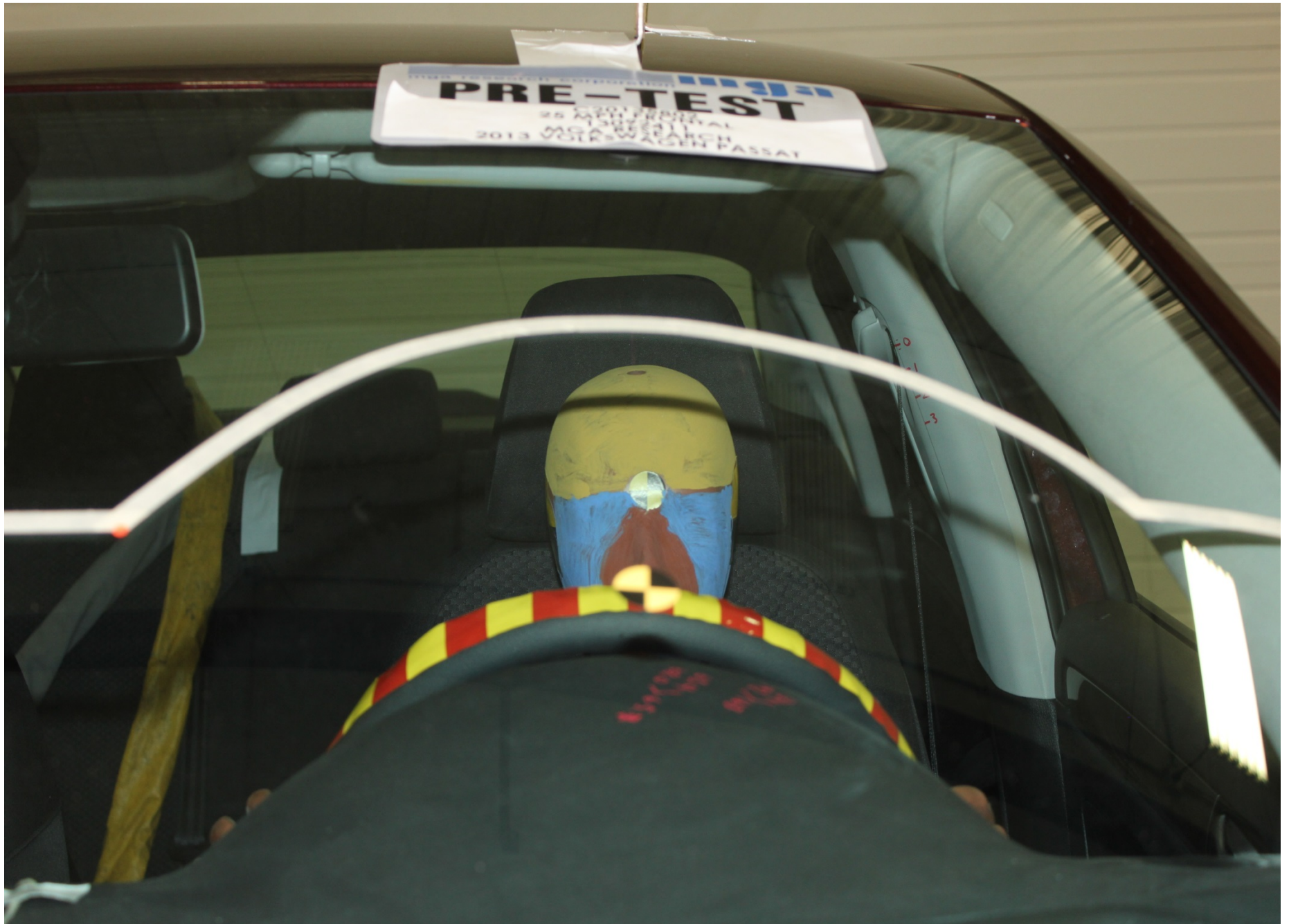
Pre-Test Driver Dummy Front View (head position)
