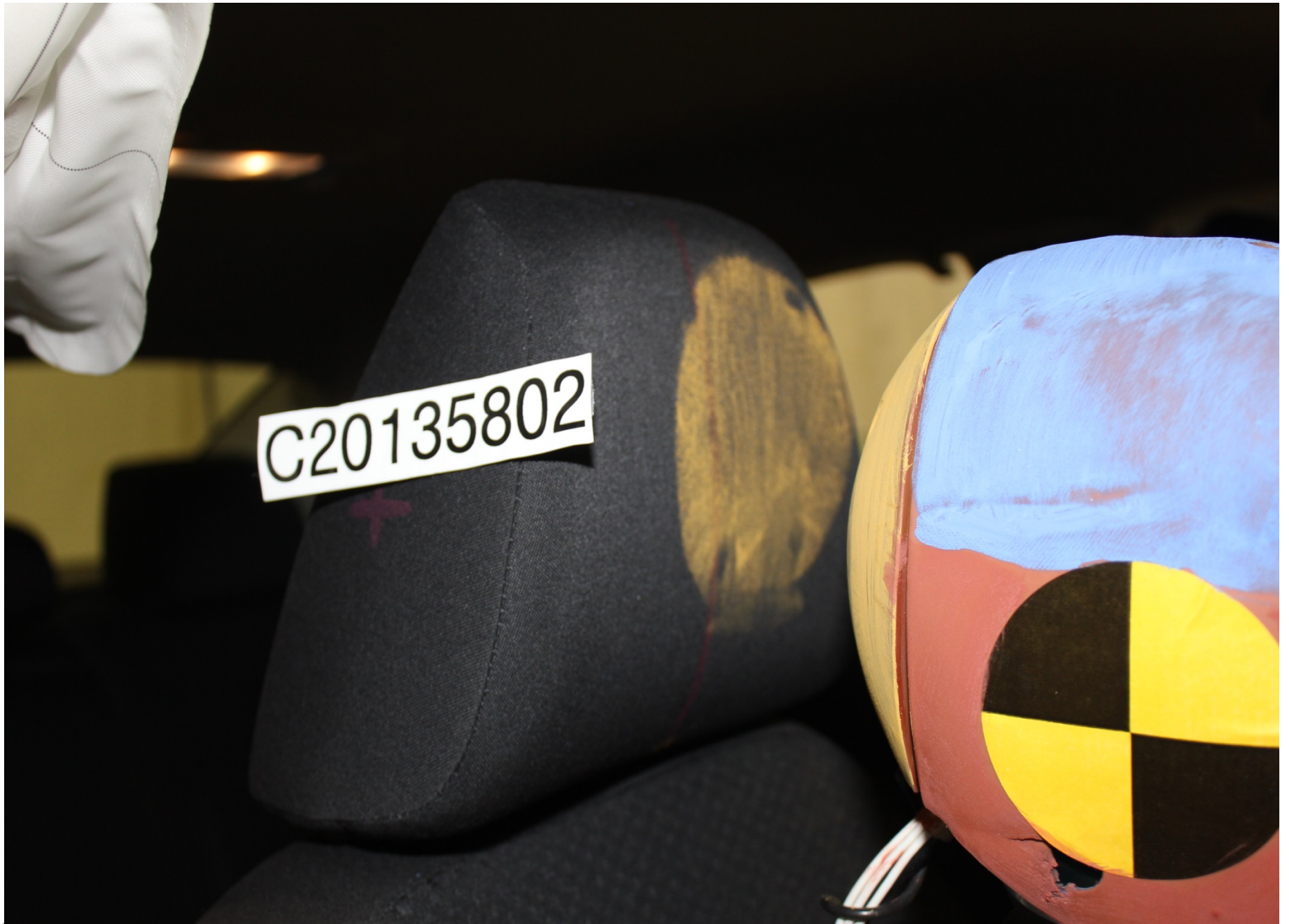
Post-Test Passenger Dummy Head Contact (headrest)
