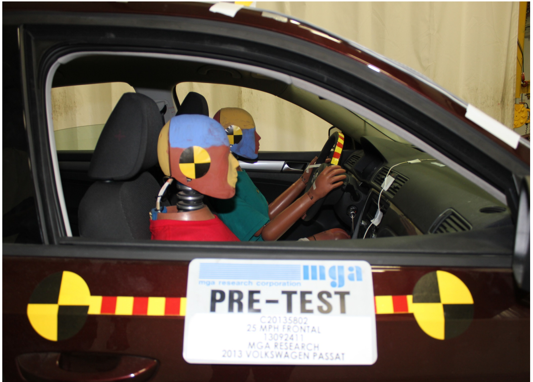
Pre-Test Passenger Dummy Position Right Side View
