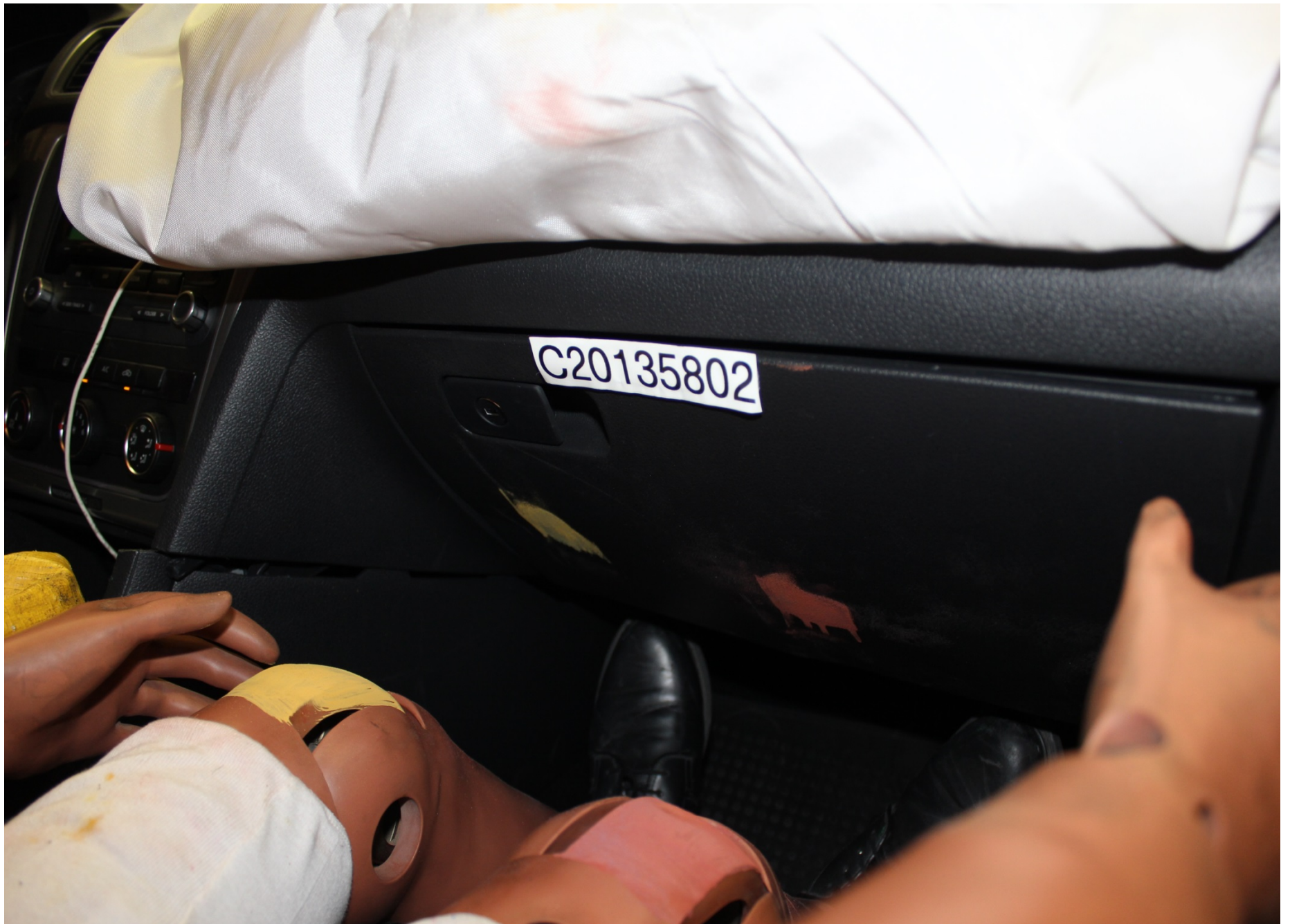
Post-Test Passenger Dummy Knee Contact
