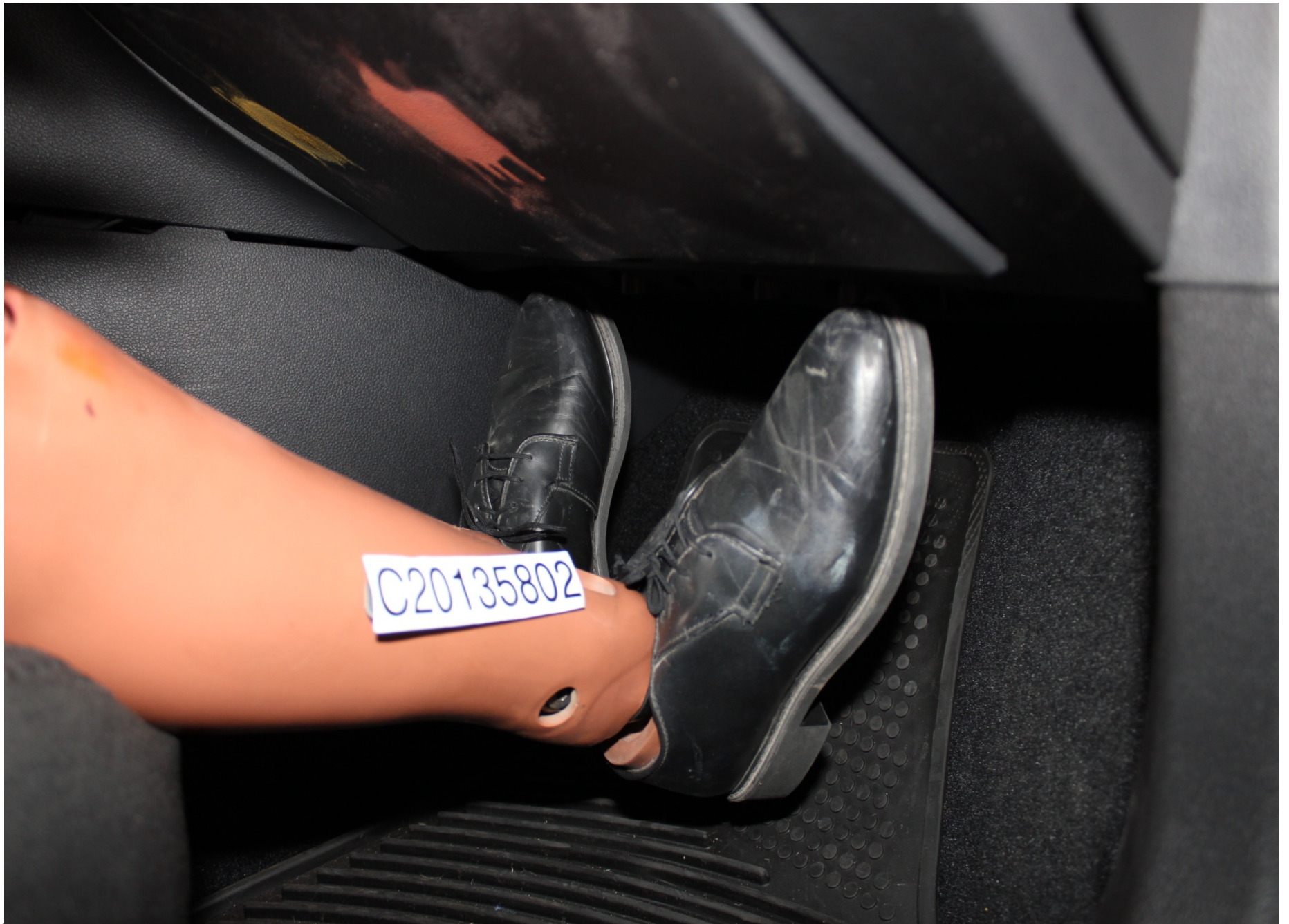
Post-Test Passenger Dummy Feet Position
