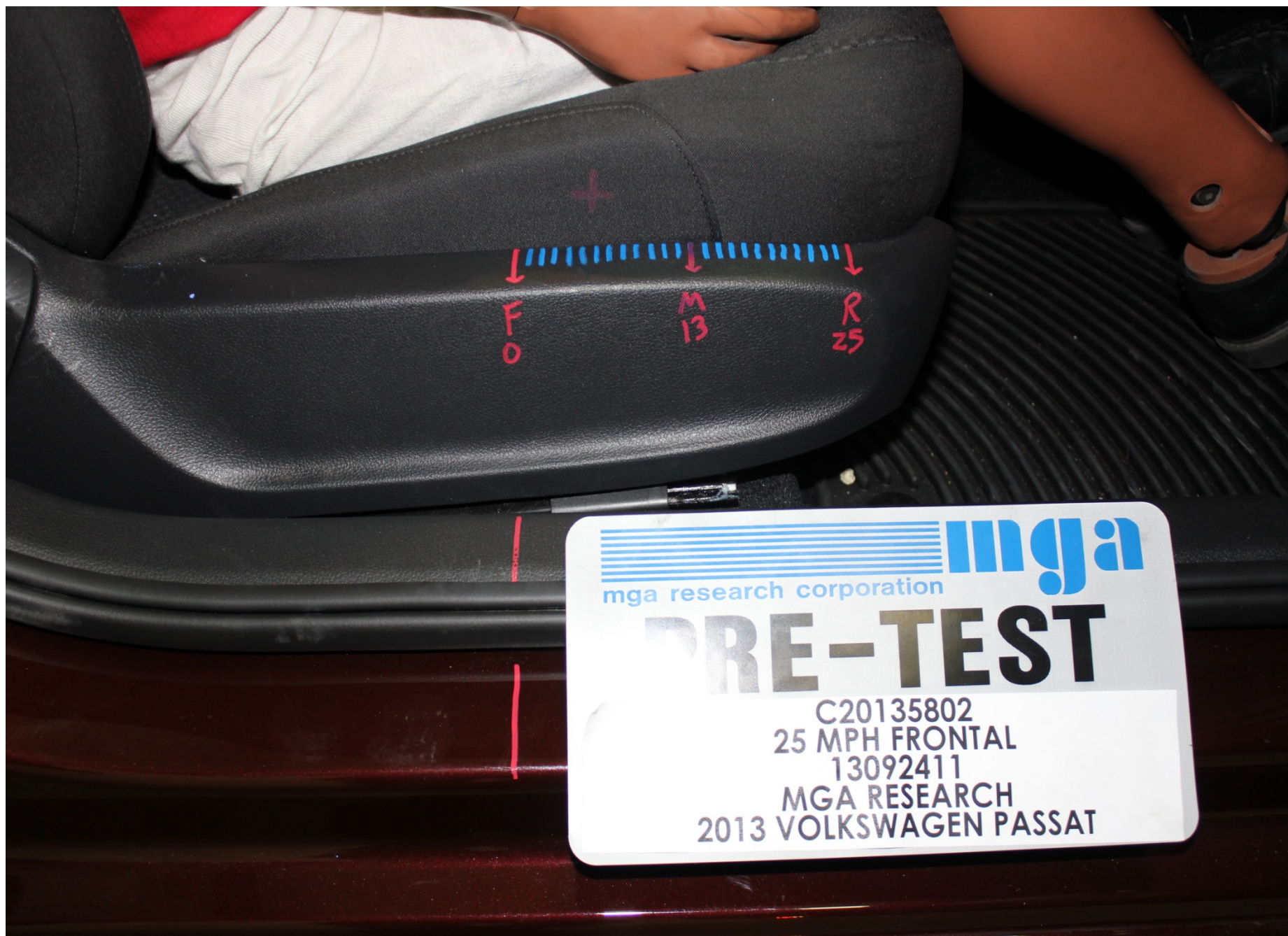
Pre-Test Passenger Dummy Seat Position
