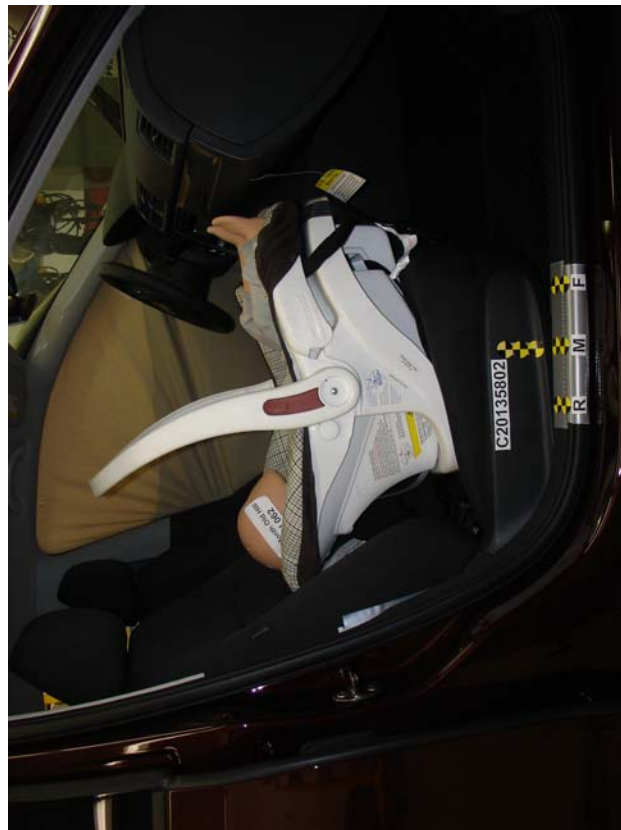
Cosco Arriva WBBase, Unbelted, Forward Facing, Middle Seat Track
