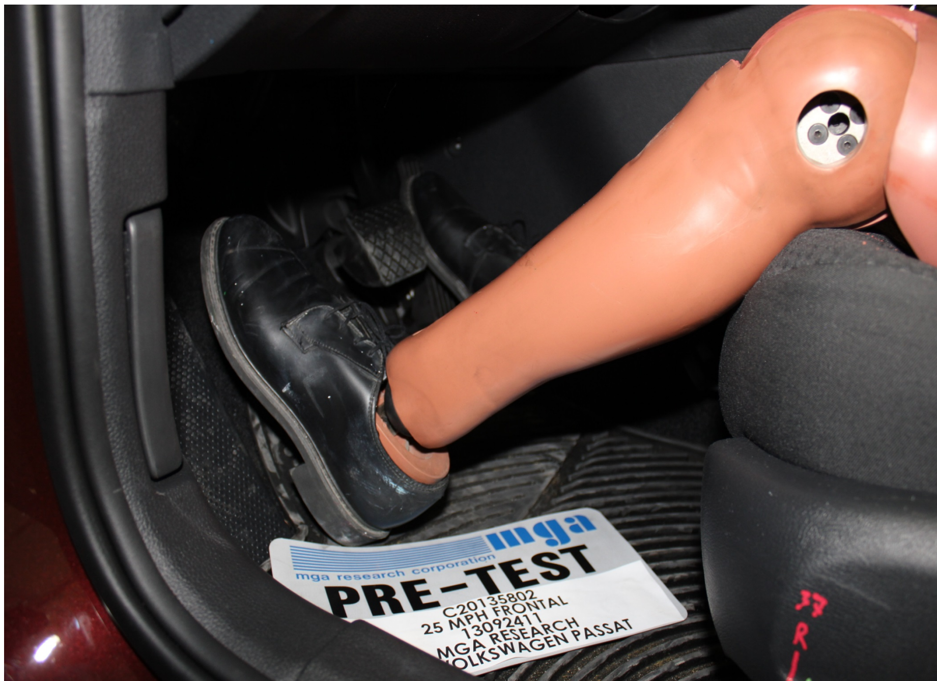
Pre-Test Driver Dummy Feet Position
