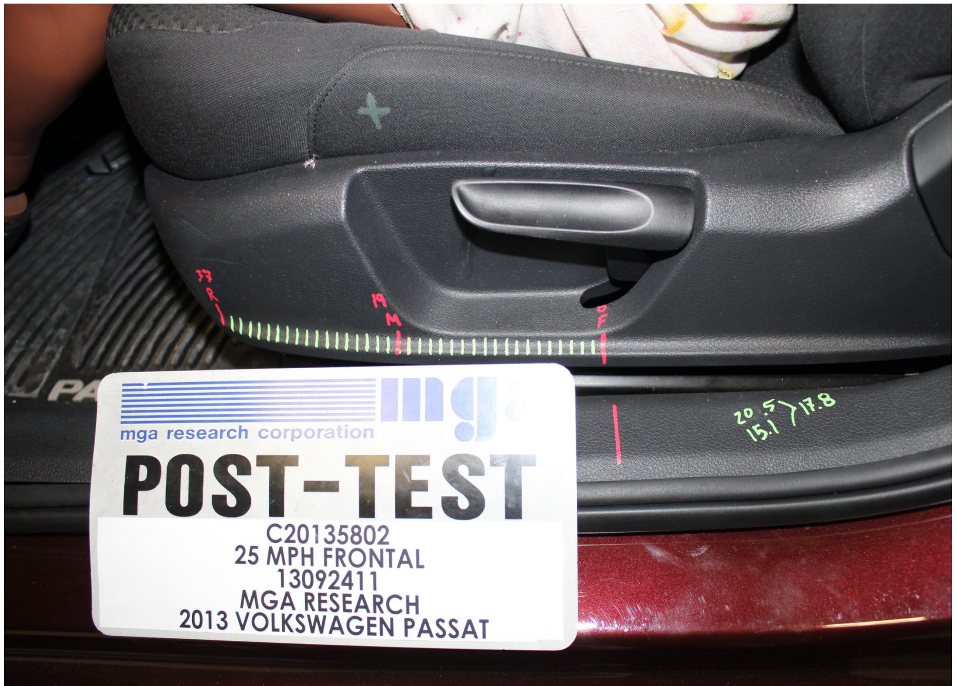
Post-Test Driver Dummy Seat Position
