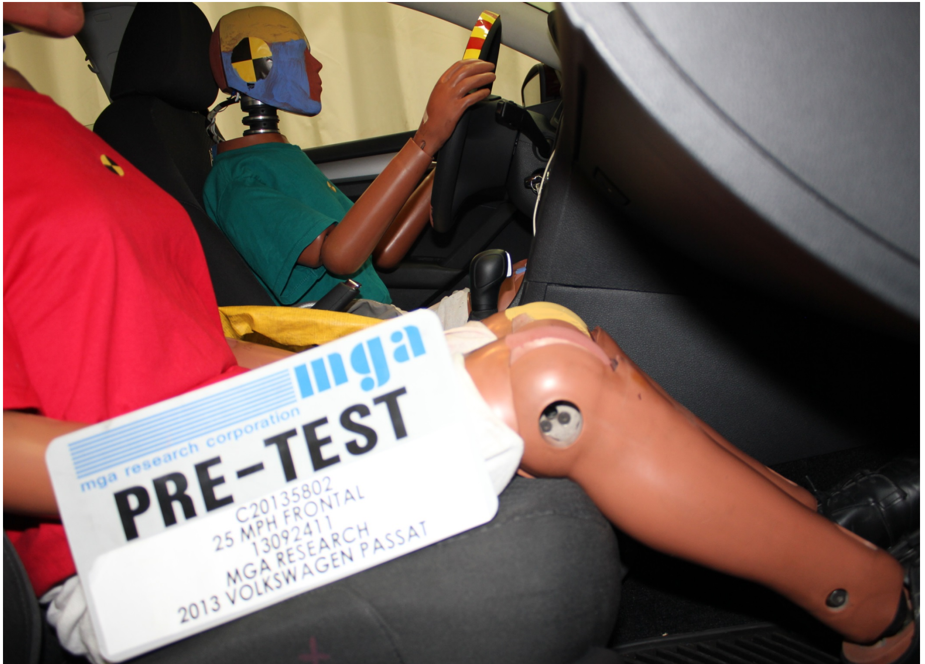
Pre-Test Passenger Side Knee Bolster View
