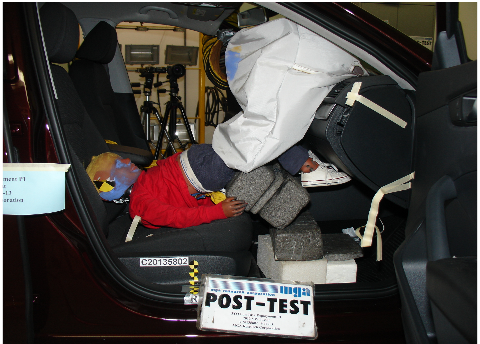
Post-Test 3YO P1 Passenger Dummy Right Side View
