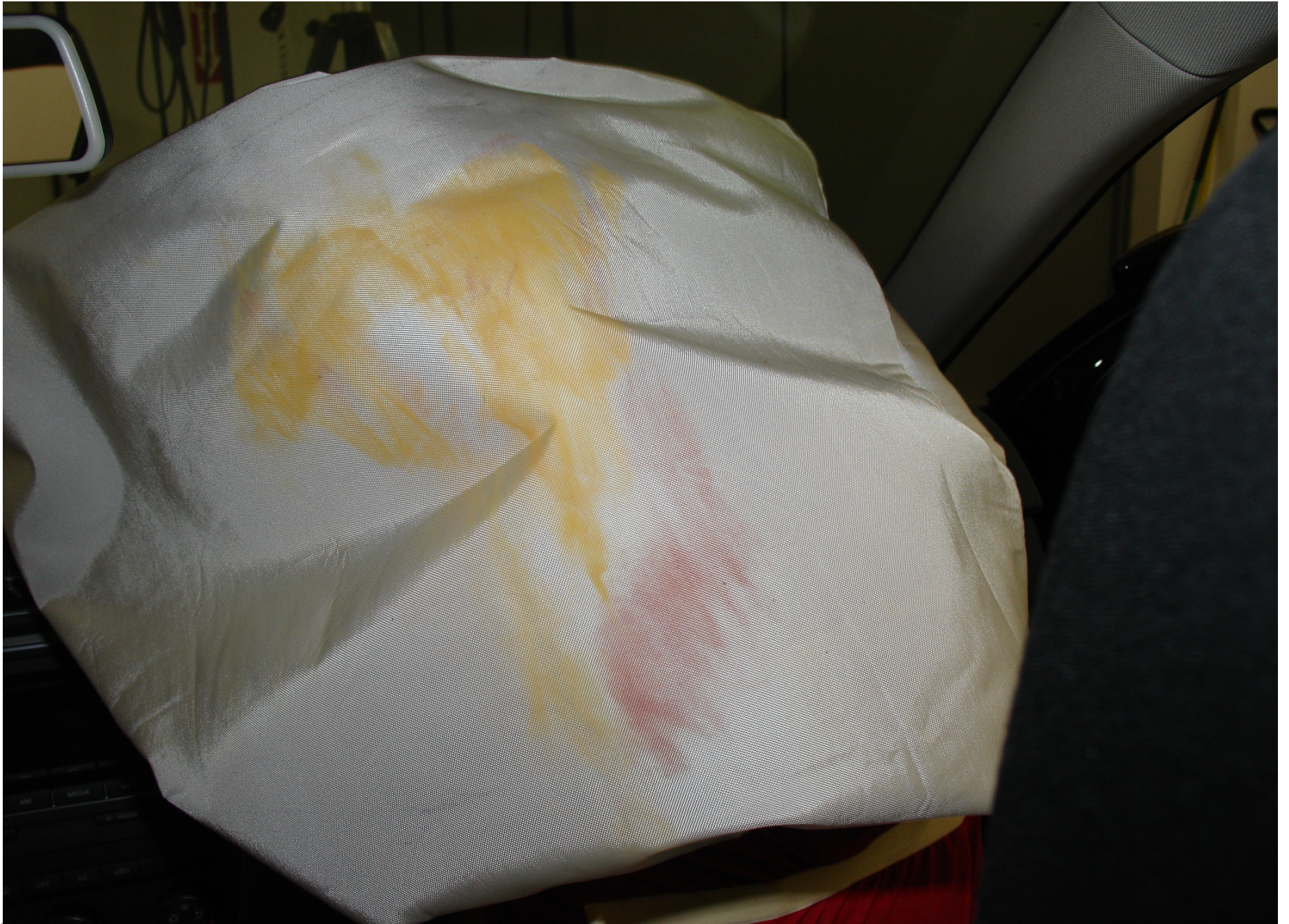
Post-Test 6YO P2 Passenger Dummy Airbag Left Side View
