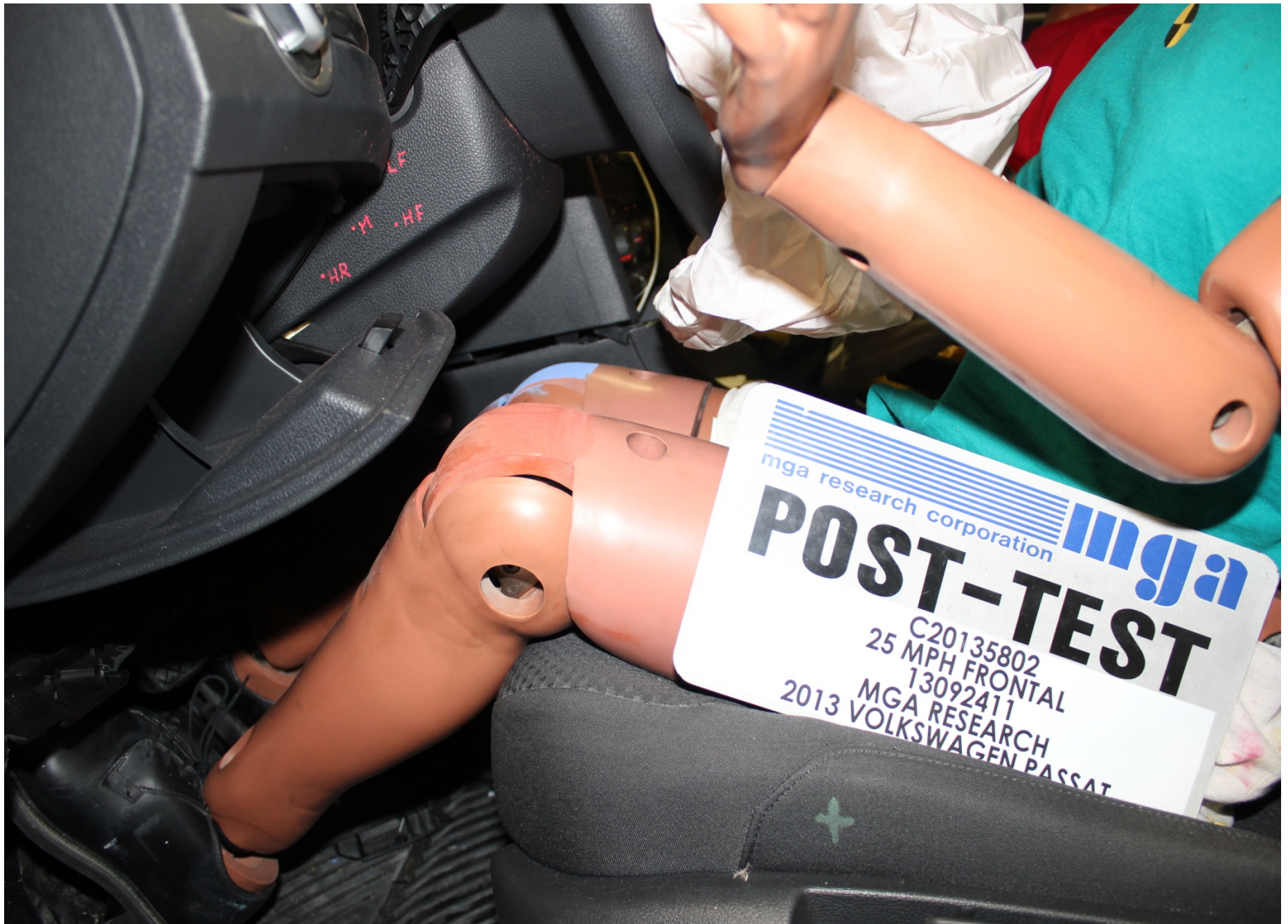
Post-Test Driver Side Knee Bolster View
