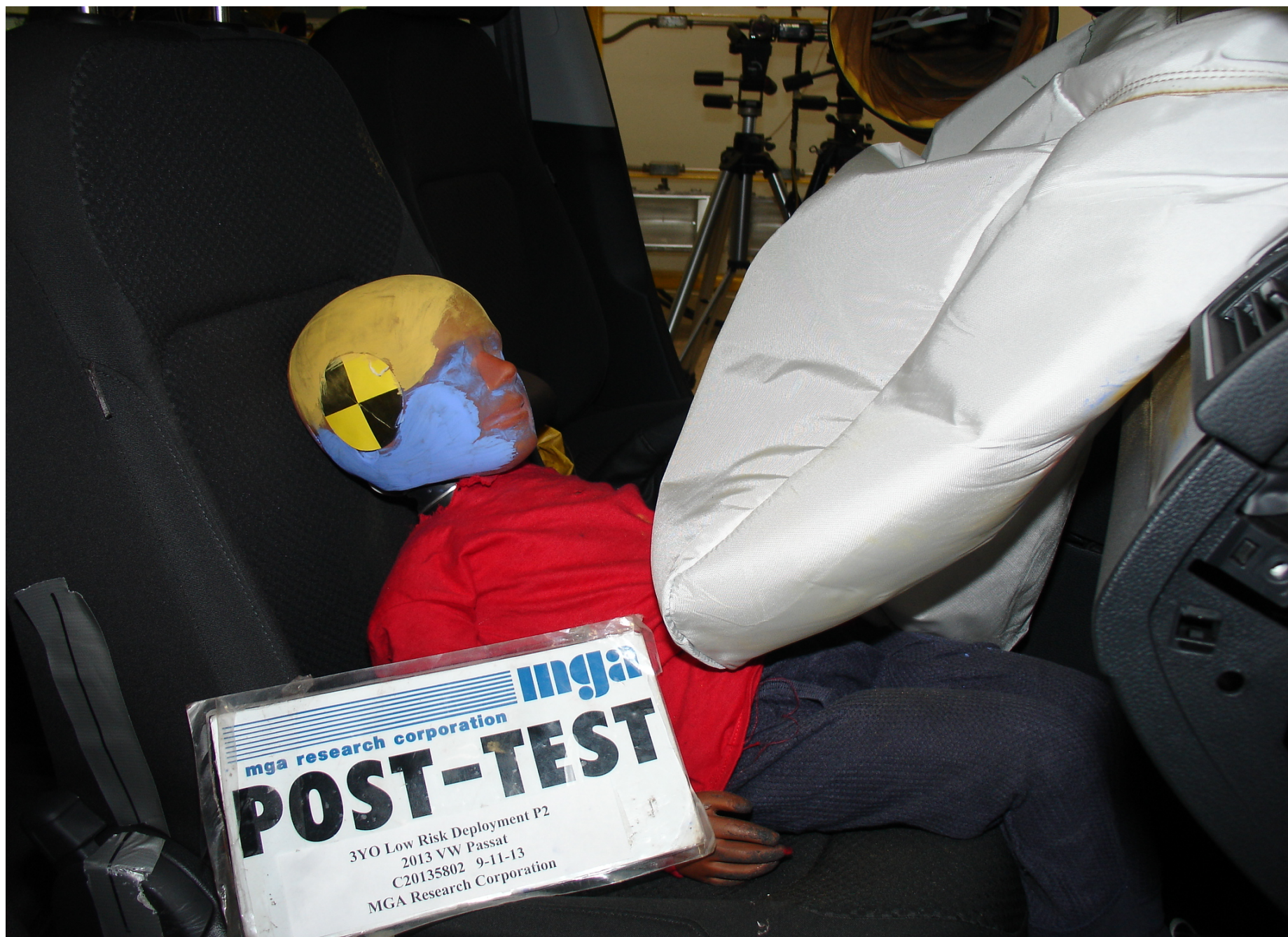
Post-Test 3YO P2 Passenger Dummy Head Contact (seat back)
