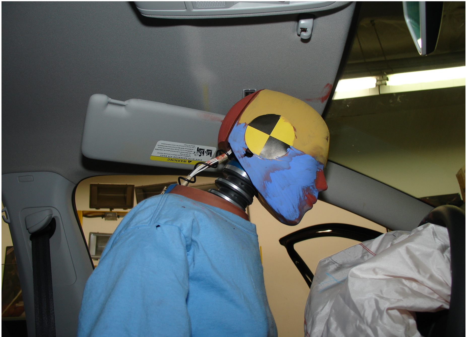
Post-Test 5th Fem. P2 Driver Dummy Head Contact (visor/roof)
