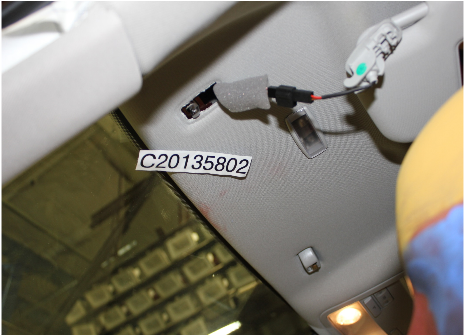
Post-Test Driver Dummy Head Contact (roofline)
