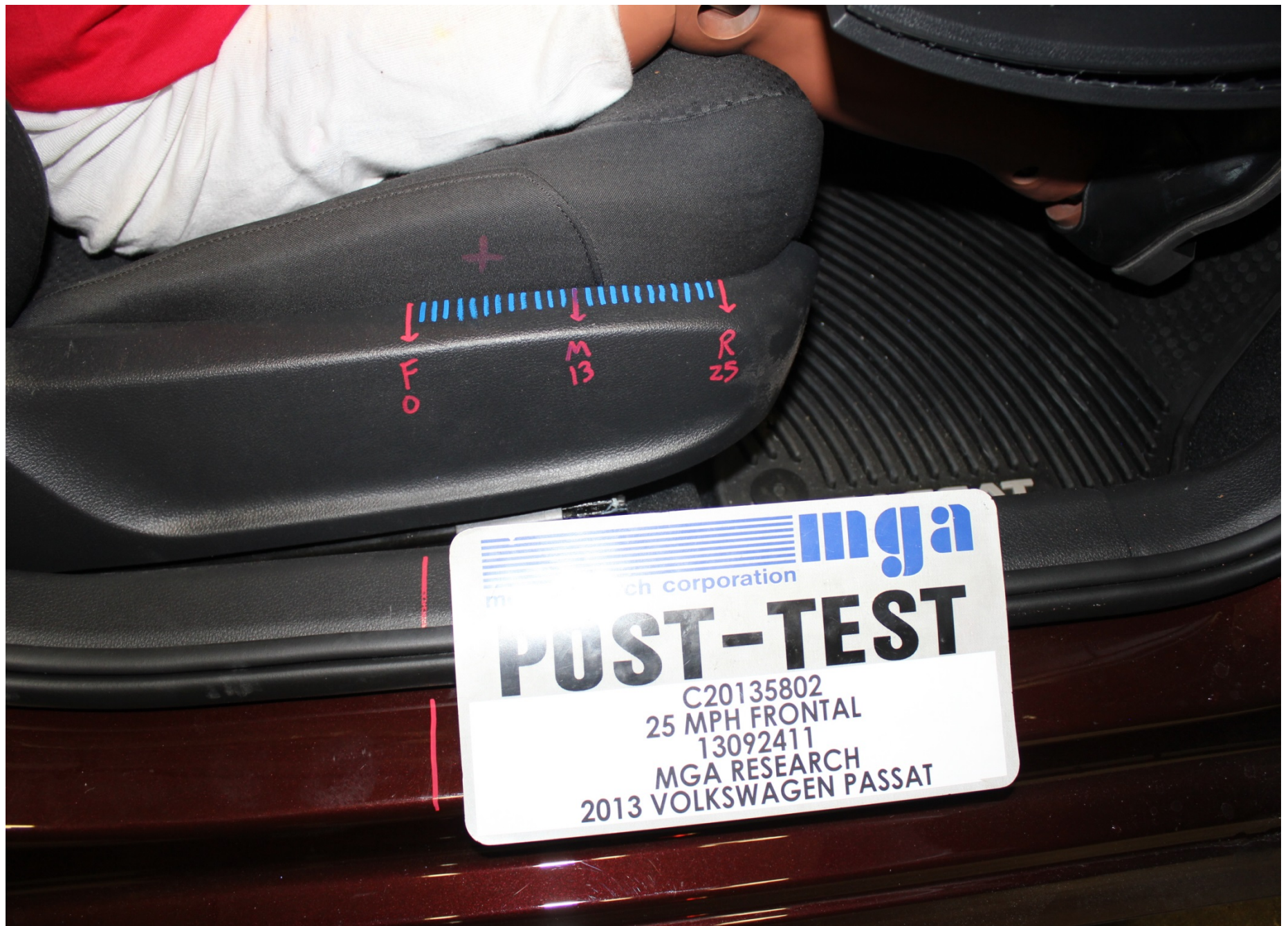
Post-Test Passenger Dummy Seat Position
