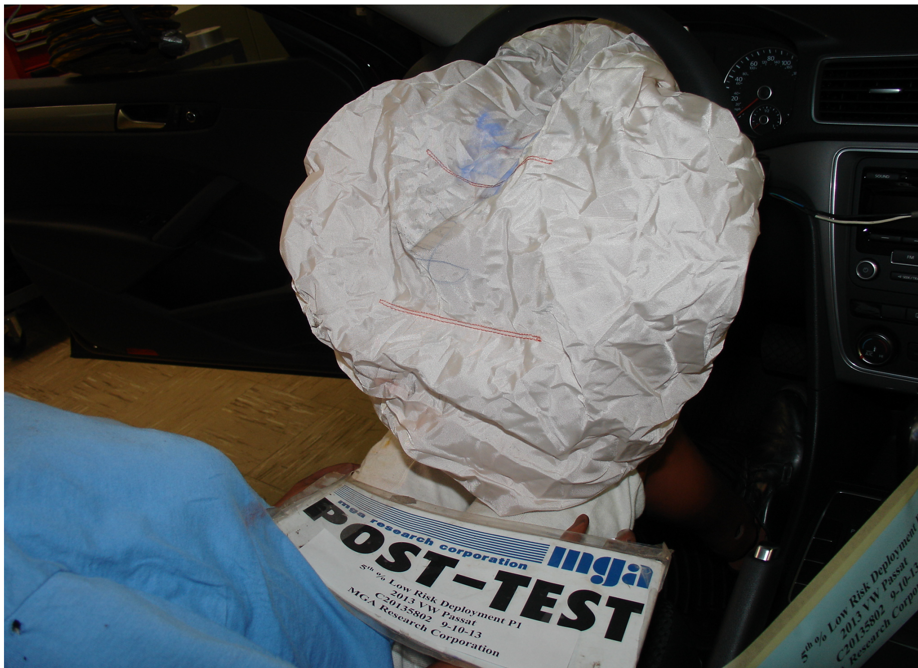
Post-Test 5th Fem. P1 Driver Dummy Airbag Right Side View
