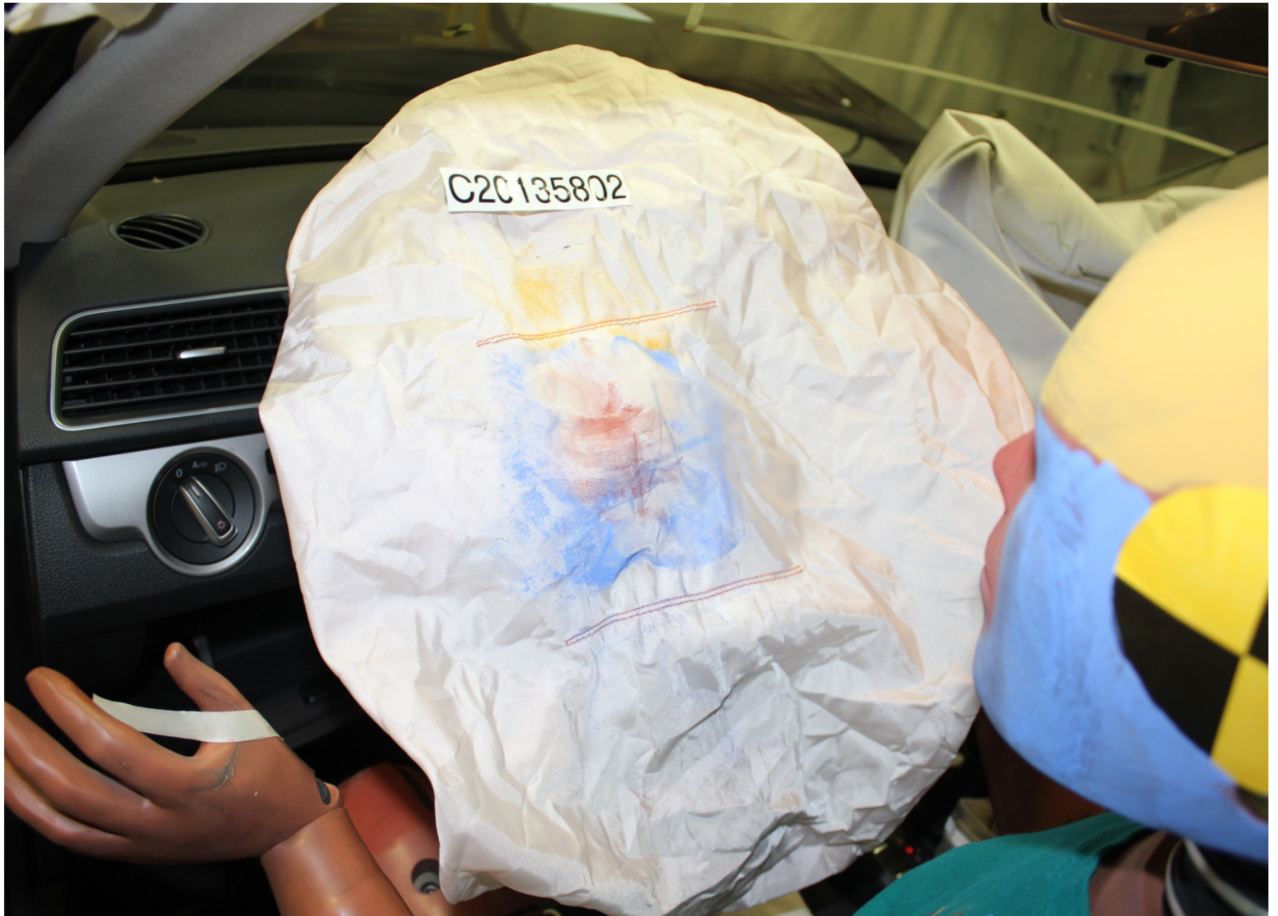
Post-Test Driver Dummy Airbag Contact
