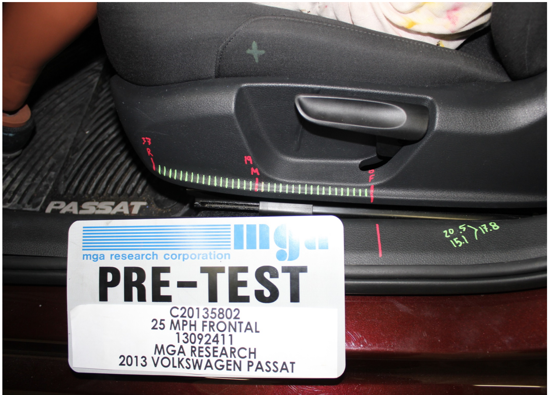
Pre-Test Driver Dummy Seat Position
