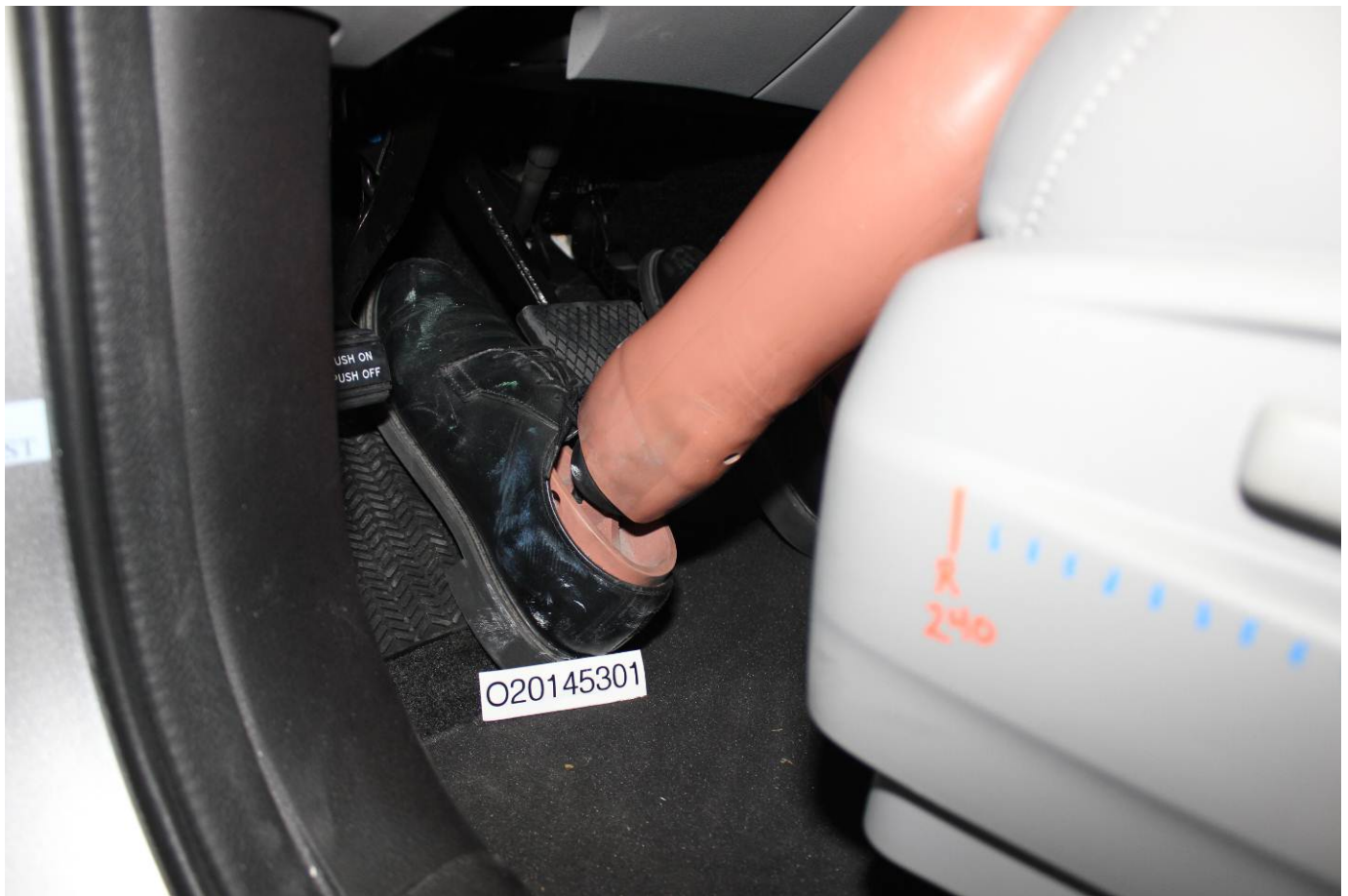
Pre-Test Placement of Dummy's Feet
