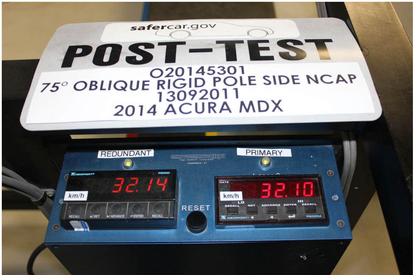
Post-Test Primary and Redundant Speed Trap Read-Out
