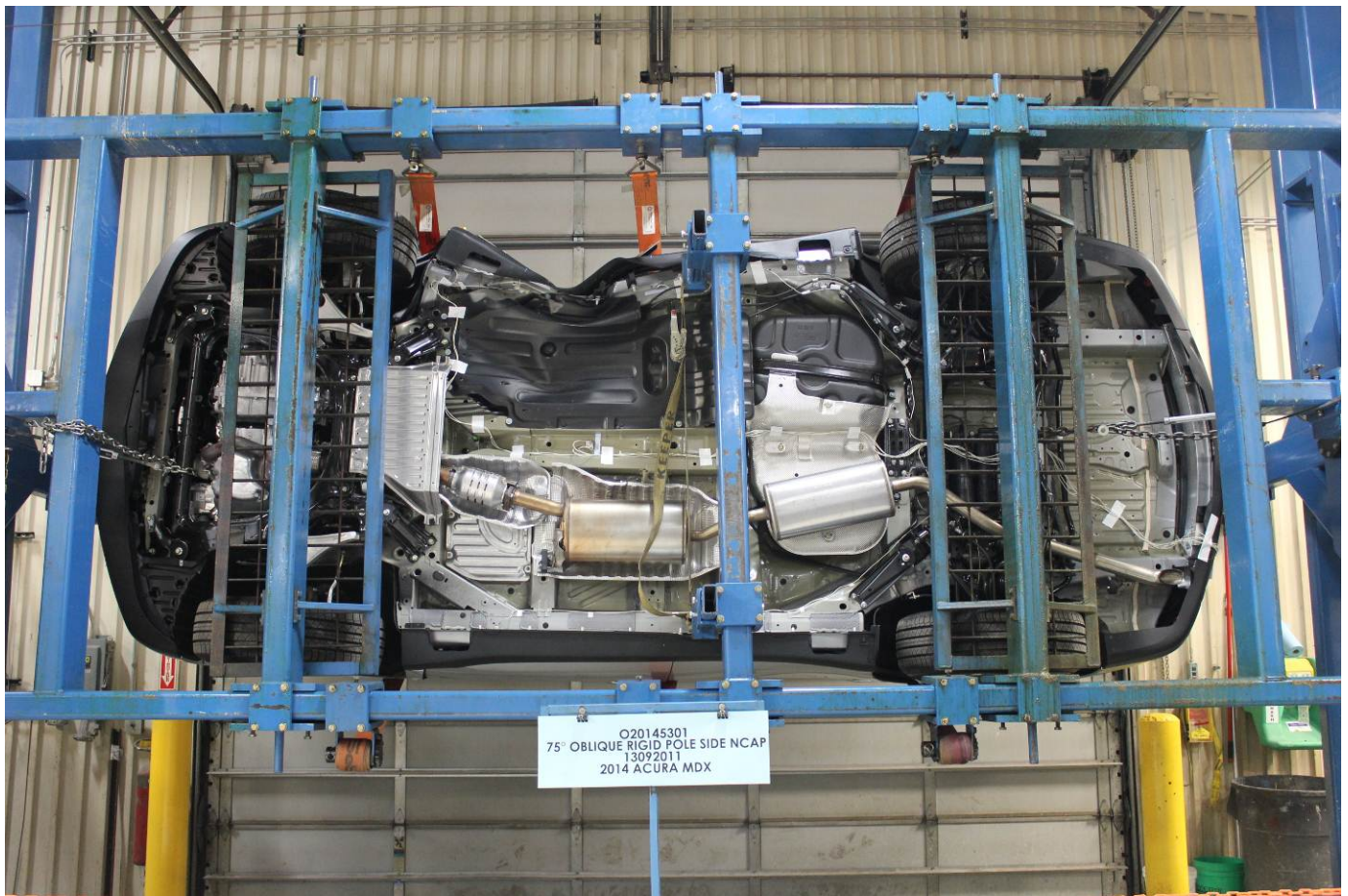
FMVSS No. 301 Static Rollover 270 Degrees
