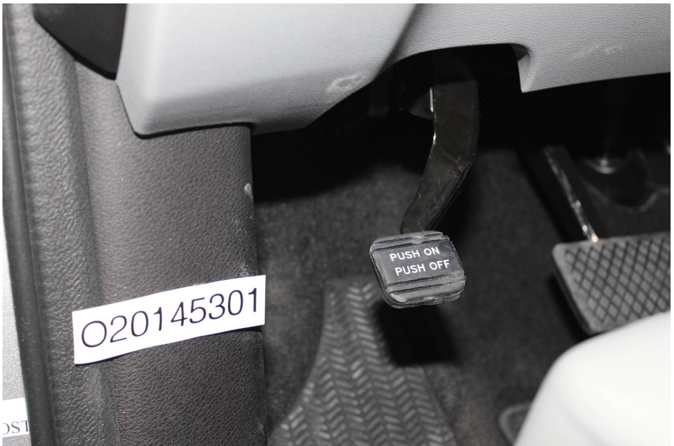
Pre-Test View of Disengaged Parking Brake
