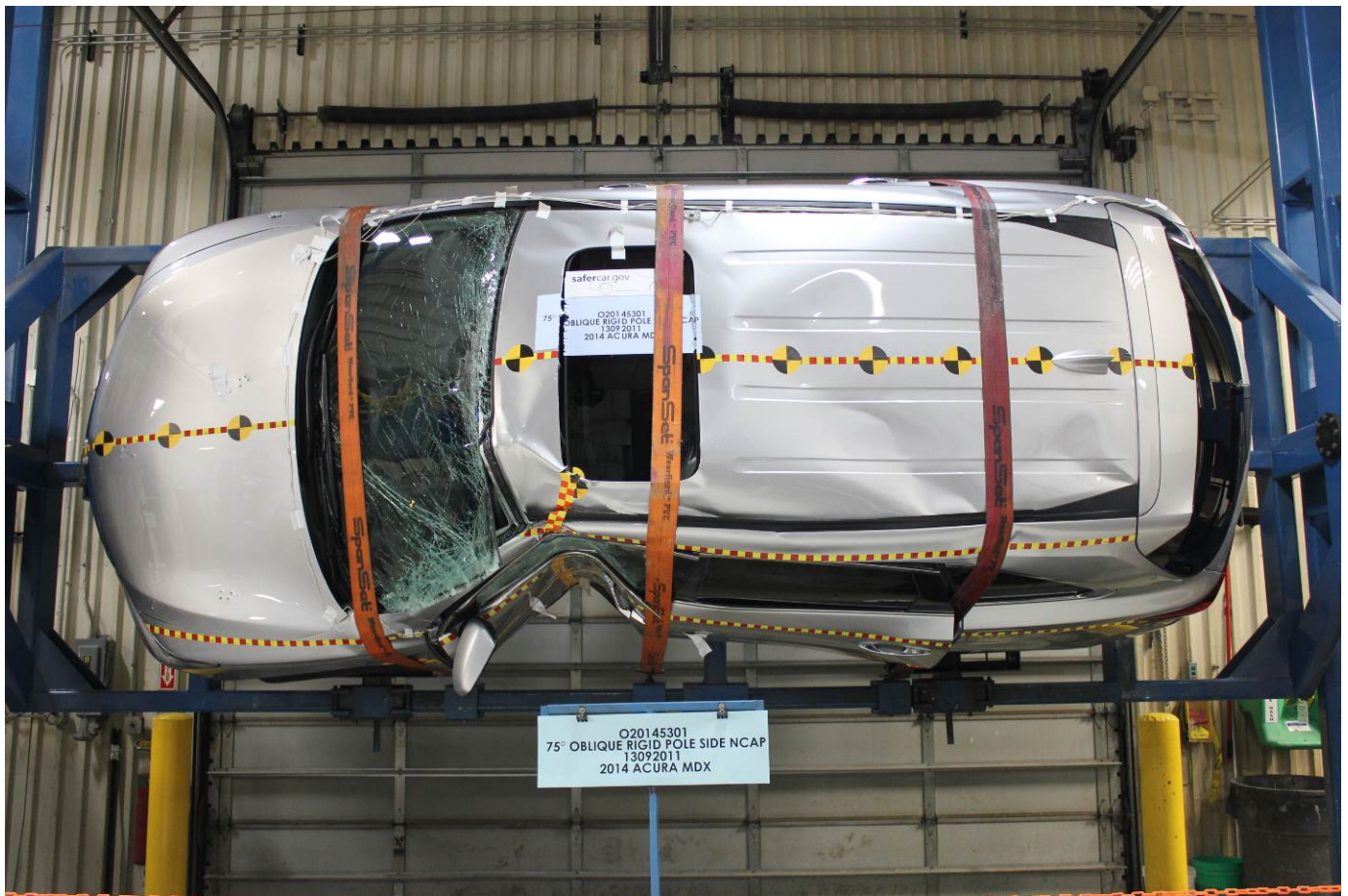
FMVSS No. 301 Static Rollover 90 Degrees
