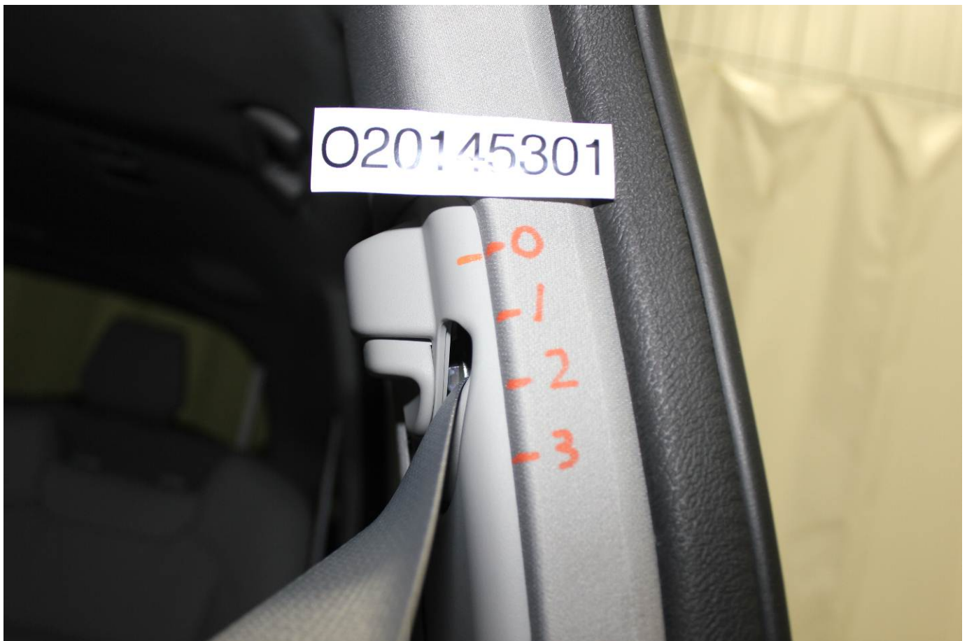
Pre-Test View of Belt Anchorage for Dummy
