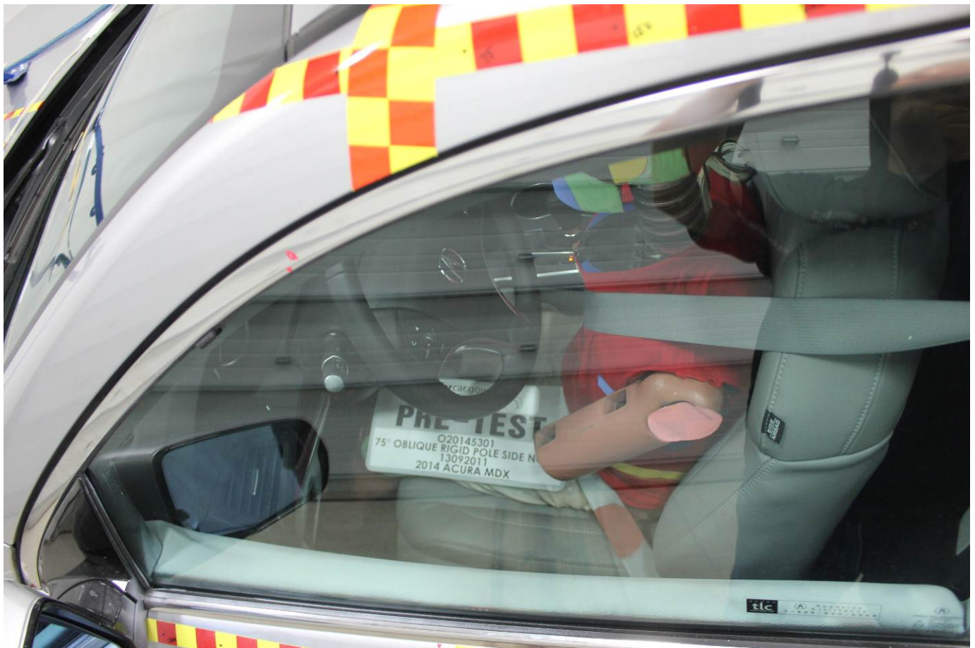
Pre-Test Dummy and Door Clearance View
