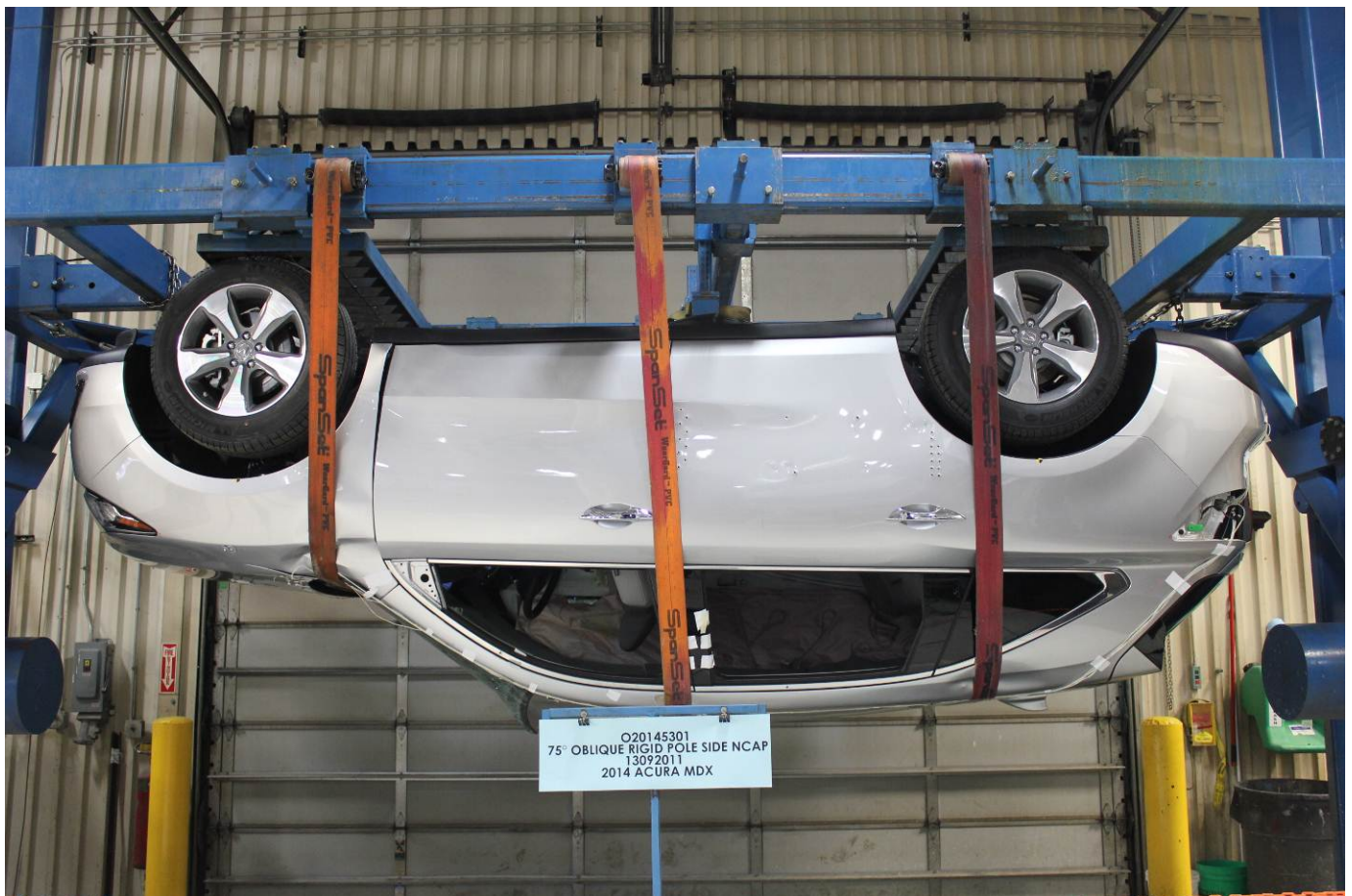
FMVSS No. 301 Static Rollover 180 Degrees
