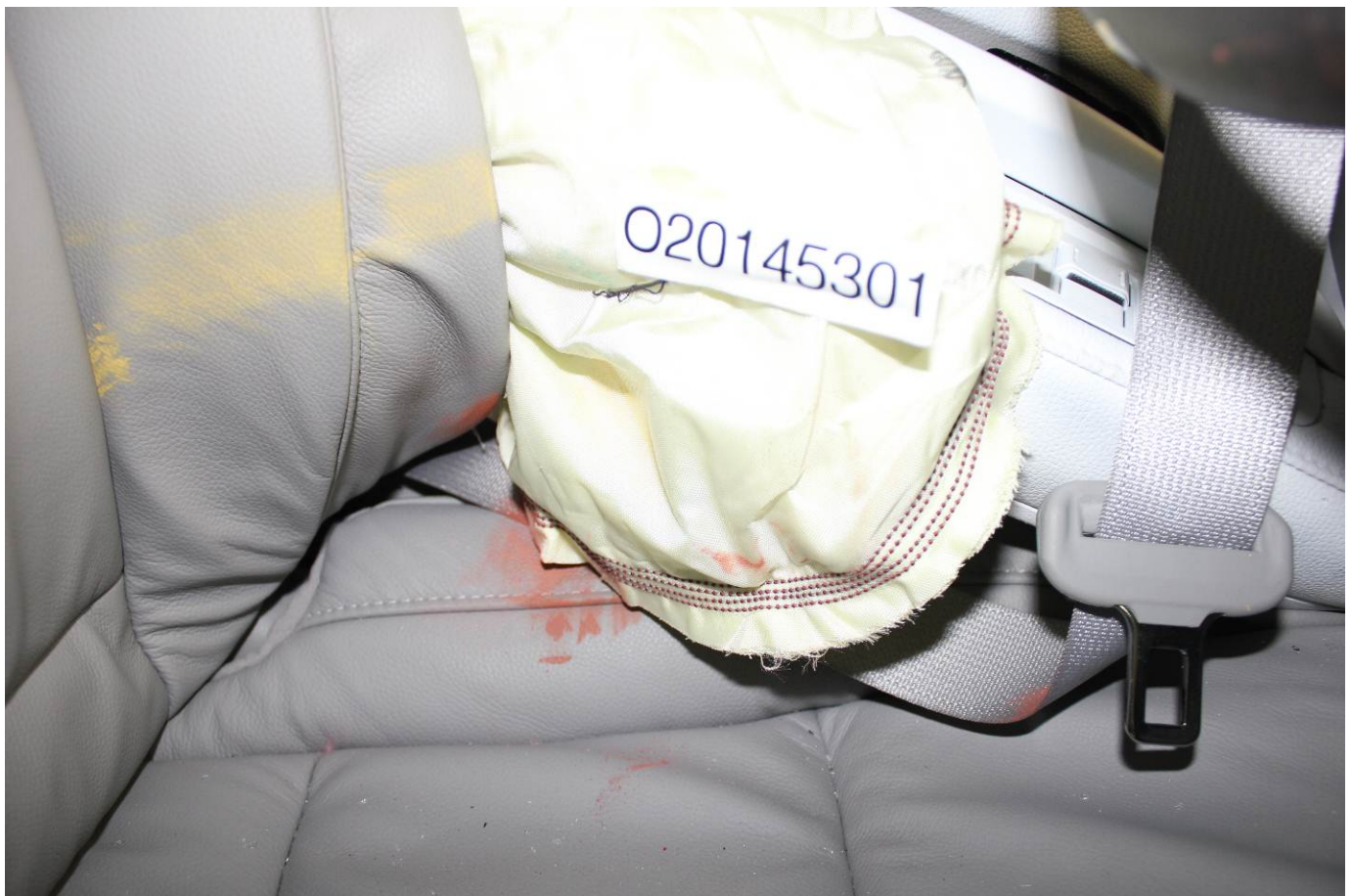
Post-Test Dummy Close-Up Pelvis Contact with Side Air Bag View
