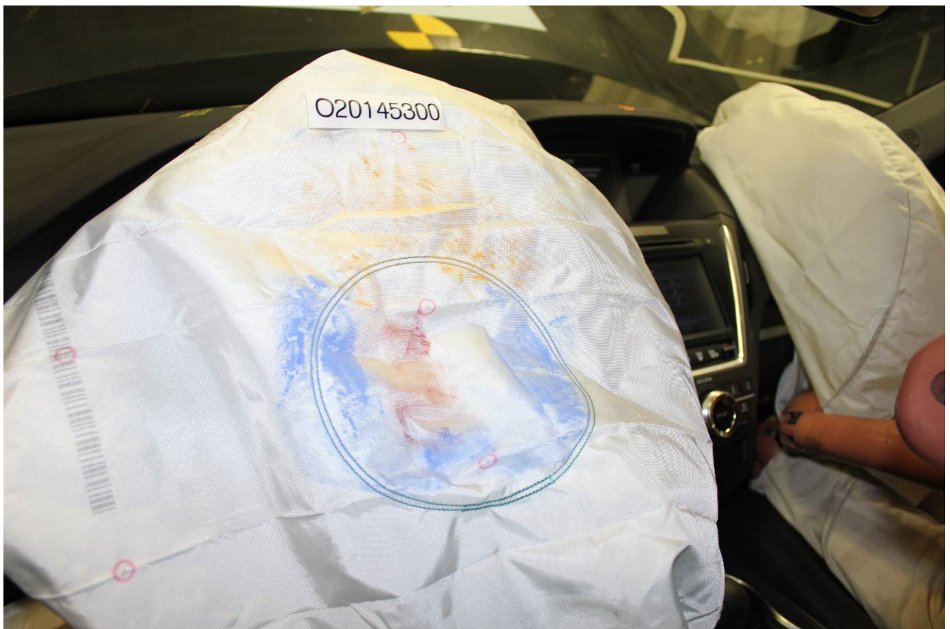
Post-Test Driver Dummy Contact with Airbag
