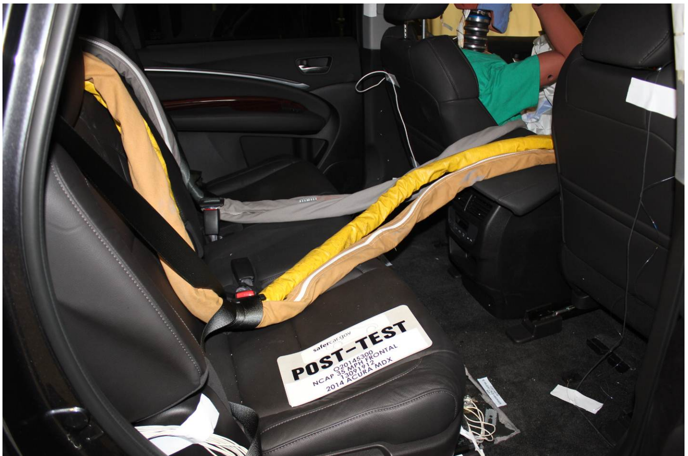
Post-Test Dummy Cable Routing
