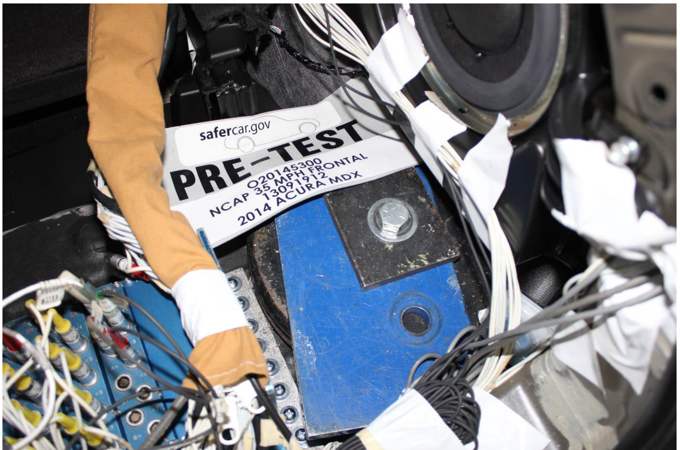
Ballast Installed in Vehicle
