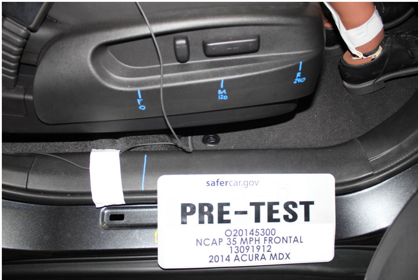
Pre-Test Passenger's Seat Fore-Aft Markings
