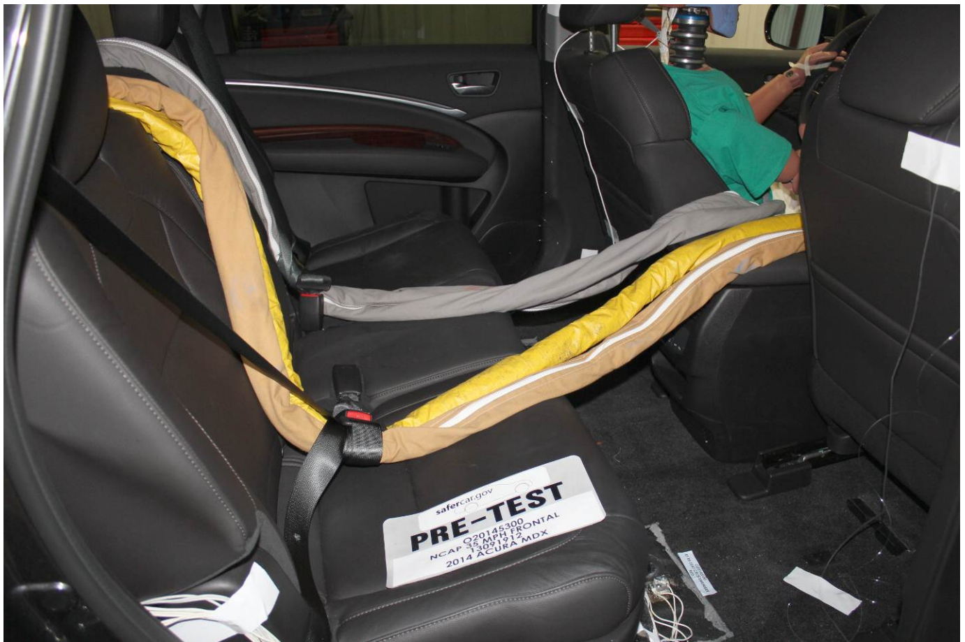
Pre-Test Dummy Cable Routing
