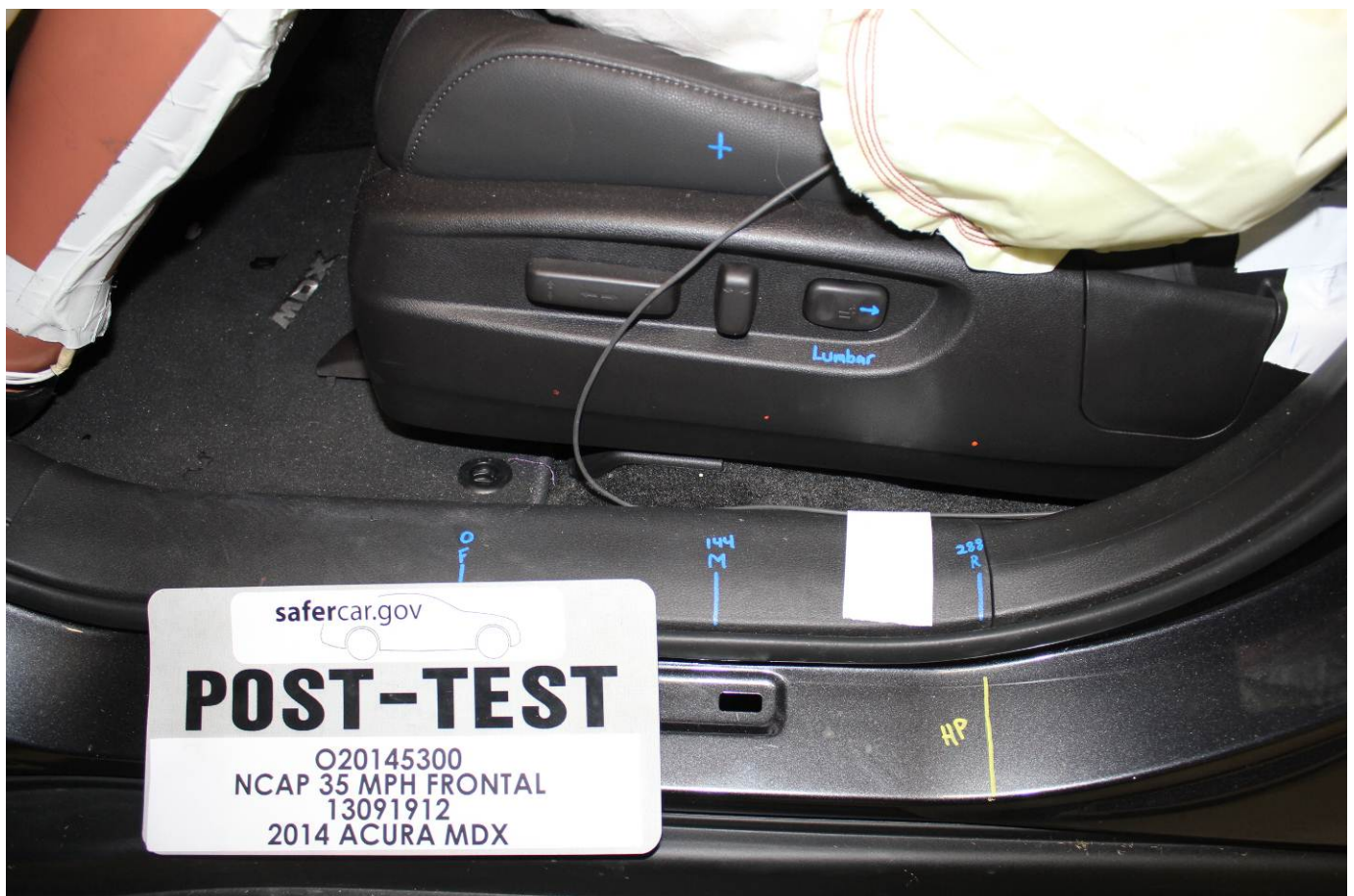
Post-Test Driver's Seat Fore-Aft Markings
