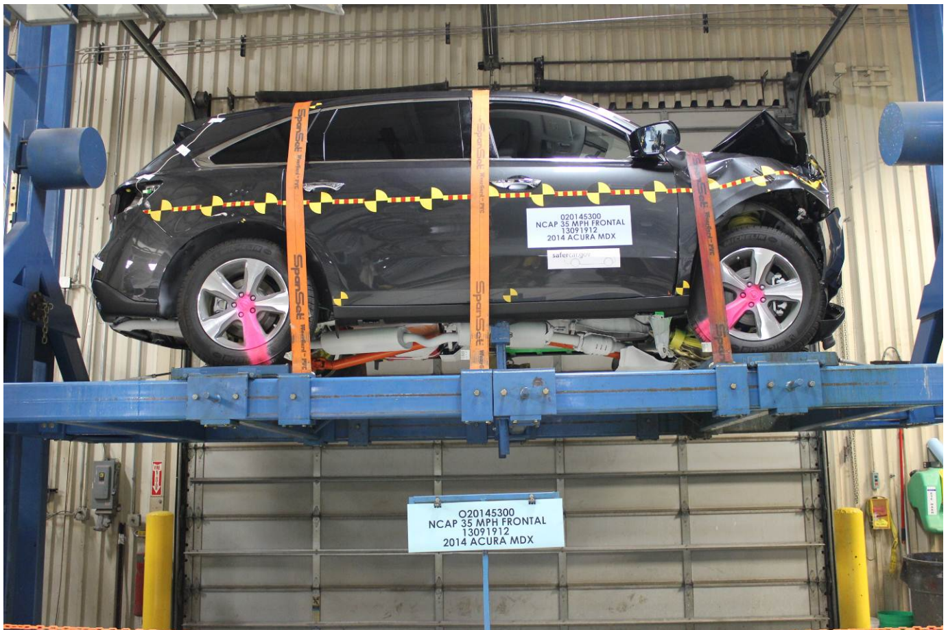
Vehicle at 360 Degrees on Static Rollover Device
