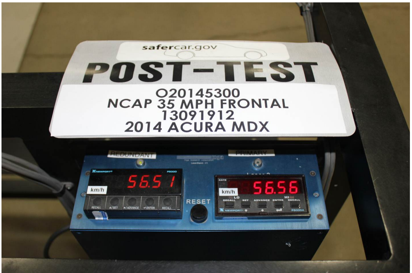
Post-Test Speed Trap Read-Out
