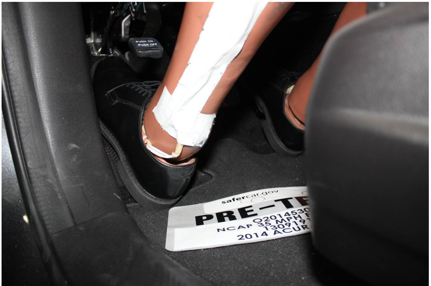
Pre-Test Driver Dummy Feet
