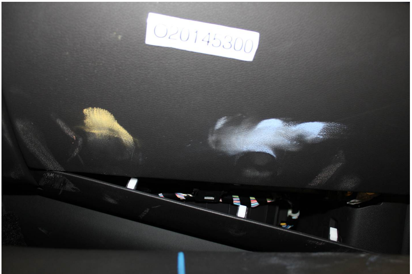
Post-Test Passenger Dummy Contact with Glovebox
