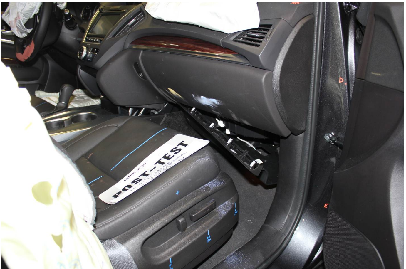
Post-Test Passenger's Side Knee Bolster (without dummy)
