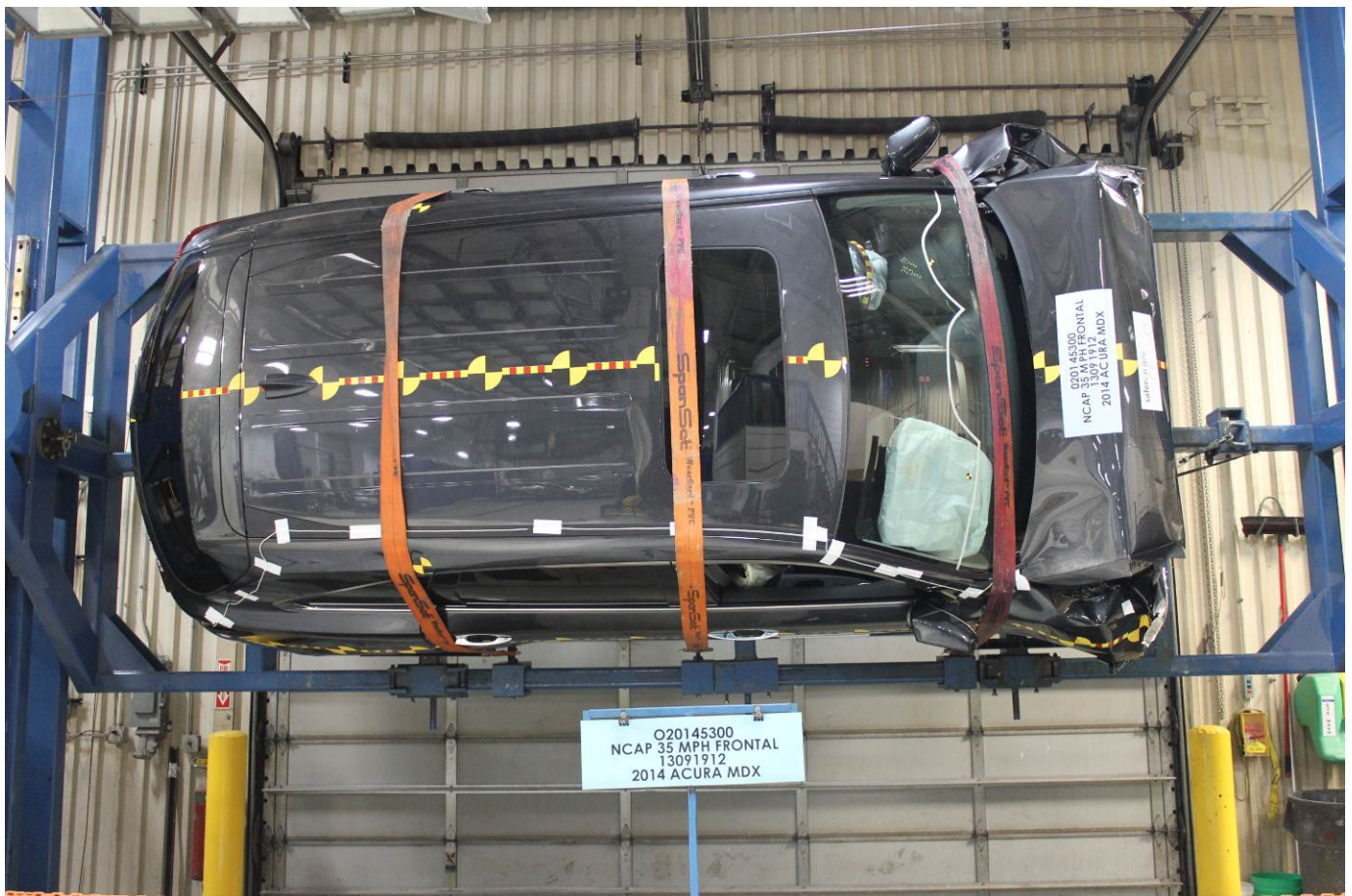
Vehicle at 270 Degree on Static Rollover Device
