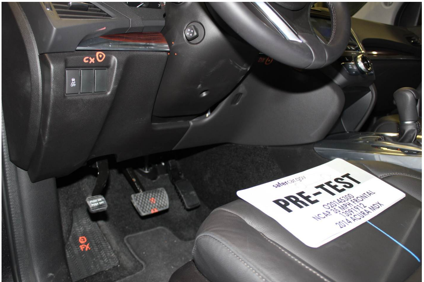
Pre-Test Driver's Side Knee Bolster (without dummy)
