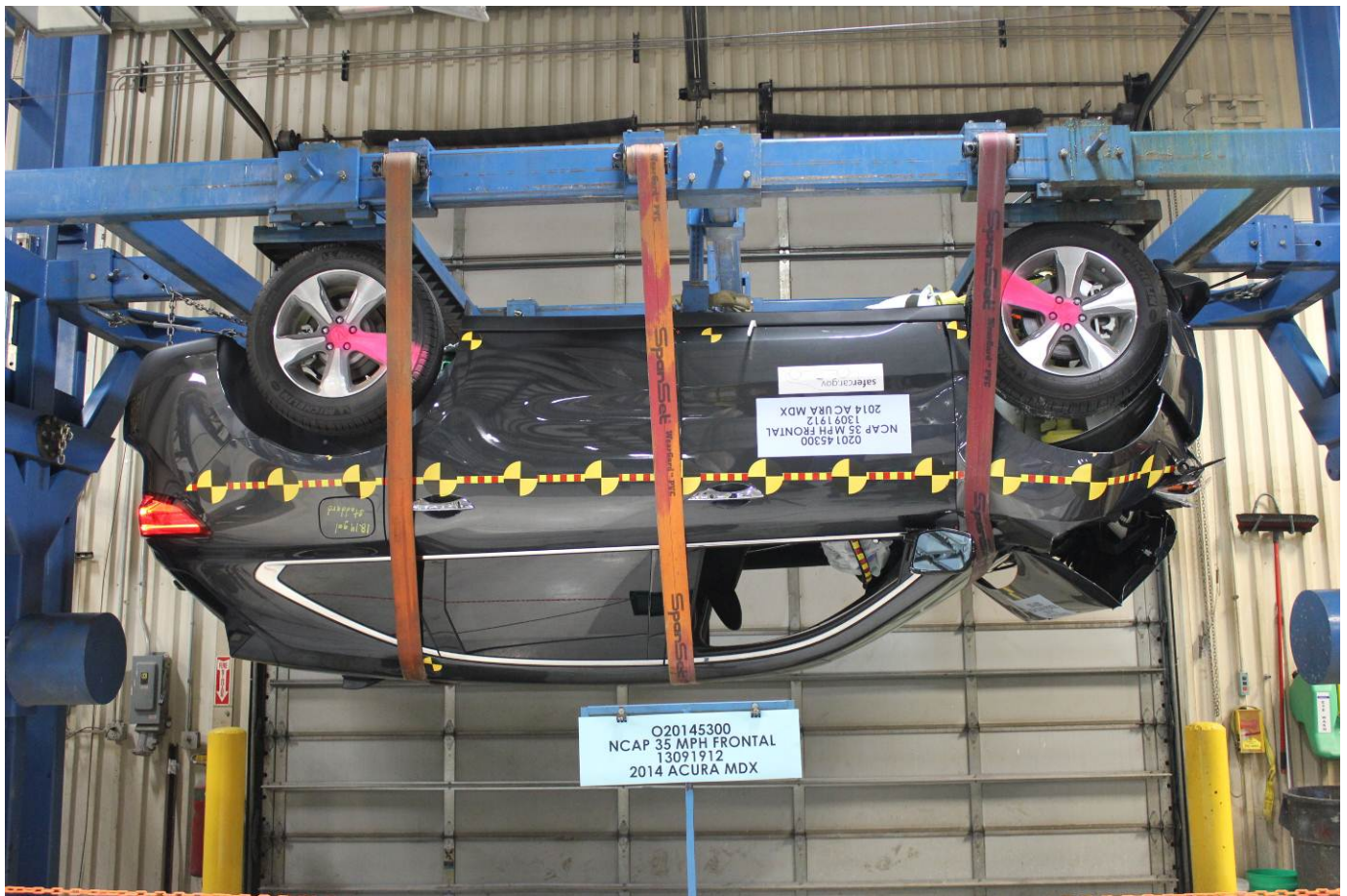
Vehicle at 180 Degrees on Static Rollover Device
