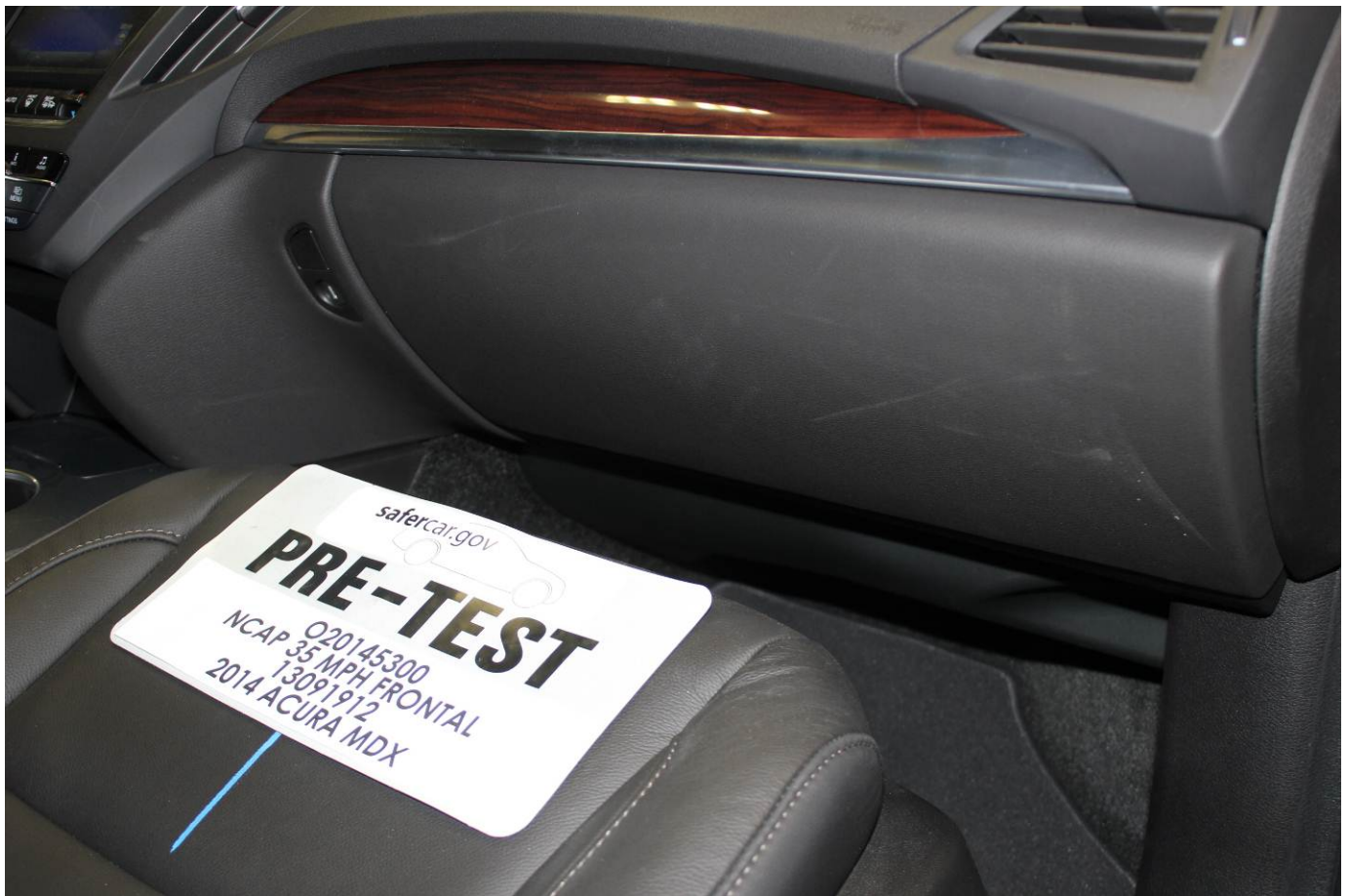
Pre-Test Passenger's Side Knee Bolster (without dummy)
