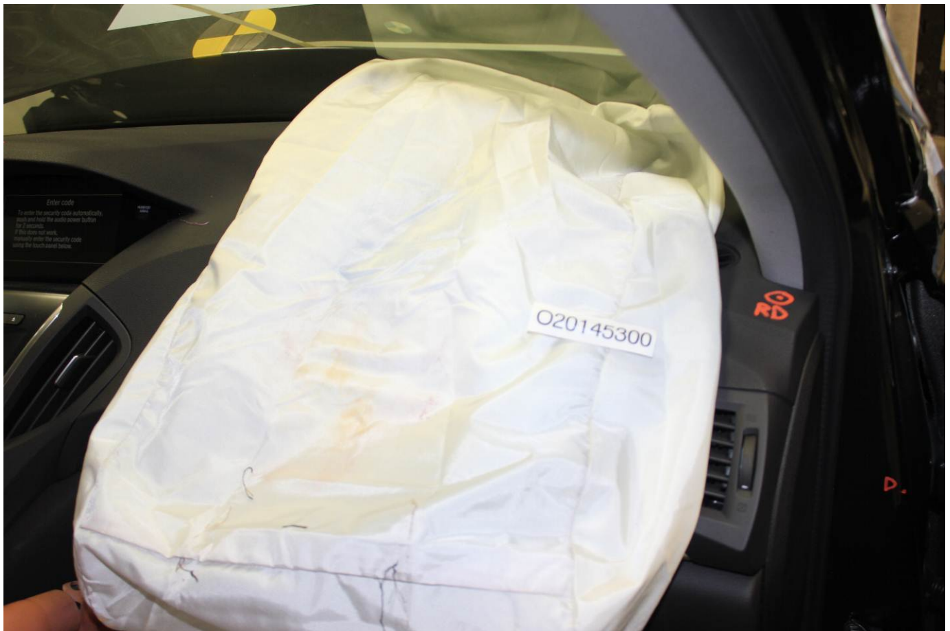
Post-Test Passenger Dummy Contact with Airbag
