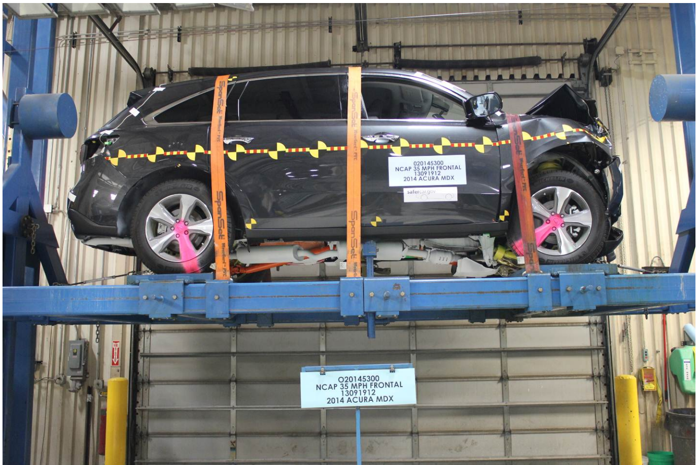
Vehicle at 0 Degree on Static Rollover Device
