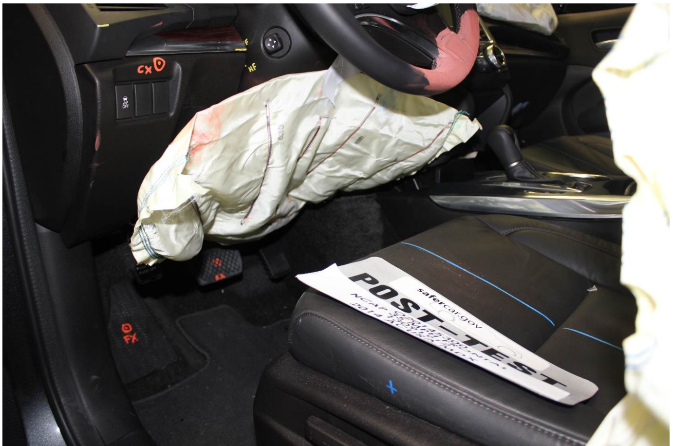
Post-Test Driver's Side Knee Bolster (without dummy)
