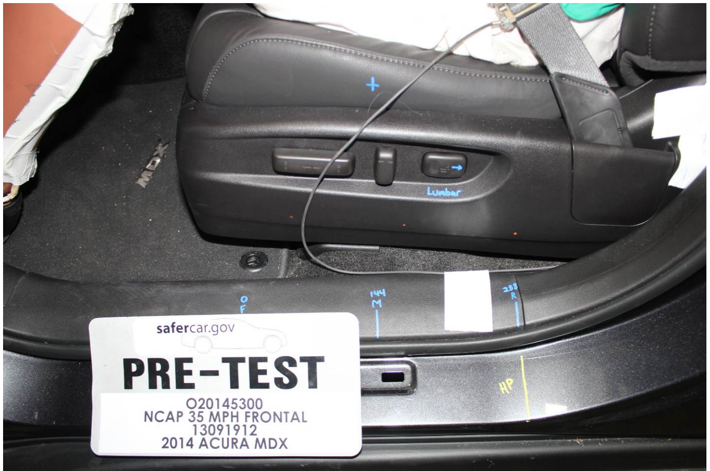
Pre-Test Driver's Seat Fore-Aft Markings
