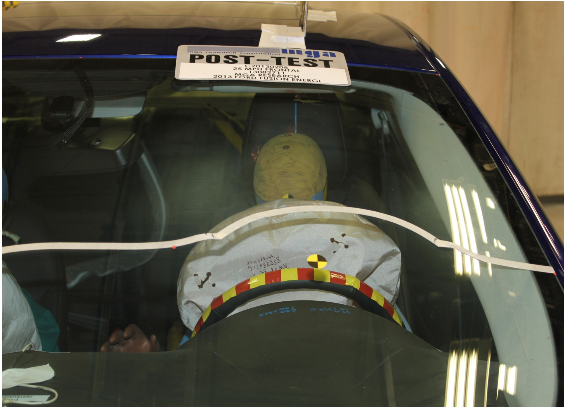
Post-Test Driver Dummy Front View (head position)
