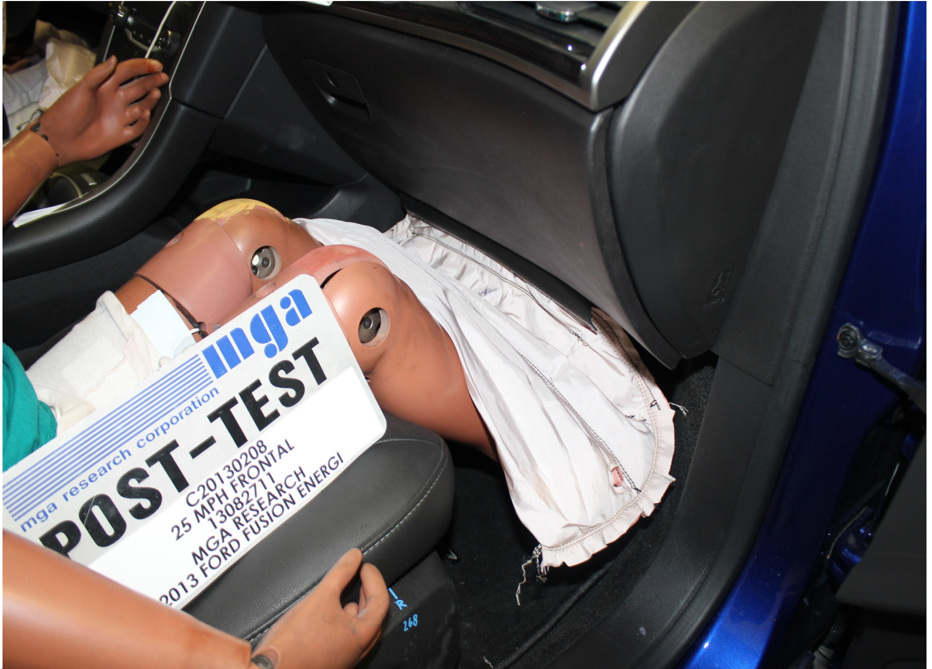
Post-Test Passenger Dummy Knee Contact
