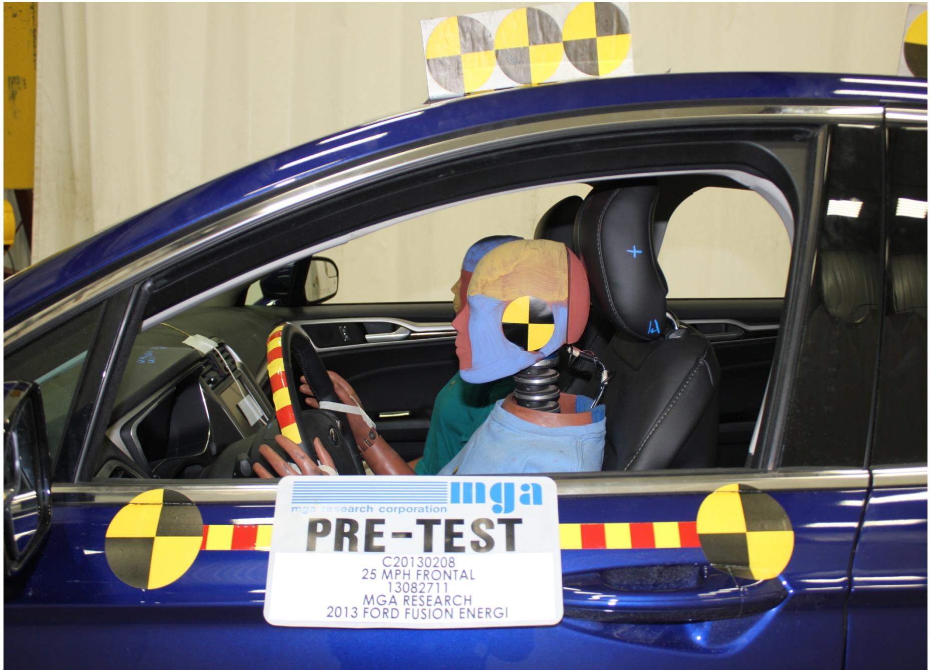
Pre-Test Driver Dummy Position Left Side View
