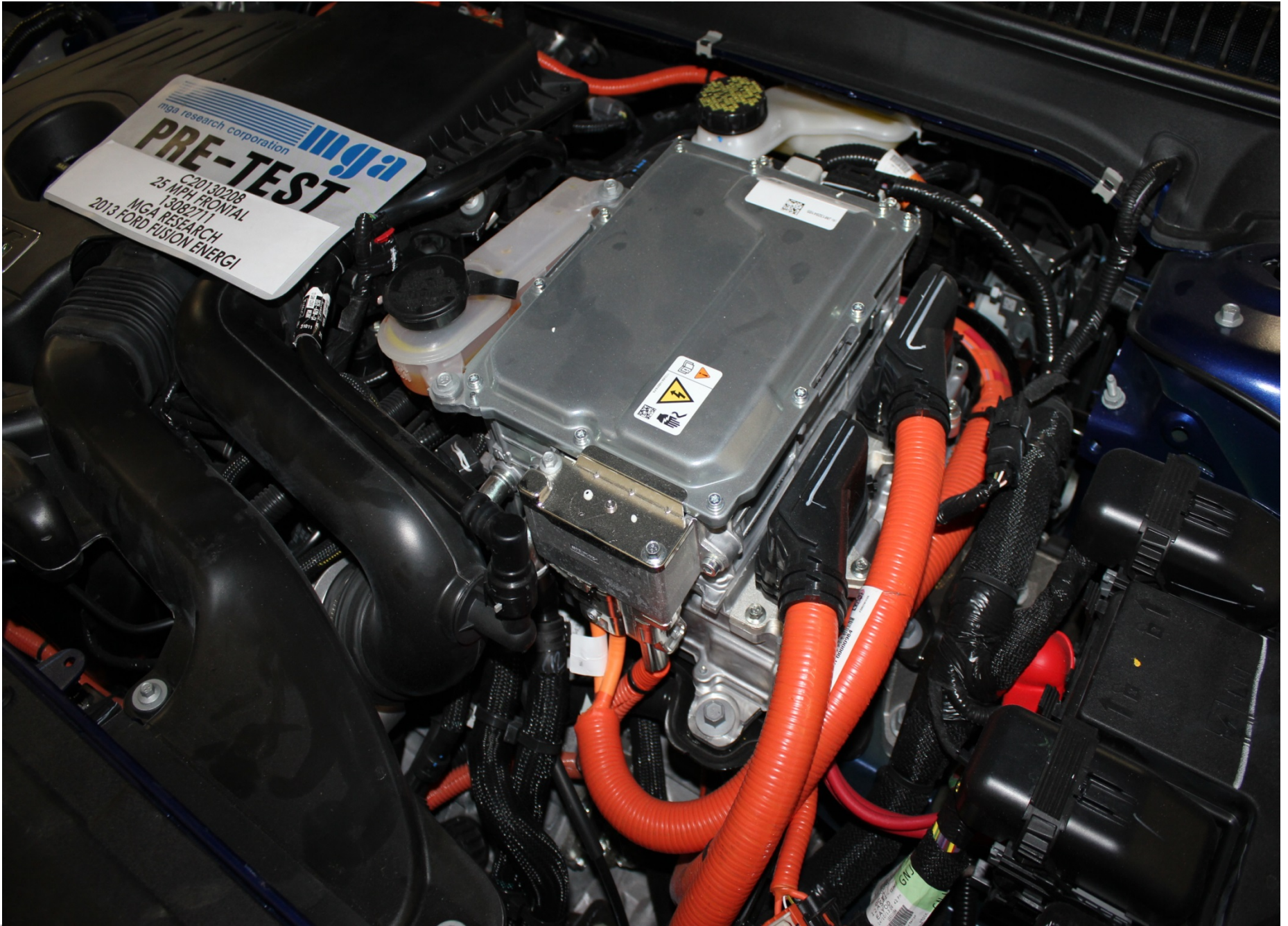
Pre-Test View of Electric Propulsion Drive
