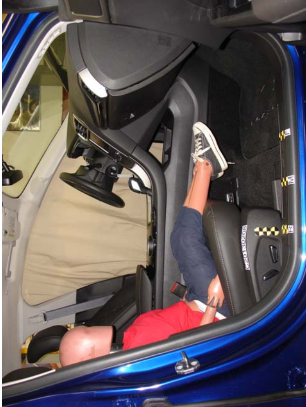
6-Year-Old Unbelted, Rearward Seat Track, Position 1
