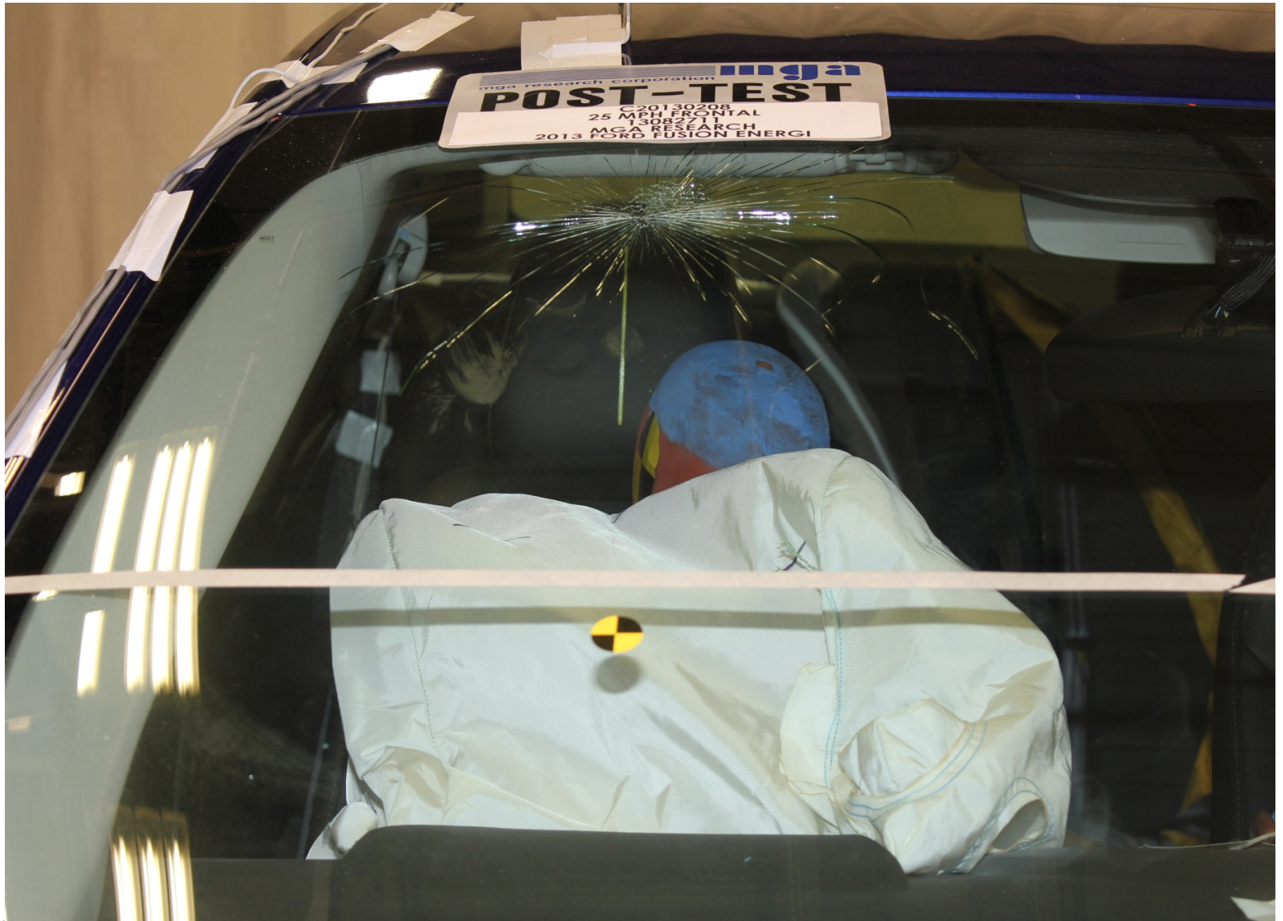
Post-Test Passenger Dummy Front View (head position)
