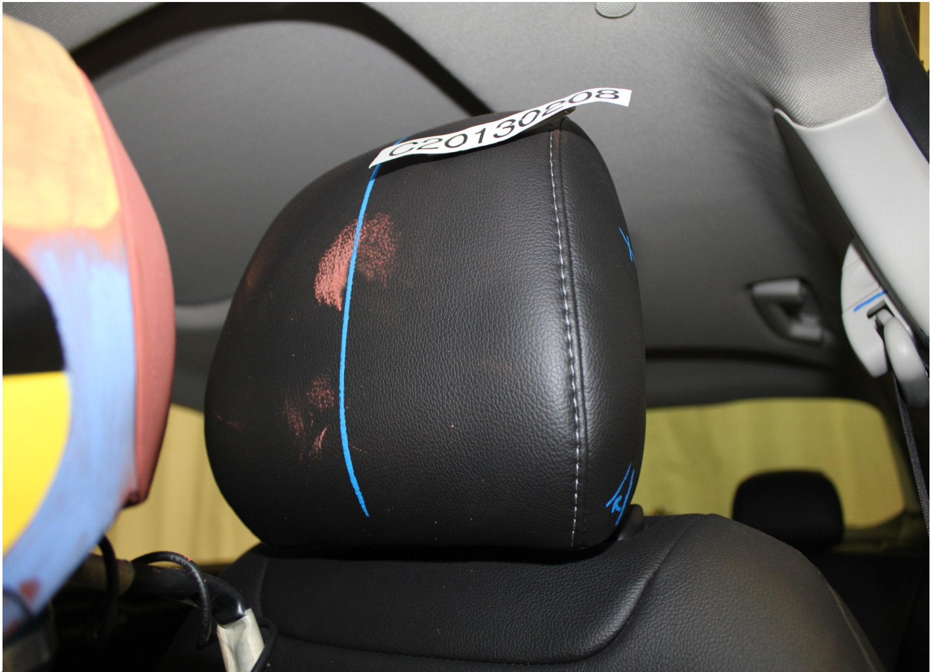
Post-Test Driver Dummy Head Contact (headrest)
