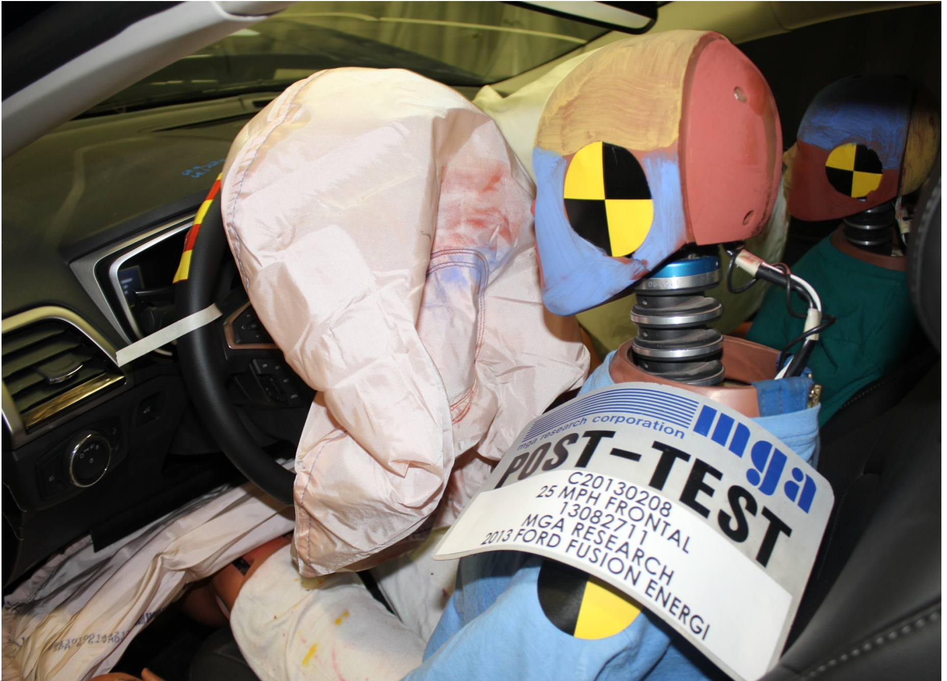
Post-Test Driver Dummy Airbag Contact
