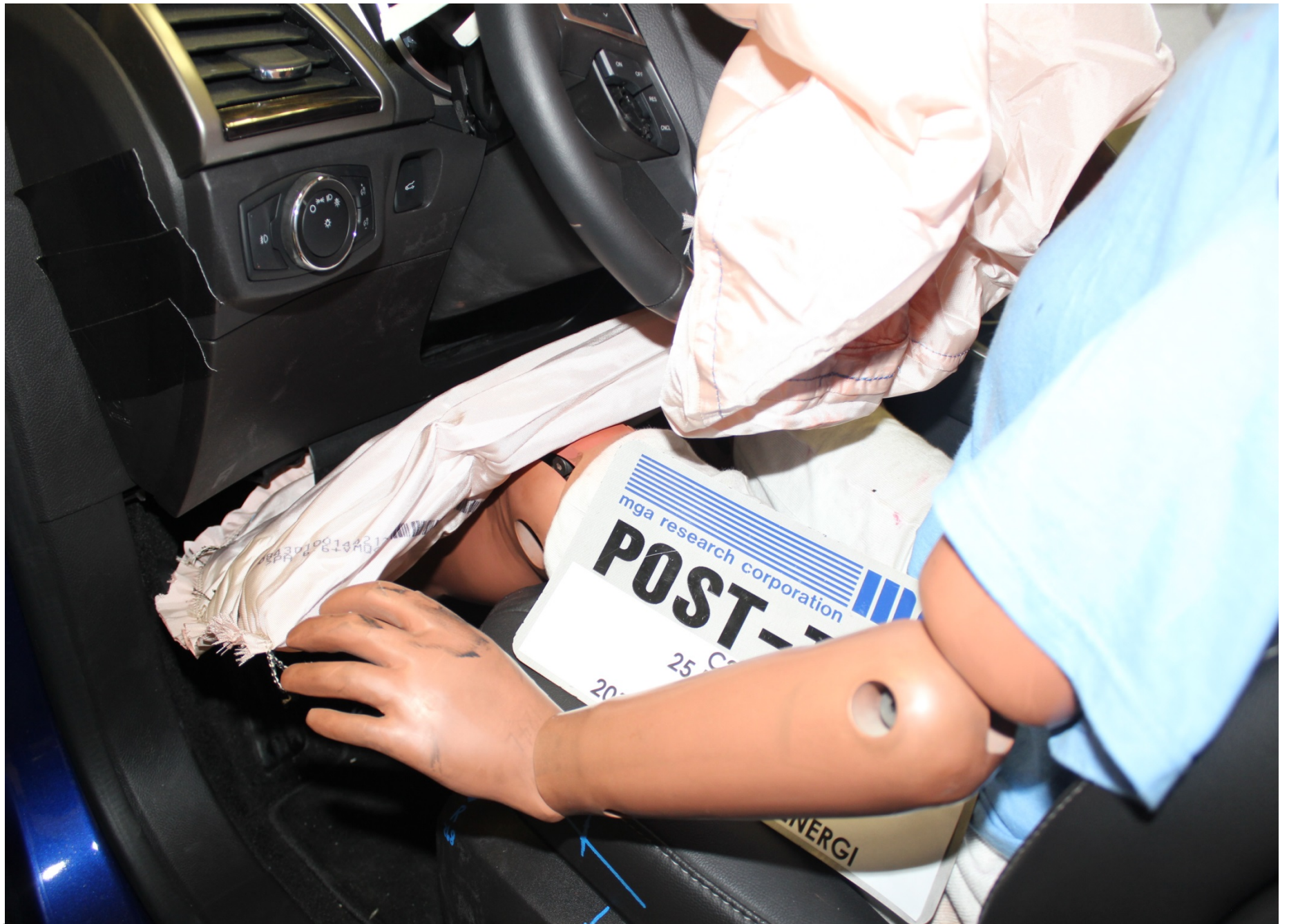
Post-Test Driver Dummy Knee Contact
