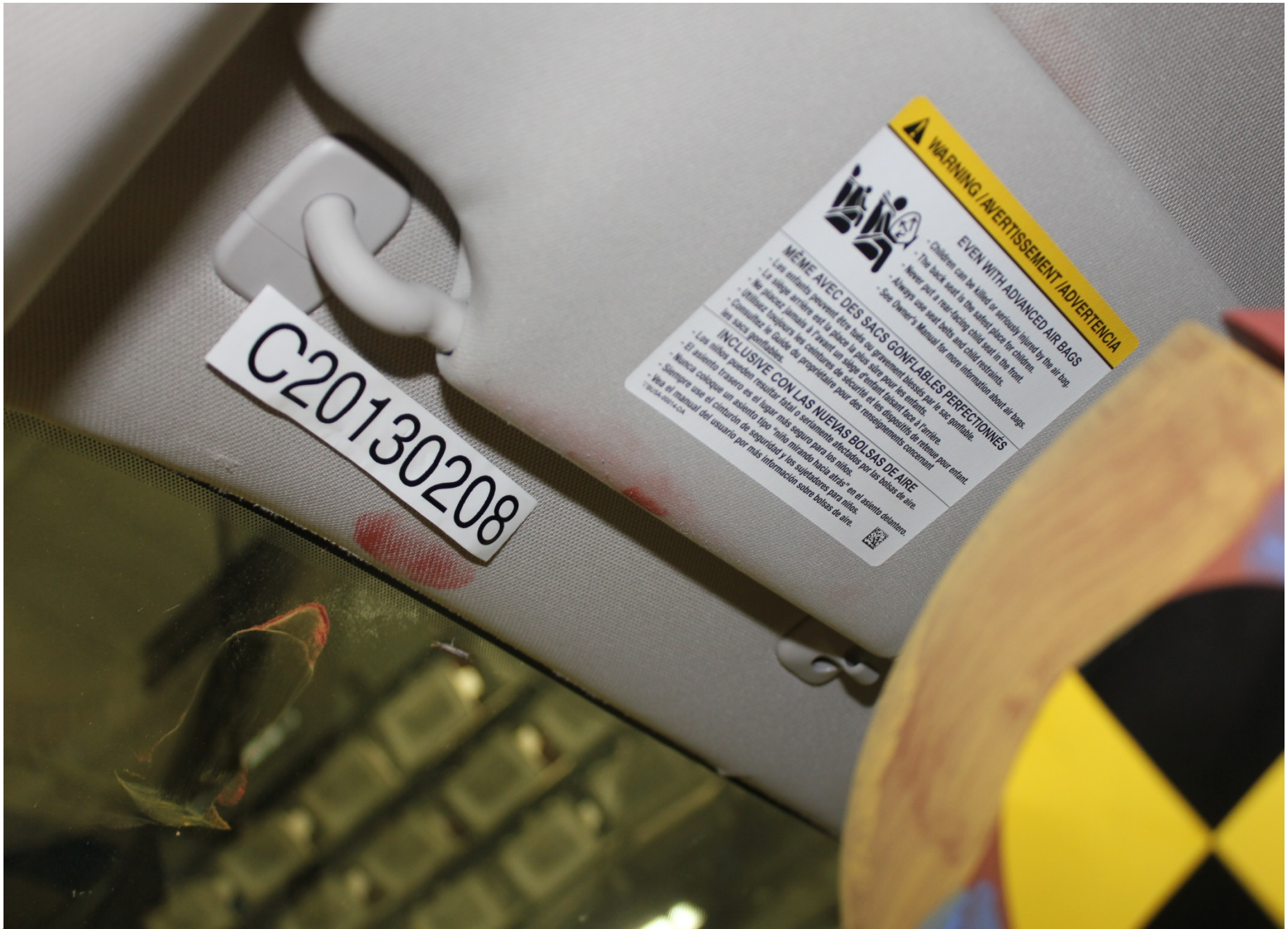
Post-Test Driver Dummy Head Contact (visor)
