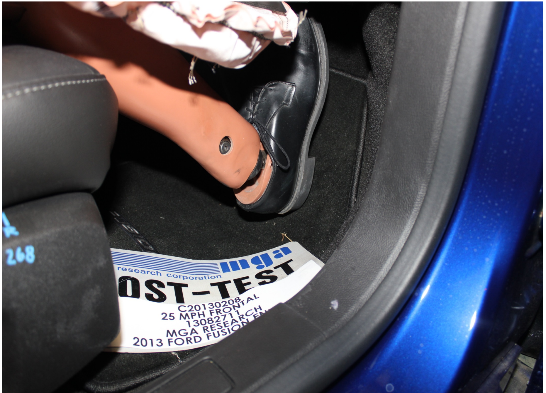
Post-Test Passenger Dummy Feet Position
