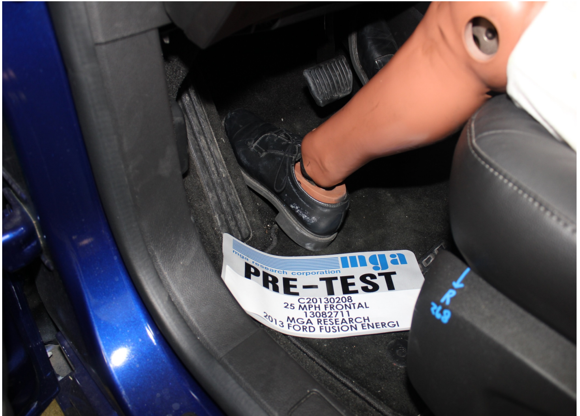
Pre-Test Driver Dummy Feet Position
