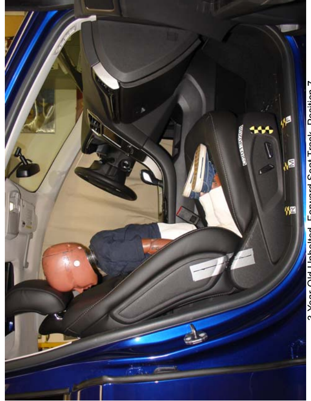
3-Year-Old Unbelted, Forward Seat Track, Position 7
