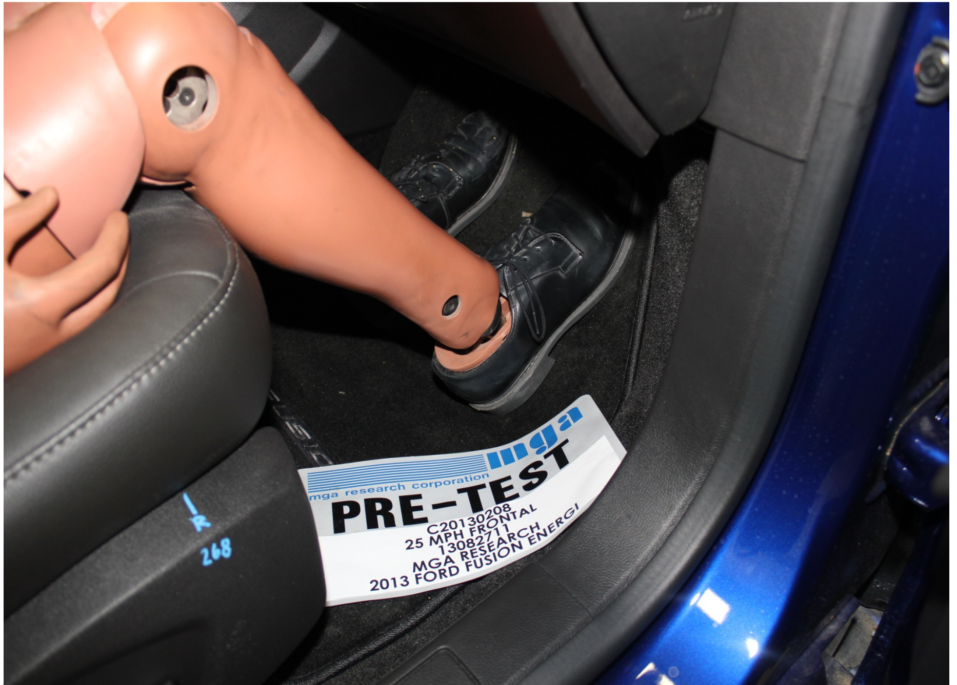
Pre-Test Passenger Dummy Feet Position
