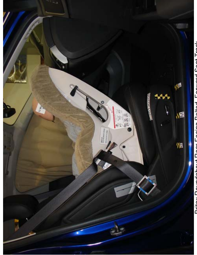
Britax Roundabout Forward Facing Unbelted, Middle Seat Track
