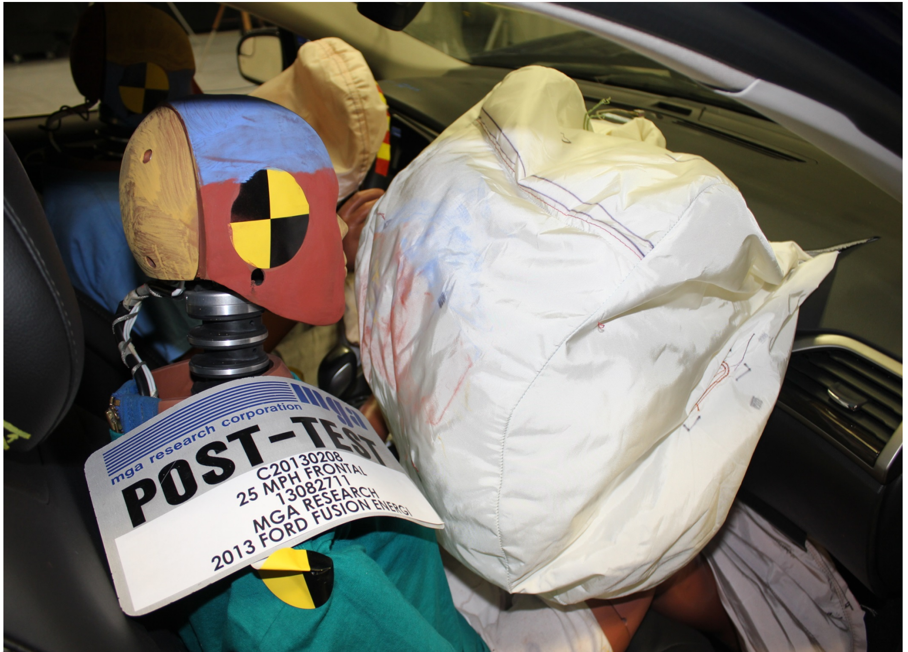
Post-Test Passenger Dummy Airbag Contact
