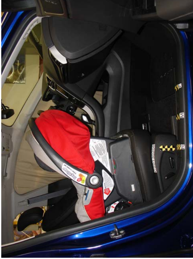
Peg Perego Viaggio WBase, Unbelted, Rear Facing, Rearward Seat Track
