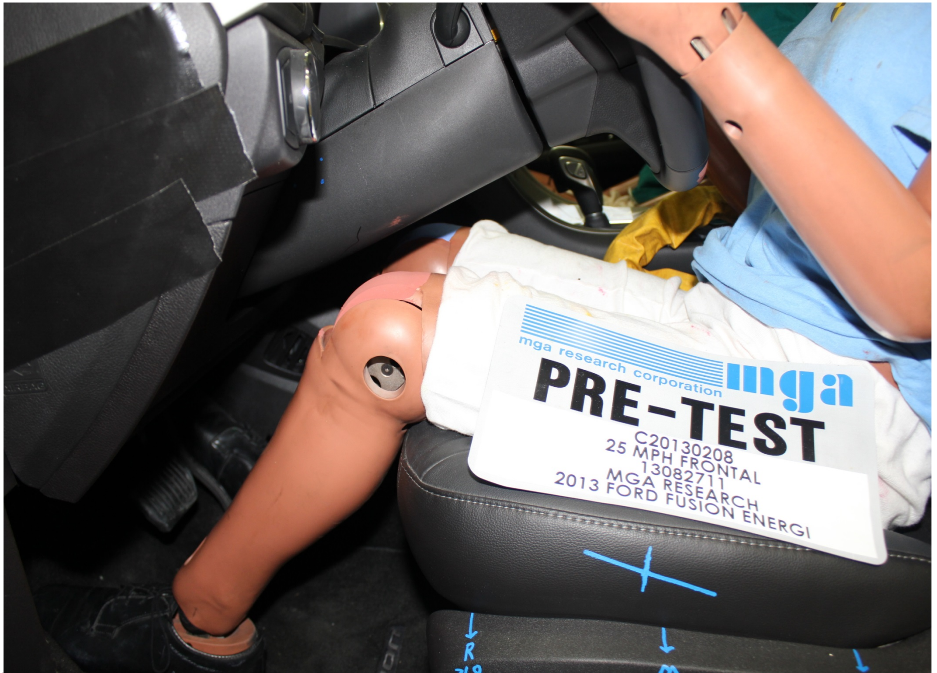
Pre-Test Driver Dummy Seat Position
