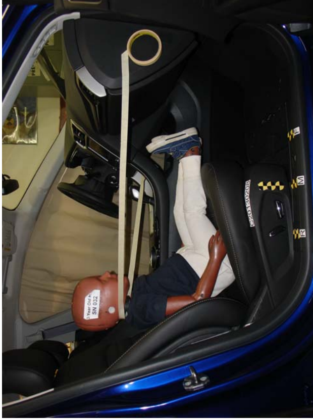
3-Year-Old Unbelted, Middle Seat Track, Position 3
