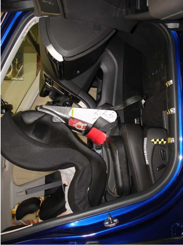
Graco Toddler Safeseat Step 2 Rear Facing Unbelted, Rearward Seat Track
