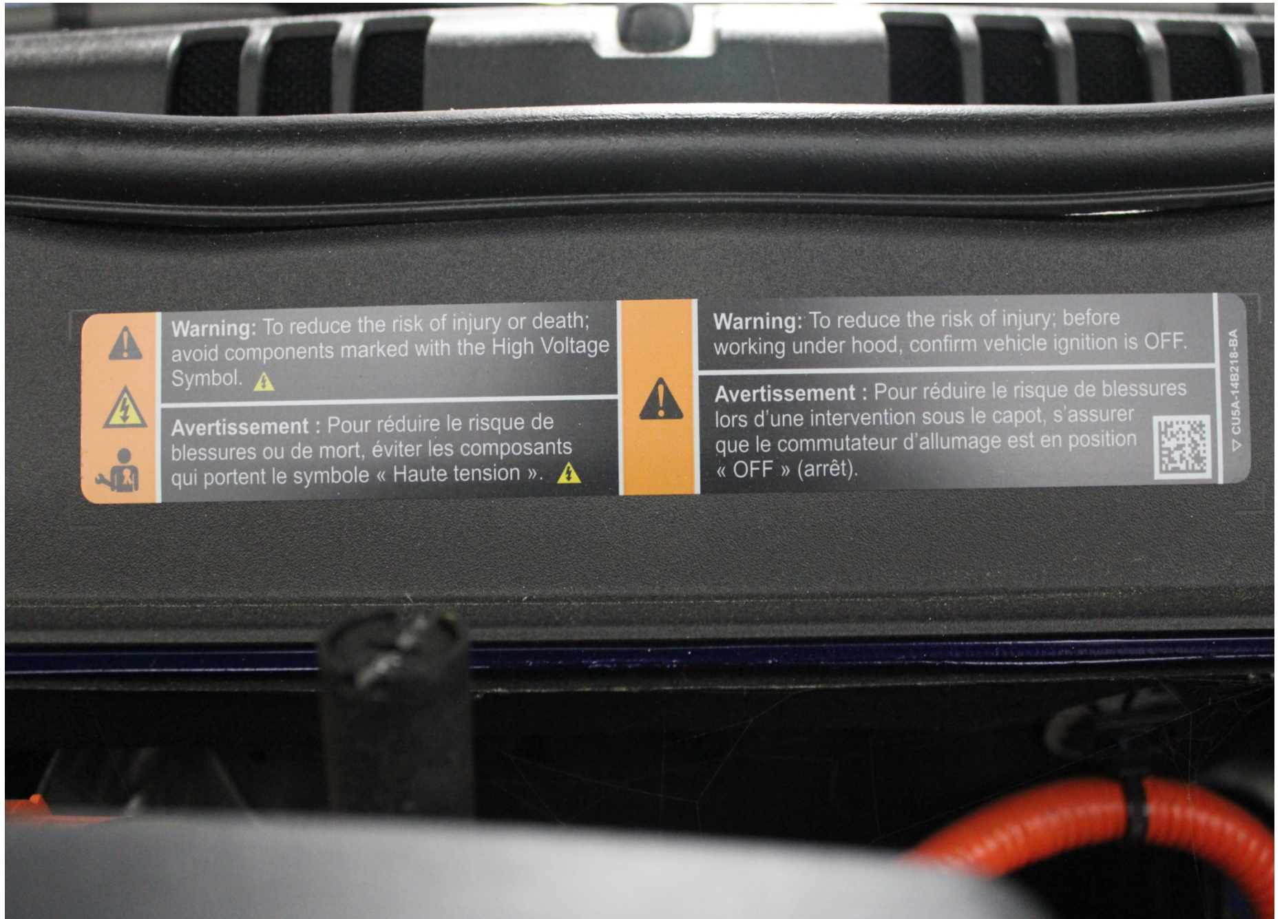
High Voltage Warning Label
