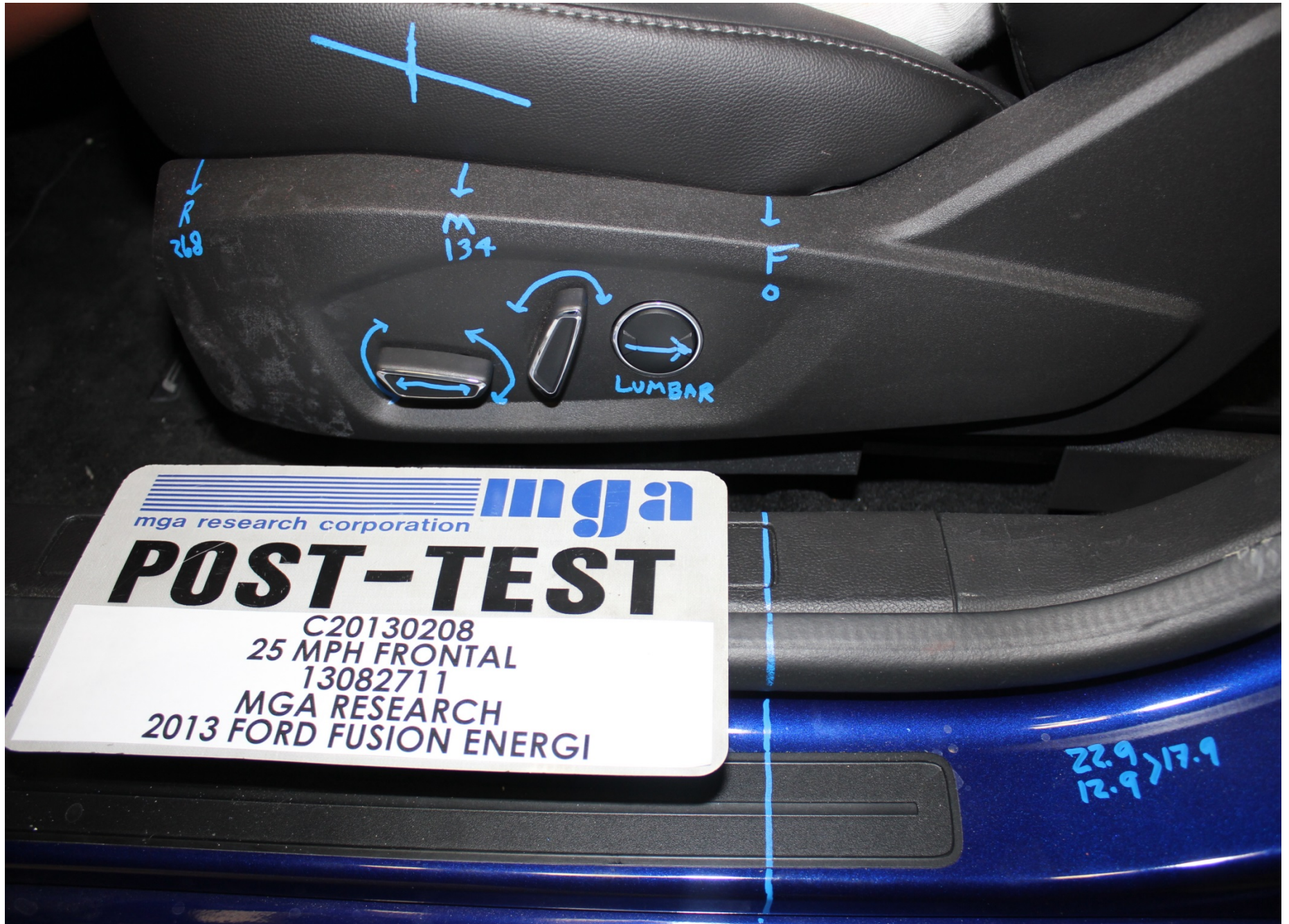
Post-Test Driver Dummy Seat Position
