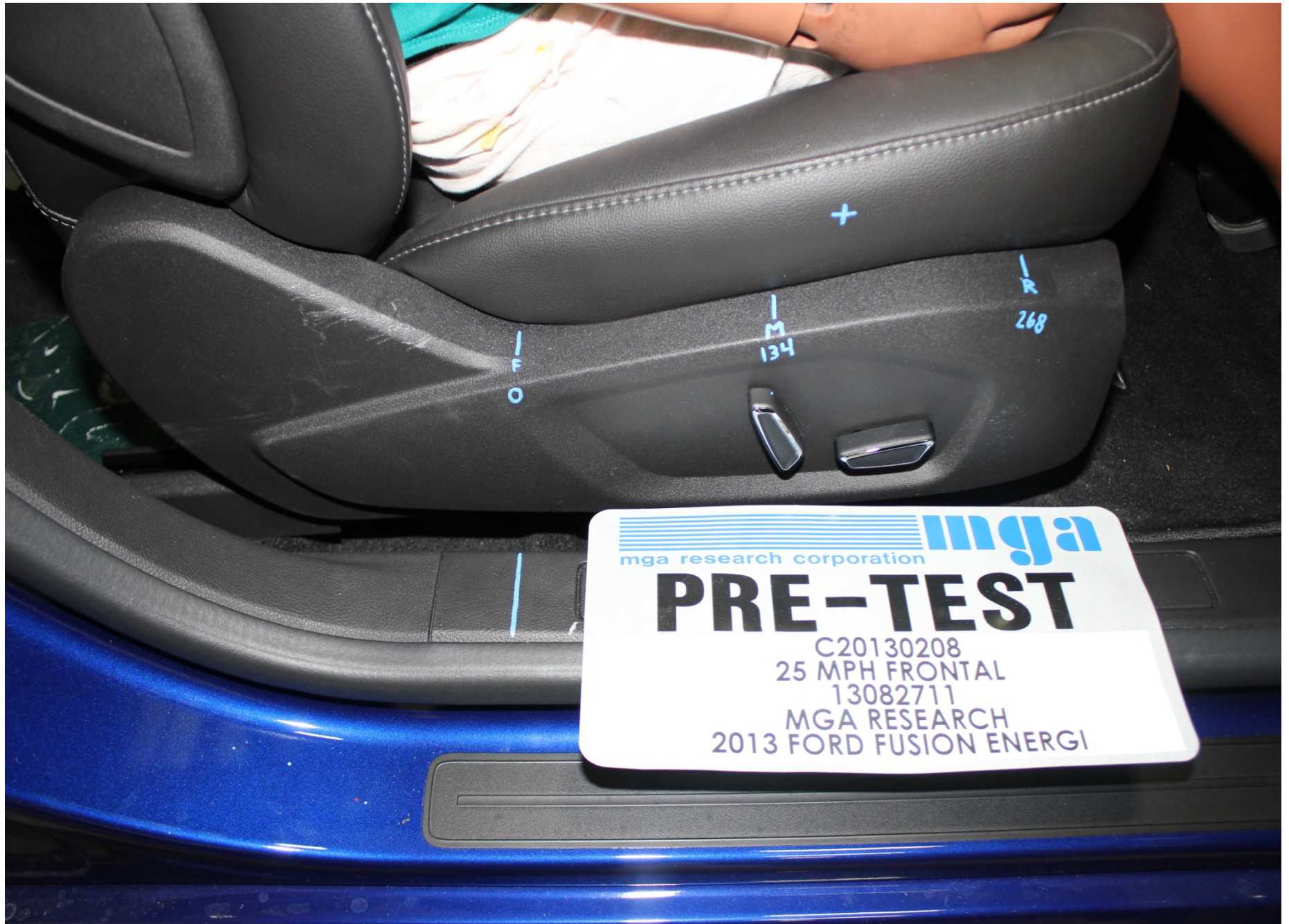
Pre-Test Passenger Dummy Seat Position
