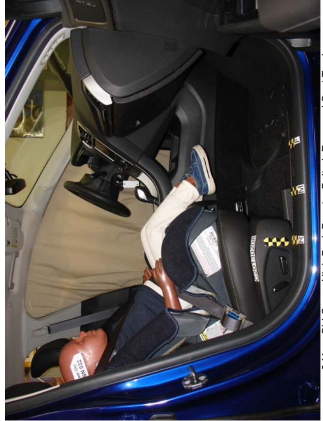
3-Year-Old Cosco High Back Booster Belted, Rearward Seat Track
