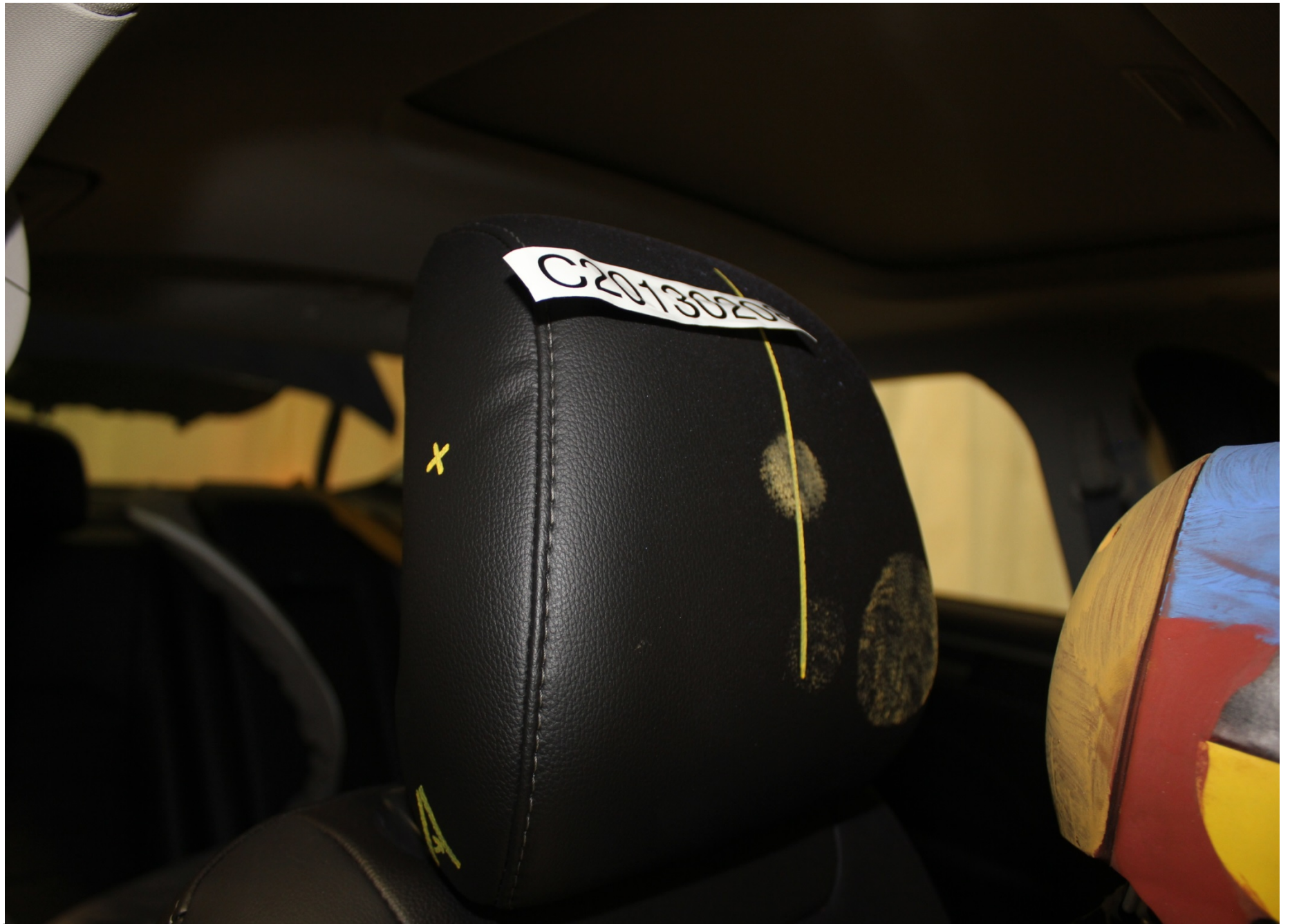
Post-Test Passenger Dummy Head Contact (visor)
