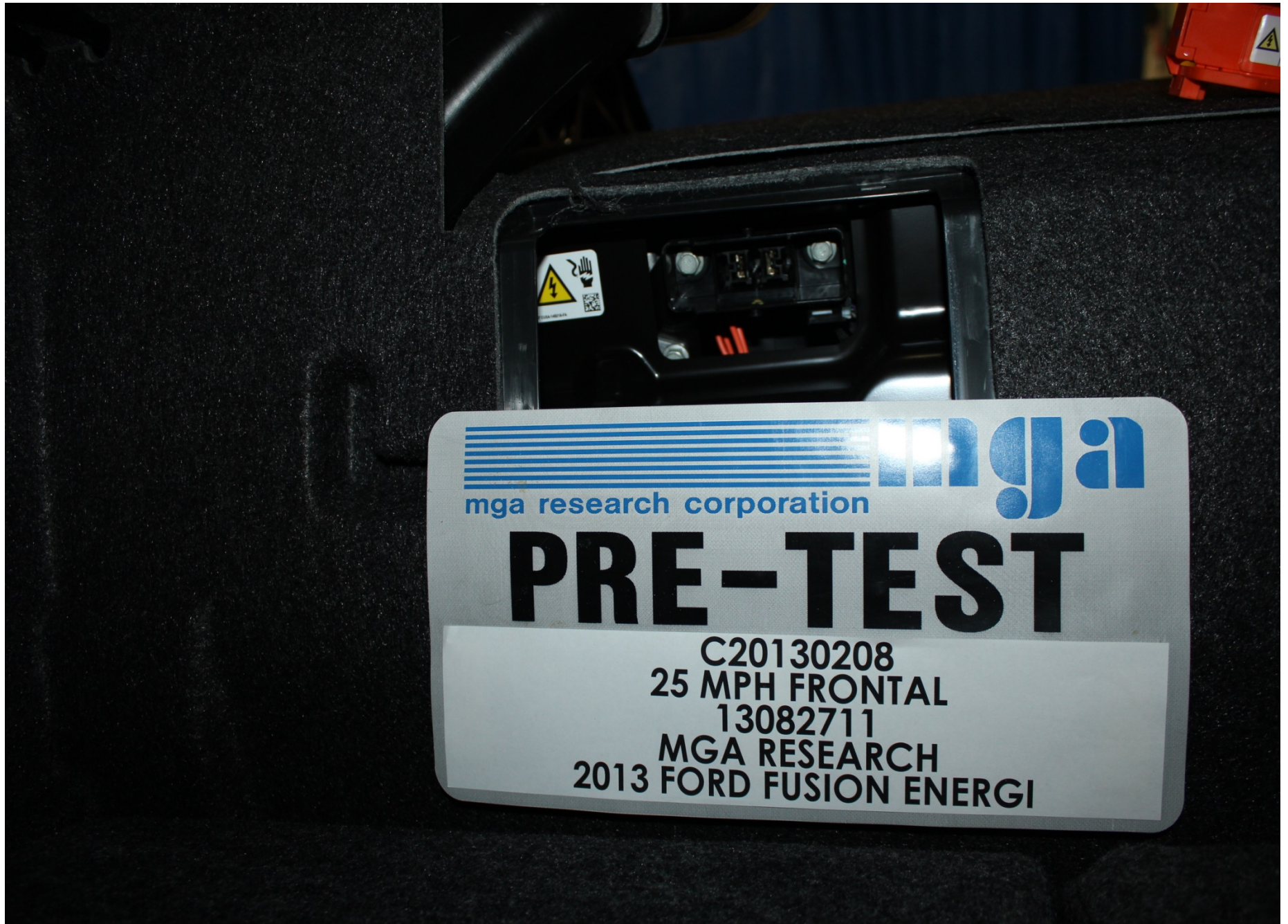
Pre-Test Manual High Voltage Service Disconnect Removed
