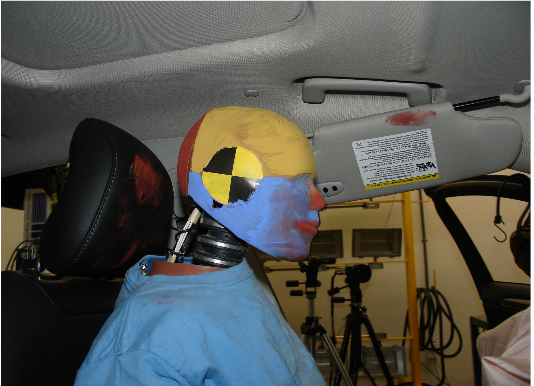
Post-Test 5th Fem. P2 Driver Dummy Head Contact (visor/ headrest)
