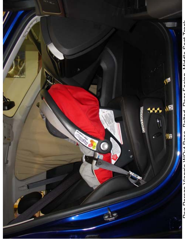
Peg Perego Viaggio W/Base, Unbelted, Forward Facing, Rearward Seat Track
