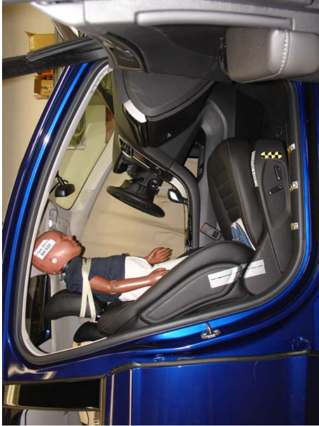
3-Year-Old Unbelted, Forward Seat Track, Position 5
