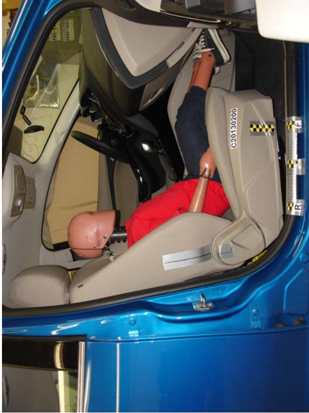
6-Year-Old Unbelted, Forward Seat Track, Position 1
