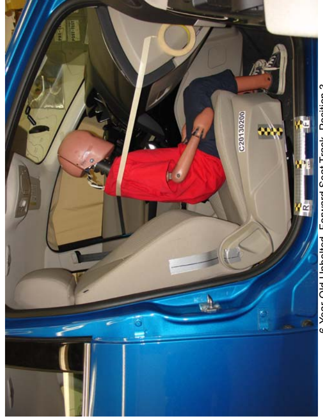
6-Year-Old Unbelted, Forward Seat Track, Position 3
