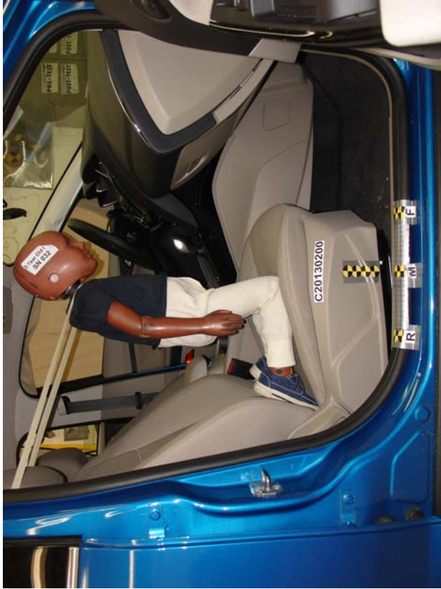
3-Year-Old Unbelted, Middle Seat Track, Position 6
