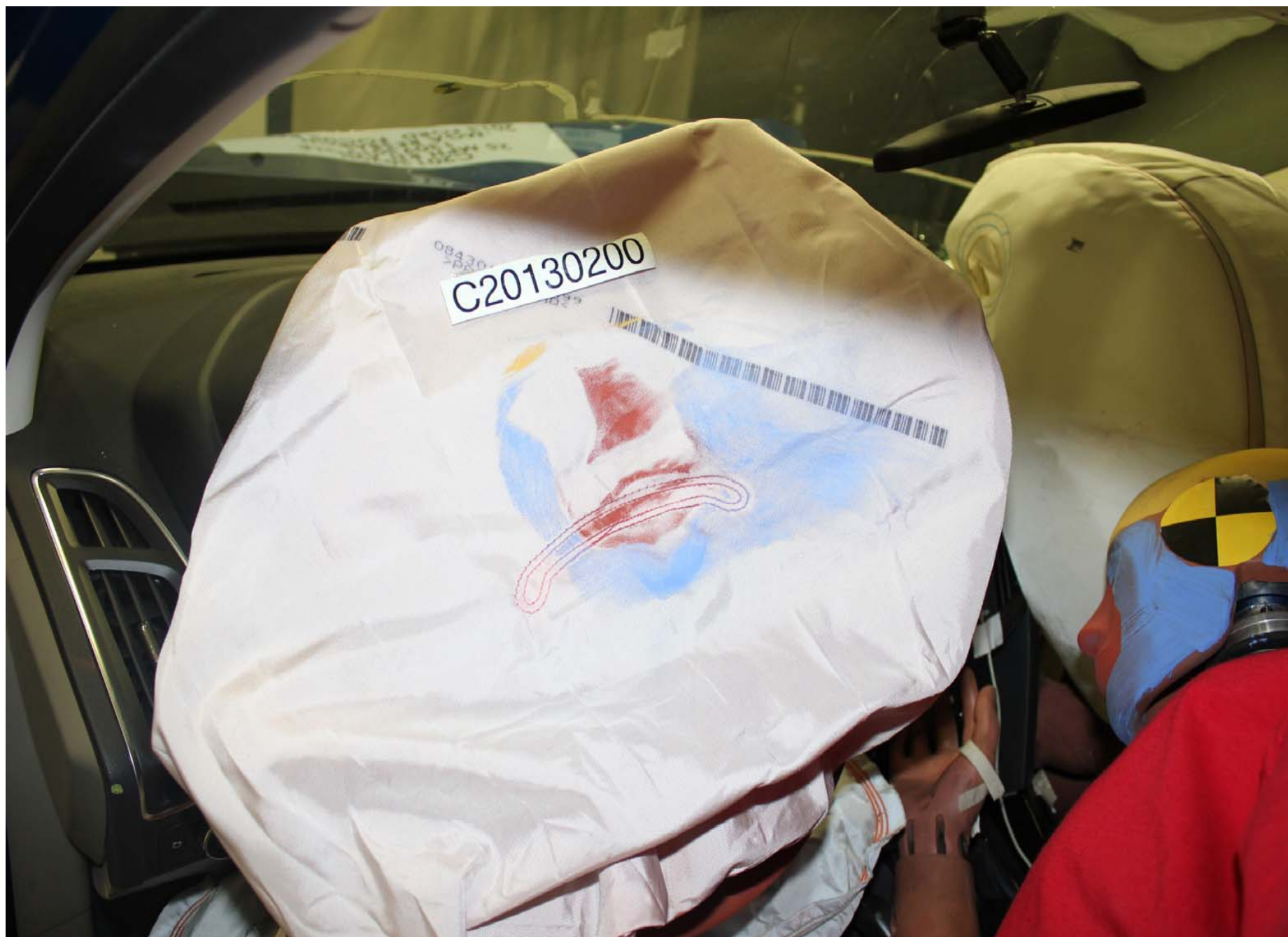
Post-Test Driver Dummy Airbag Contact
