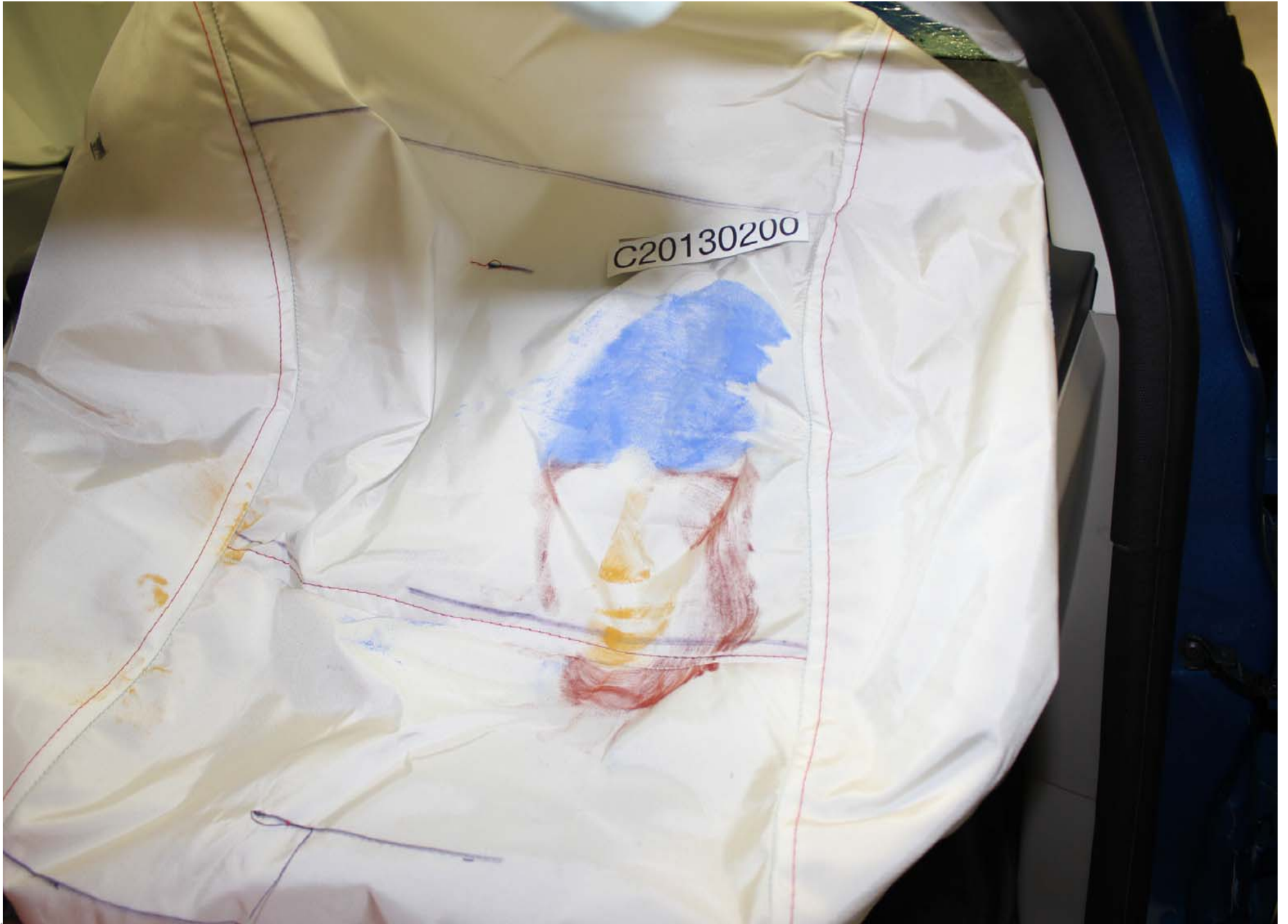
Post-Test Passenger Dummy Airbag Contact
