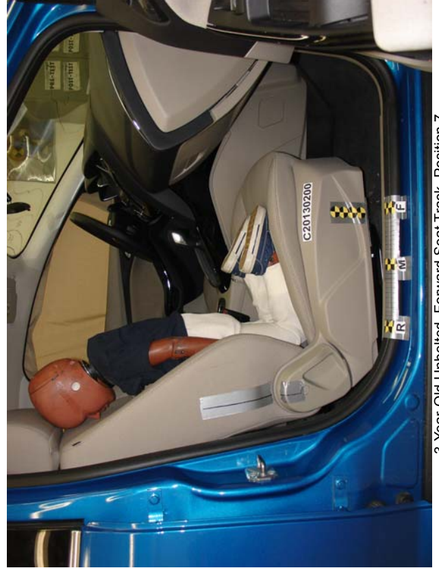
3-Year-Old Unbelted, Forward Seat Track, Position 7
