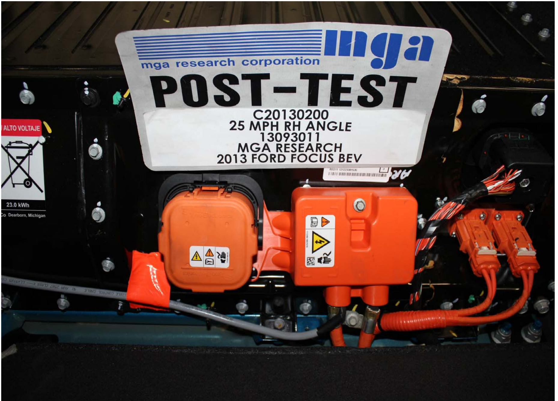
Post-Test Manual High Voltage Service Disconnect in Place
