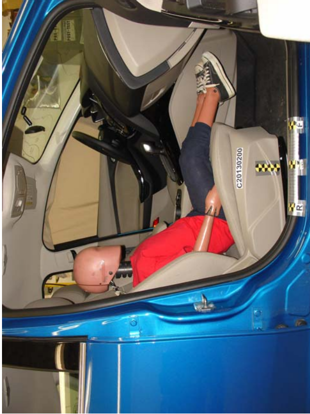
6-Year-Old Unbelted, Middle Seat Track, Position 1
