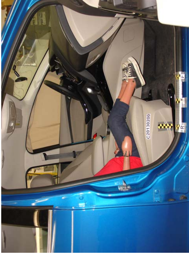
6-Year-Old Unbelted, Rearward Seat Track, Position 2
