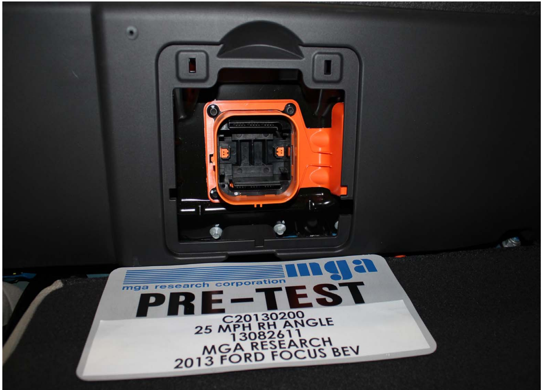
Pre-Test Manual High Voltage Service Disconnect Removed
