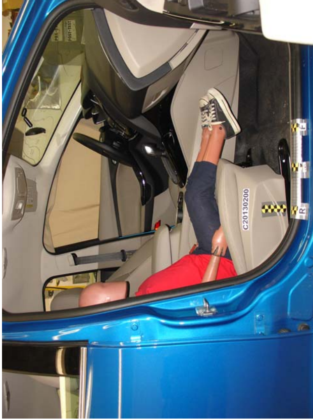
6-Year-Old Unbelted, Rearward Seat Track, Position 1
