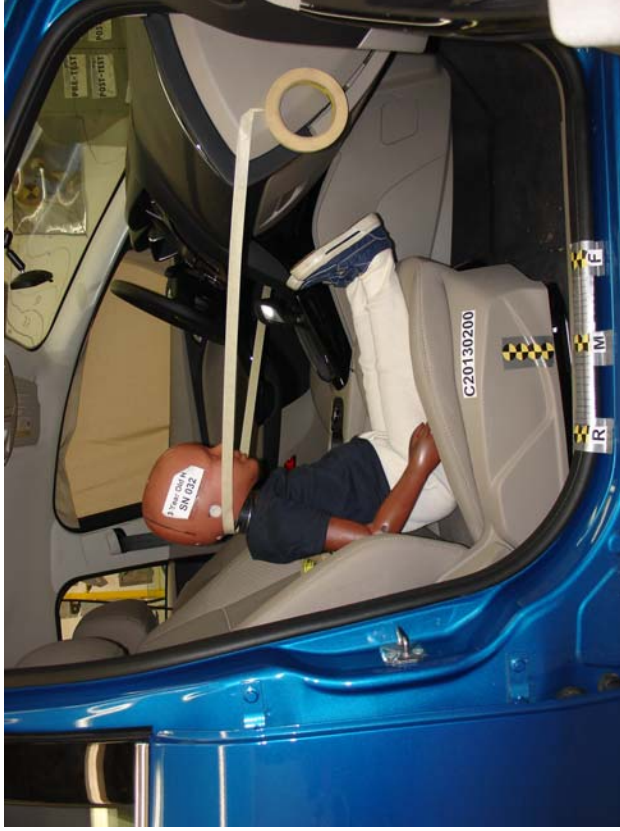
3-Year-Old Unbelted, Middle Seat Track, Position 3
