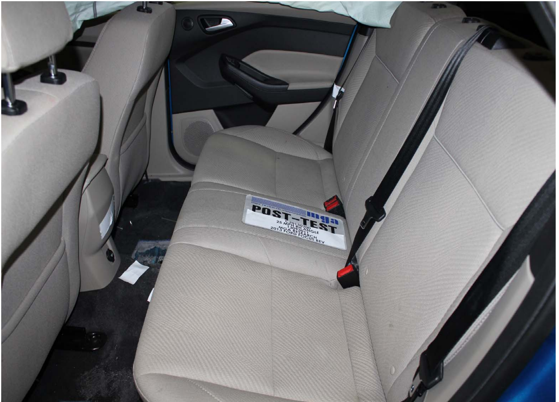
Post-Test Passenger Compartment Adjacent to Electric Energy Storage System
