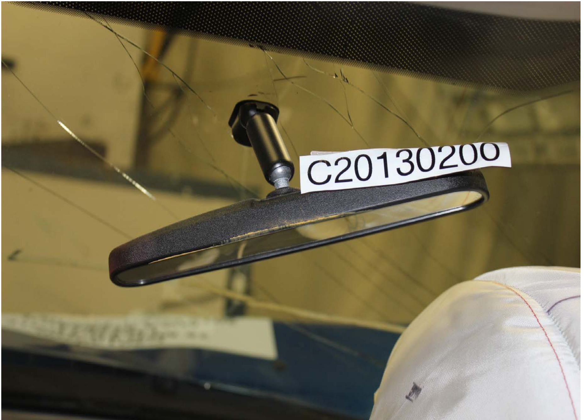
Post-Test Driver Dummy Head Contact (rearview mirror)
