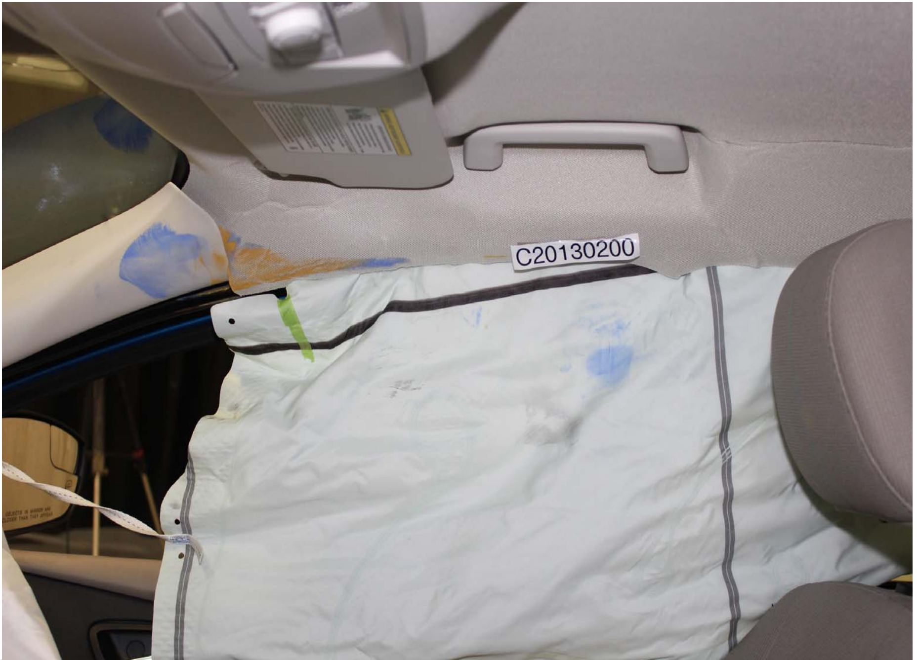
Post-Test Passenger Dummy Head Contact (A-post/headliner)
