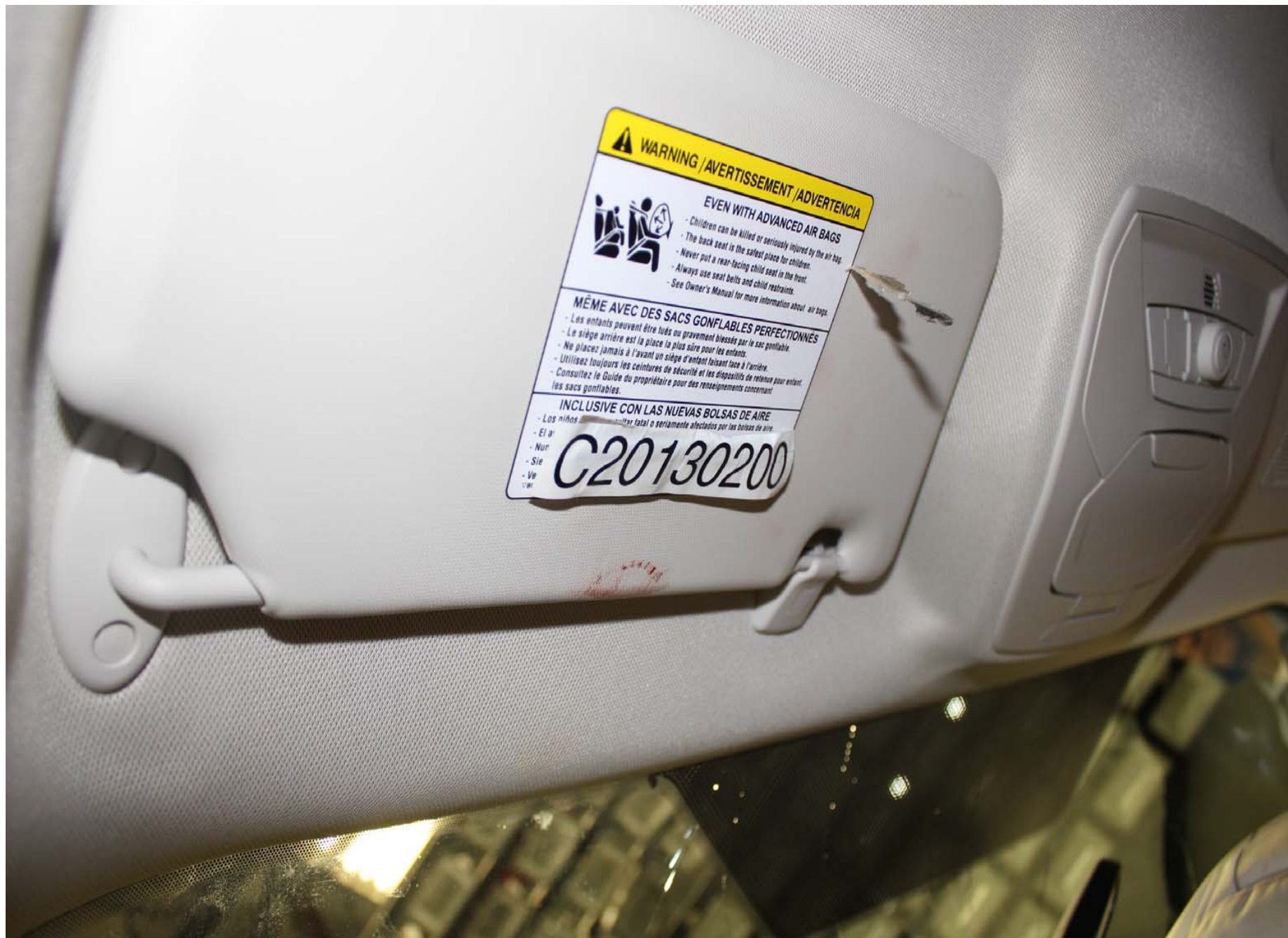
Post-Test Driver Dummy Head Contact (visor)
