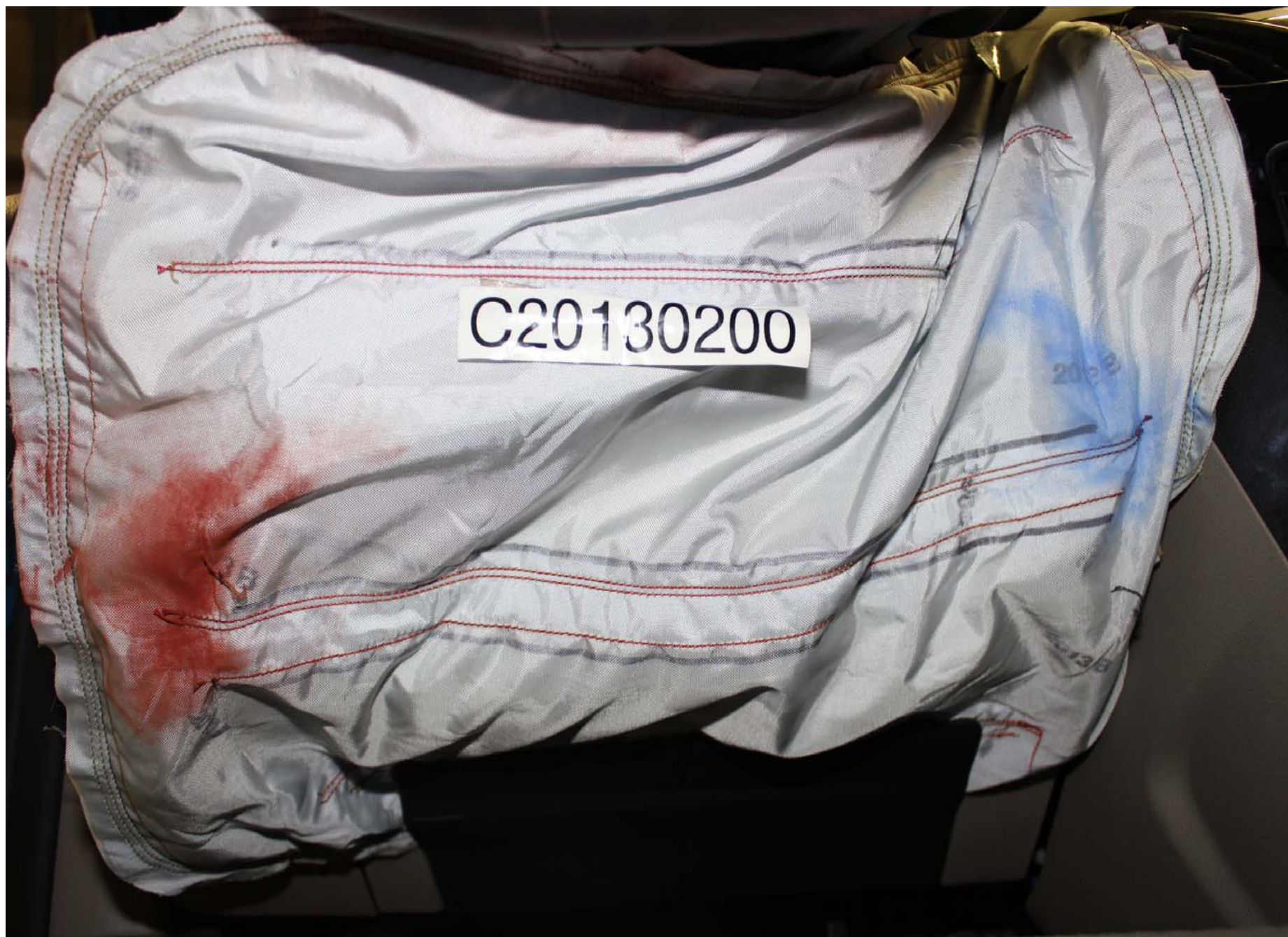
Post-Test Driver Dummy Knee Contact
