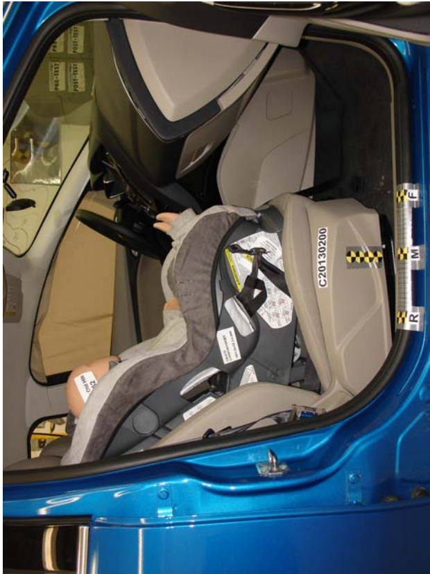
Graco Comfortsport Forward Facing Unbelted, Middle Seat Track
