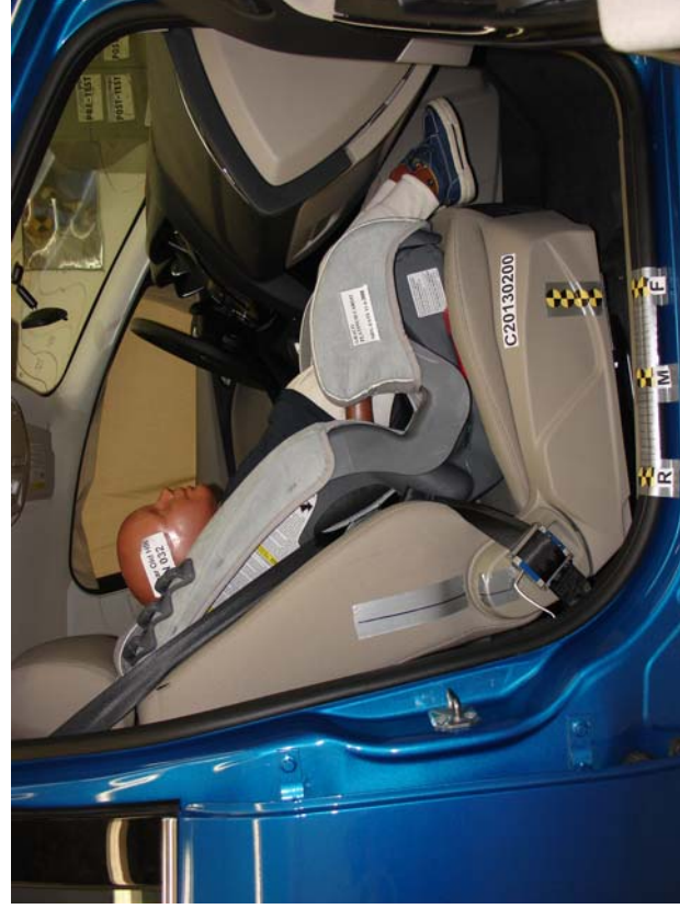
3-Year-Old Graco Platinum Cargo Belted With Harness, Forward Seat Track
