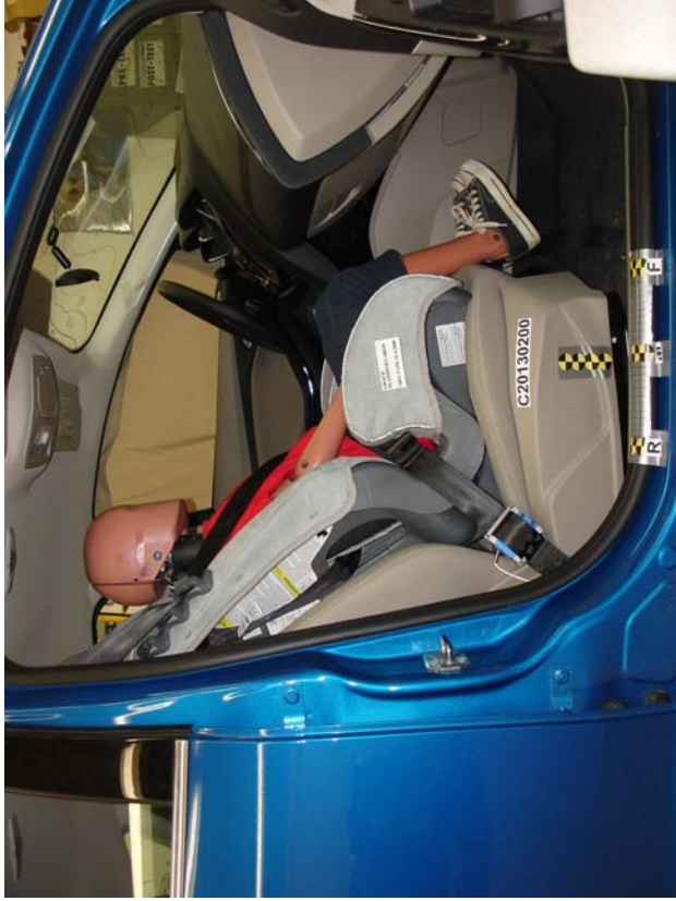
6-Year-Old Graco Platinum Cargo Belted, Middle Seat Track
