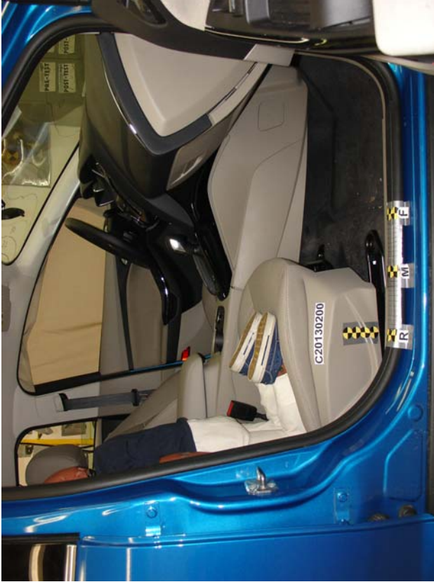
3-Year-Old Unbelted, Rearward Seat Track, Position 7
