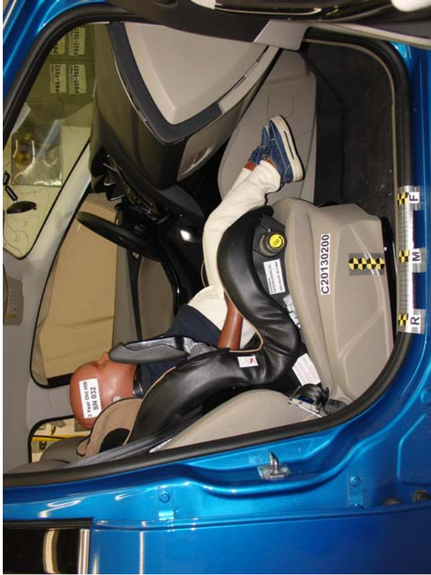
3-Year-Old Forward Facing Evenflo Generations Cinched With Harness, Middle Seat
