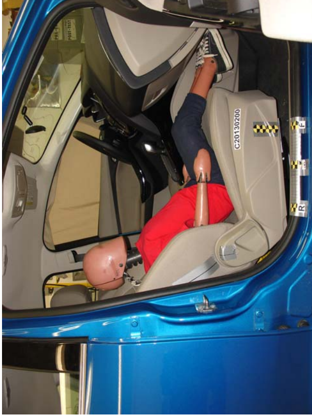
6-Year-Old Unbelted, Forward Seat Track, Position 2
