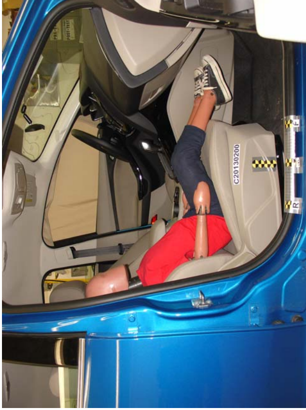
6-Year-Old Unbelted, Middle Seat Track, Position 2
