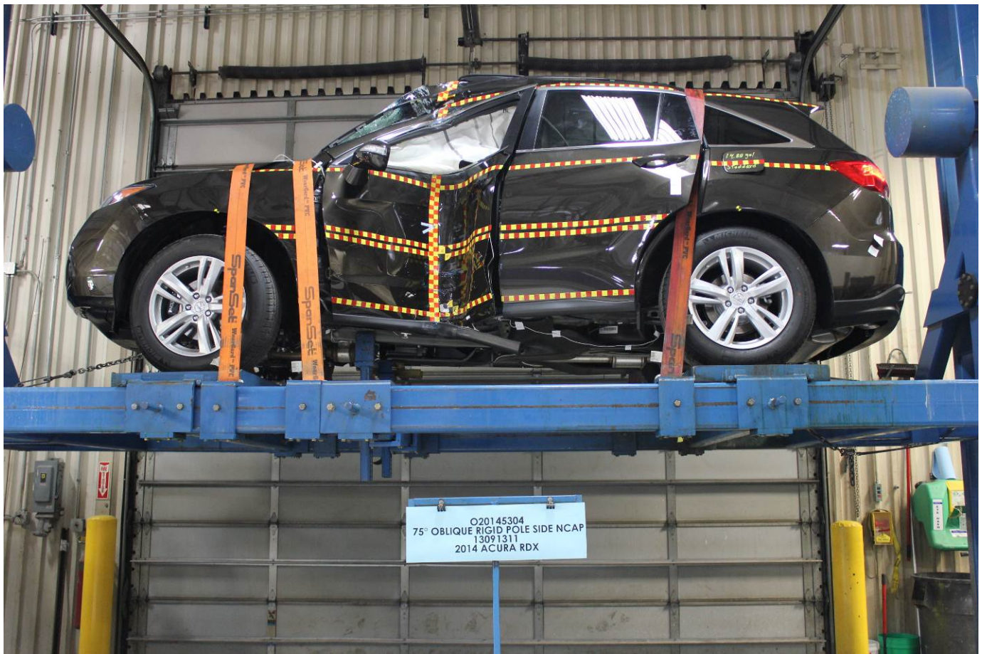
FMVSS No. 301 Static Rollover 360 Degrees
