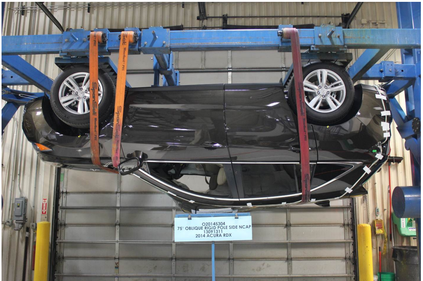
FMVSS No. 301 Static Rollover 180 Degrees
