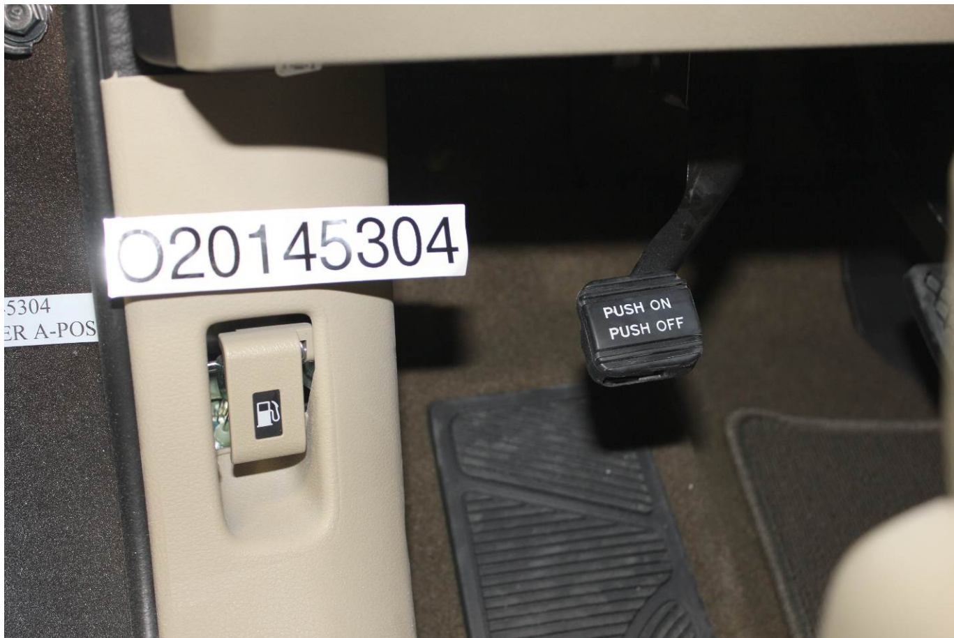
Pre-Test View of Disengaged Parking Brake
