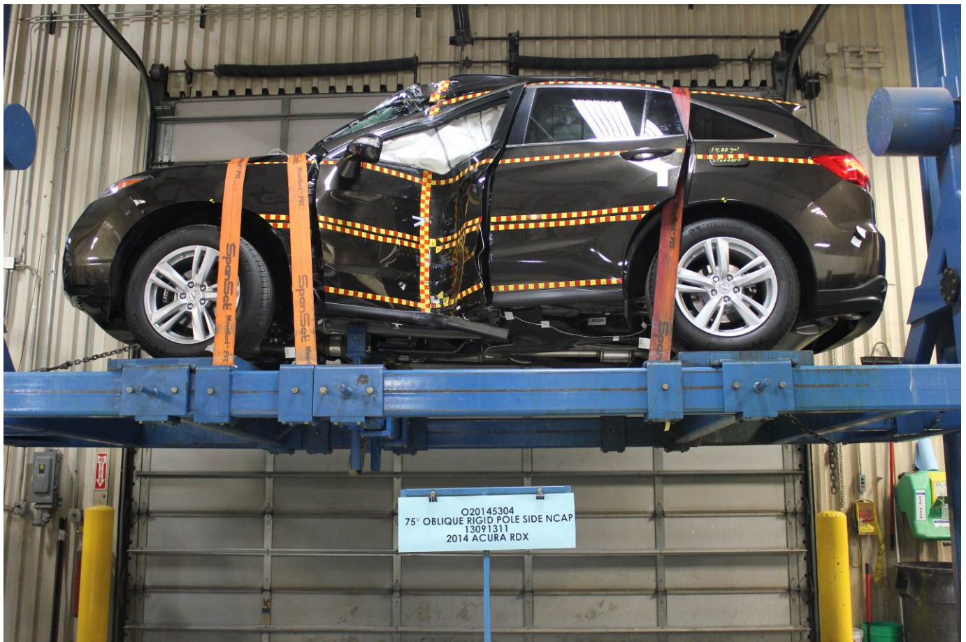
FMVSS No. 301 Static Rollover 0 Degrees
