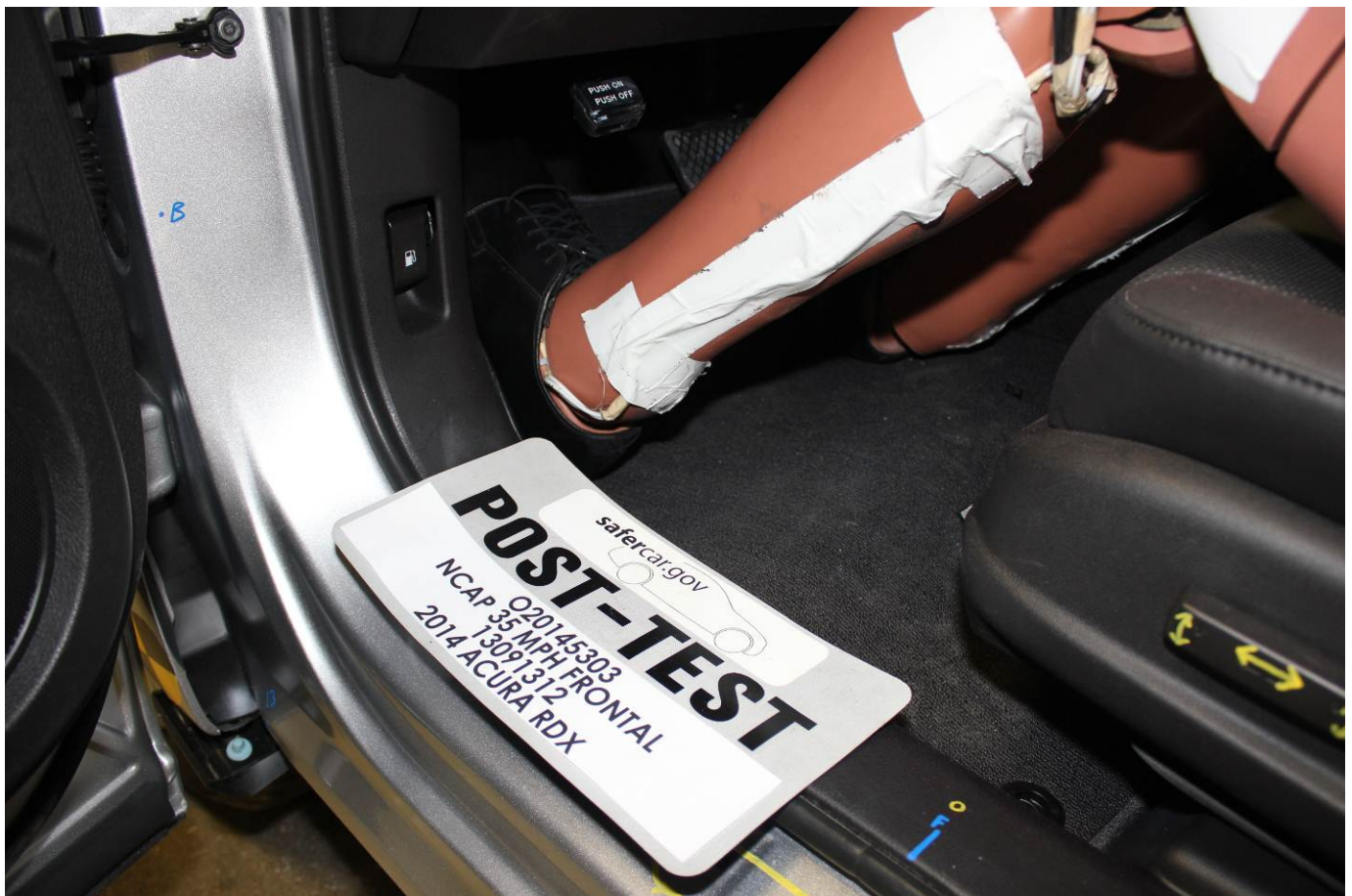
Post-Test Driver Dummy Feet
