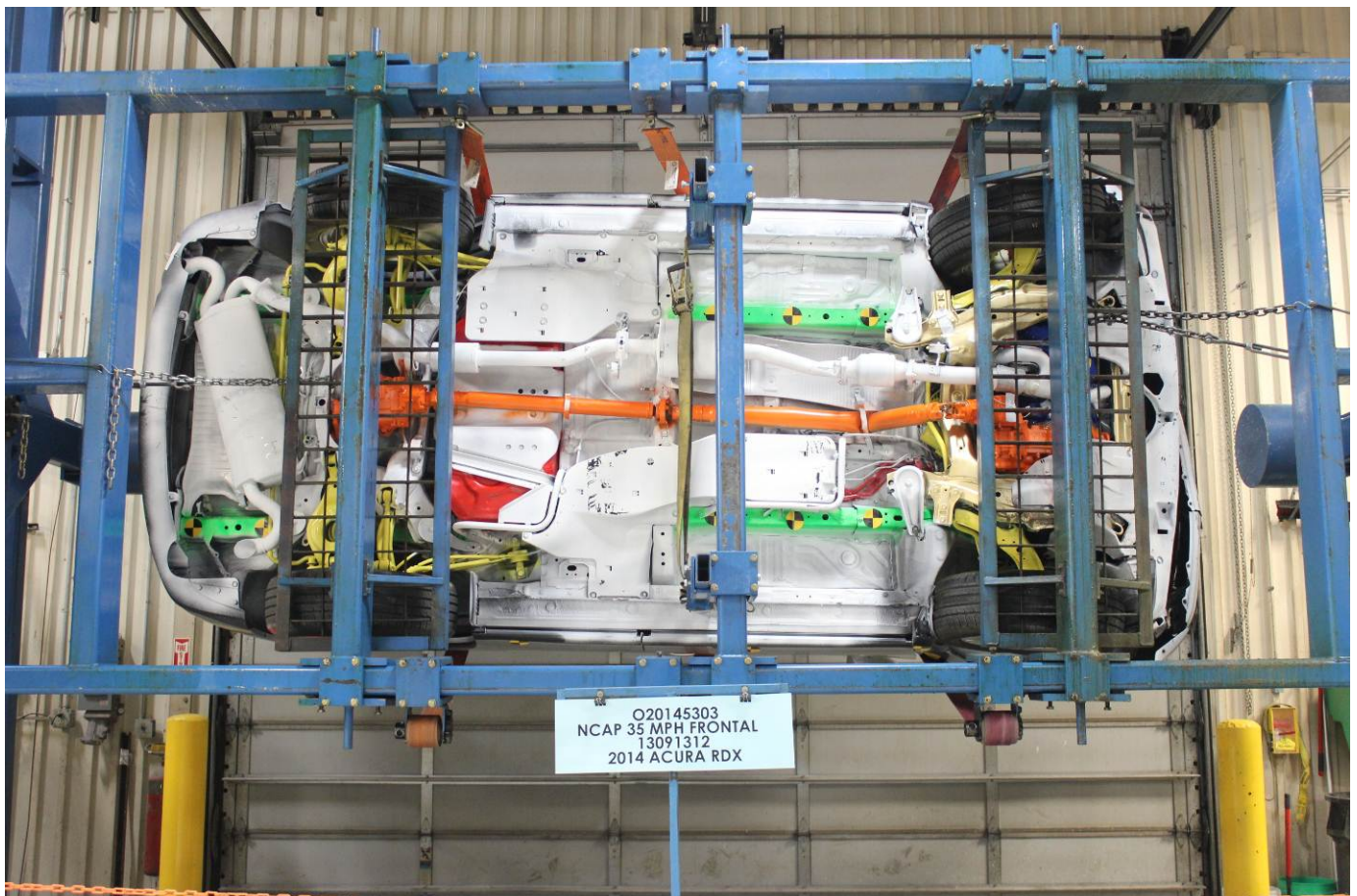
Vehicle at 90 Degrees on Static Rollover Device
