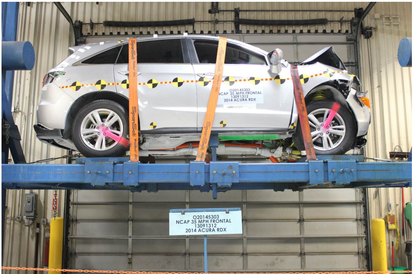
Vehicle at 0 Degree on Static Rollover Device
