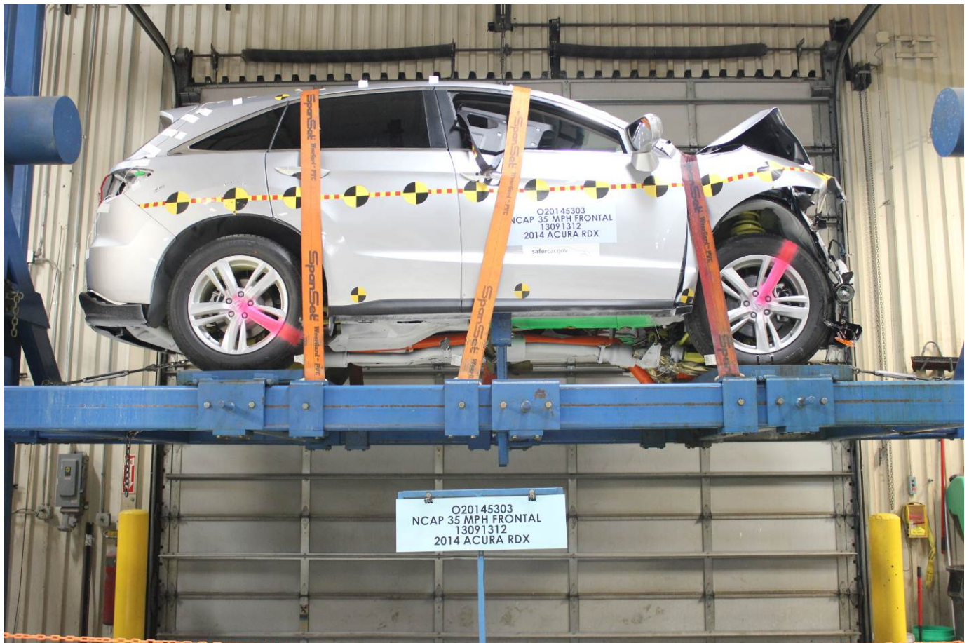
Vehicle at 360 Degrees on Static Rollover Device
