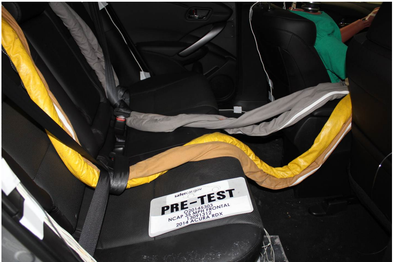
Pre-Test Dummy Cable Routing
