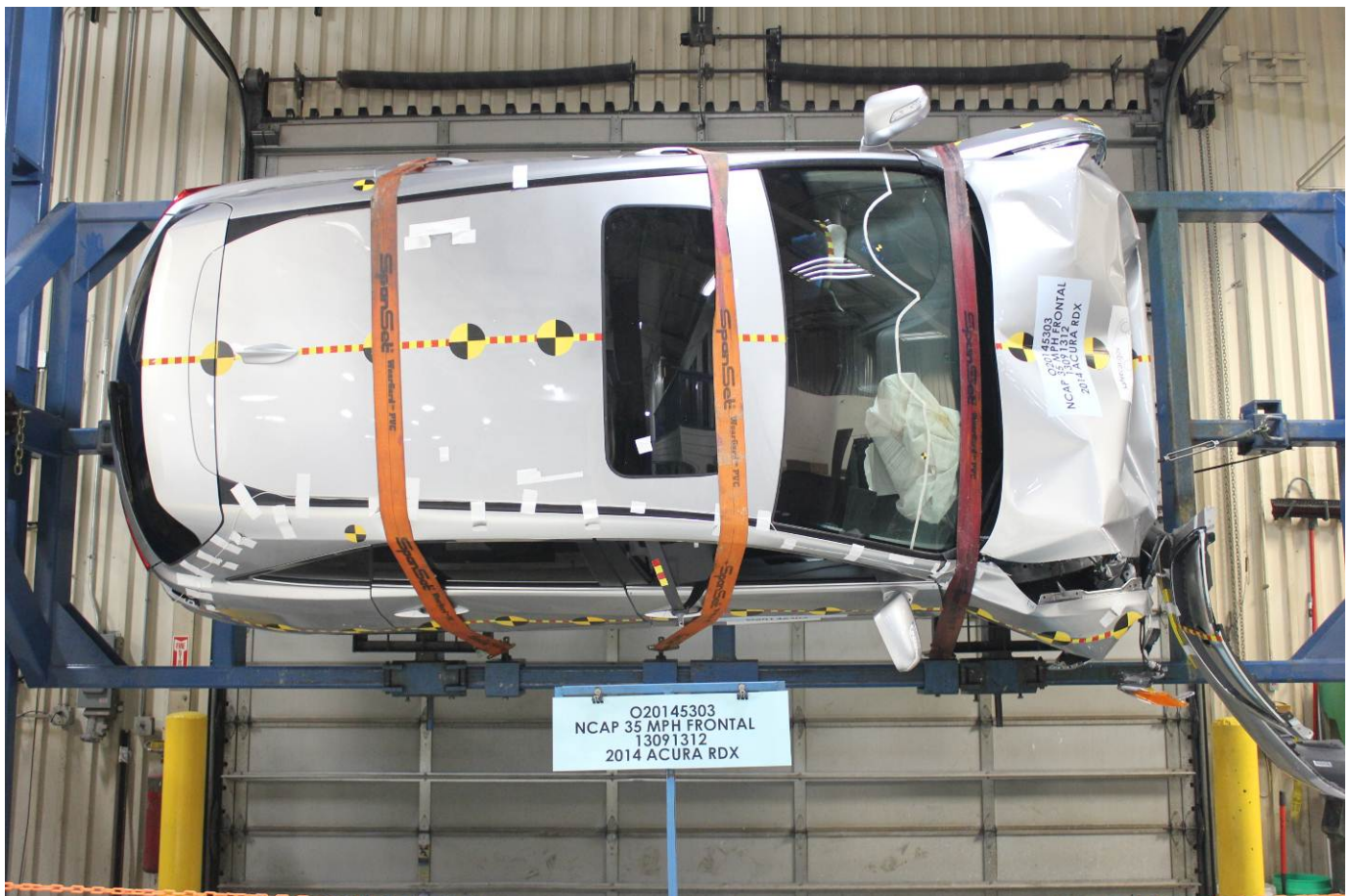
Vehicle at 270 Degrees on Static Rollover Device
