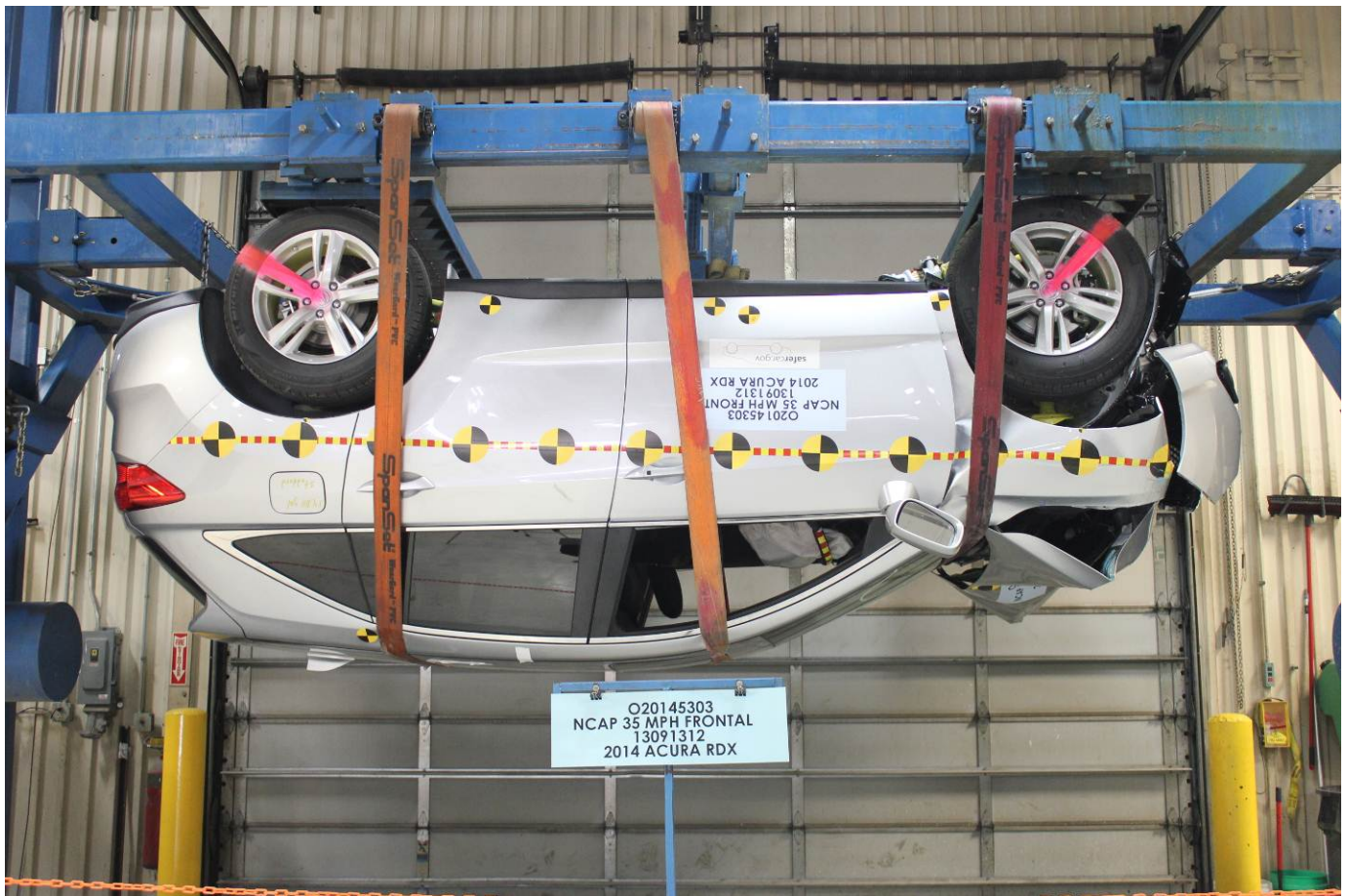
Vehicle at 180 Degrees on Static Rollover Device
