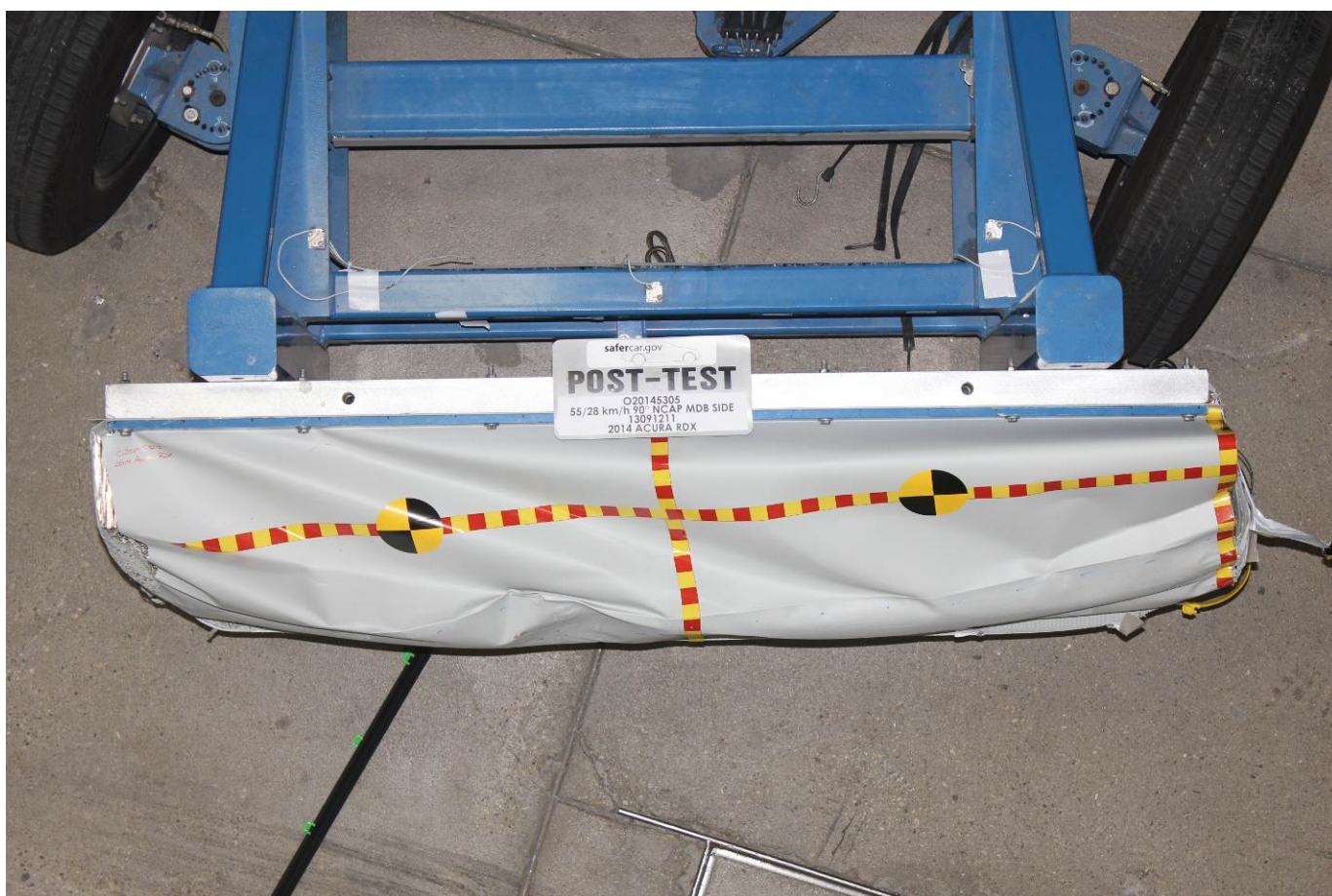
Post-Test Top View of MDB Impactor Face
