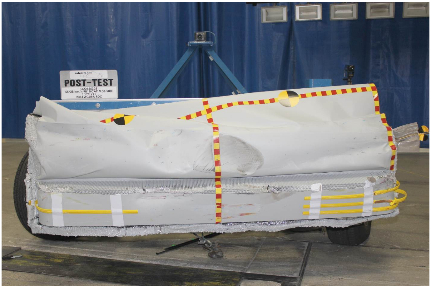
Post-Test Front View of MDB Impactor Face
