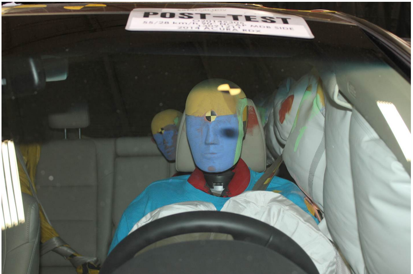
Post-Test Front Close-Up View of Driver Dummy
