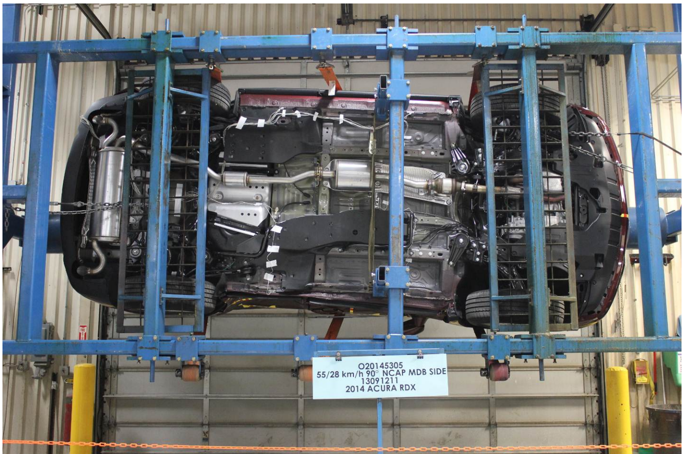
FMVSS No. 301 Static Rollover 90 Degrees
