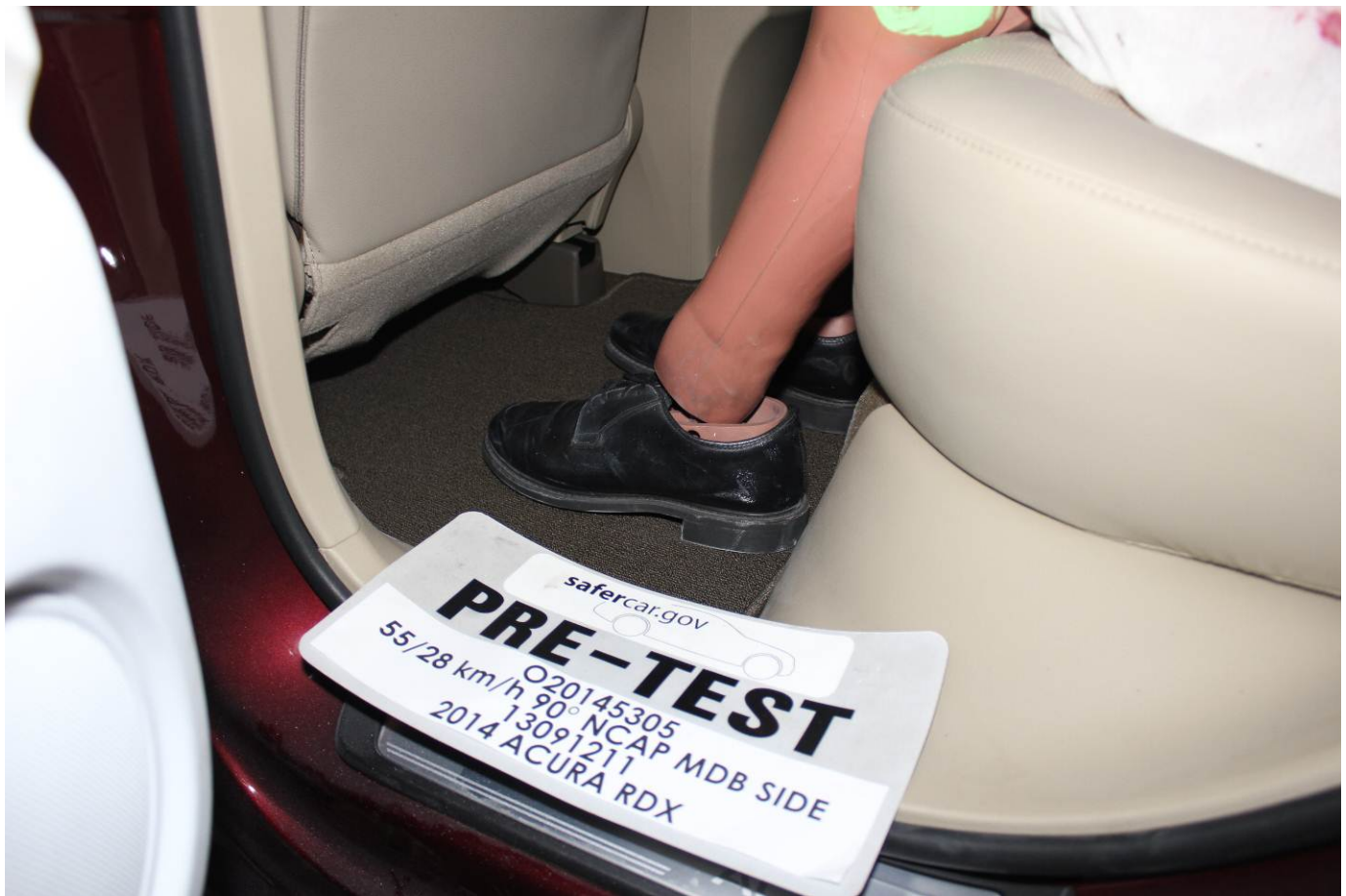
Pre-Test Placement of Rear Passenger Dummy's Feet
