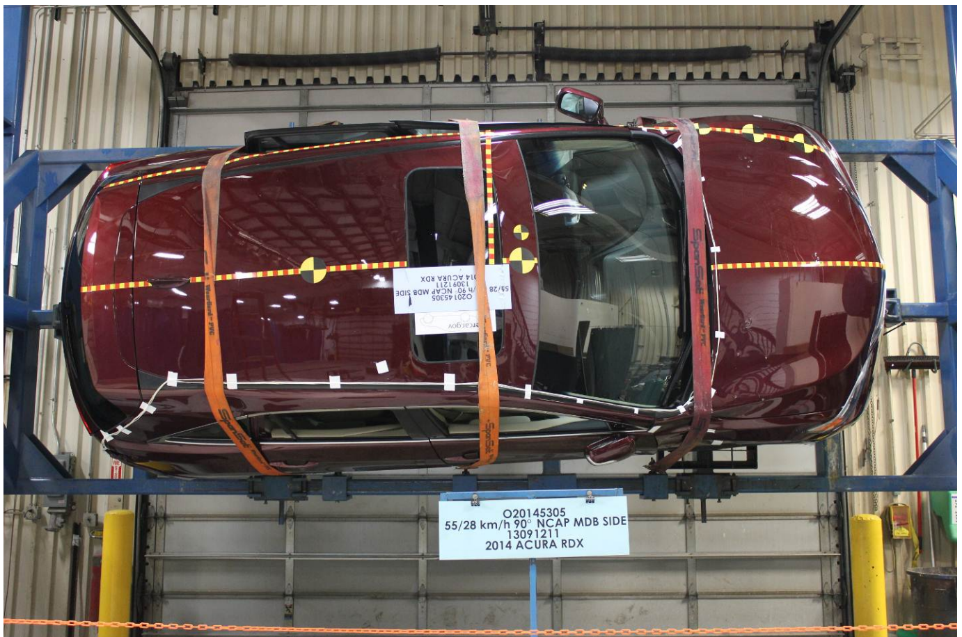
FMVSS No. 301 Static Rollover 270 Degrees
