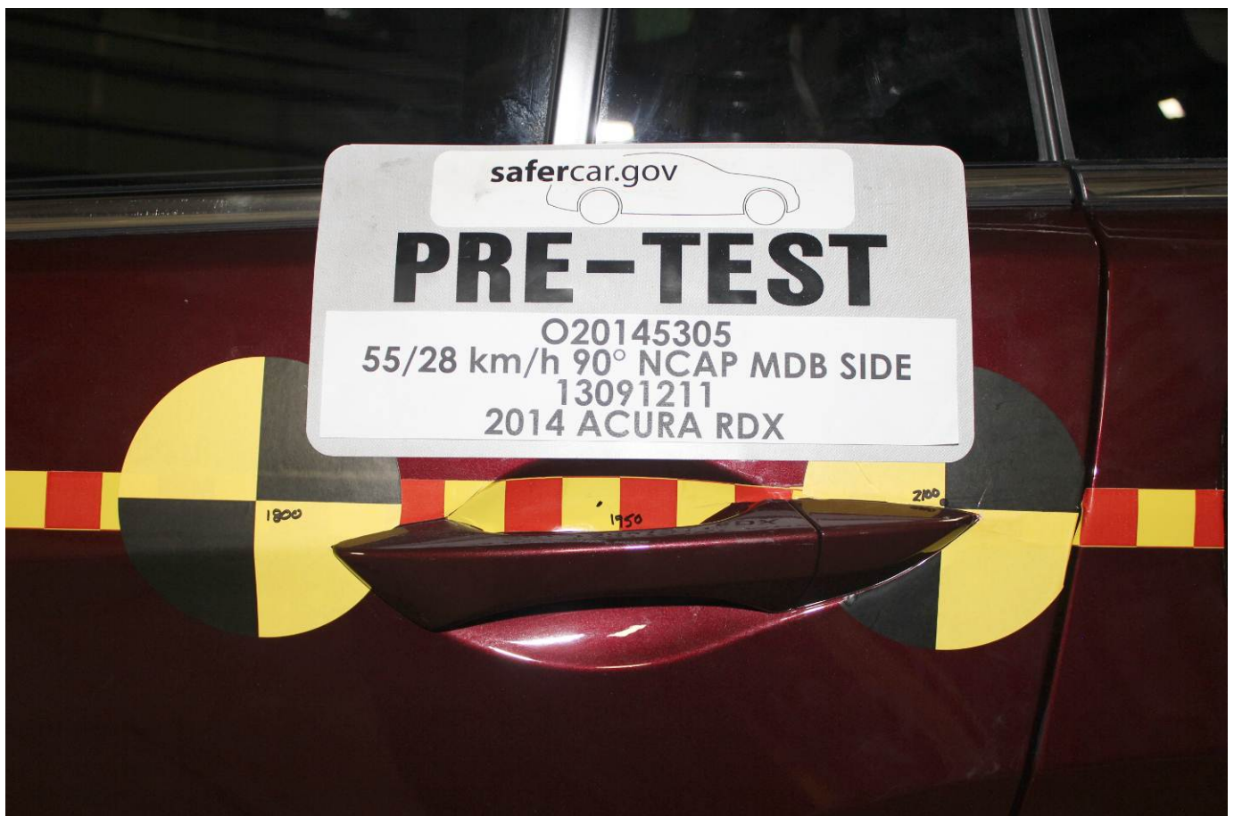
Pre-Test Left Rear Door Latch Close-Up
