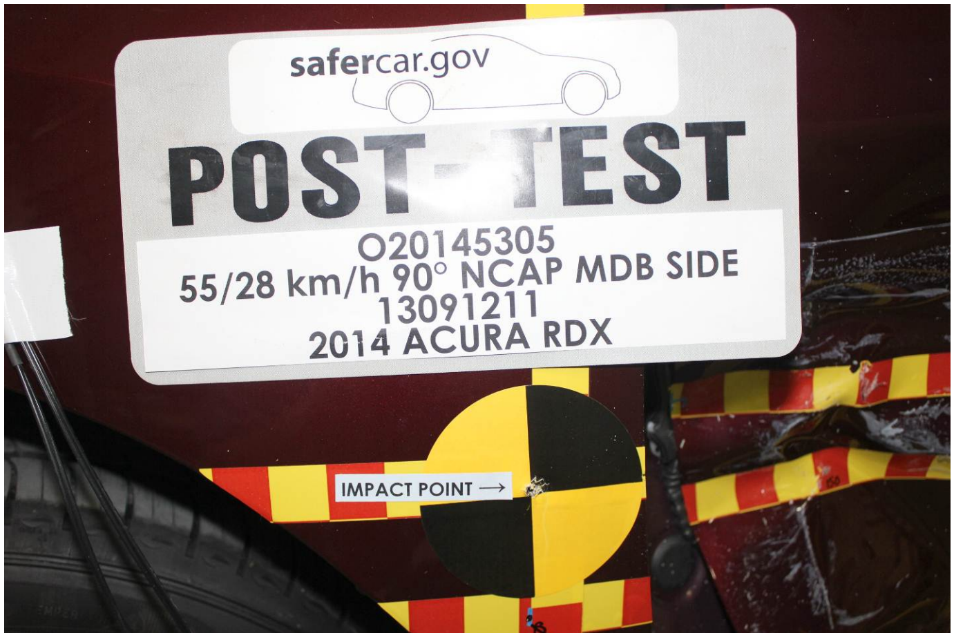
Post-Test Close-Up View of Impact Point Target
