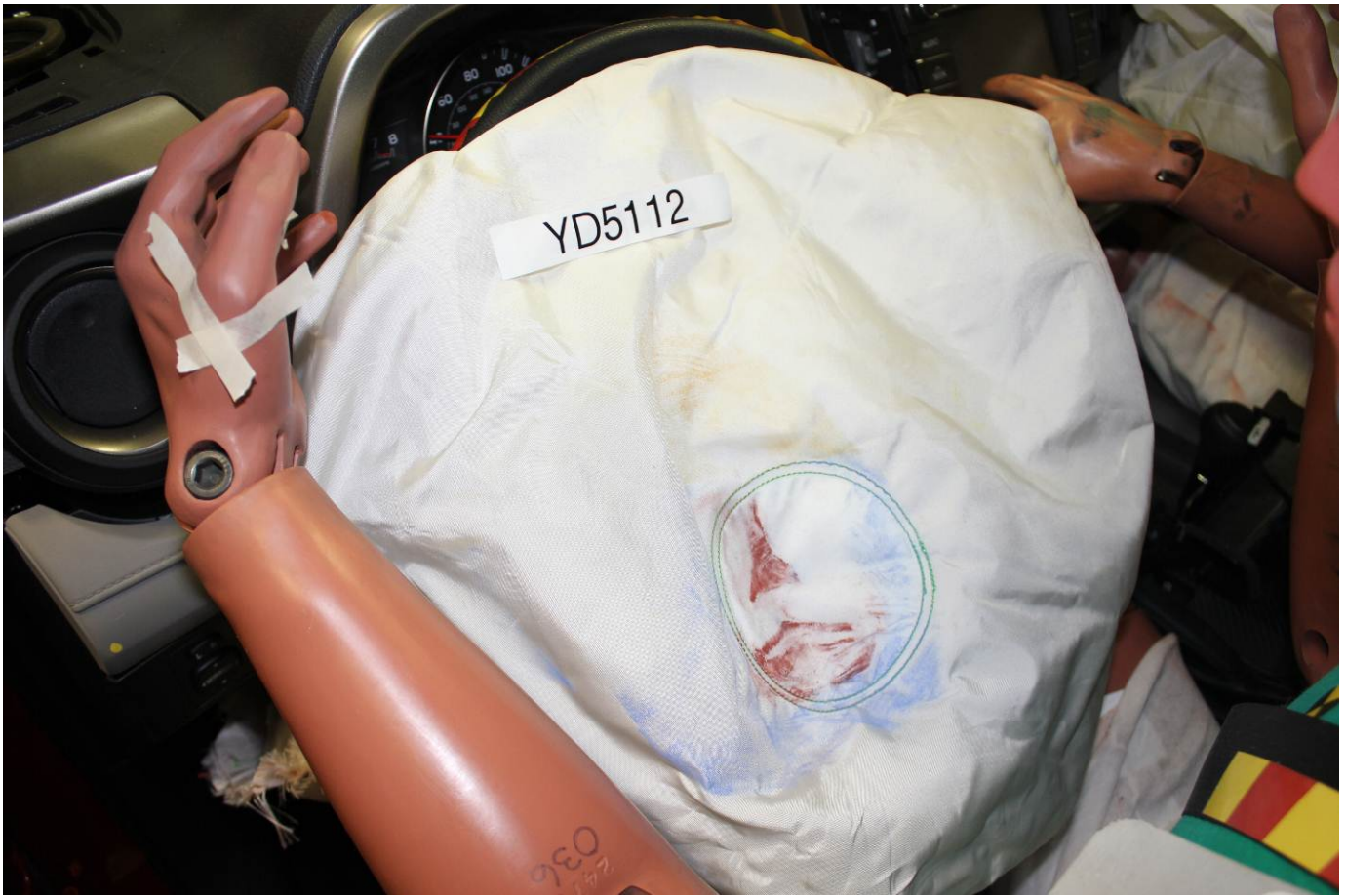
Post-Test Driver Dummy Contact with Airbag
