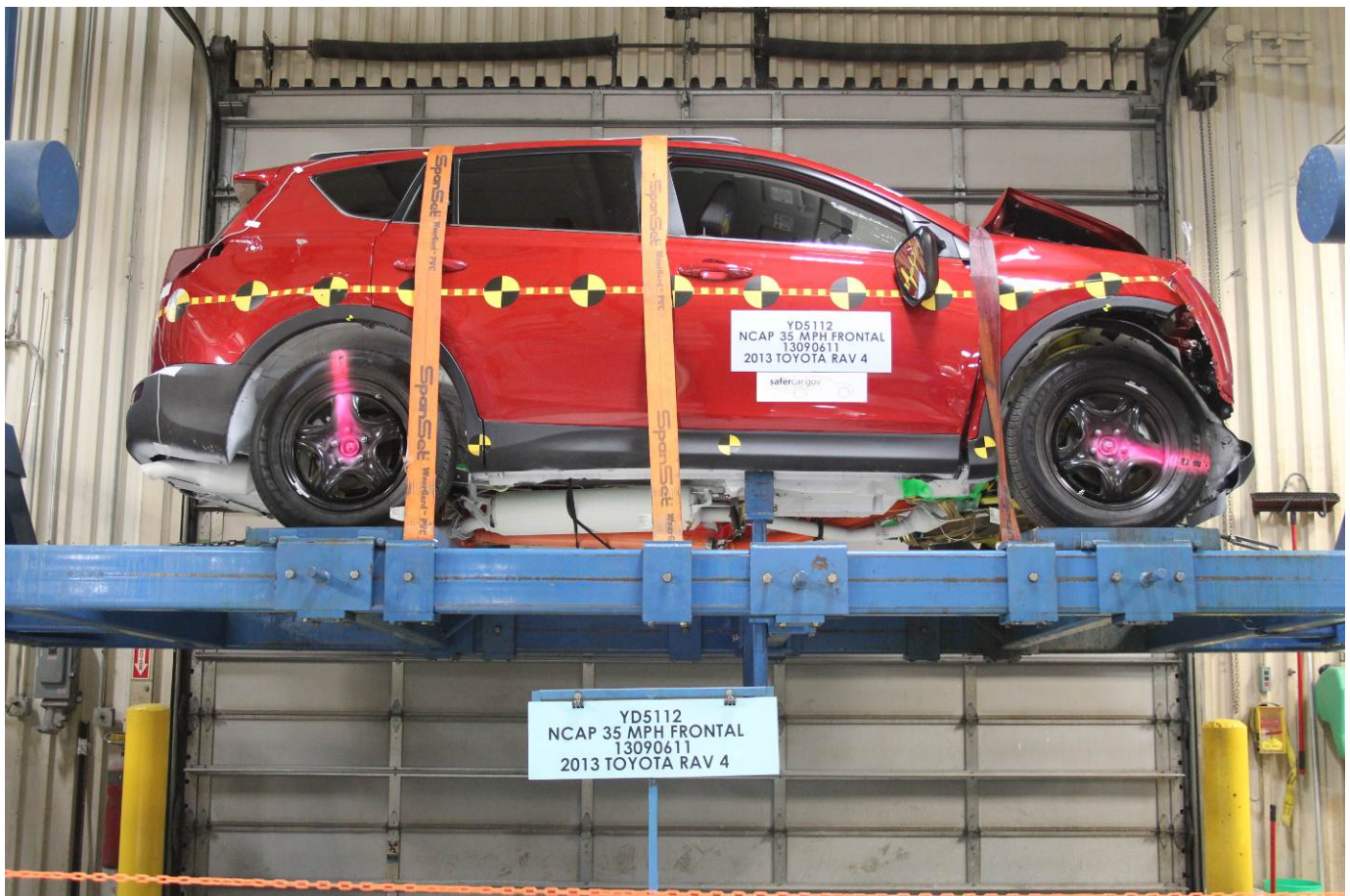
Vehicle at 0 Degree on Static Rollover Device
