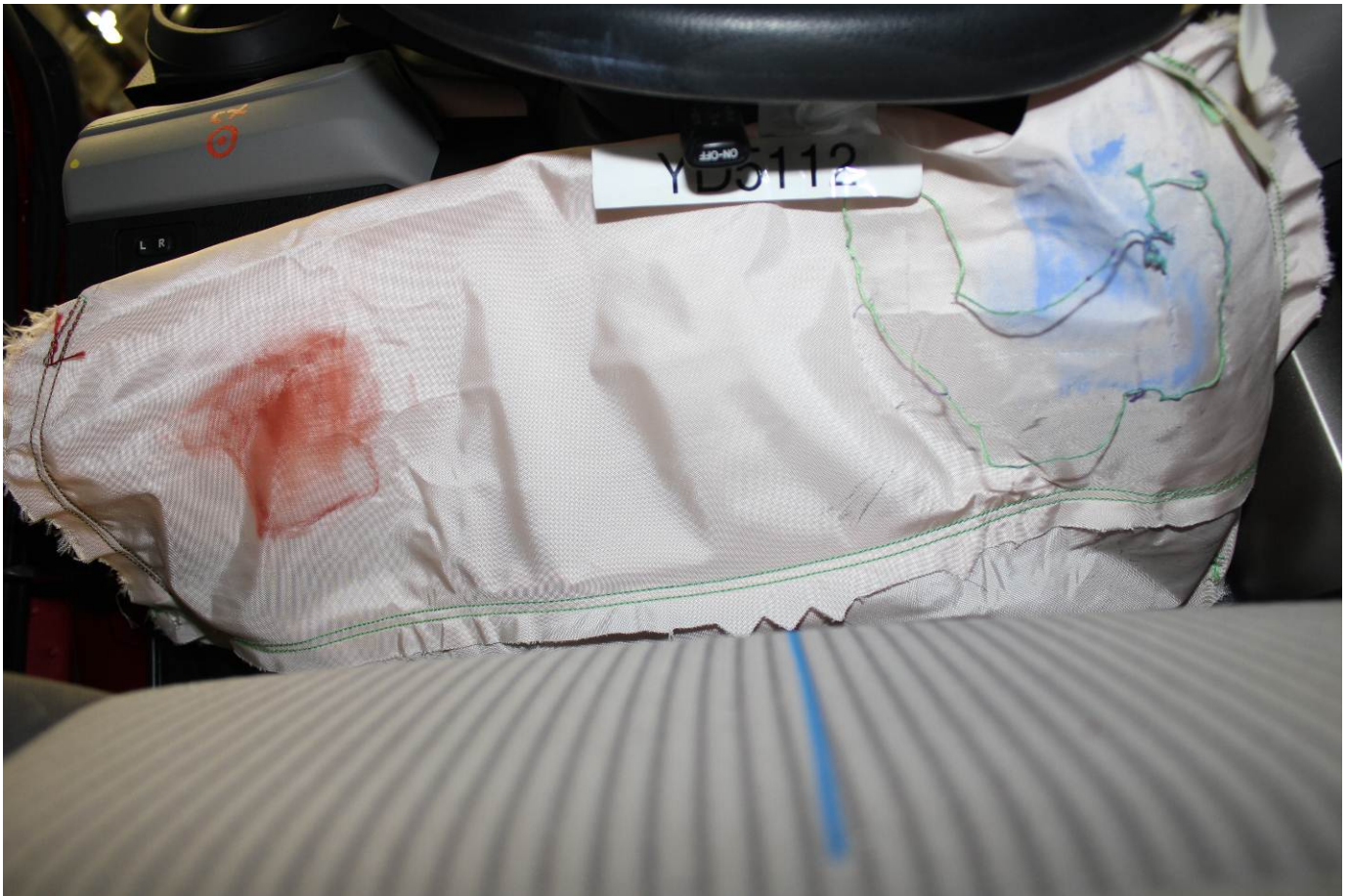
Post-Test Driver Dummy Contact with Knee Airbag
