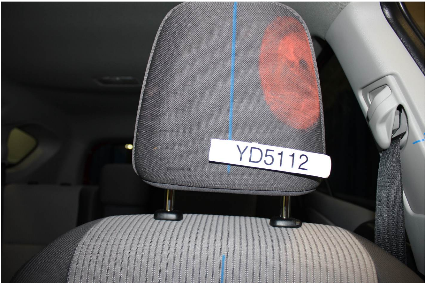
Post-Test Driver Dummy Contact with Headrest
