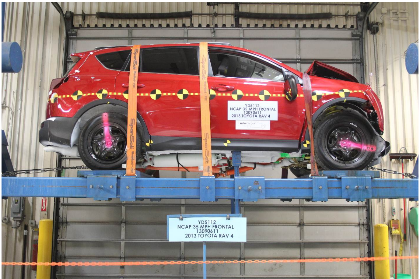
Vehicle at 360 Degrees on Static Rollover Device
