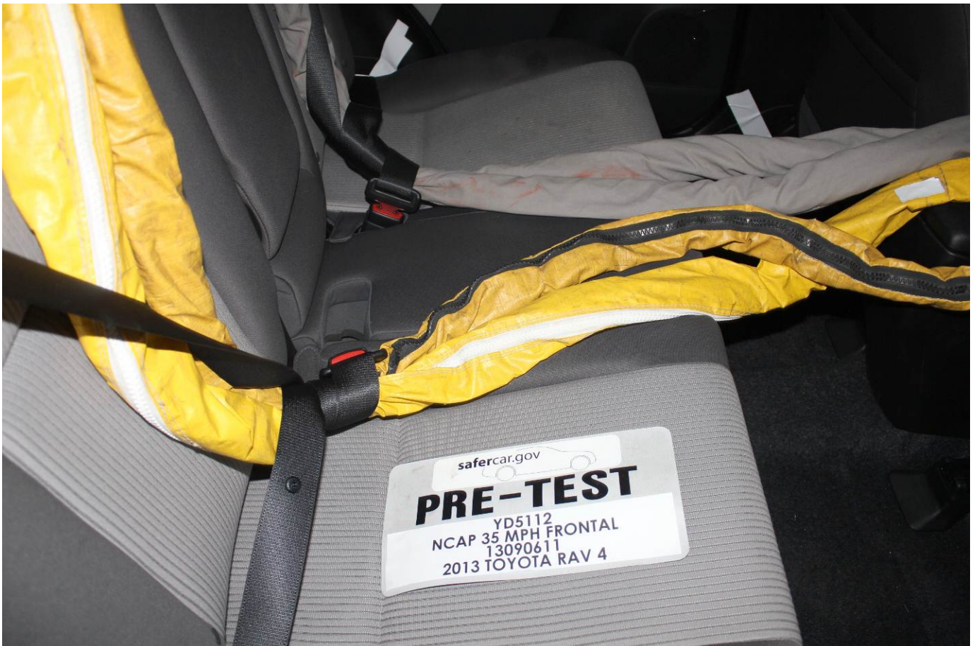
Pre-Test Dummy Cable Routing
