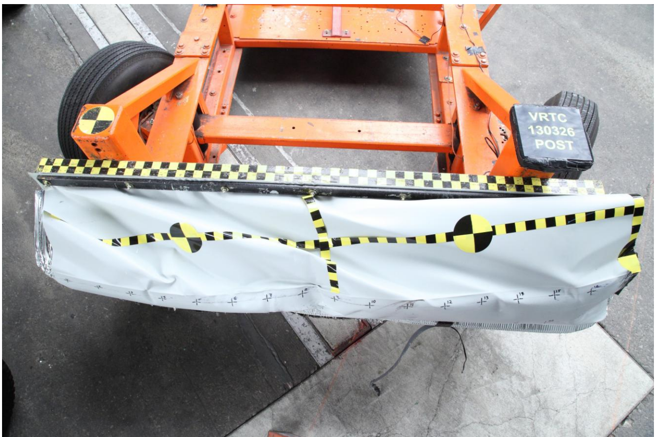
Figure A-46 Post-Test MDB Face Top View
