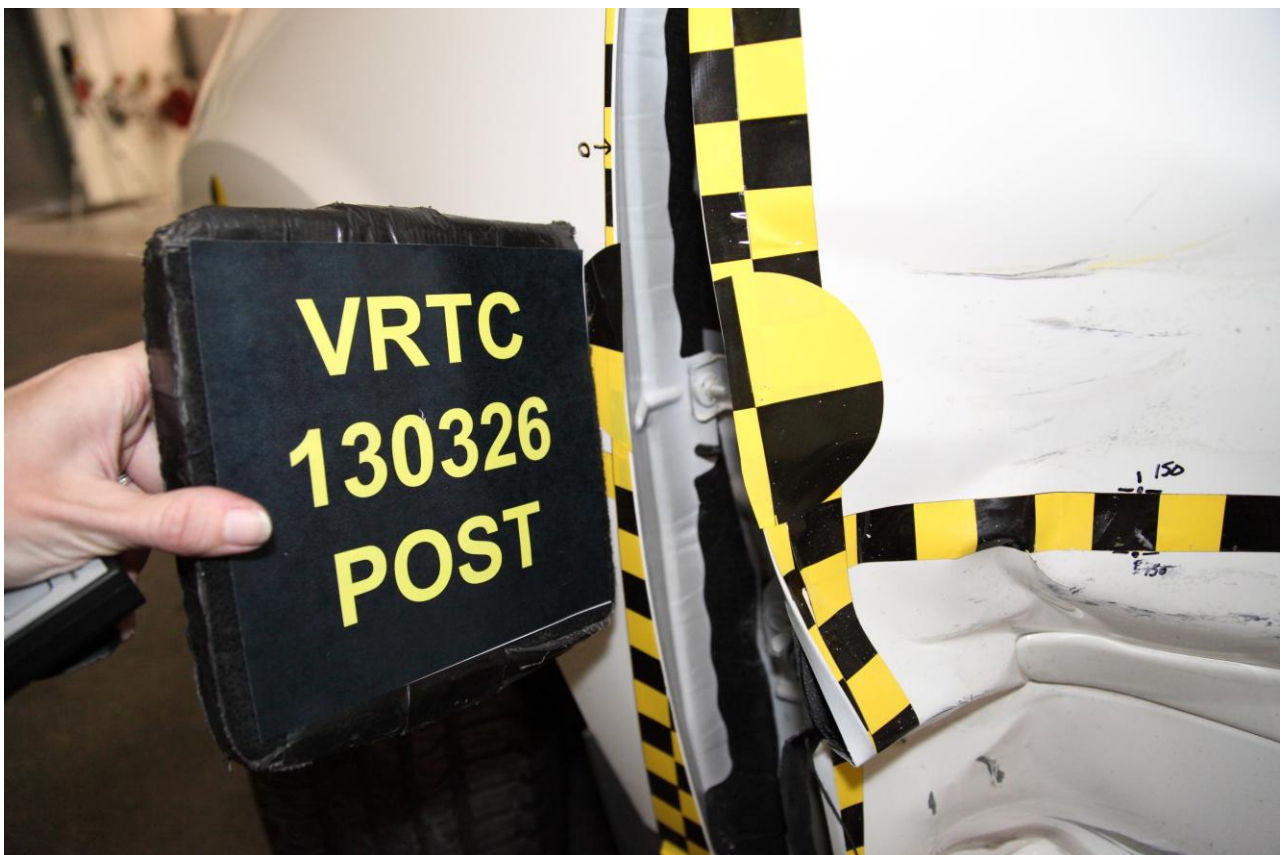
Figure A-16 Post-Test Primary Impact Point View
