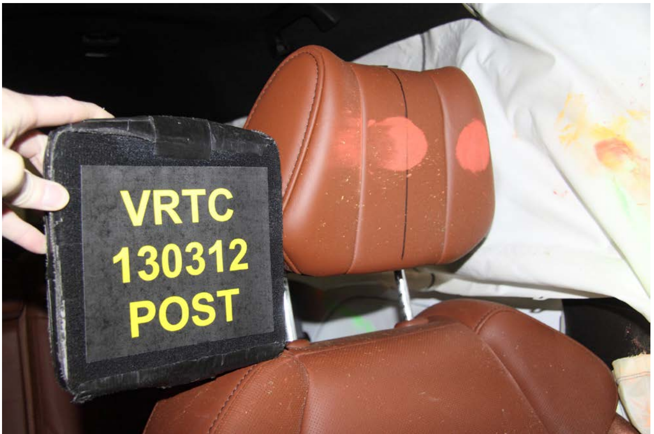
Figure A-27 Post-Test Driver Dummy Contact – View 1
