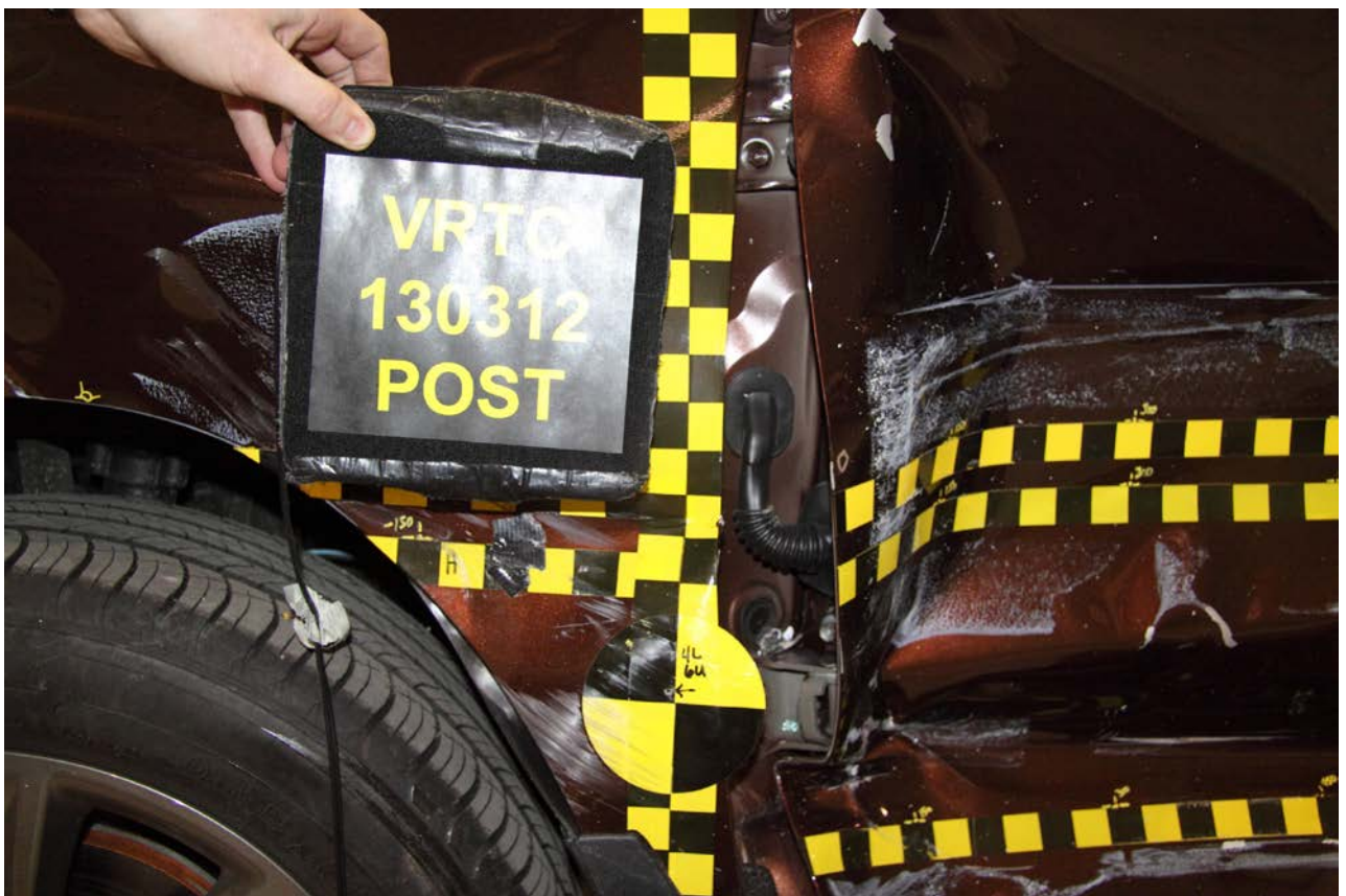
Figure A-16 Post-Test Primary Impact Point View
