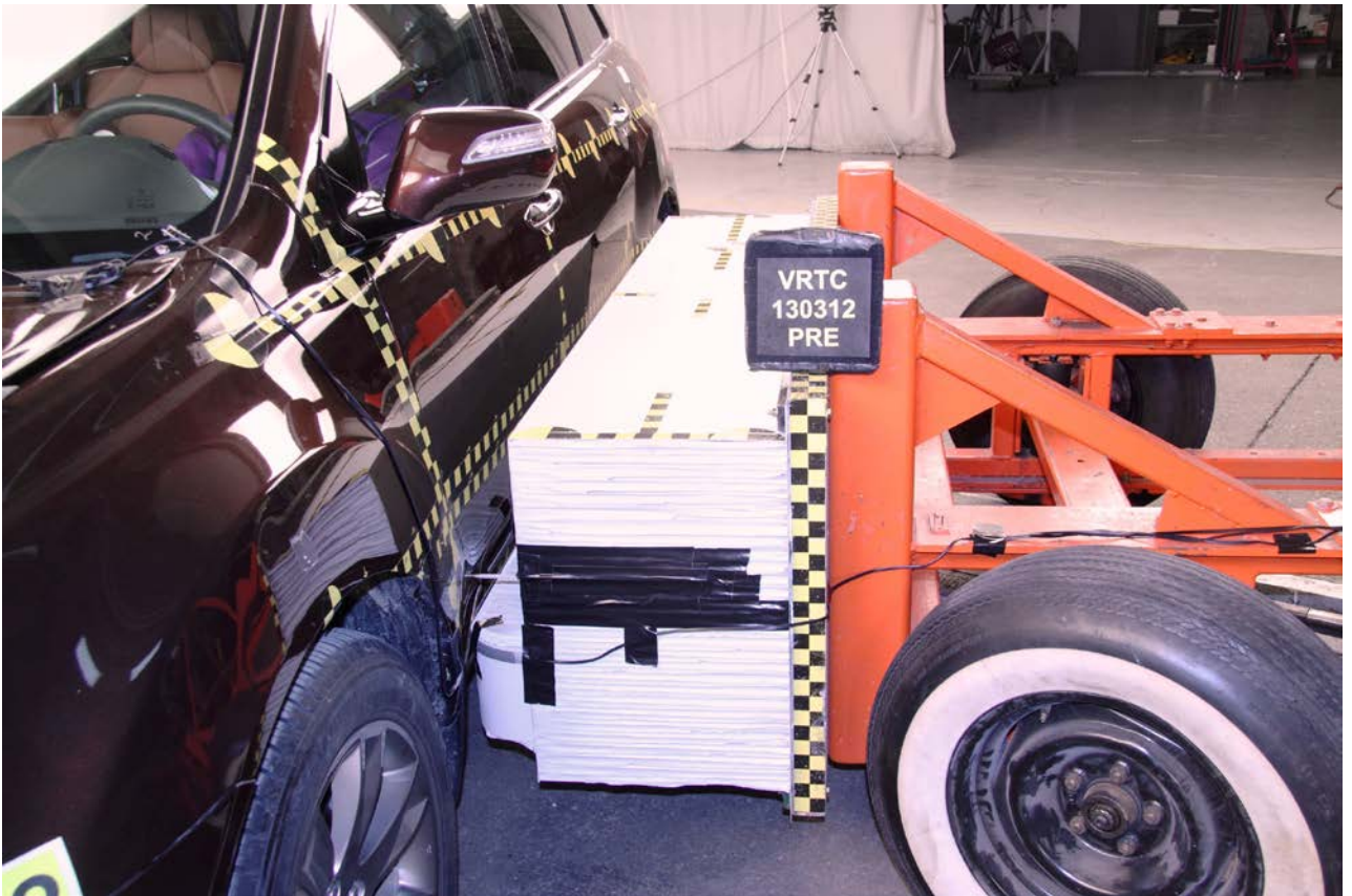
Figure A-47 Pre-Test MDB Face Left Side View
