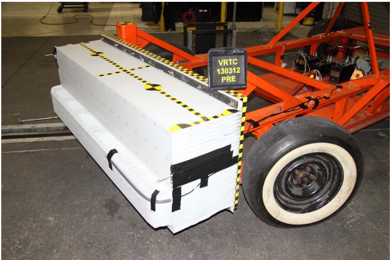
Figure A-43 Pre-Test MDB Face Left Front View
