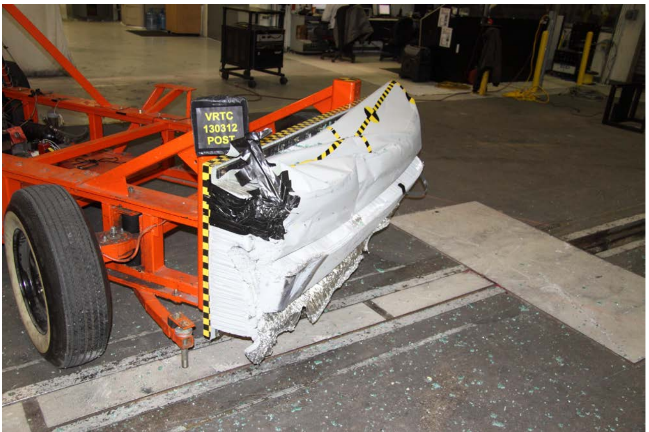
Figure A-46 Post-Test MDB Face Right Front View
