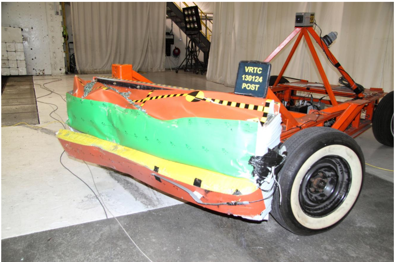
Figure A-44 Post-Test MDB Face Left Front View
