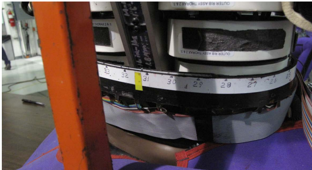
Figure 1. Rear of WorldSID 5th female dummy showing chest band location
