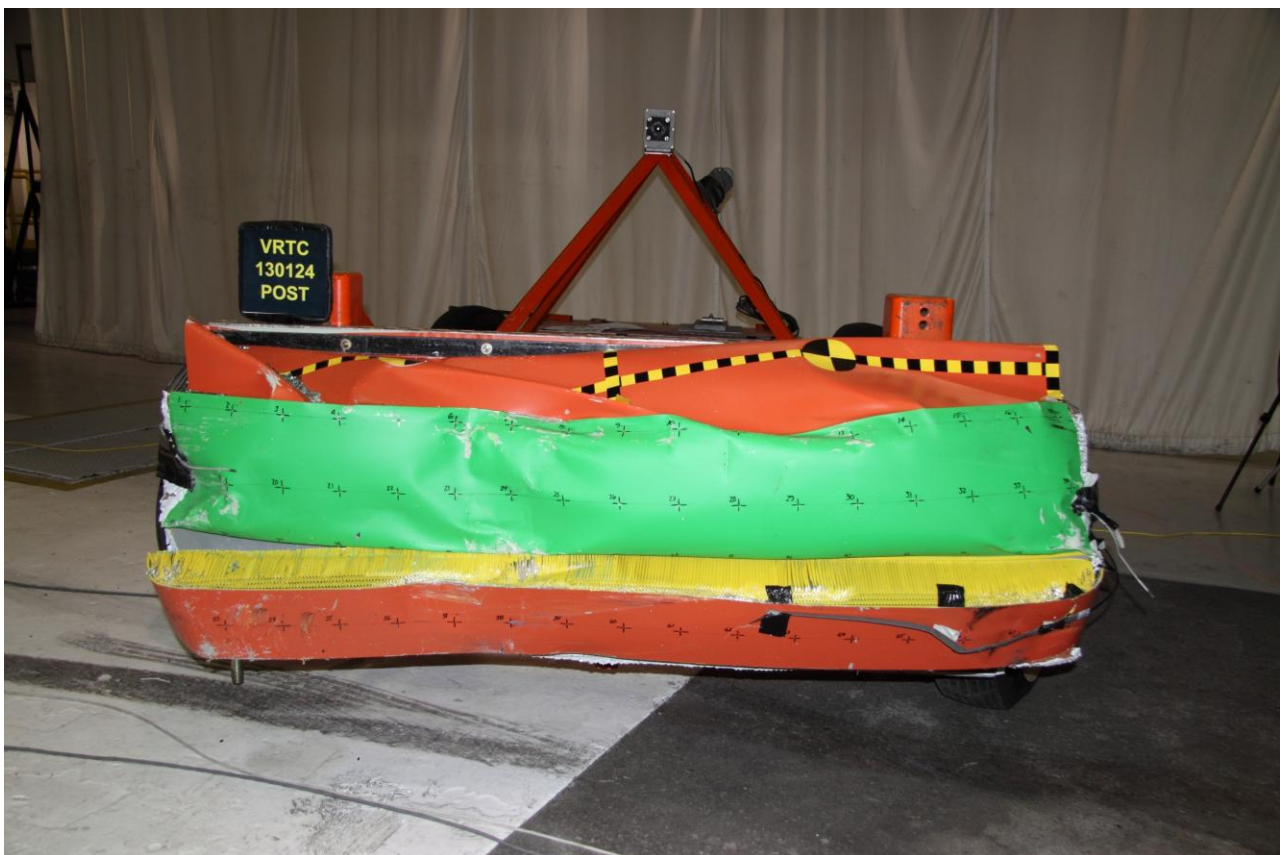
Figure A-40 Post-Test MDB Face Front View
