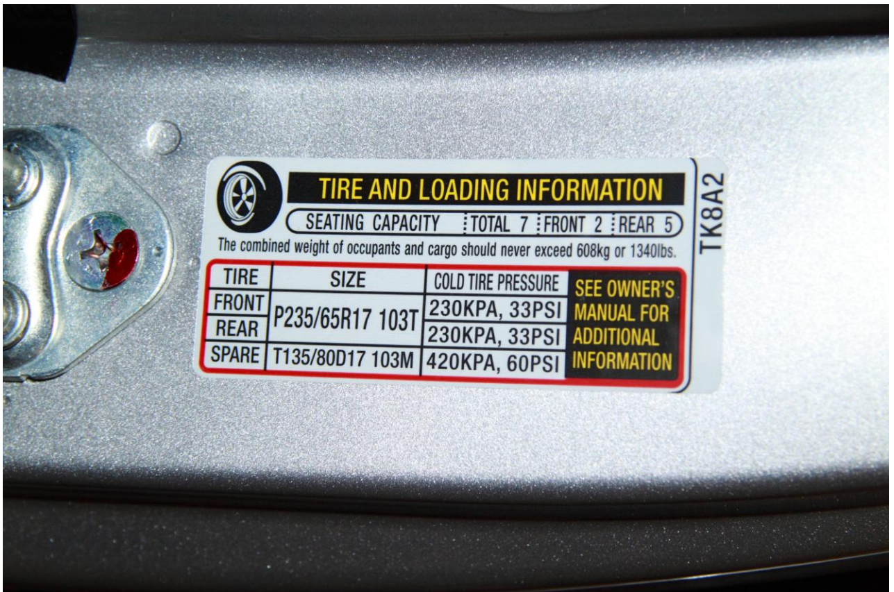
Figure A-50 Tire Pressure Label
