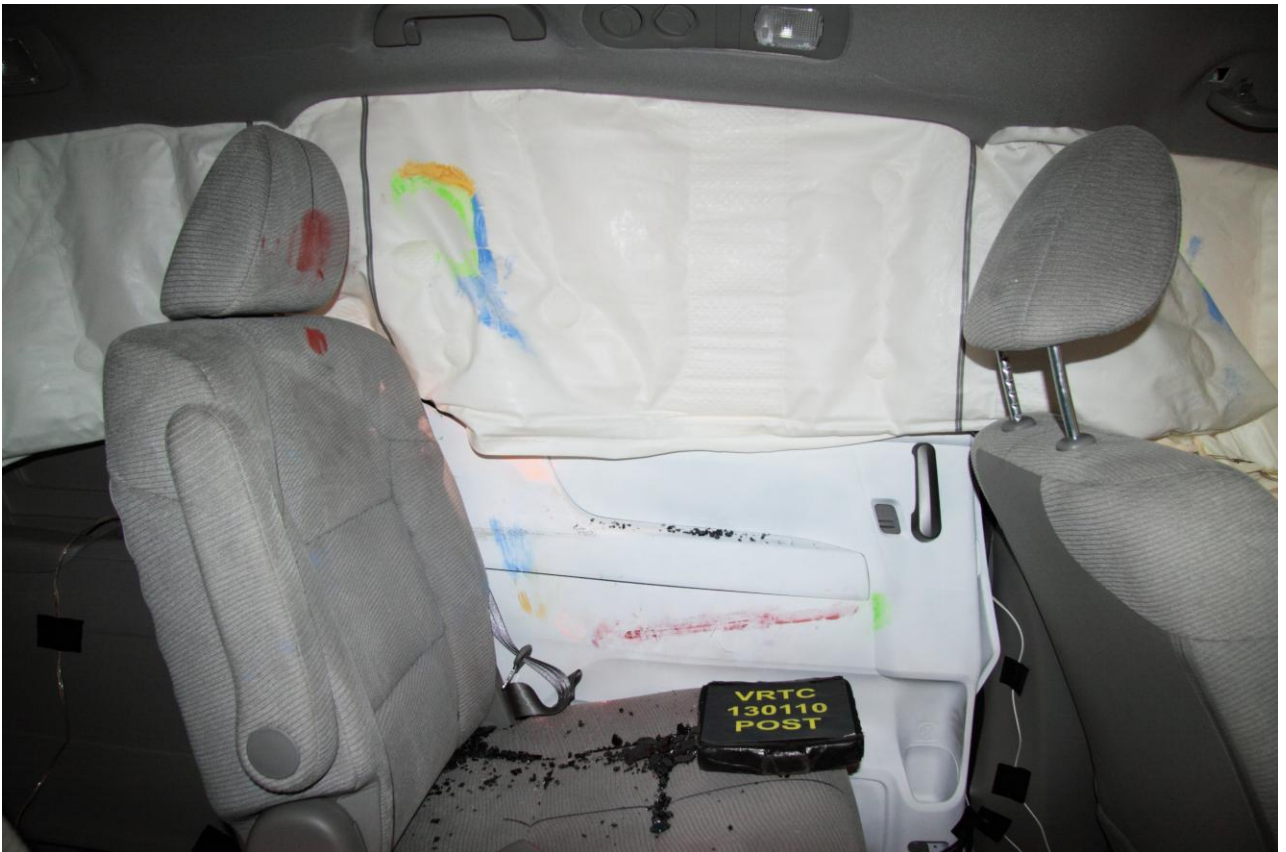
Figure A-36 Post-Test Rear Passenger Door Panel View
