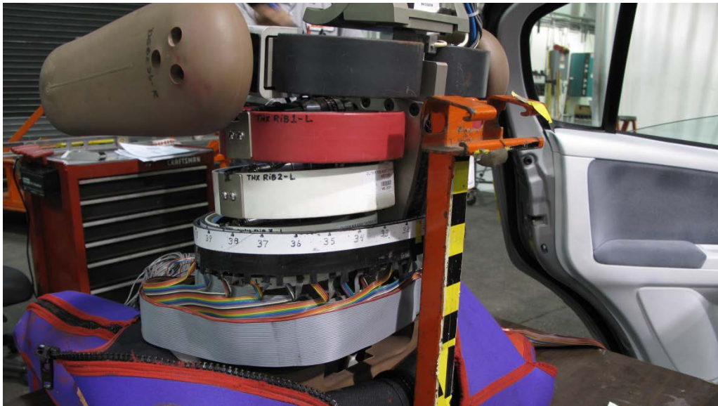
Figure 1. Rear of WorldSID 5th female dummy showing chest band location
