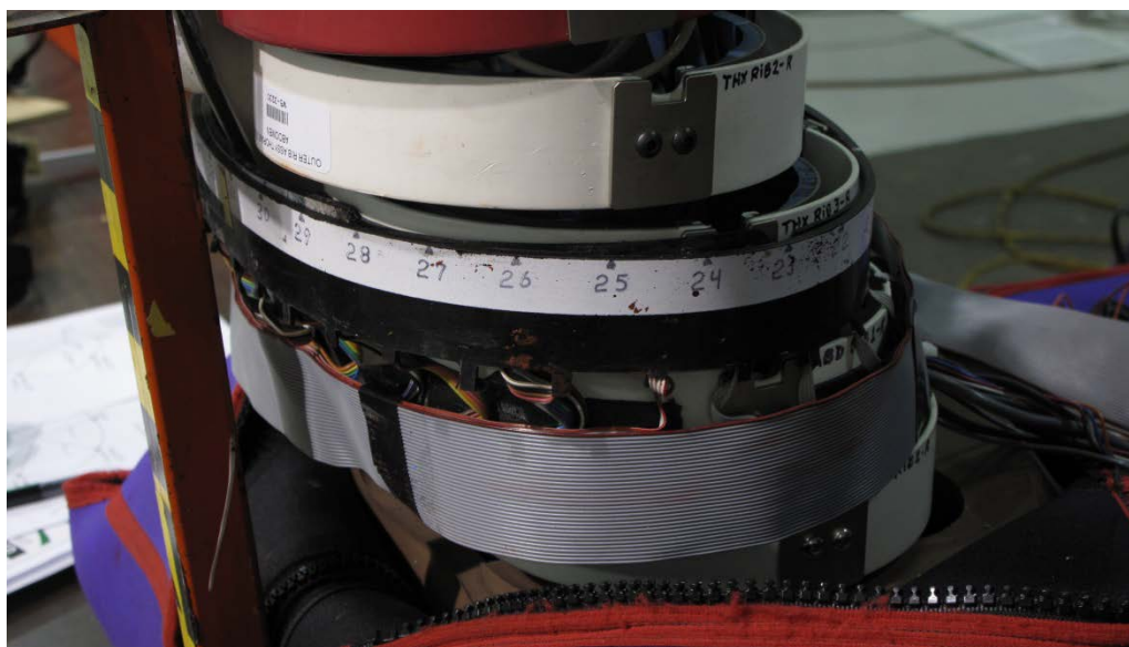
Figure 4. Right side of WorldSID 5th female dummy showing chest band location
