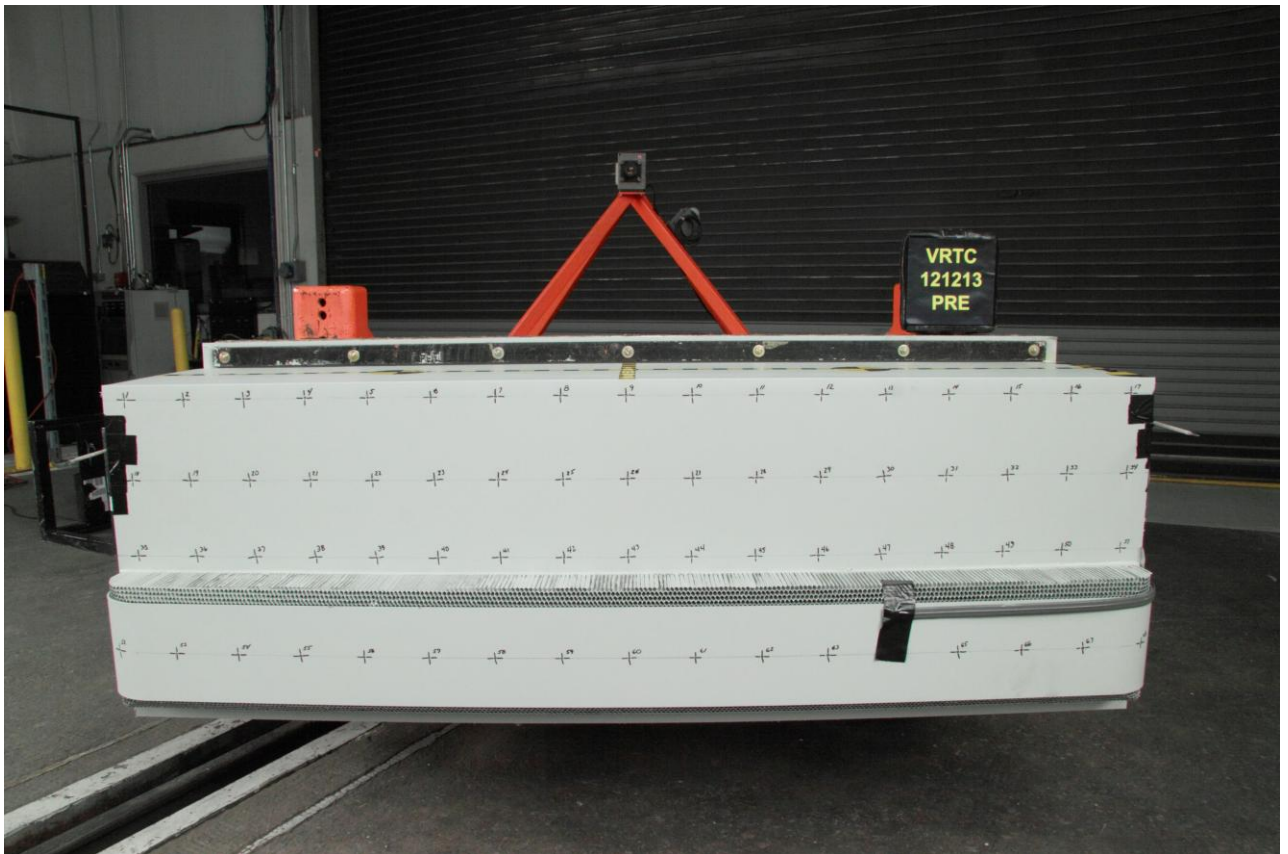
Figure A-49 Pre-Test MDB Face Front View
