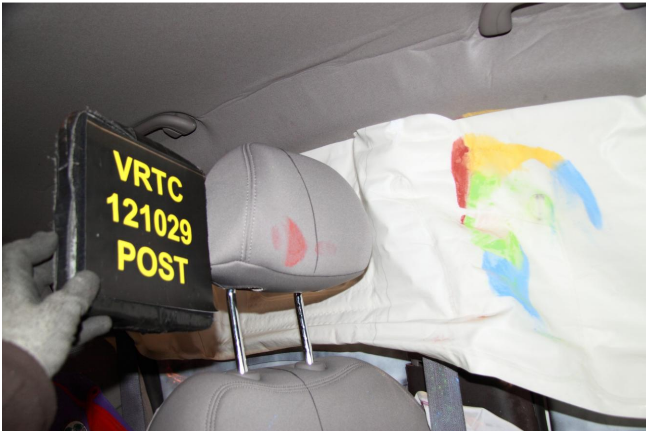
Figure A-31 Post-Test Driver Dummy Contact - View 1
