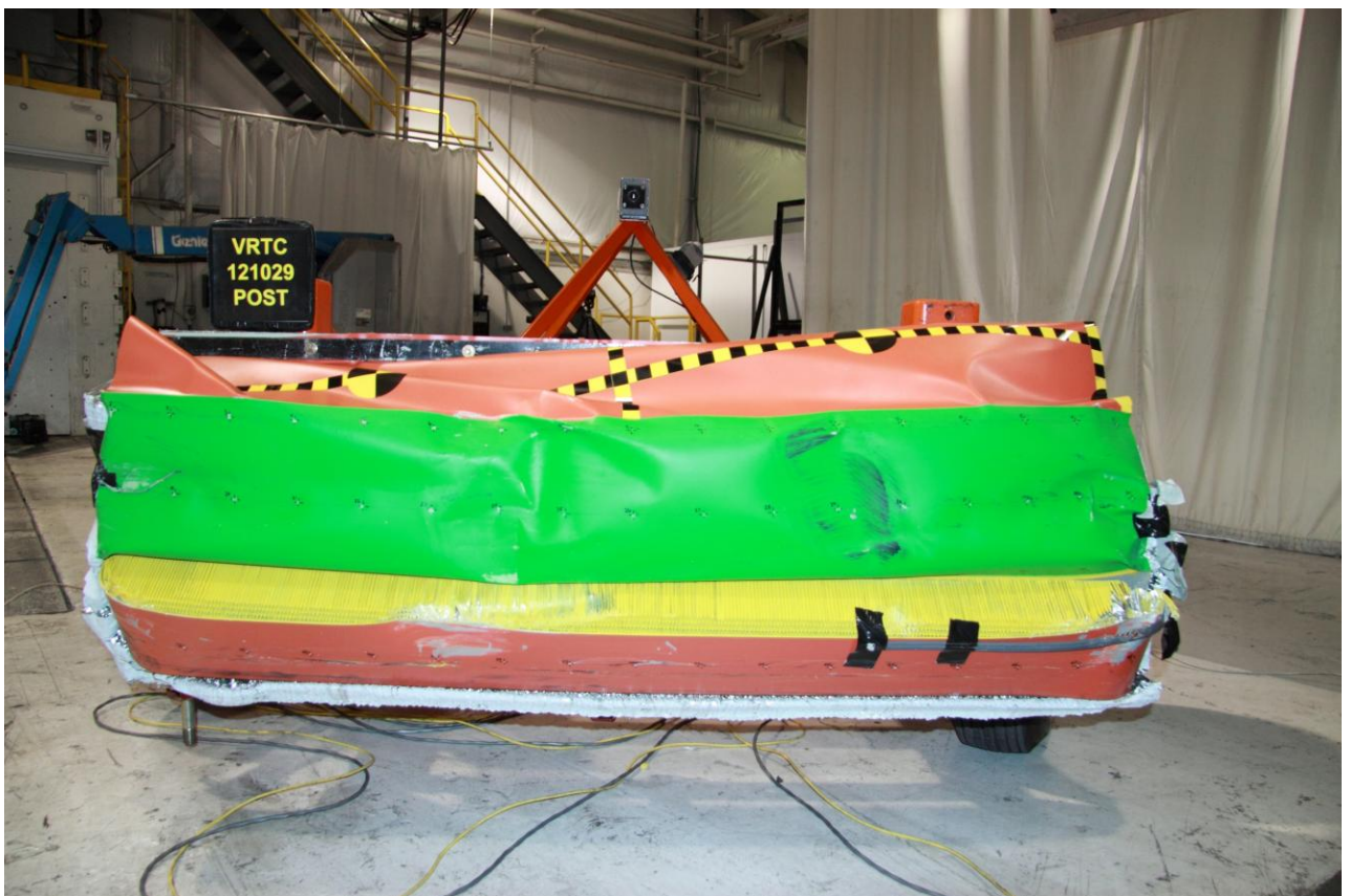
Figure A-44 Post-Test MDB Face Front View
