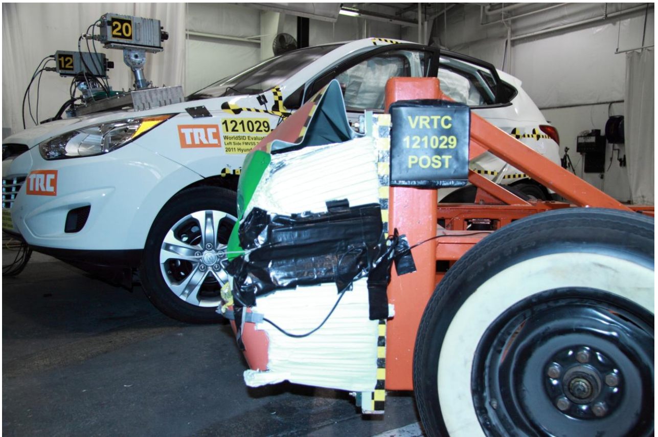
Figure A-51 Post-Test MDB Face Left Side View
