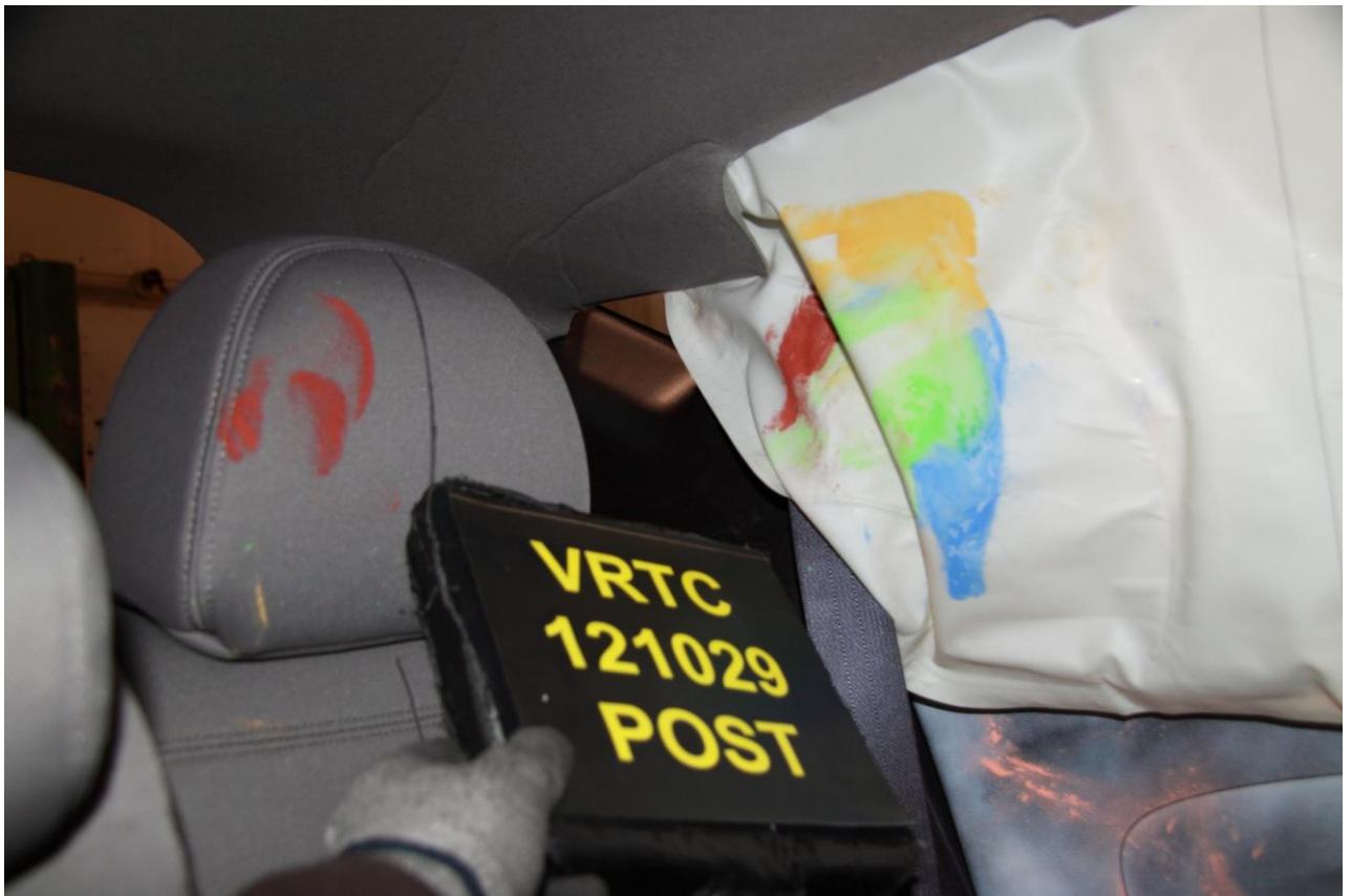
Figure A-41 Post-Test Rear Passenger Dummy Contact – View 1
