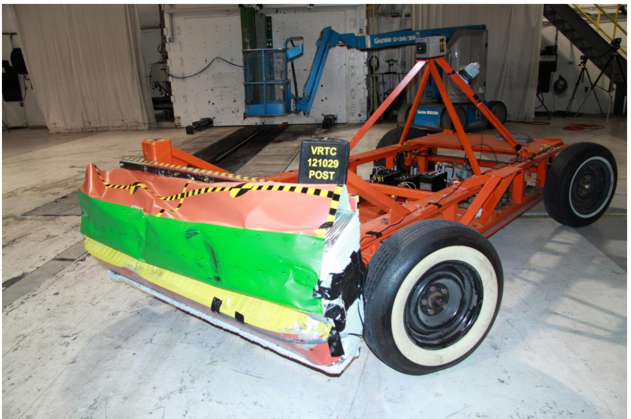
Figure A-48 Post-Test MDB Face Left Front View
