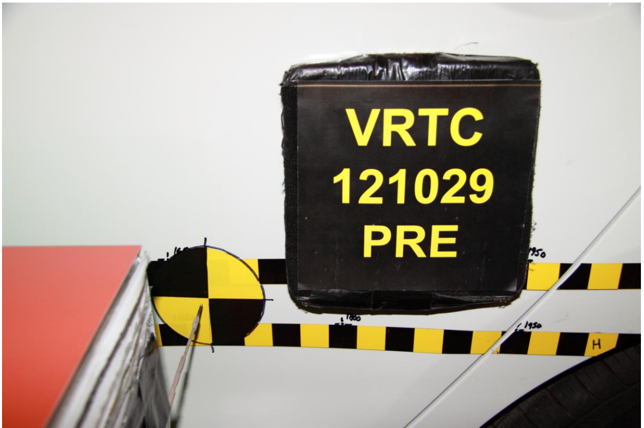
Figure A-21 Pre-Test Secondary Impact Point View
