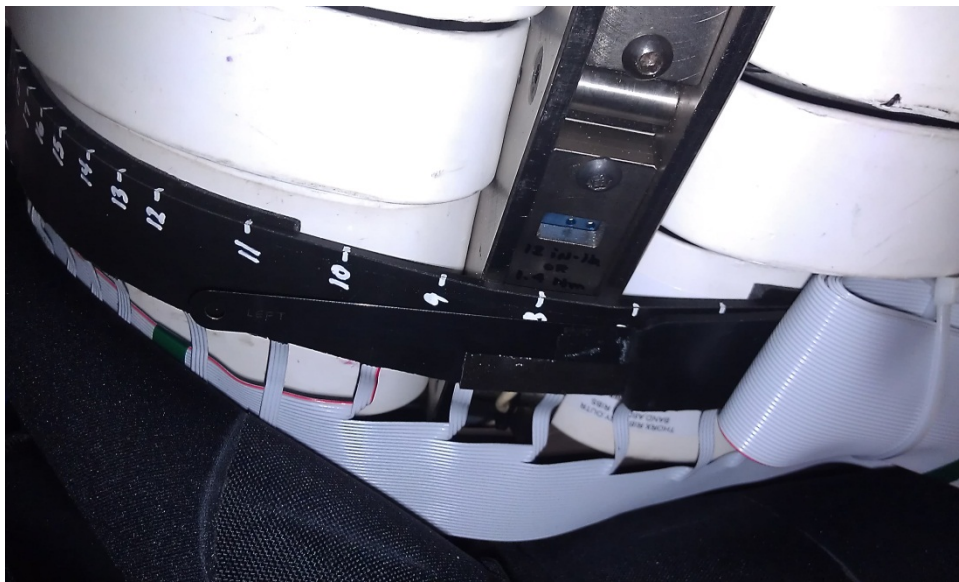
Figure 1. Rear of WorldSID 50th male dummy showing chest band location
