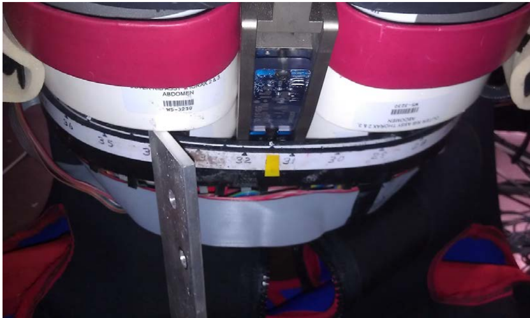
Figure 5. Rear of WorldSID 5th female dummy showing chest band location
