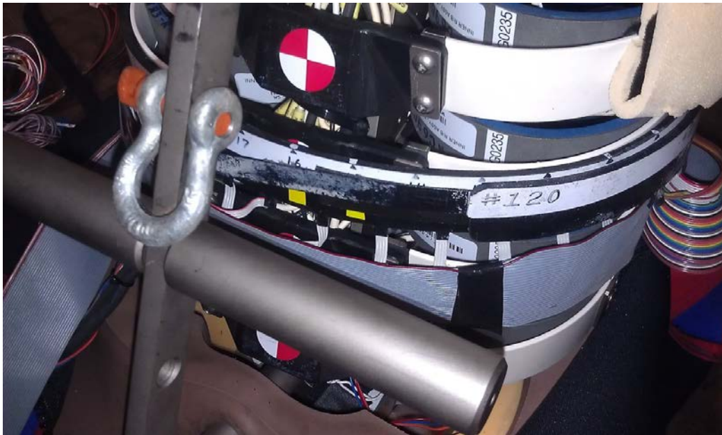
Figure 7. Front of WorldSID 5th female dummy showing chest band location
