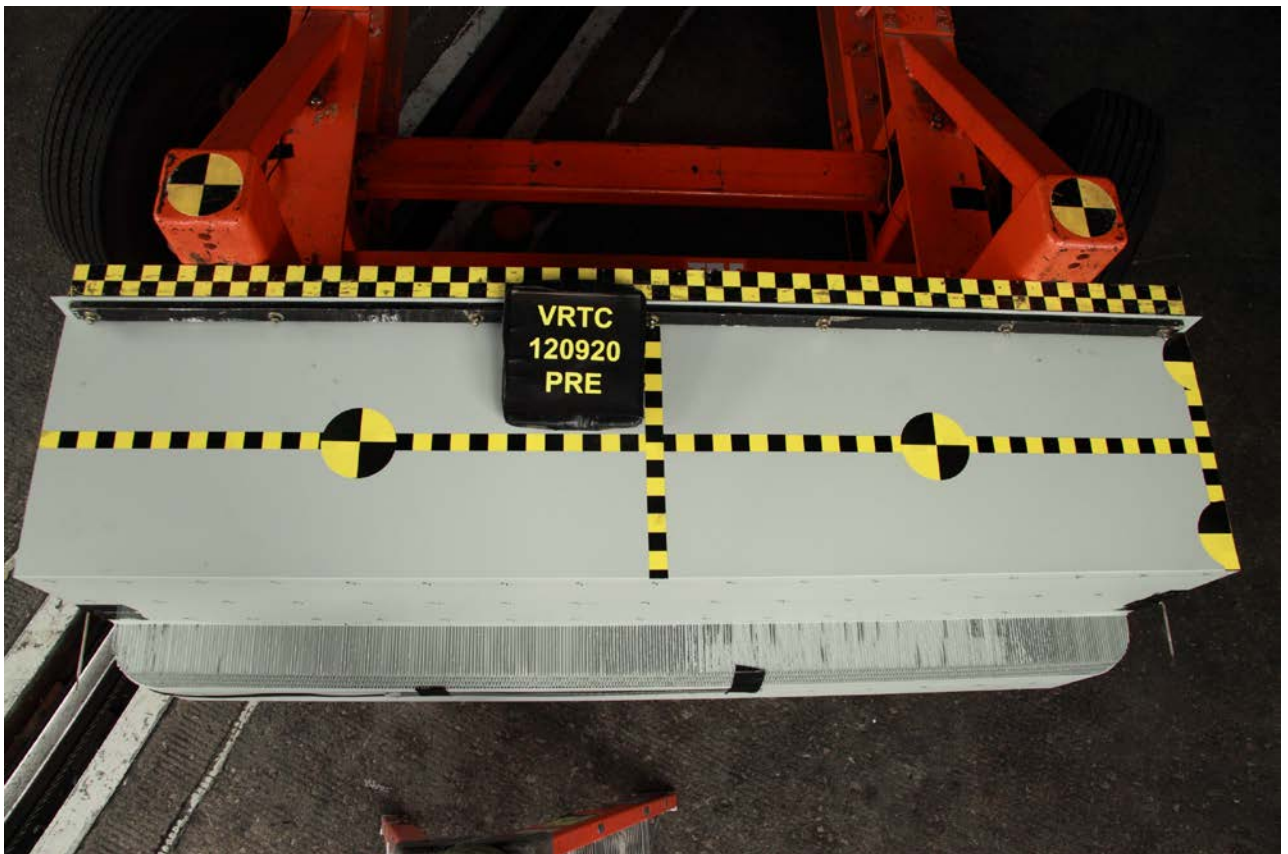
Figure A-45 Pre-Test MDB Face Top View
