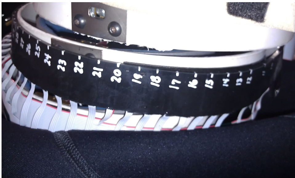
Figure 2. Left side of WorldSID 50 th male dummy showing chest band location
