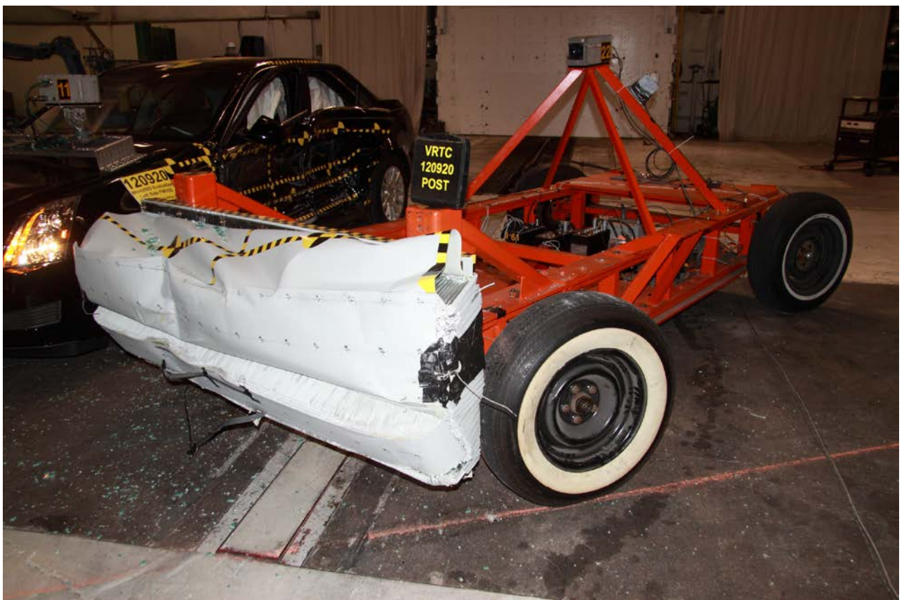
Figure A-50 Post-Test MDB Face Left Front View
