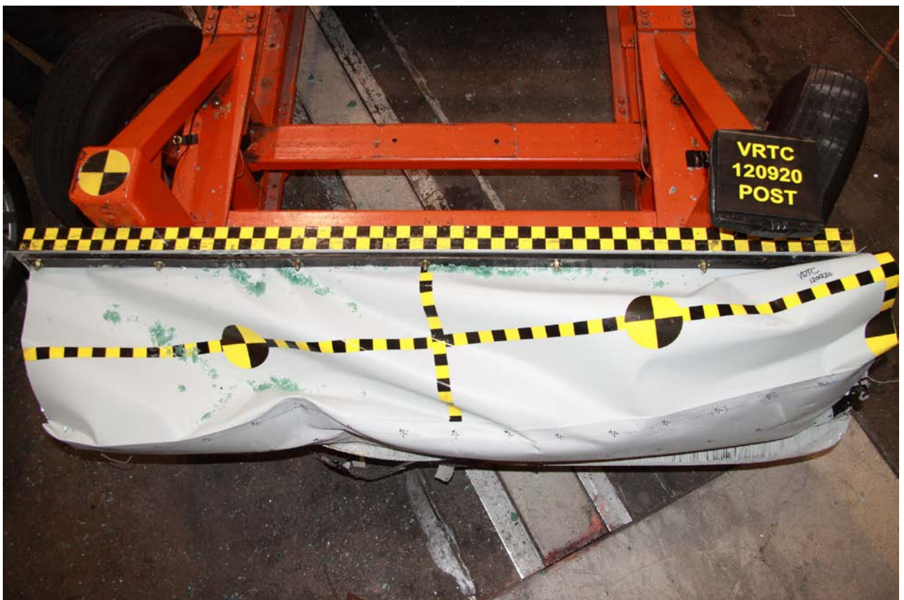
Figure A-46 Post-Test MDB Face Top View
