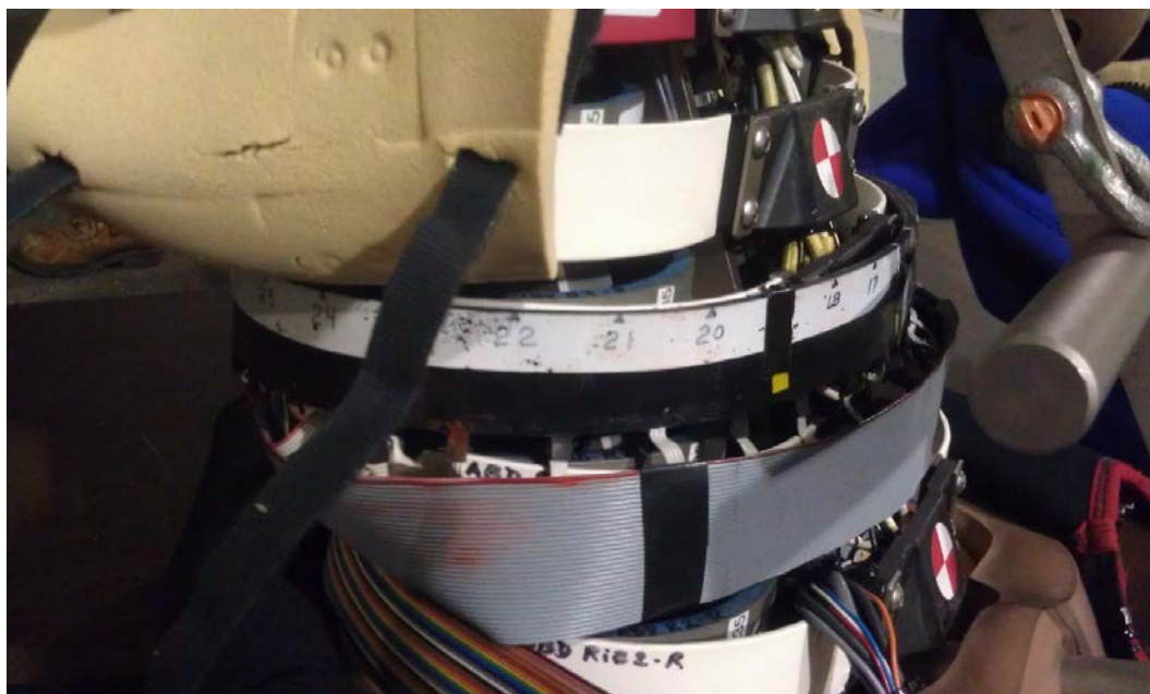
Figure 8. Right side of WorldSID 5th female dummy showing chest band location
