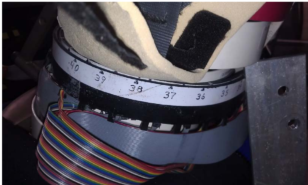
Figure 6. Left side of WorldSID 5th female dummy showing chest band location
