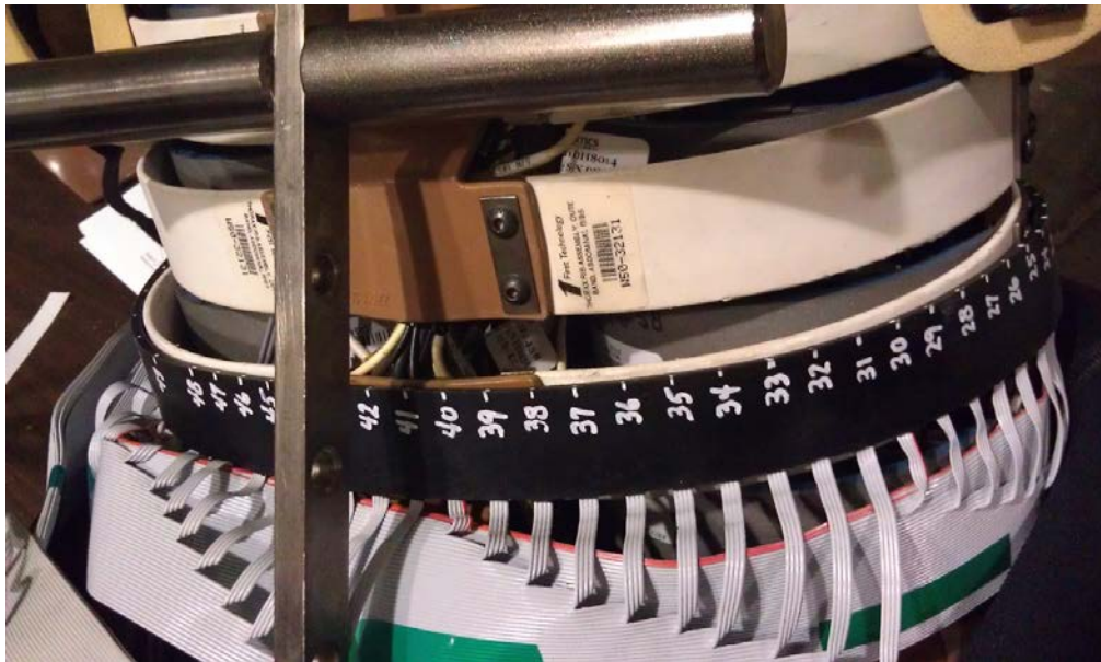
Figure 3. Front of WorldSID 50th male dummy showing chest band location
