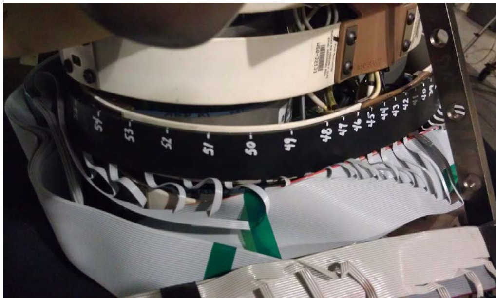
Figure 4. Right side of WorldSID 50th dummy showing chest band location
