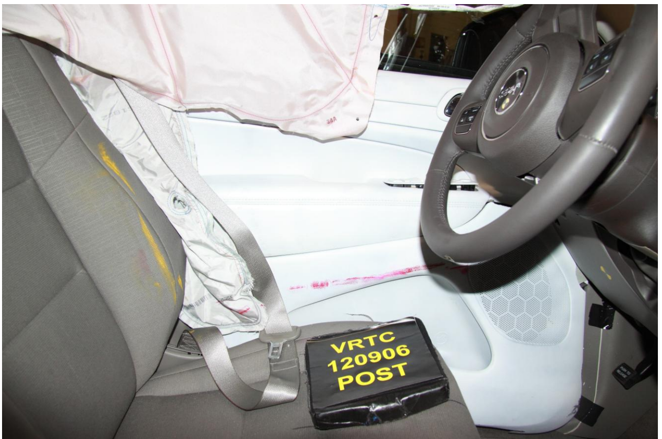
Figure A-26 Post-Test Driver Door Panel View
