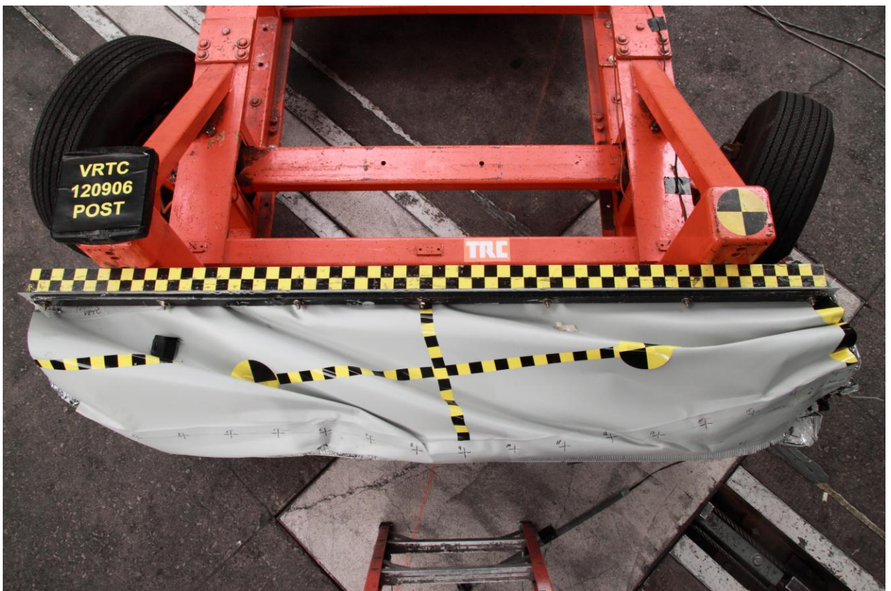
Figure A-42 Post-Test MDB Face Top View
