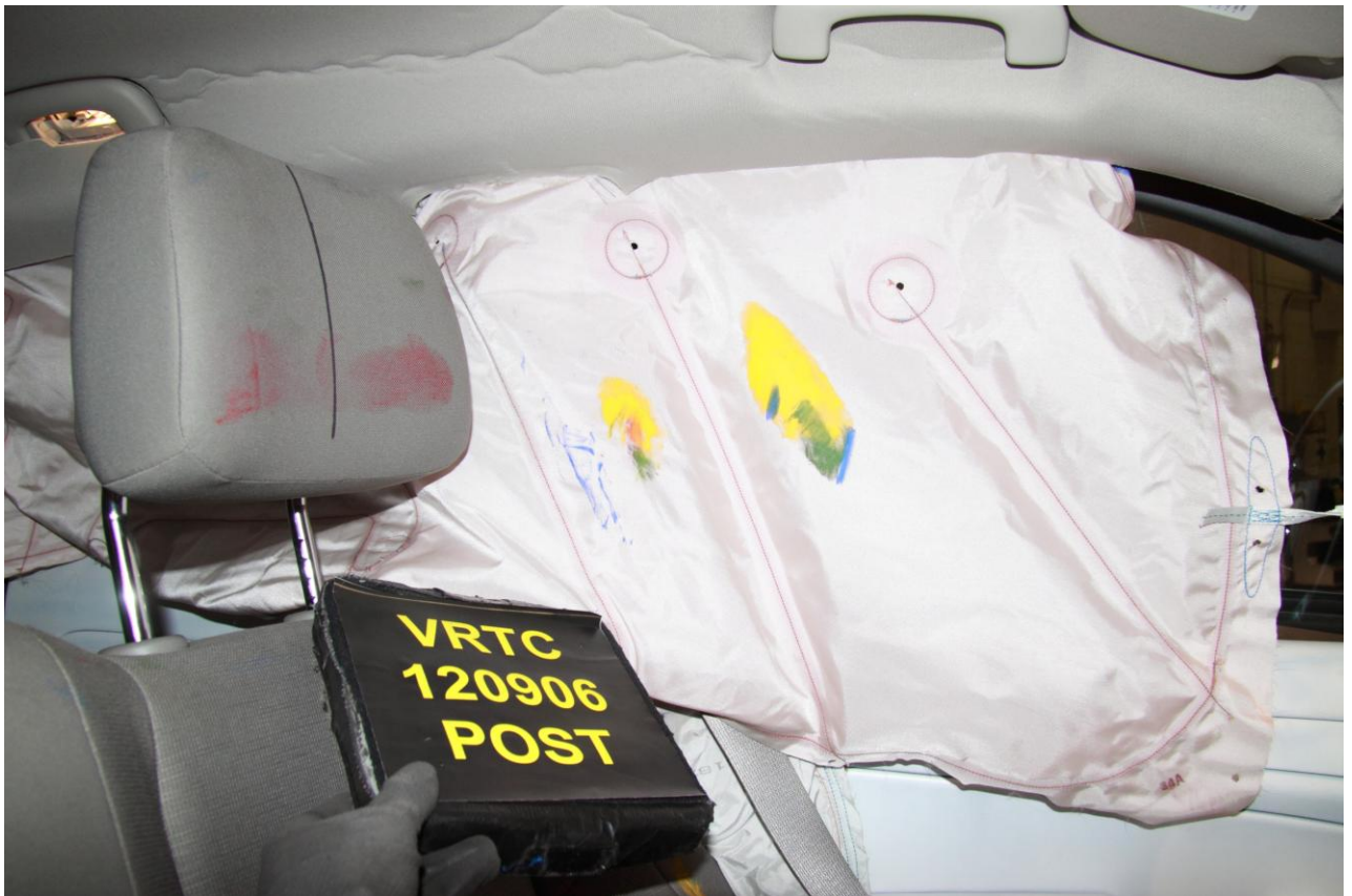
Figure A-27 Post-Test Driver Dummy Contact - View 1
