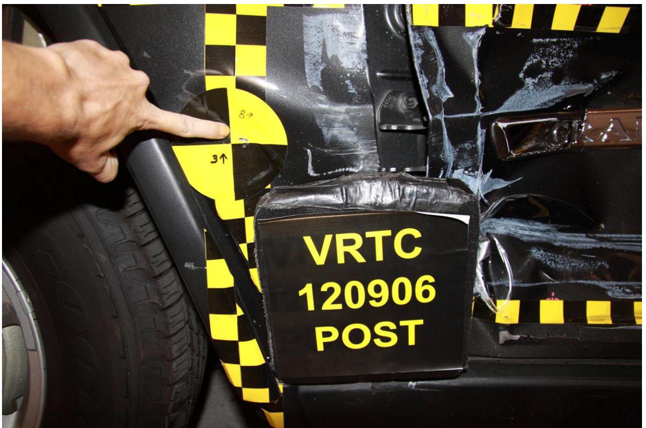
Figure A-16 Post-Test Primary Impact Point View
