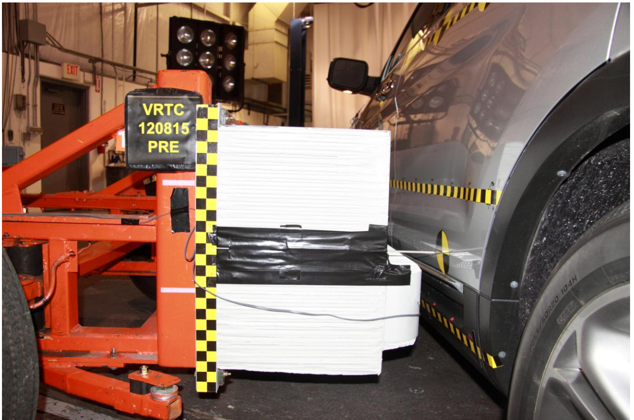
Figure A-47 Pre-Test MDB Face Right Side View
