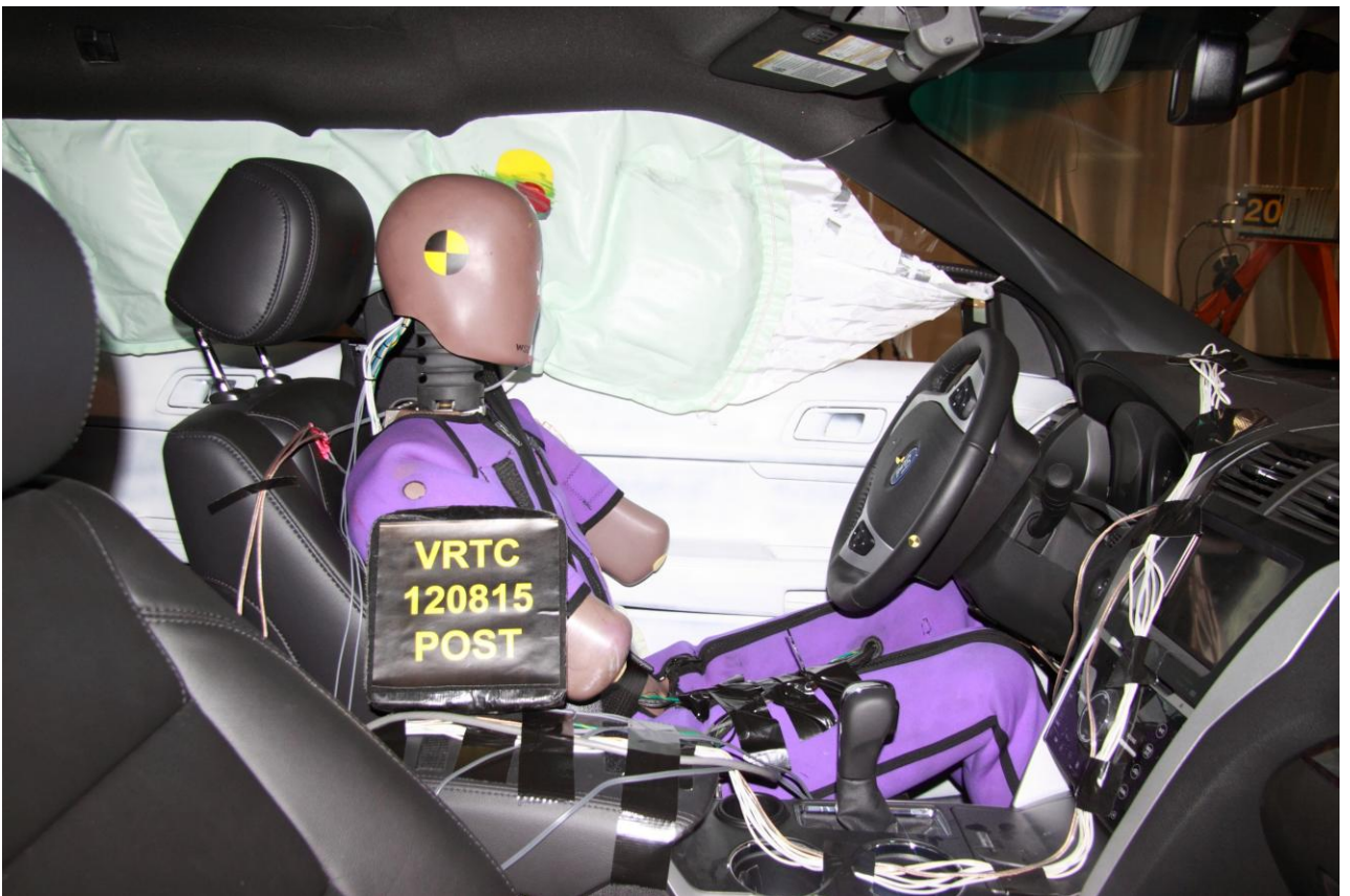
Figure A-26 Post-Test Driver Dummy - View 3
