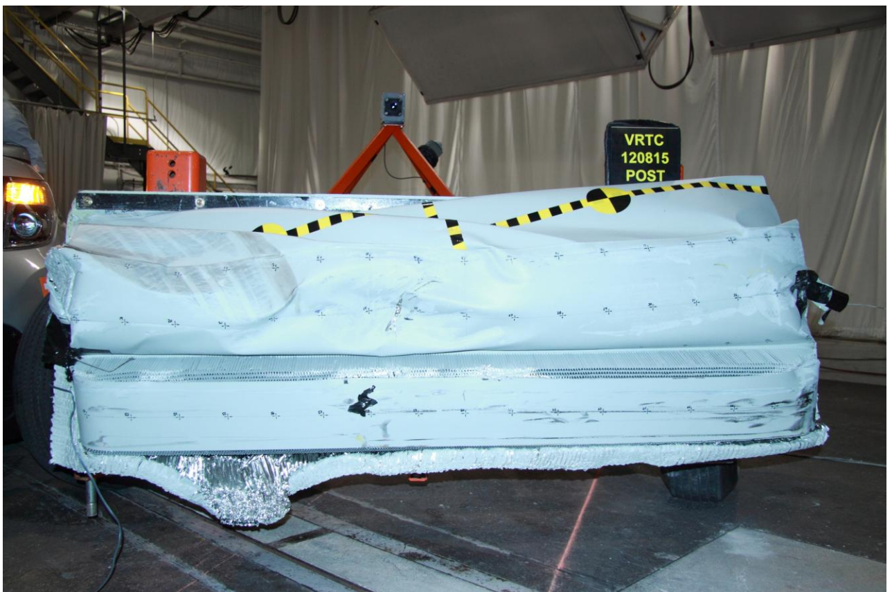
Figure A-42 Post-Test MDB Face Front View
