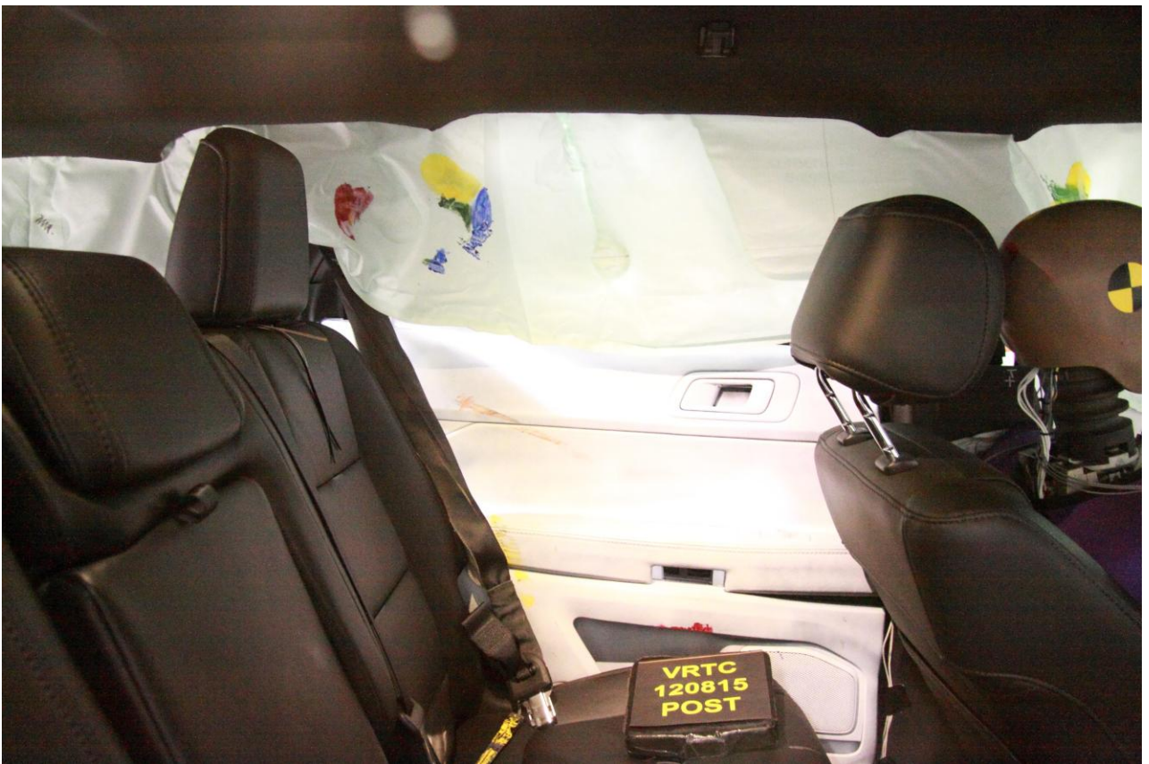
Figure A-37 Post-Test Rear Passenger Door Panel View
