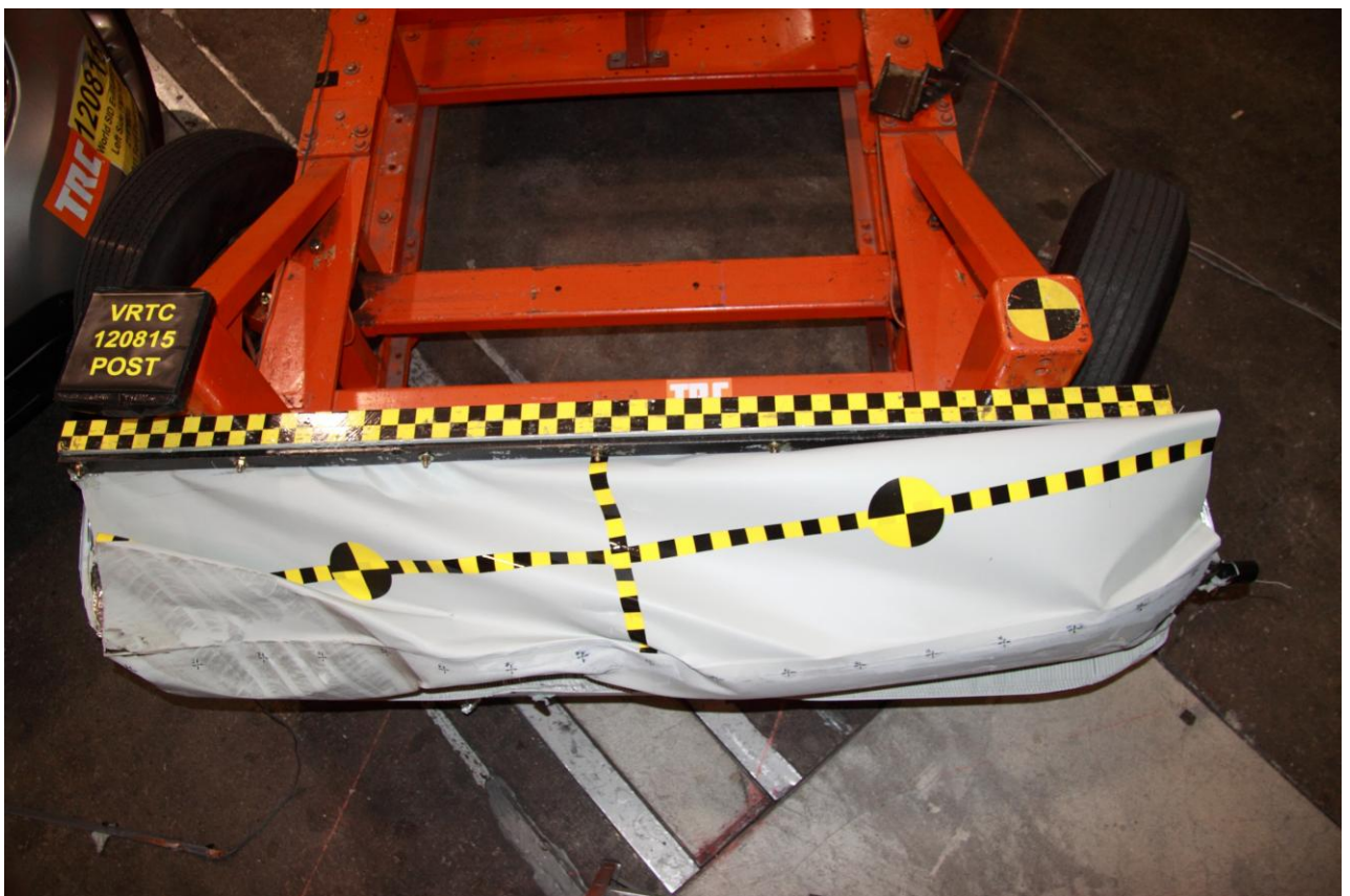
Figure A-44 Post-Test MDB Face Top View
