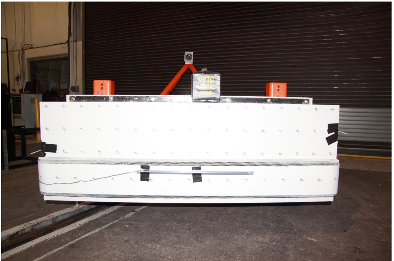
Figure A-41 Pre-Test MDB Face Front View
