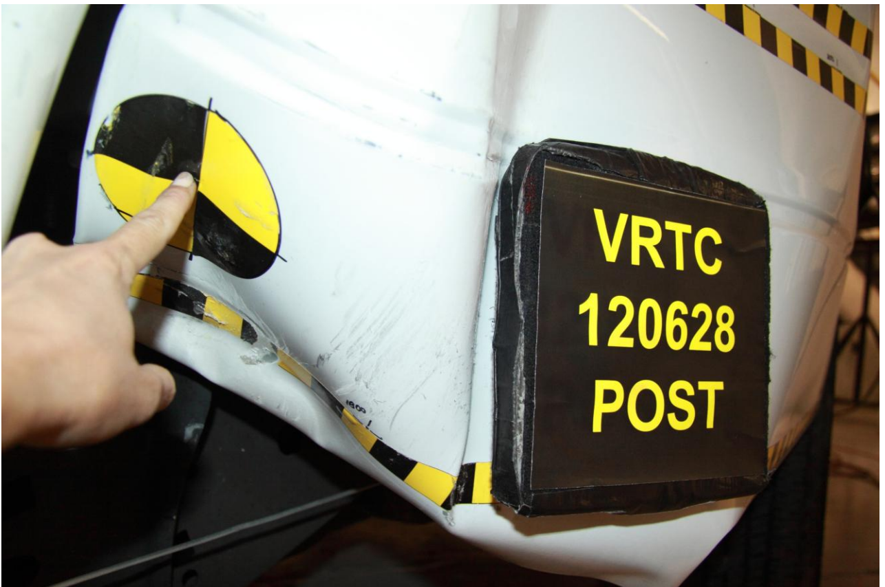
Figure A-20 Post-Test Secondary Impact Point View
