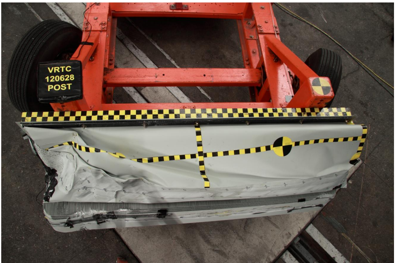
Figure A-43 Post-Test MDB Face Top View
