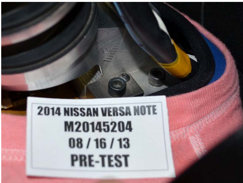
FIGURE 30. Pre-Test Left Side View of Dummy's Neck Showing Position of Adjustable Neck Bracket
