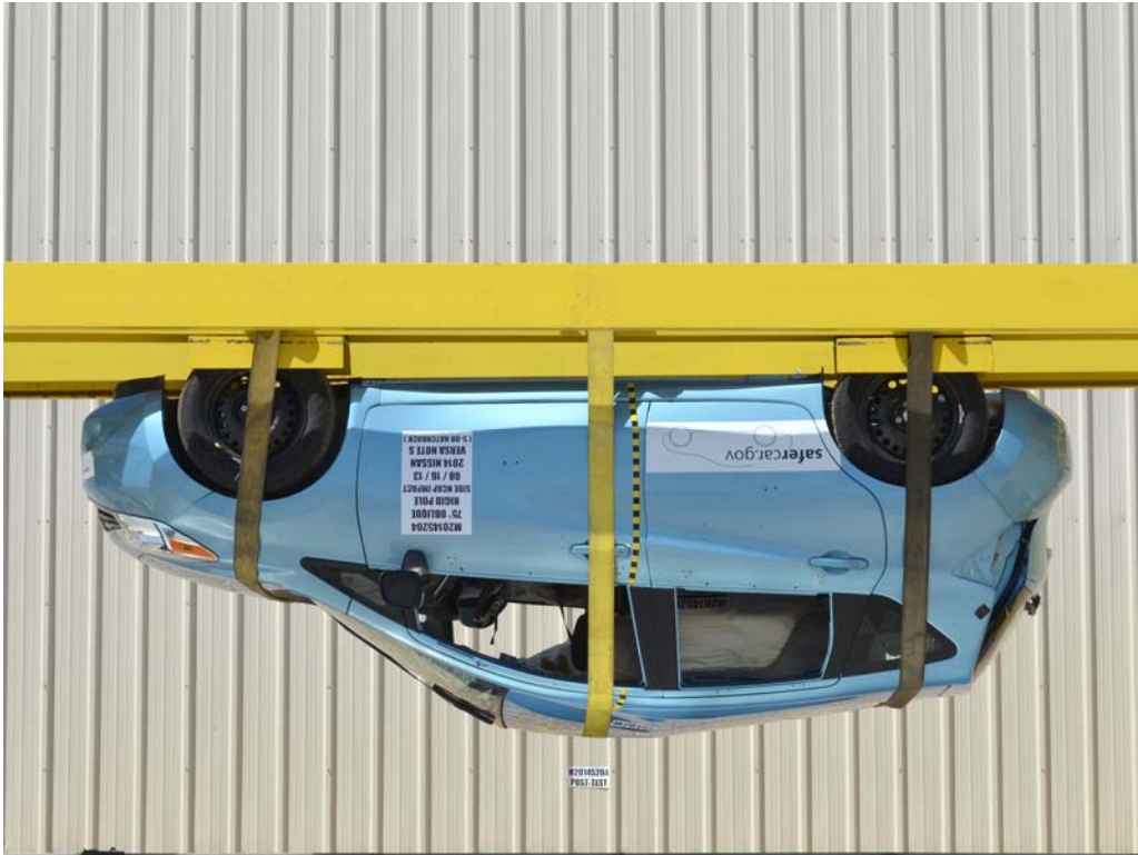
FIGURE 65. FMVSS No. 301 Static Rollover 180 Degrees
