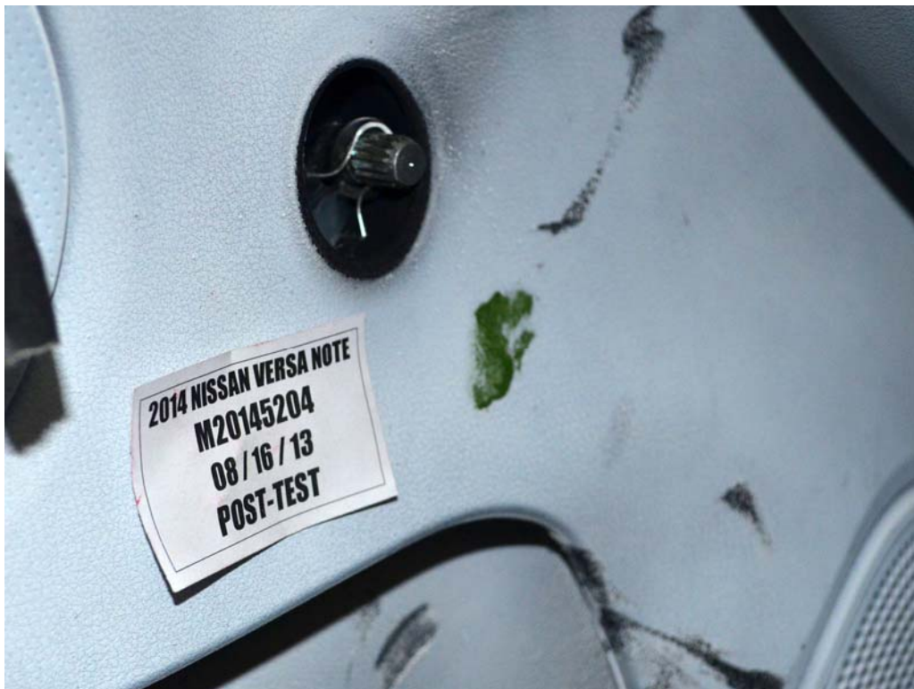
FIGURE 52. Post-Test Dummy Close-Up Knee Contact with Vehicle Interior View
