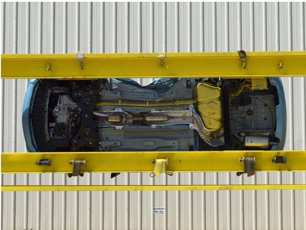
FIGURE 66. FMVSS No. 301 Static Rollover 270 Degrees
