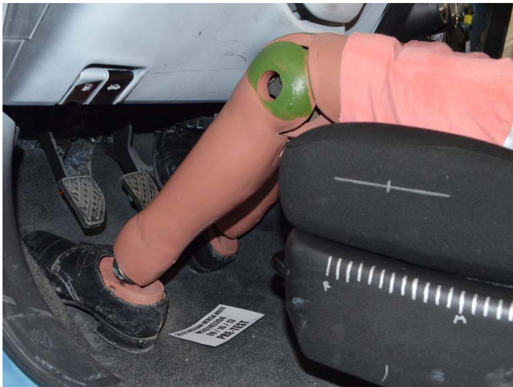
FIGURE 32. Pre-Test Placement of Dummy's Feet
