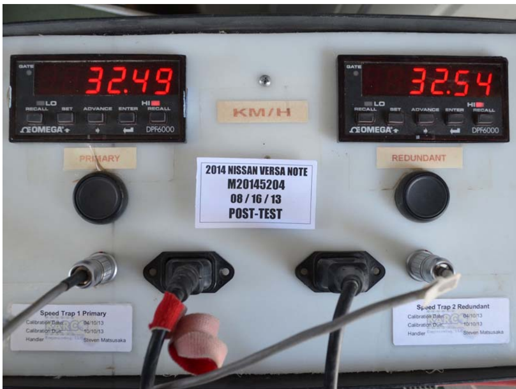
FIGURE 62. Post-Test Primary and Redundant Speed Trap Read-Out
