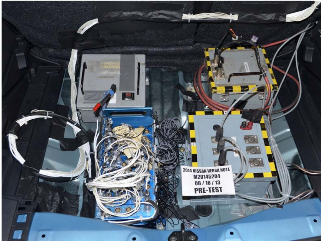
FIGURE 61. Pre-Test Ballast View
