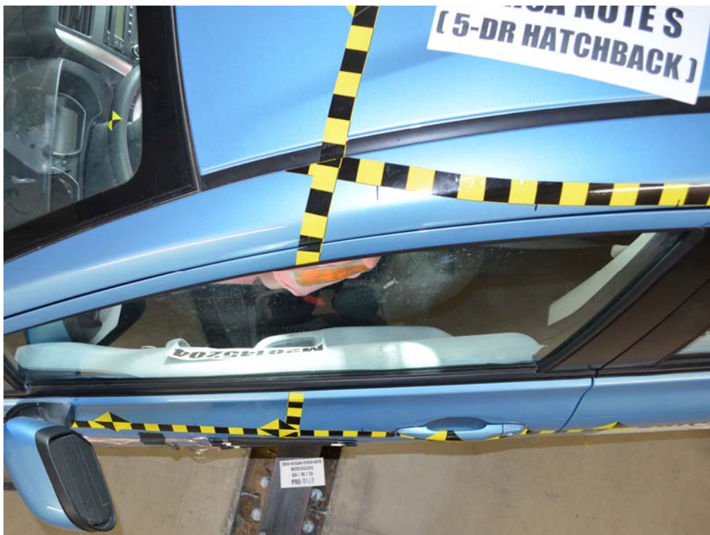
FIGURE 40. Pre-Test Dummy and Door Clearance View
