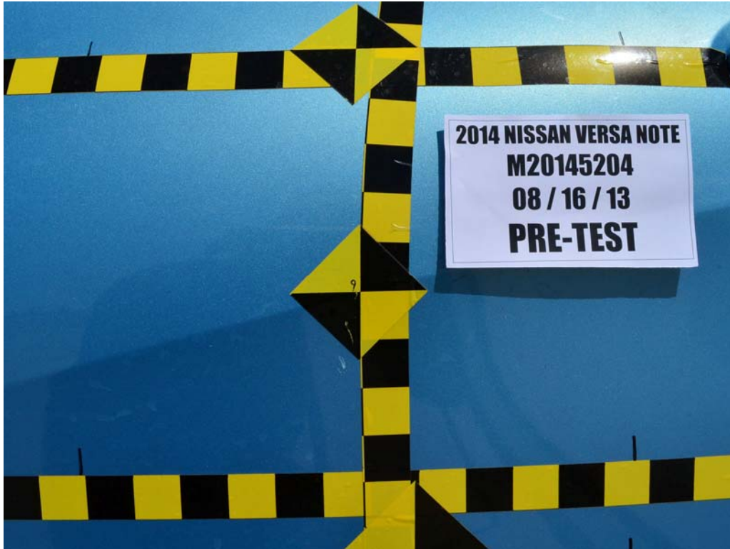
FIGURE 19. Pre-Test Close-Up View of Impact Point Target
