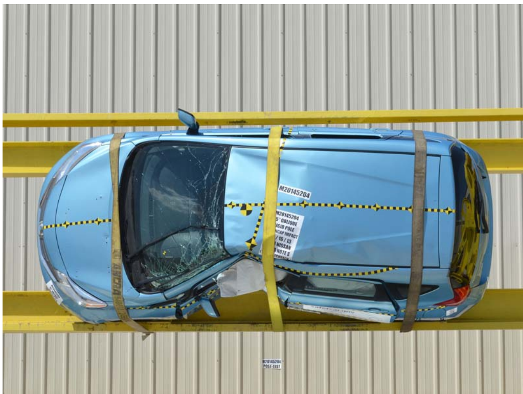
FIGURE 64. FMVSS No. 301 Static Rollover 90 Degrees
