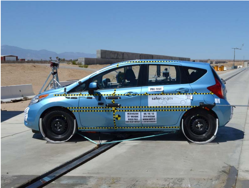
FIGURE 7. Pre-Test Left Side View of Test Vehicle
