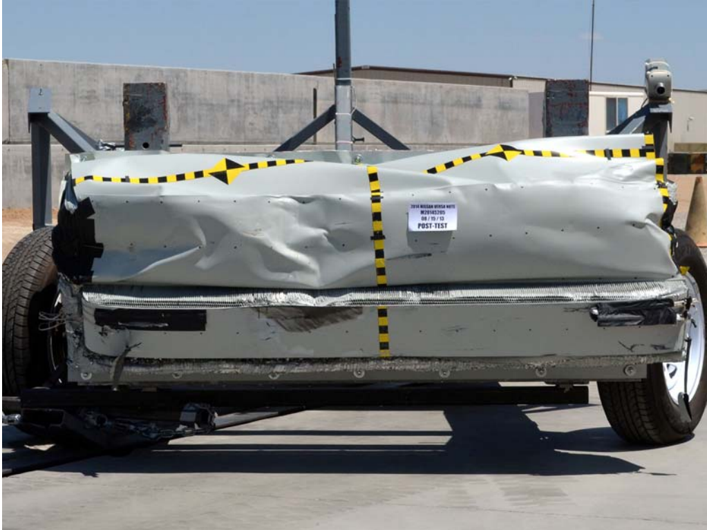
FIGURE 85. Post-Test Front View of MDB Impactor Face
