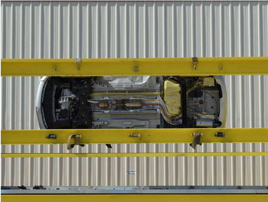
FIGURE 99. FMVSS No. 301 Static Rollover 270 Degrees
