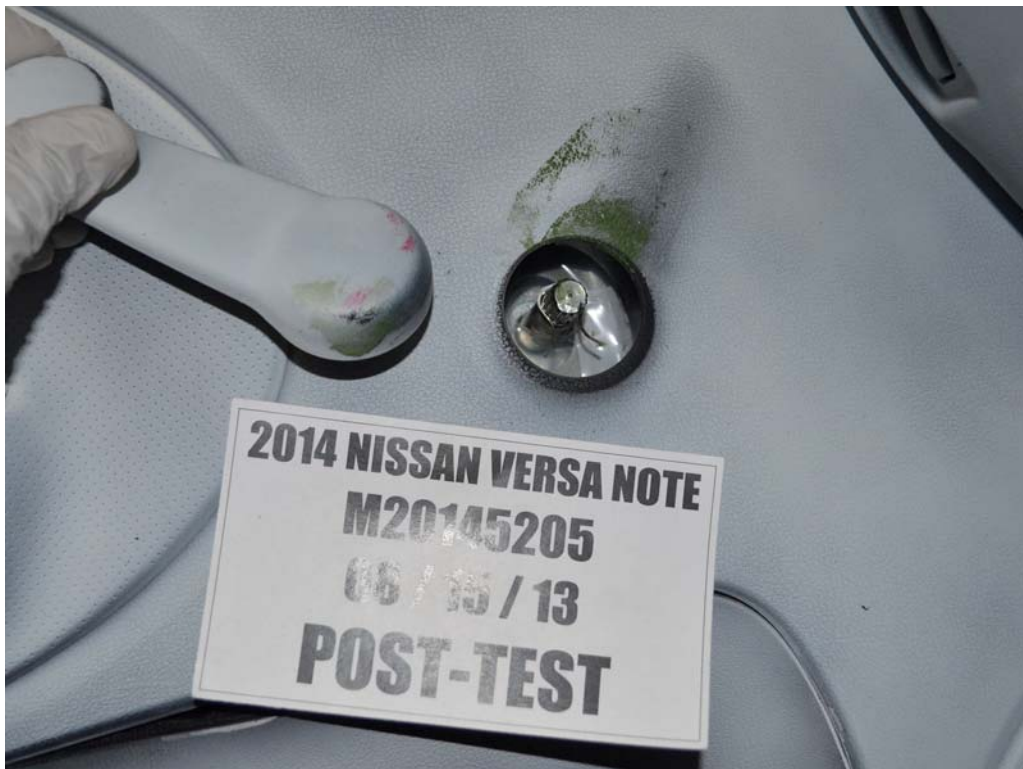
FIGURE 54. Post-Test Driver Dummy Close-Up Knee Contact View
