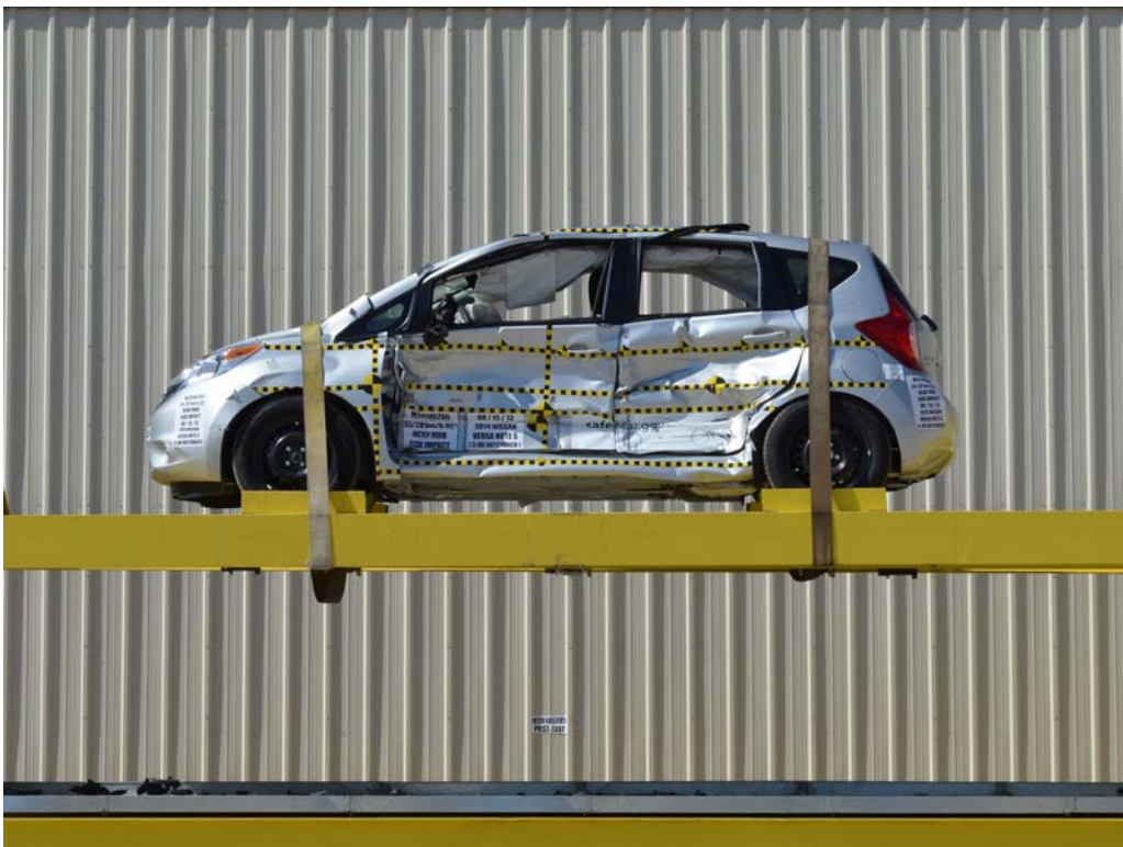
FIGURE 100. FMVSS No. 301 Static Rollover 360 Degrees
