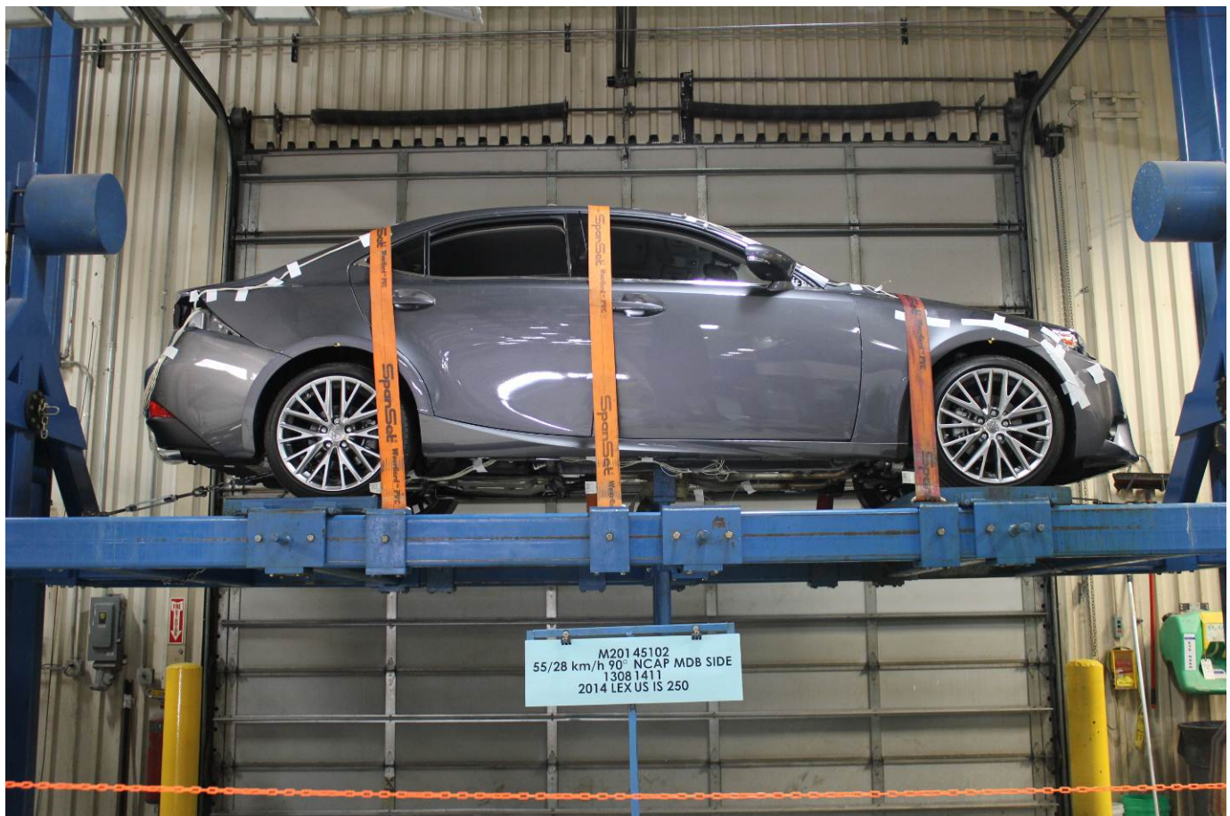
FMVSS No. 301 Static Rollover 0 Degrees
