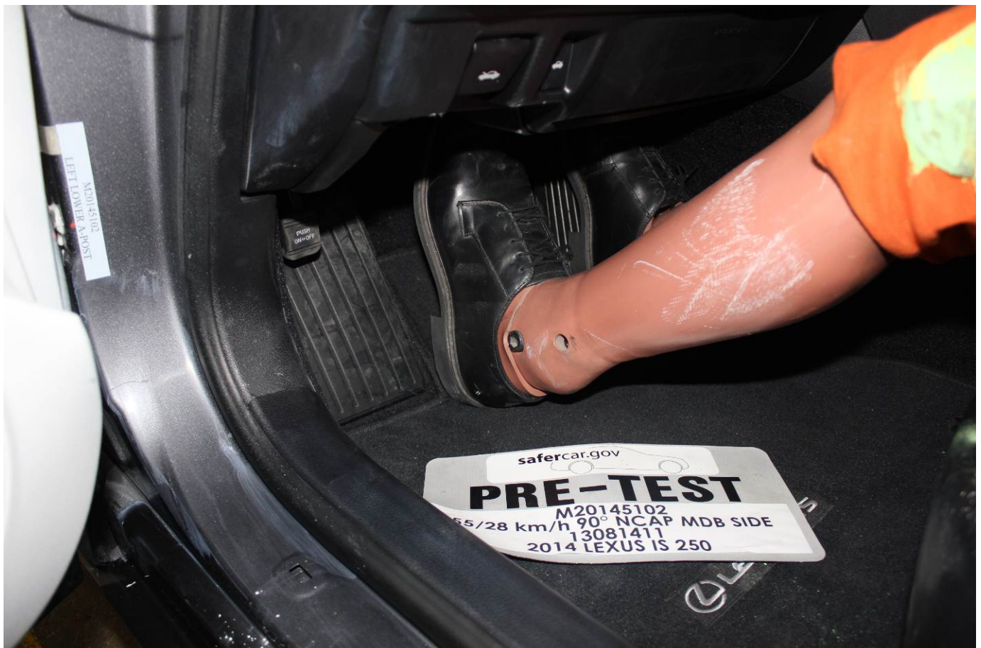
Pre-Test Placement of Driver Dummy's Feet
