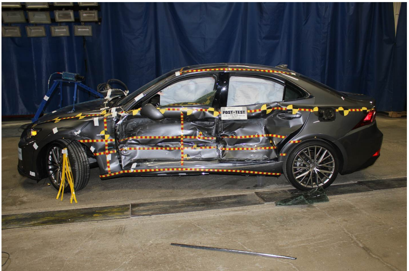
Post-Test Left Side View of Test Vehicle
