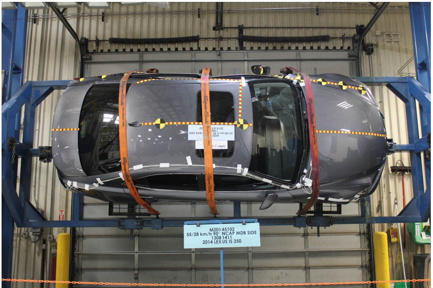
FMVSS No. 301 Static Rollover 270 Degrees
