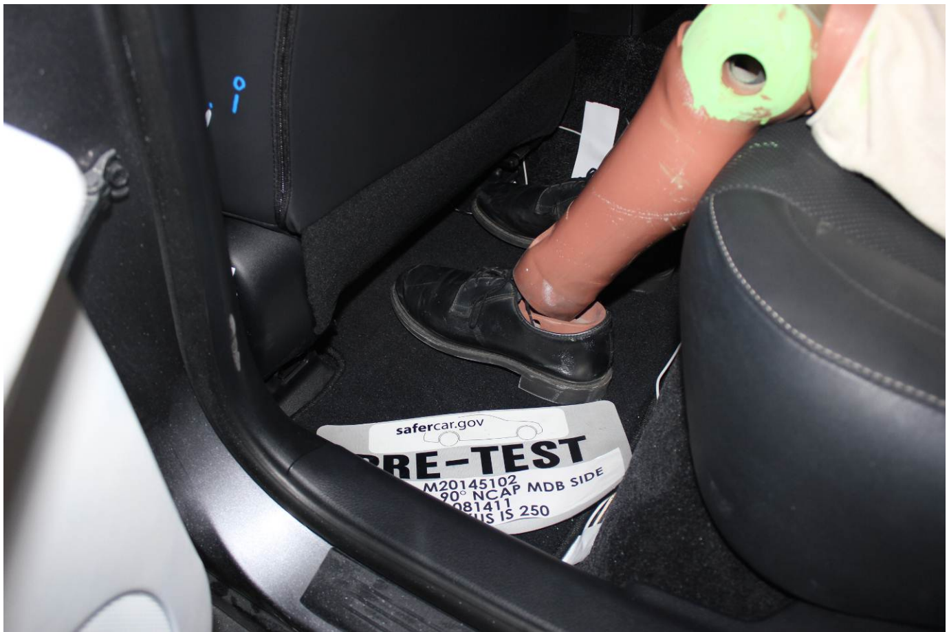
Pre-Test Placement of Rear Passenger Dummy's Feet
