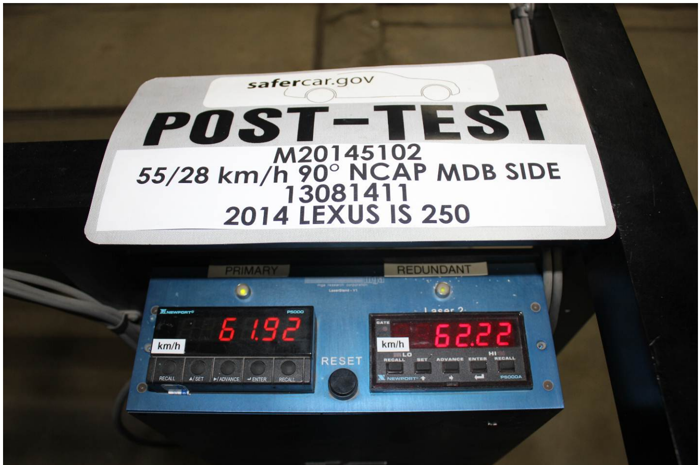
Post-Test Primary and Redundant Speed Trap Read-Out
