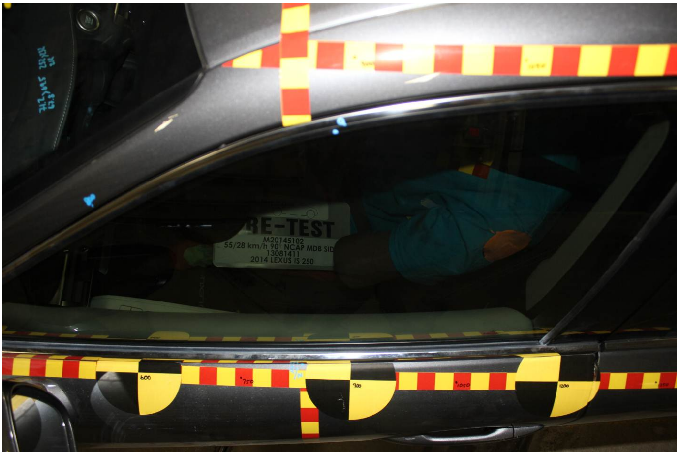
Pre-Test Driver Dummy and Door Clearance View
