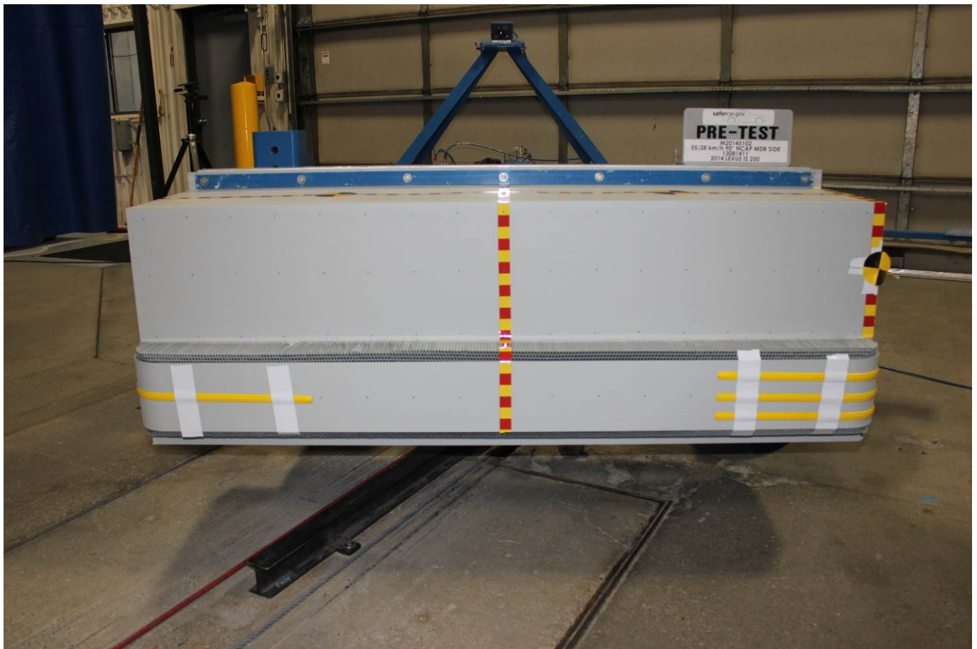
Pre-Test Front View of MDB Impactor Face
