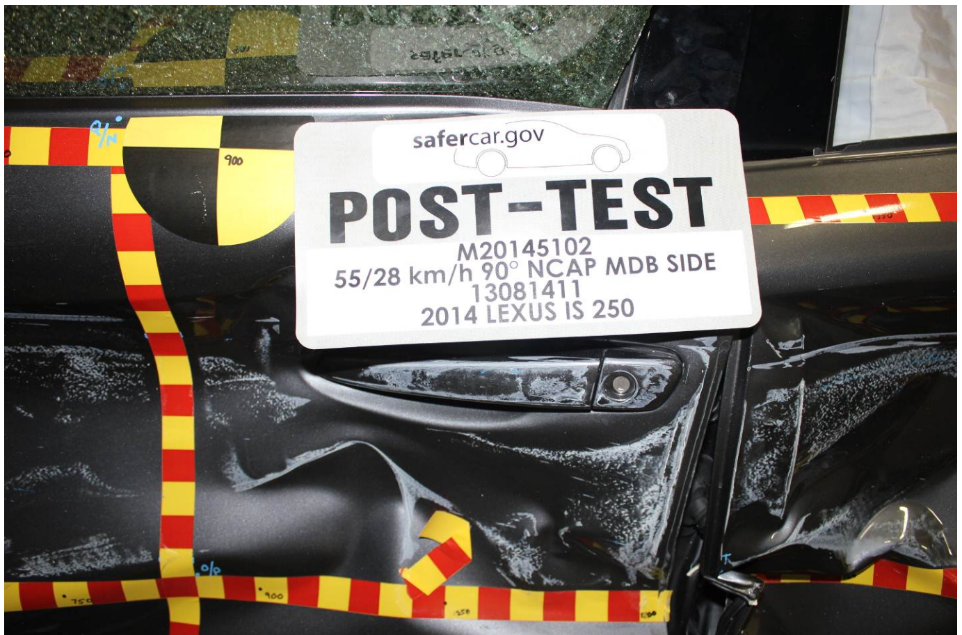
Post-Test Left Front Door Latch Close-Up
