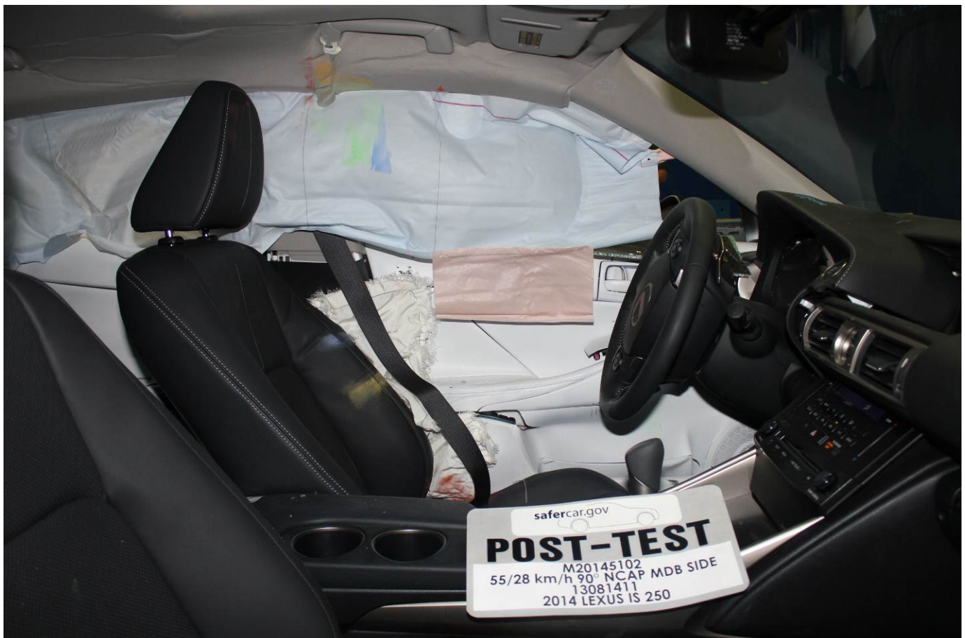
Post-Test Driver Inner Door Panel View
