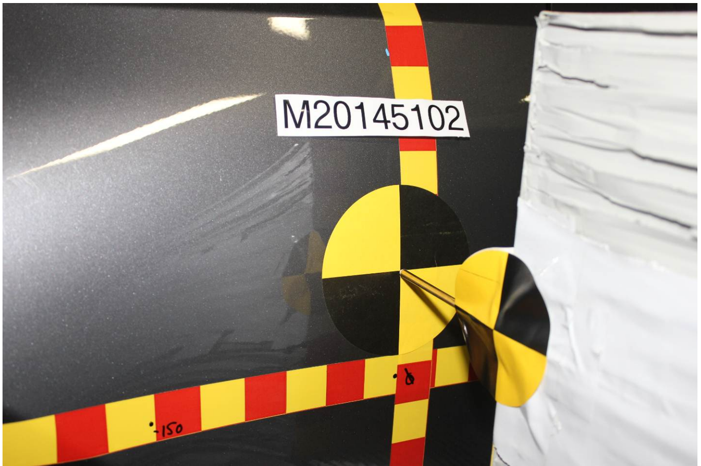
Pre-Test Close-Up View of Impact Point Target
