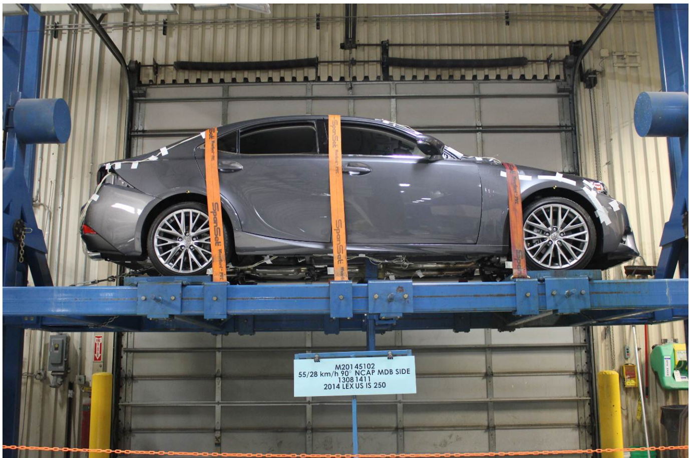
FMVSS No. 301 Static Rollover 360 Degrees
