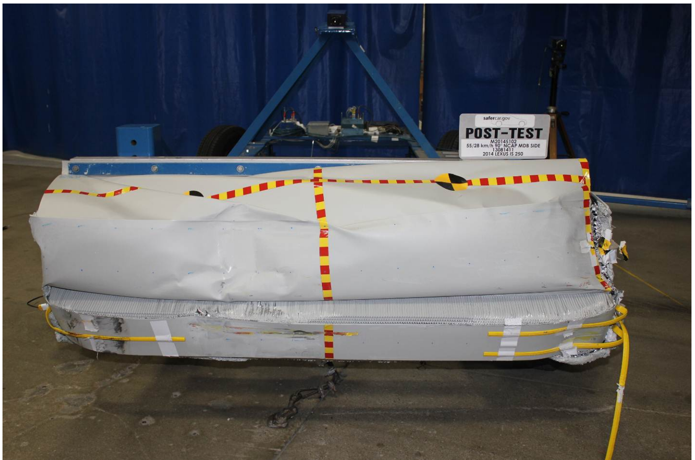
Post-Test Front View of MDB Impactor Face
