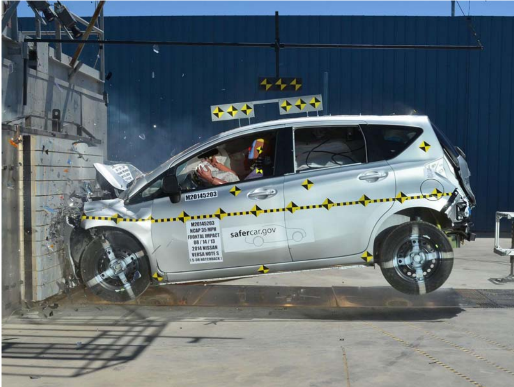
FIGURE 75. 2014 Nissan Versa Note Frontal Impact Event
