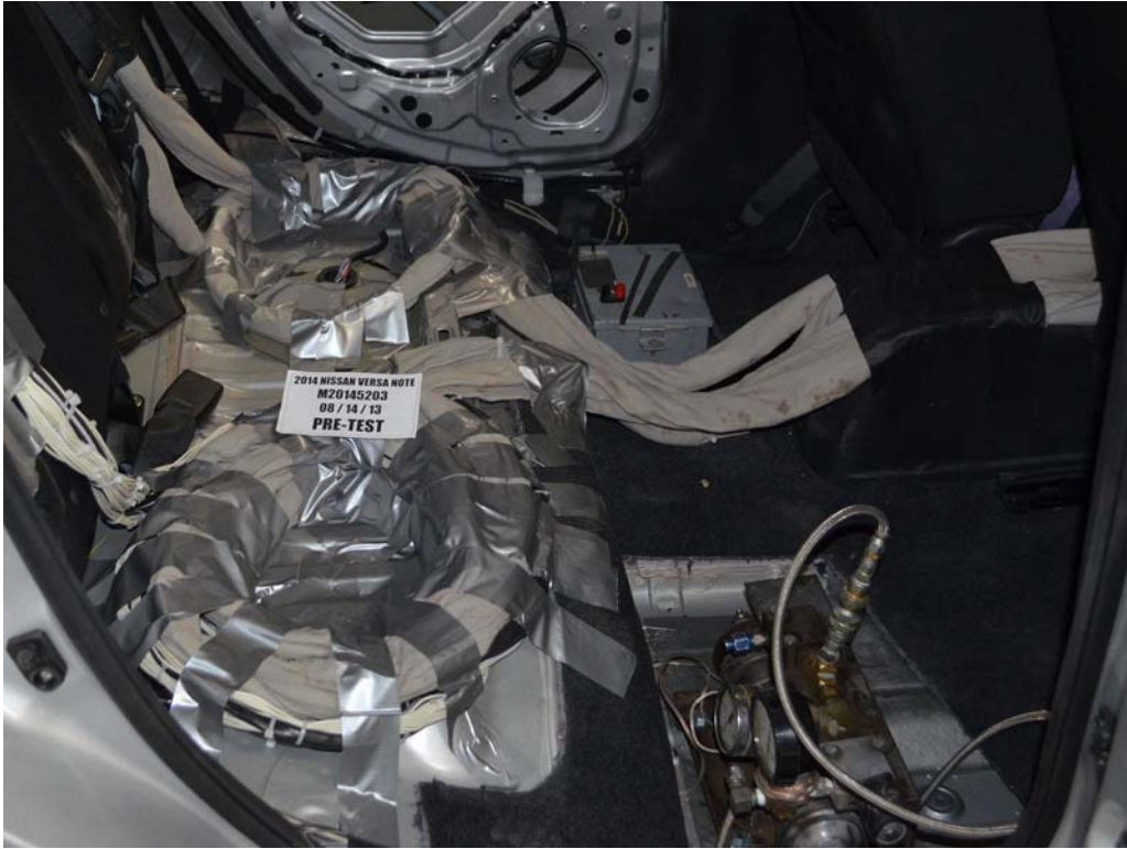
FIGURE 27. Pre-Test Dummy Cable Routing
