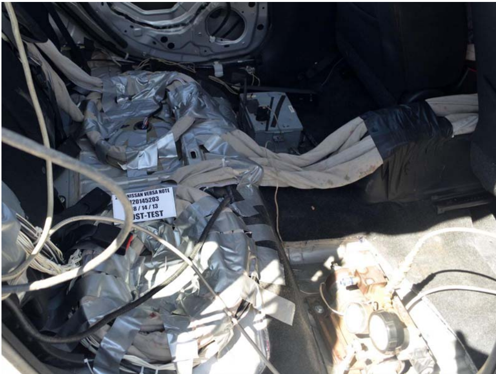
FIGURE 28. Post-Test Dummy Cable Routing
