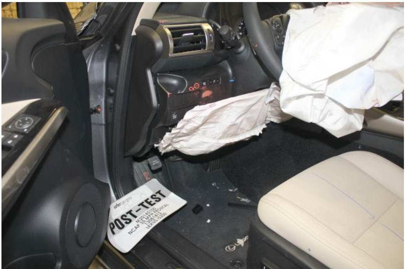
Post-Test Driver Dummy Contact with Knee Bolster
