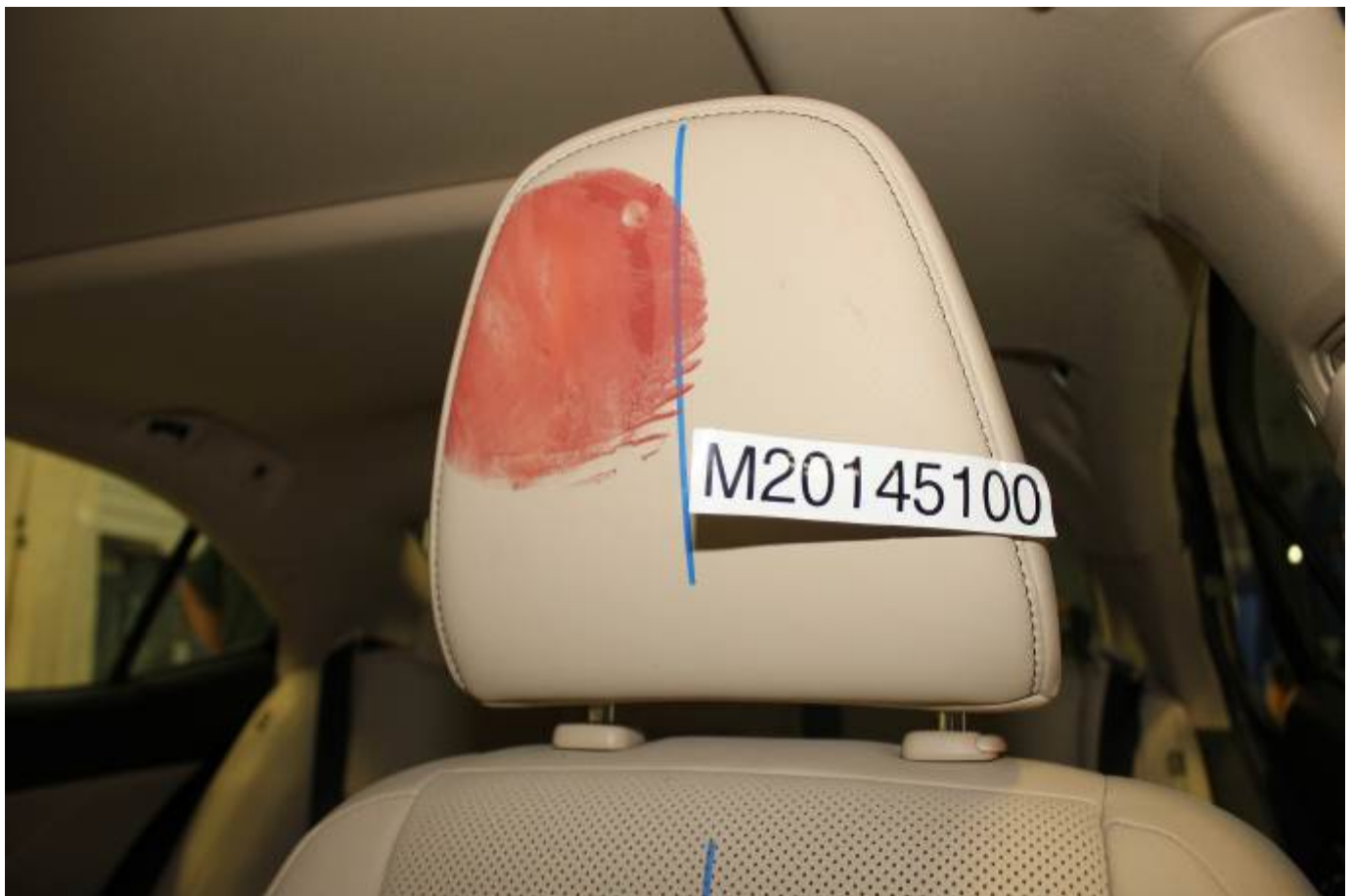
Post-Test Driver Dummy Contact with Headrest
