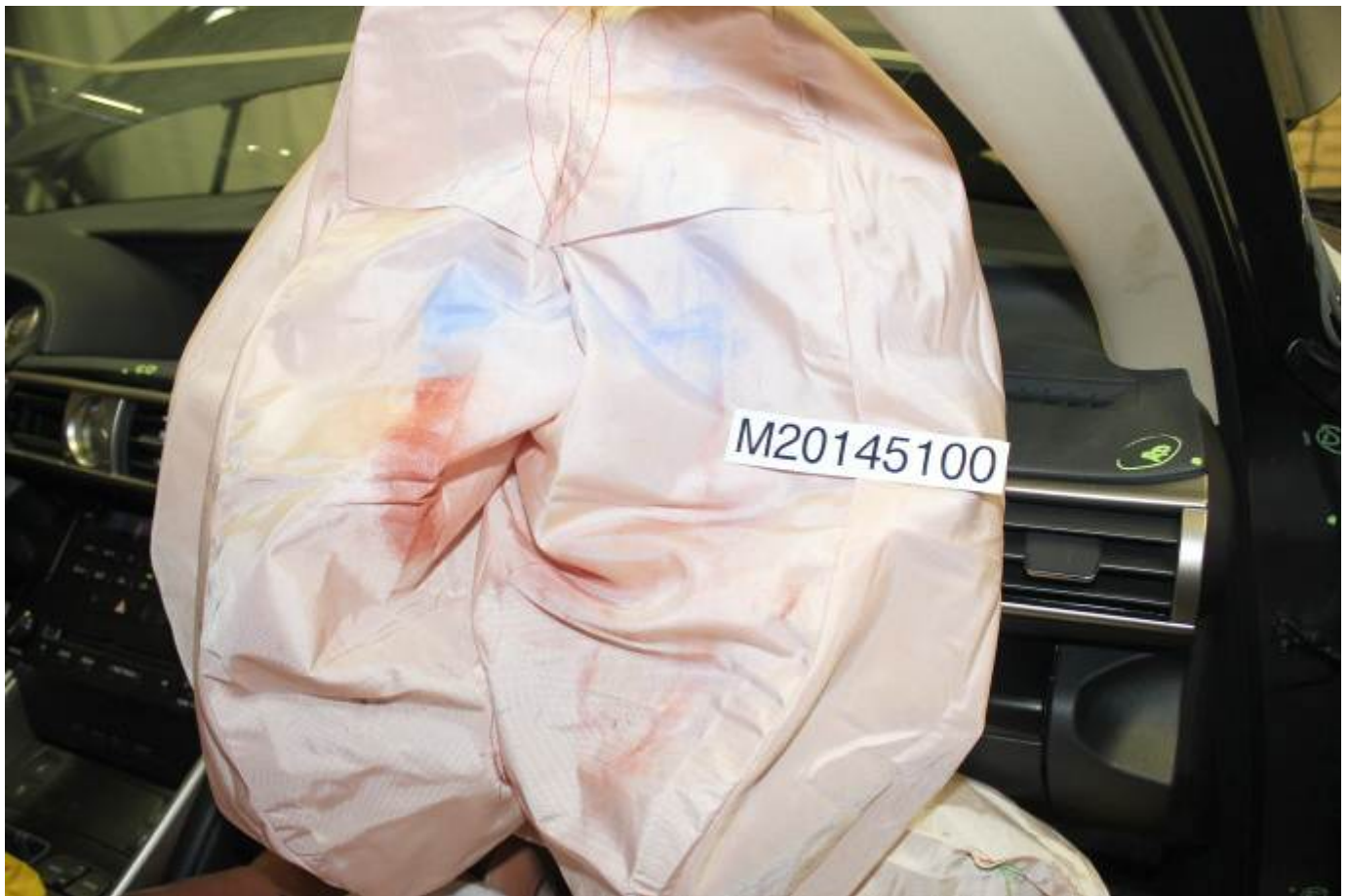
Post-Test Passenger Dummy Contact with Airbag
