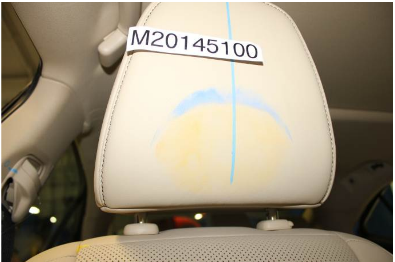
Post-Test Passenger Dummy Contact with Headrest
