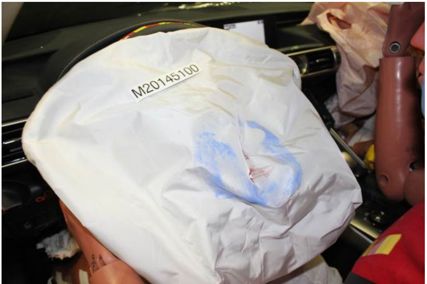
Post-Test Driver Dummy Contact with Airbag
