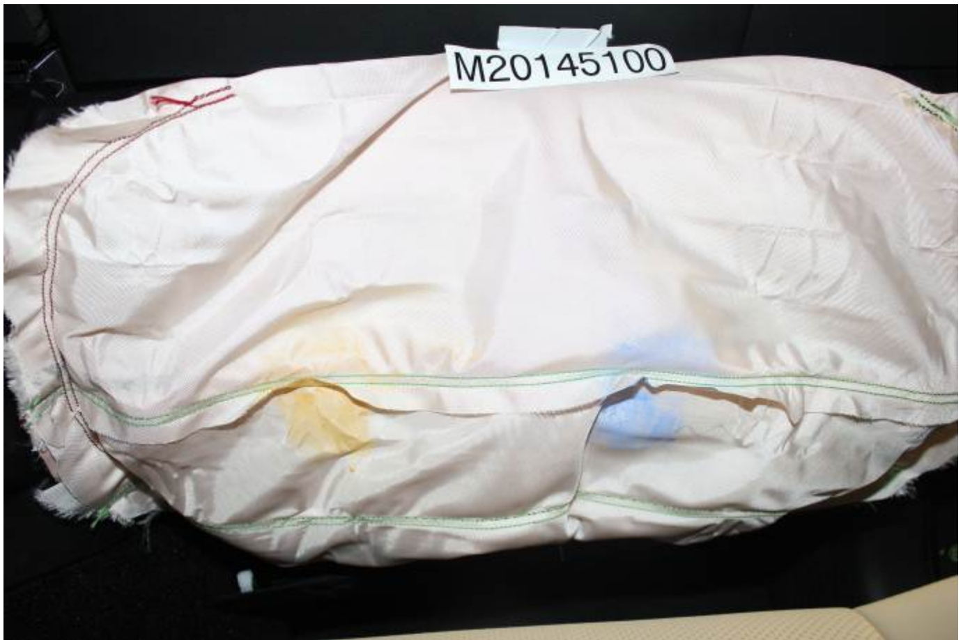
Post-Test Passenger Dummy Contact with Knee Airbag
