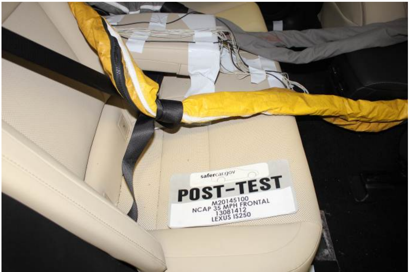
Post-Test Dummy Cable Routing
