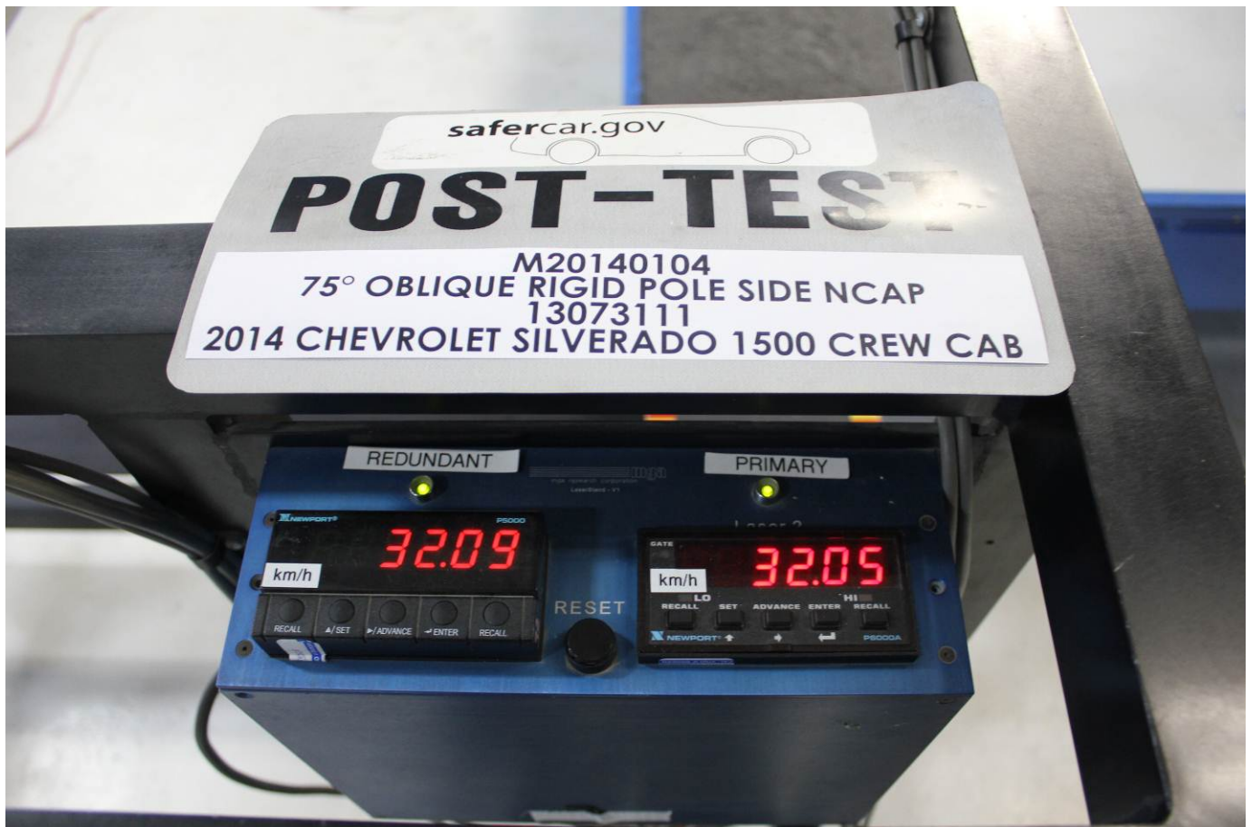
Post-Test Primary and Redundant Speed Trap Read-Out
