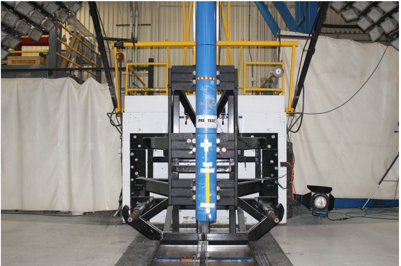
Pre-Test Pole Barrier Front View
