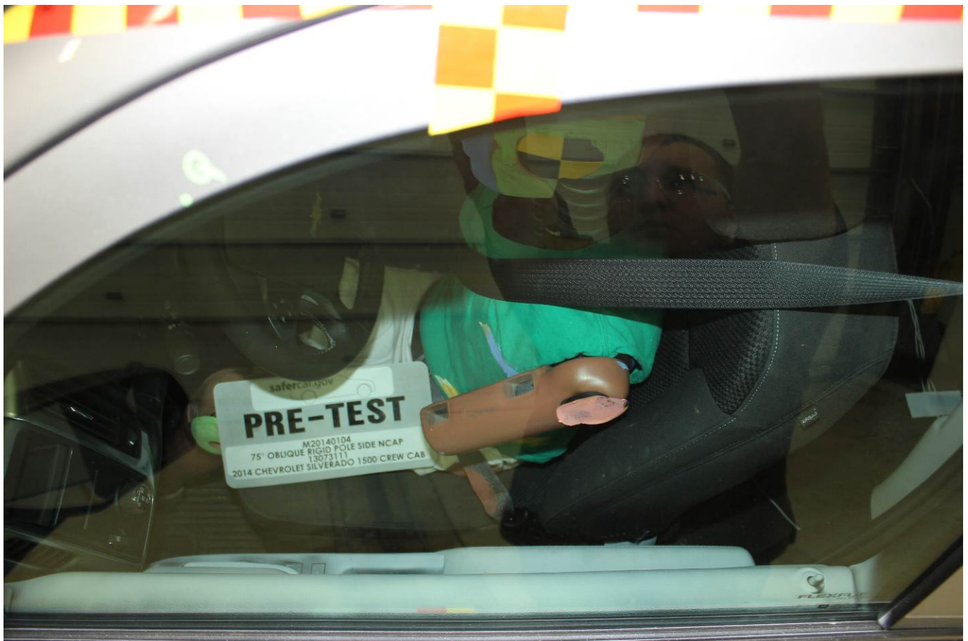
Pre-Test Dummy and Door Clearance View
