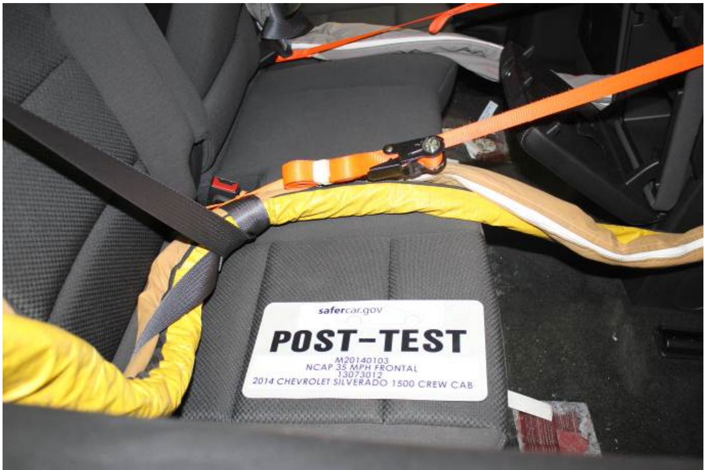
Post-Test Dummy Cable Routing
