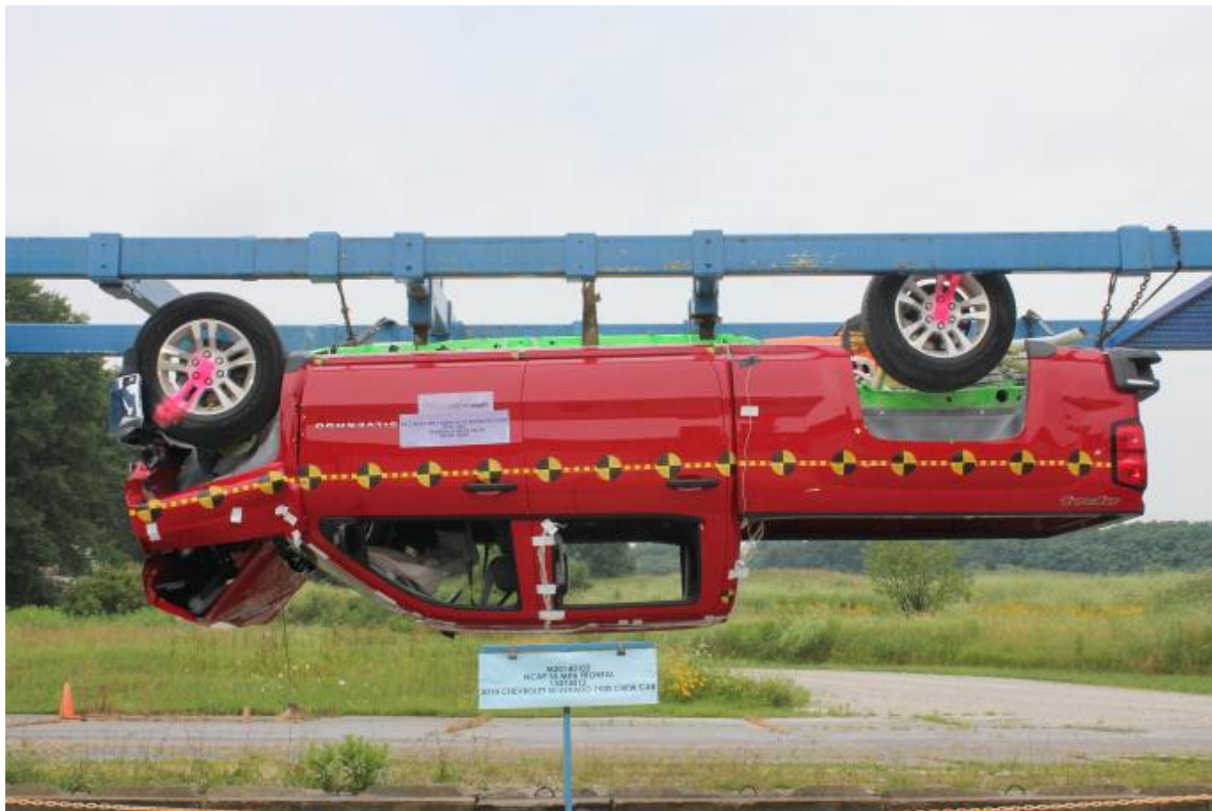
Vehicle at 180° on Static Rollover Device
