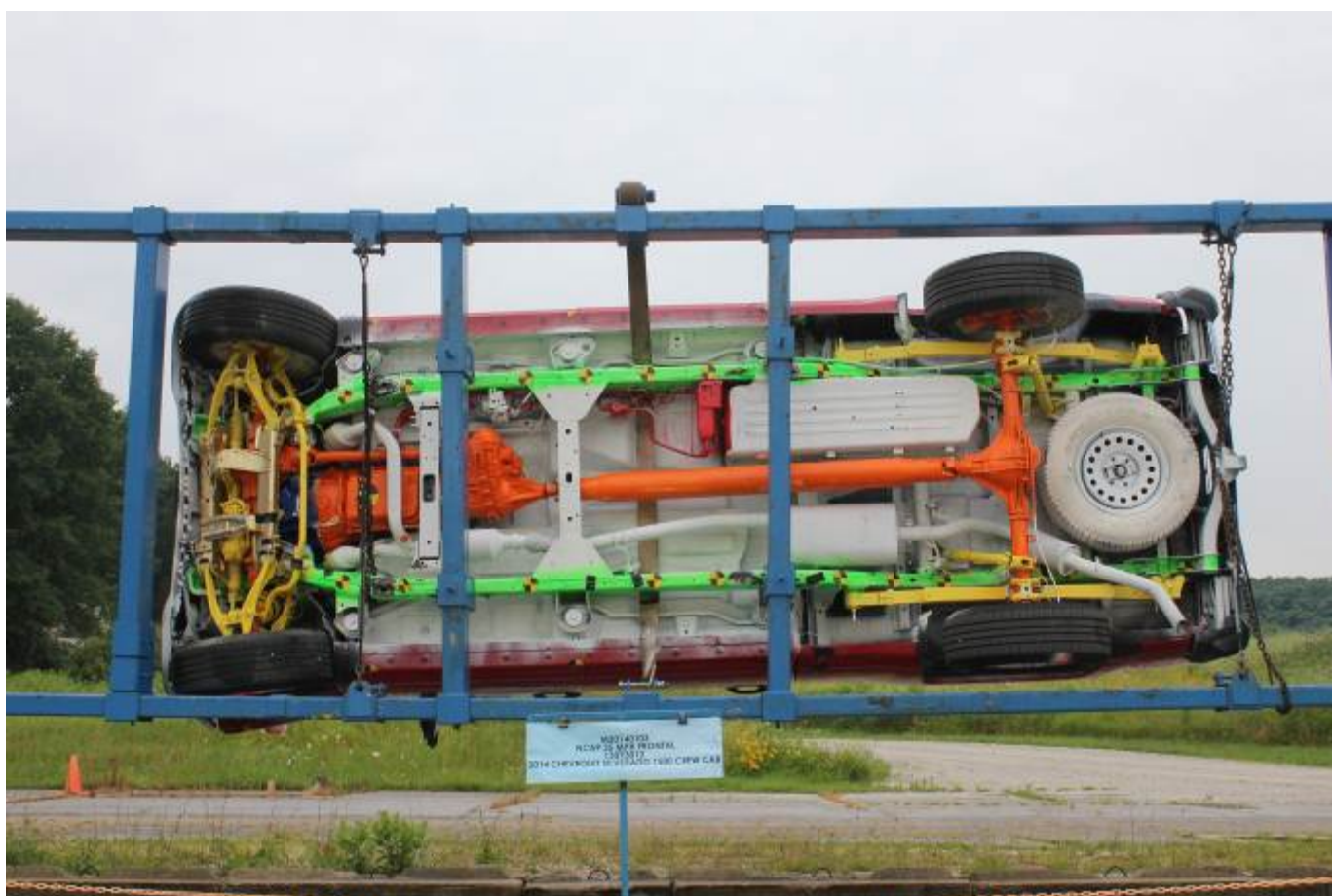
Vehicle at 270° on Static Rollover Device
