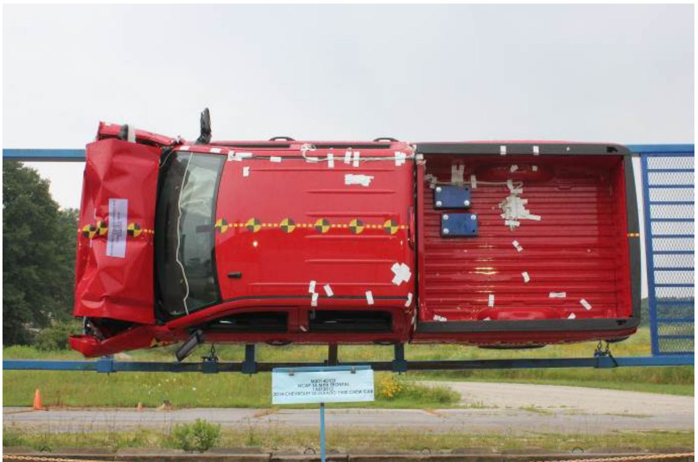
Vehicle at 90° on Static Rollover Device
