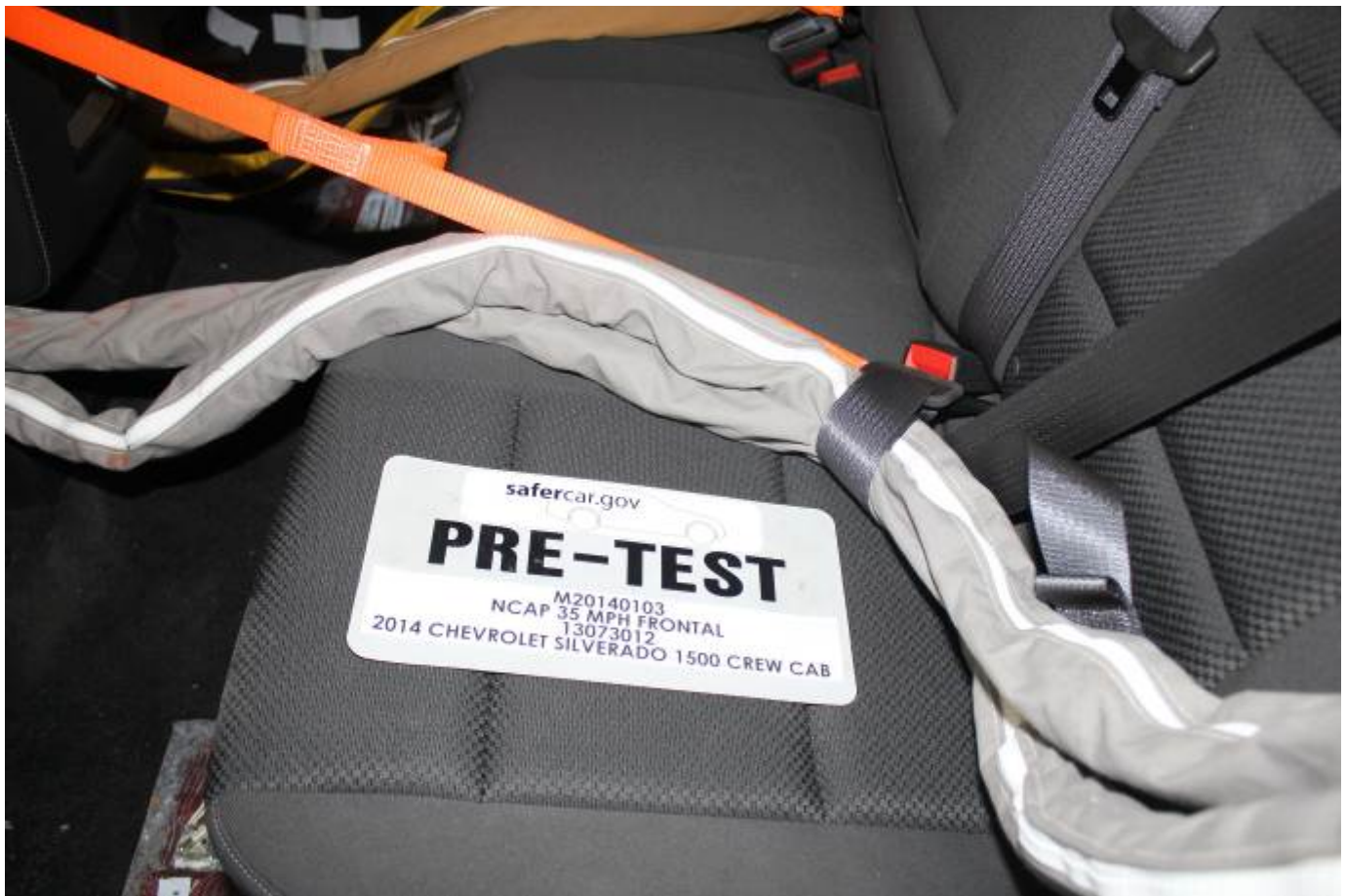
Pre-Test Dummy Cable Routing
