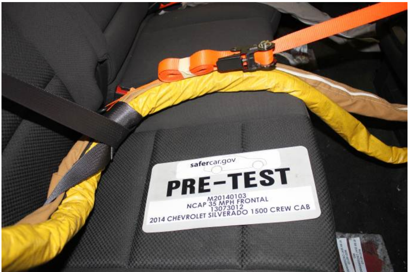
Pre-Test Dummy Cable Routing
