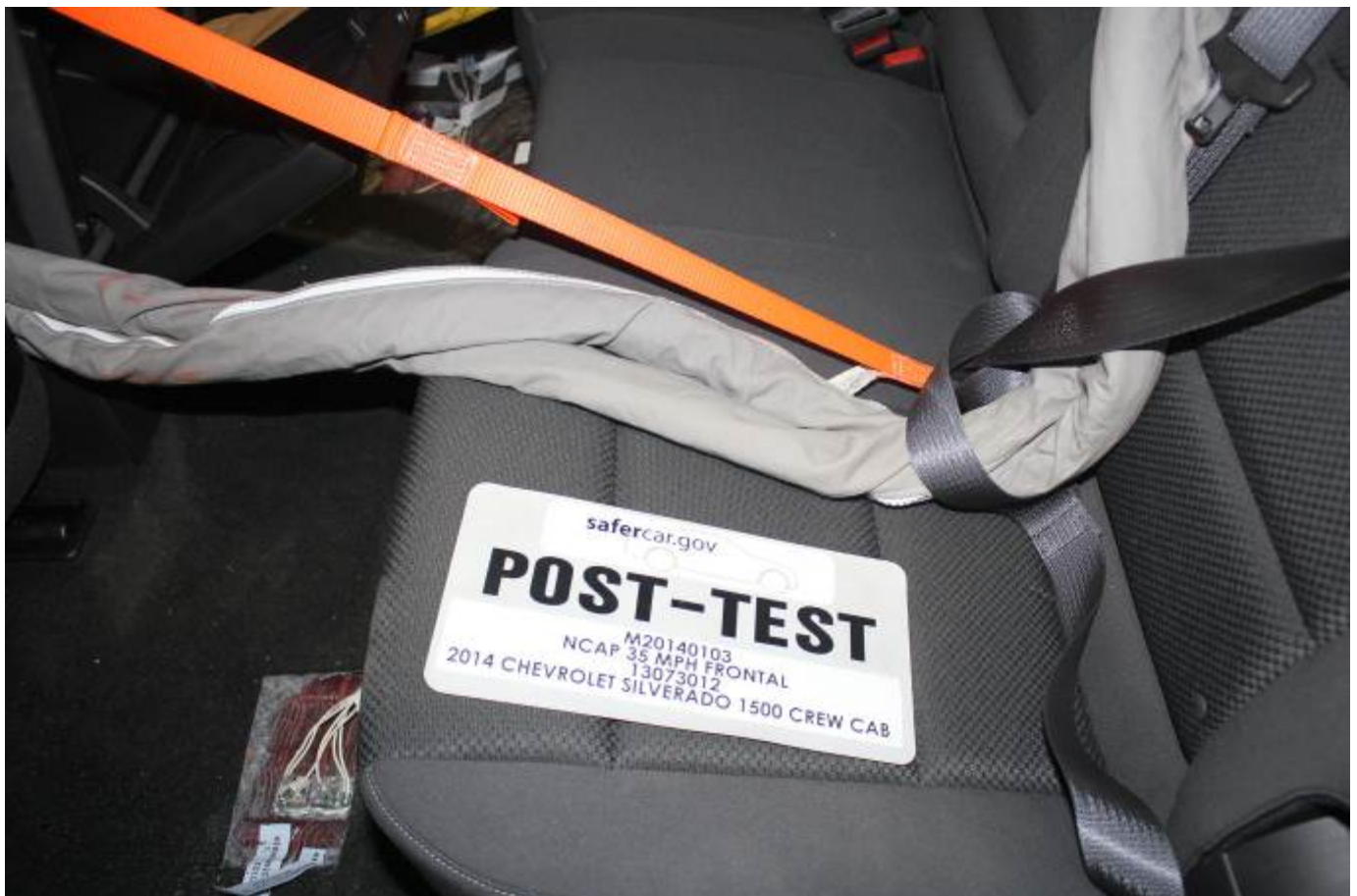
Post-Test Dummy Cable Routing
