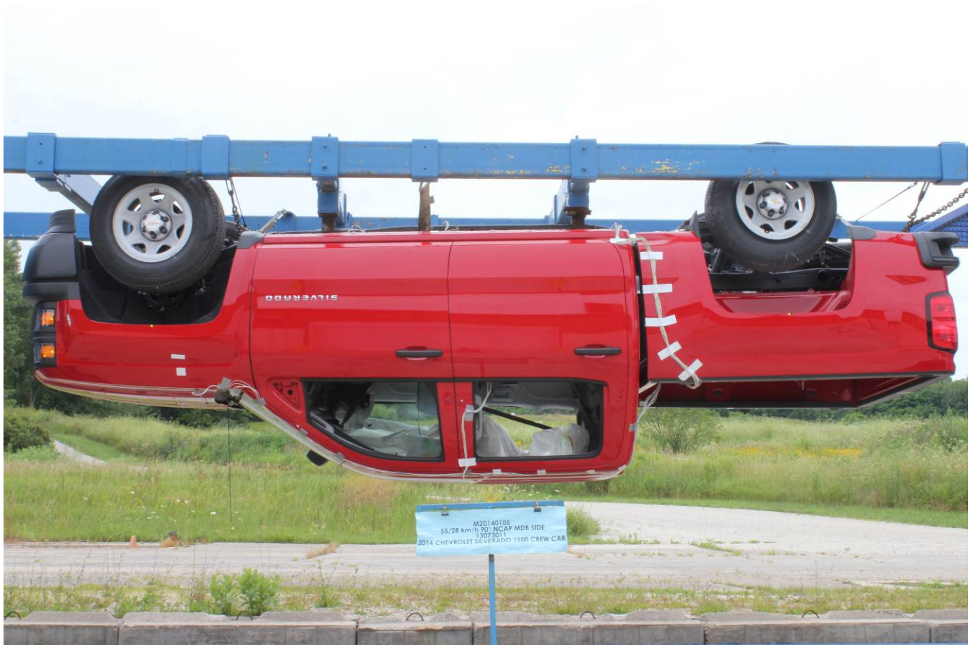
FMVSS No. 301 Static Rollover 180 Degrees
