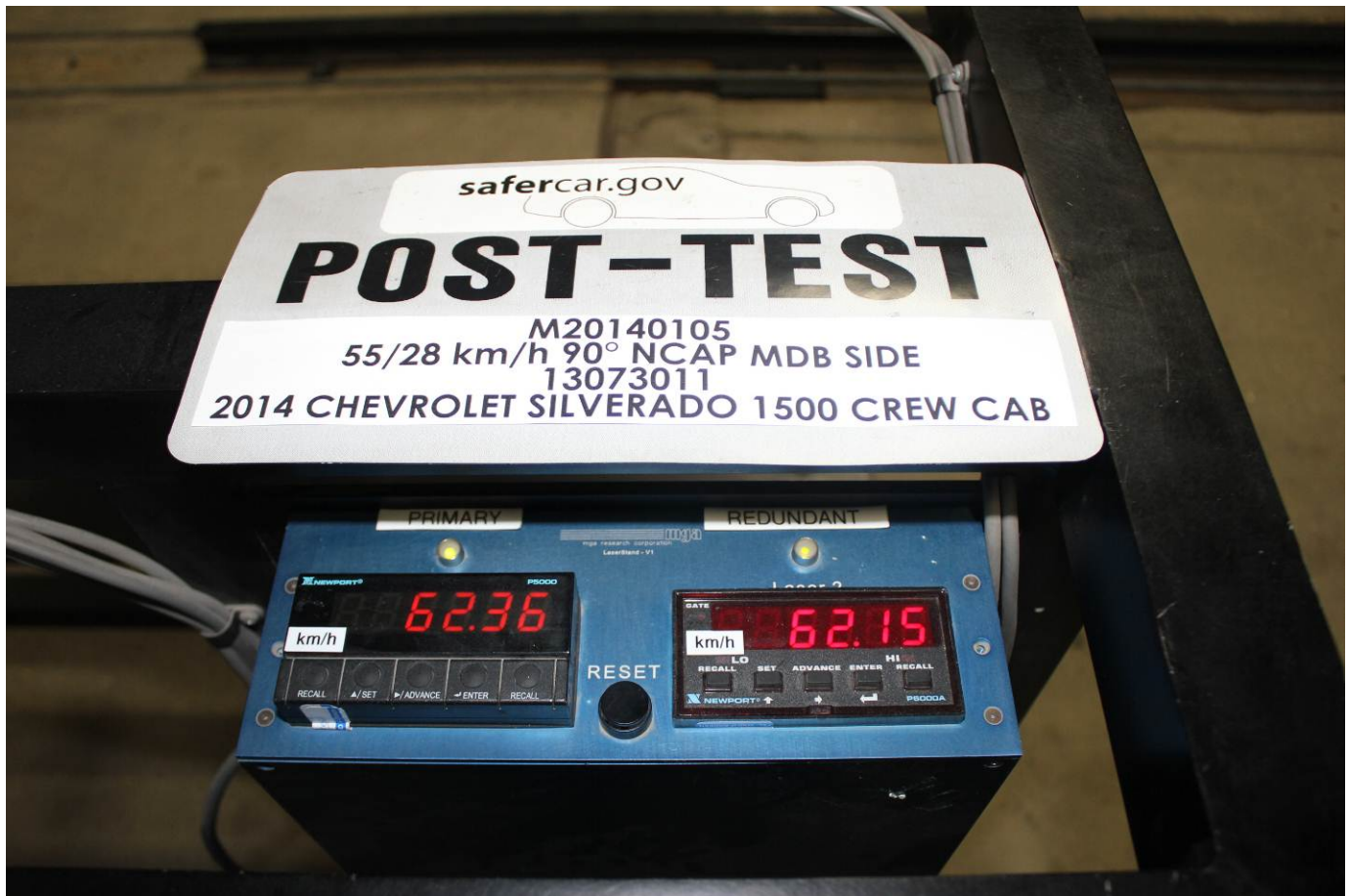
Post-Test Primary and Redundant Speed Trap Read-Out
