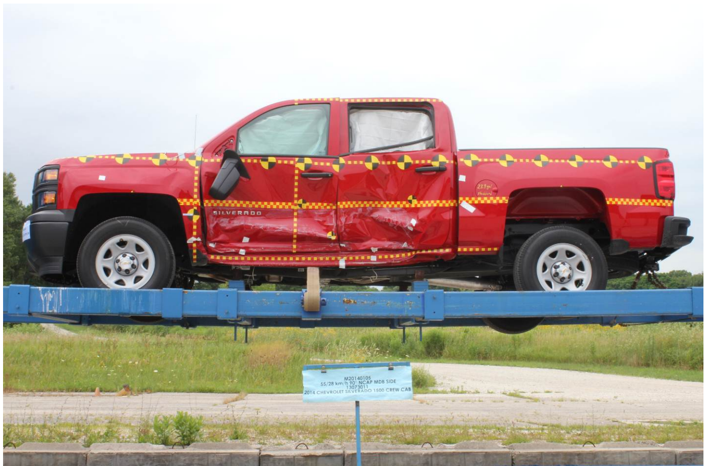
FMVSS No. 301 Static Rollover 0 Degrees
