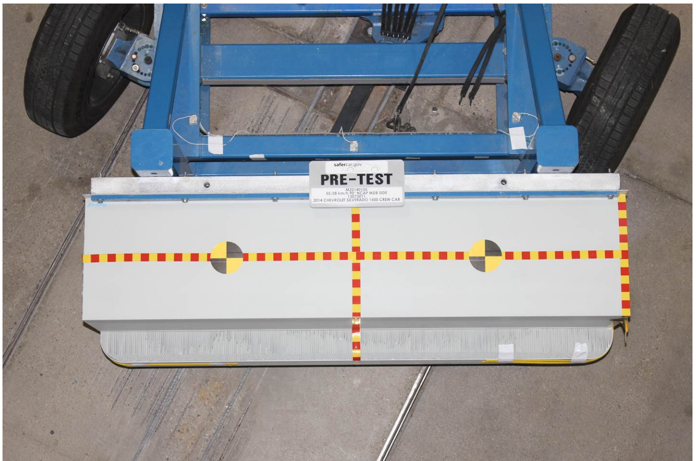
Pre-Test Top View of MDB Impactor Face
