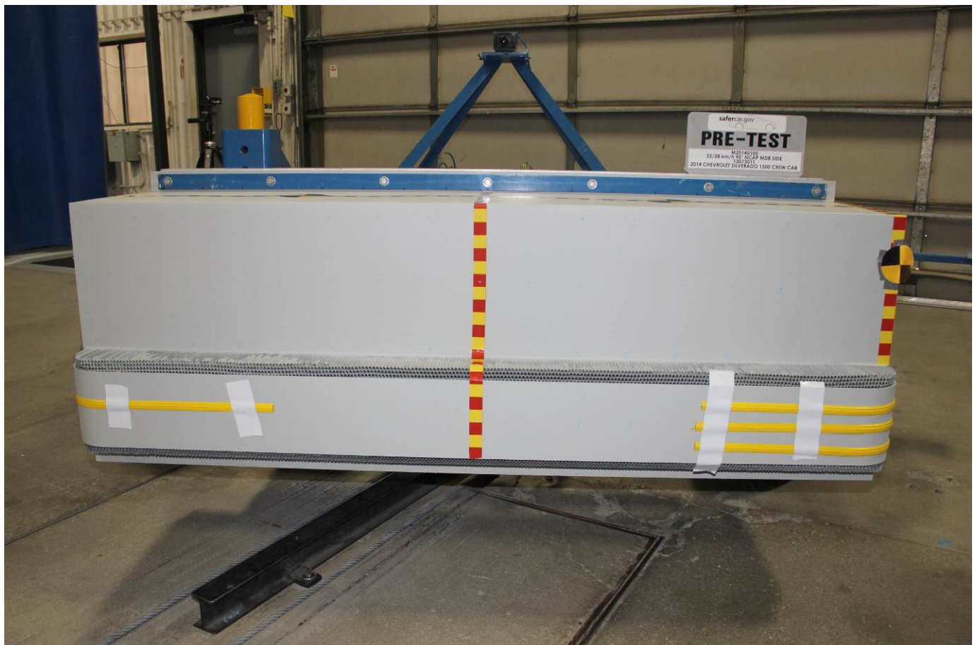
Pre-Test Front View of MDB Impactor Face
