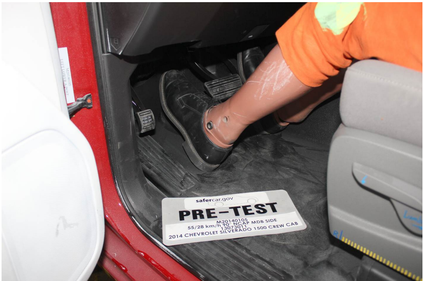
Pre-Test Placement of Driver Dummy's Feet
