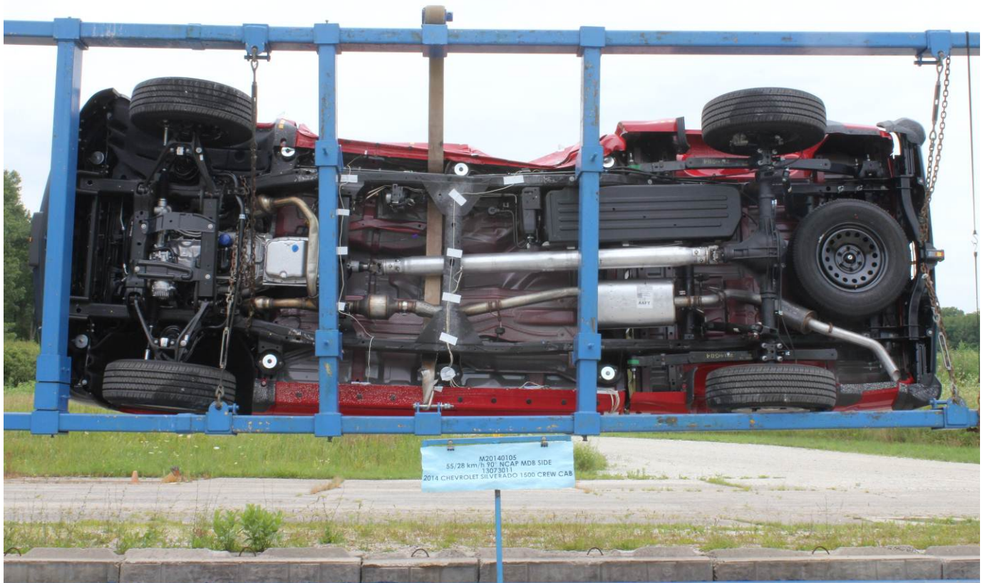
FMVSS No. 301 Static Rollover 270 Degrees
