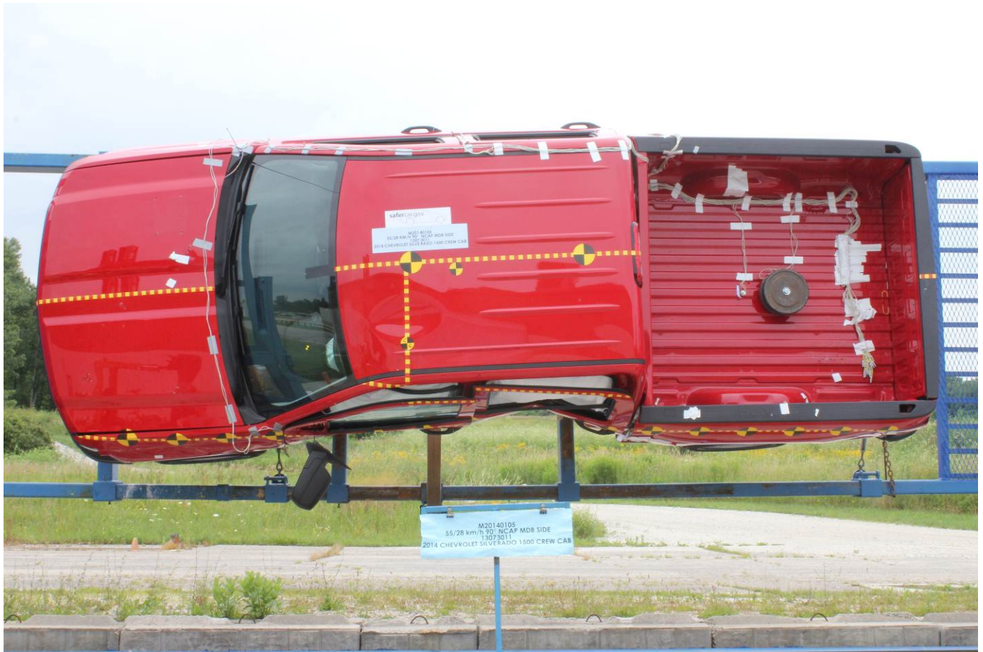
FMVSS No. 301 Static Rollover 90 Degrees
