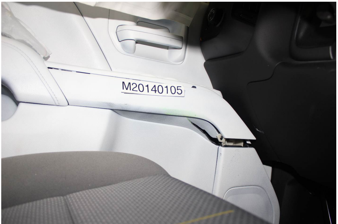
Post-Test Driver Dummy Close-up Knee Contact View
