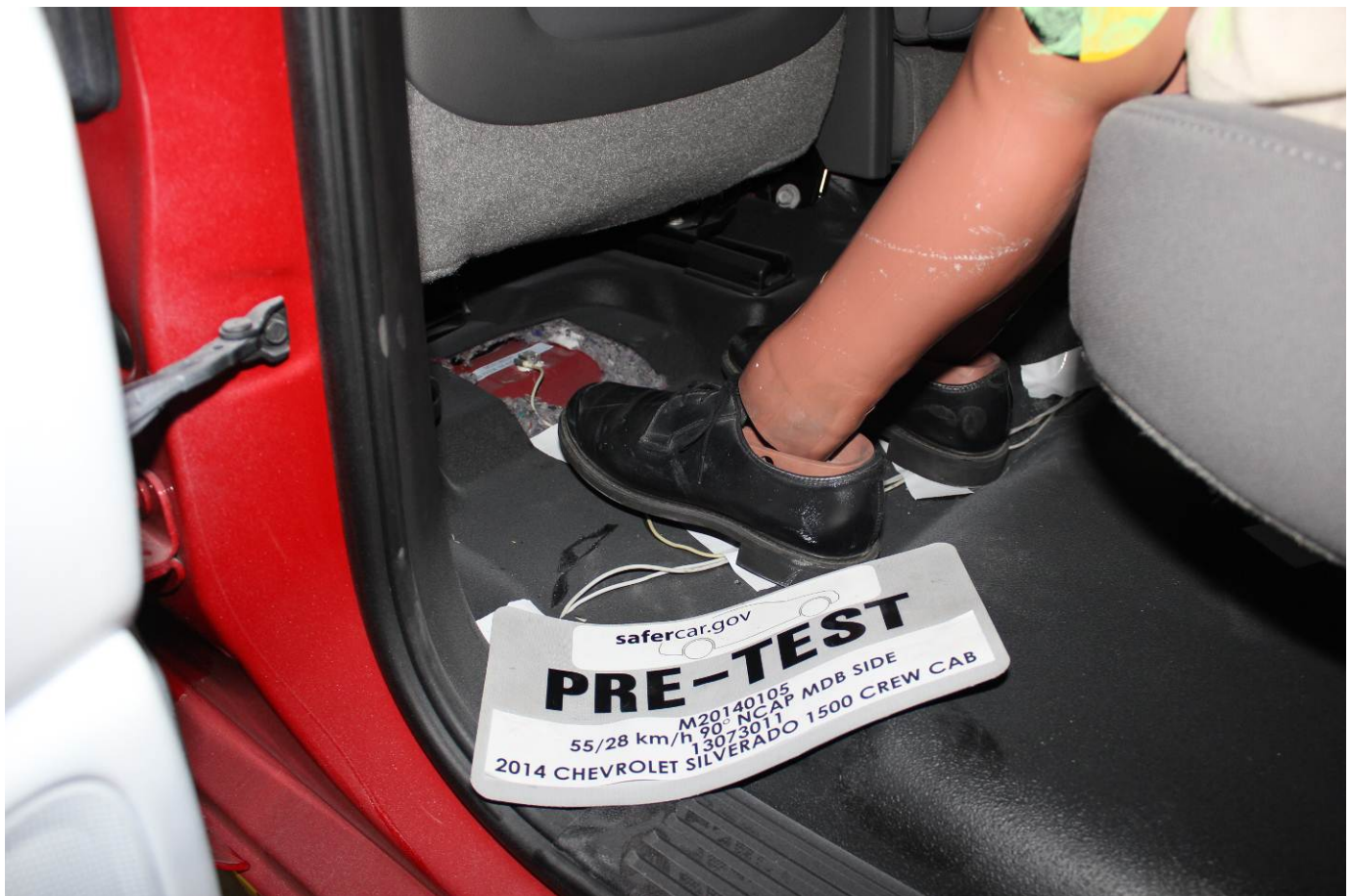
Pre-Test Placement of Rear Passenger Dummy's Feet
