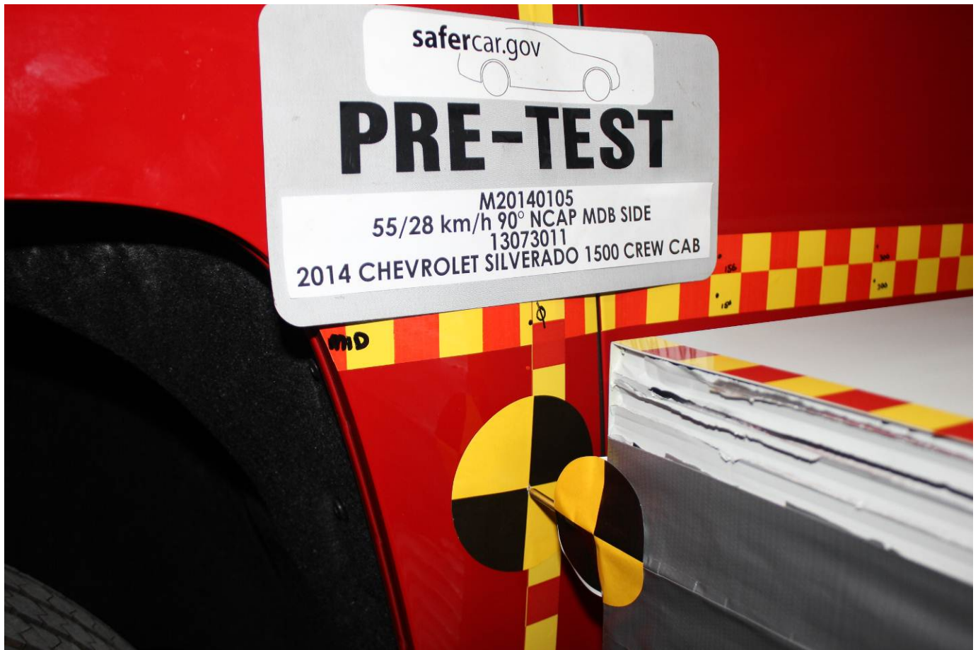
Pre-Test Close-Up View of Impact Point Target
