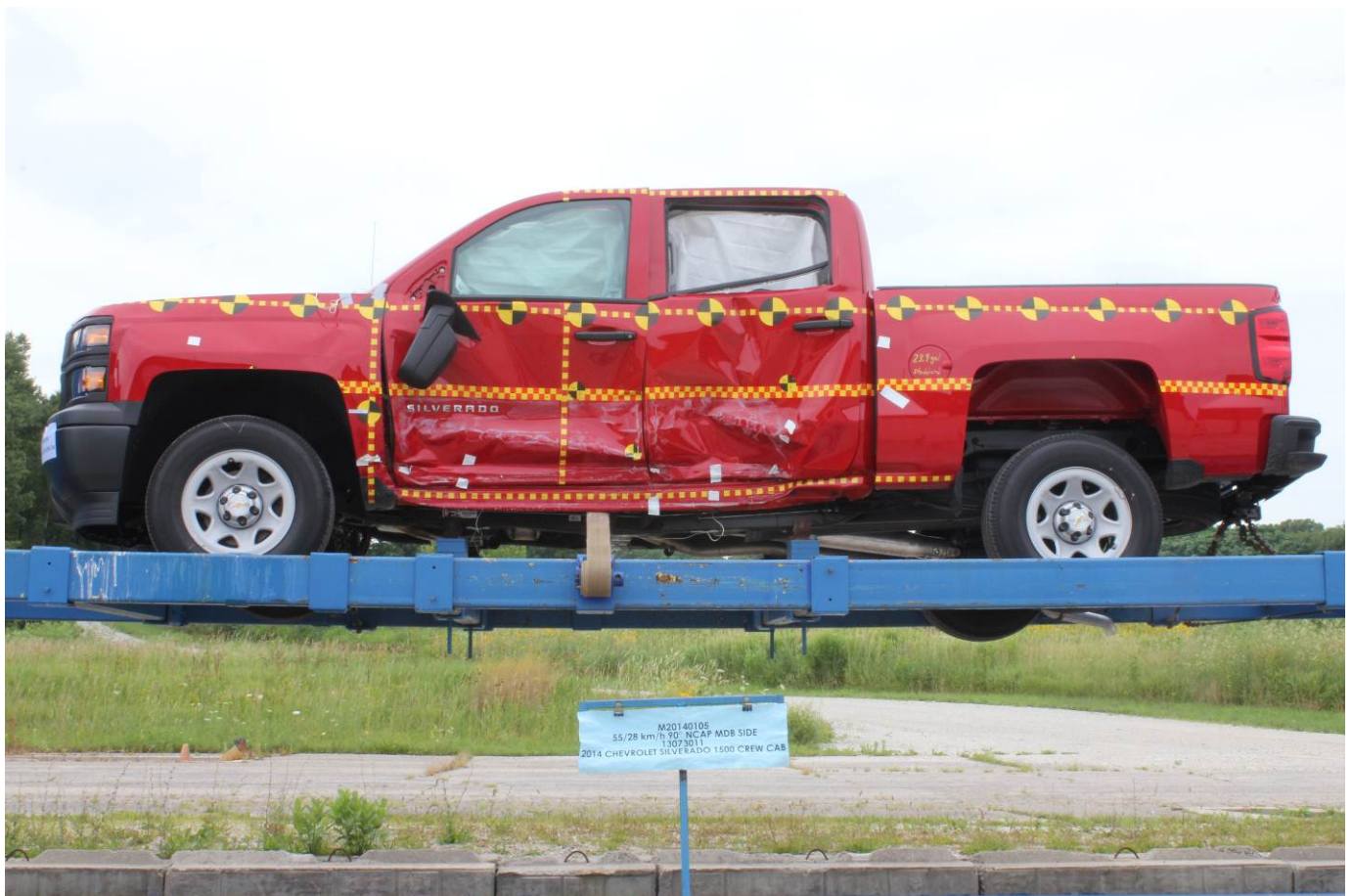
FMVSS No. 301 Static Rollover 360 Degrees
