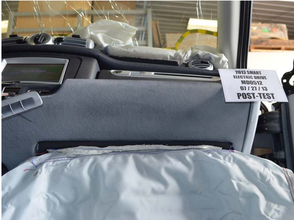
FIGURE 63. Post-Test Passenger's Side Knee Bolster
