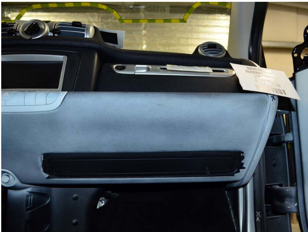
FIGURE 62. Pre-Test Passenger's Side Knee Bolster
