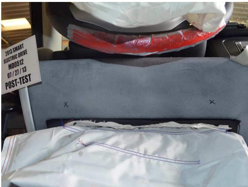
FIGURE 42. Post-Test Driver's Side Knee Bolster
