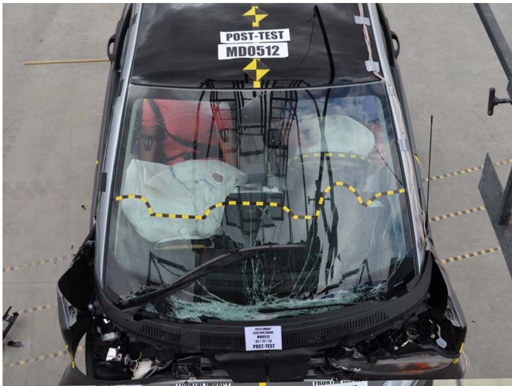
FIGURE 18. Post-Test Windshield View
