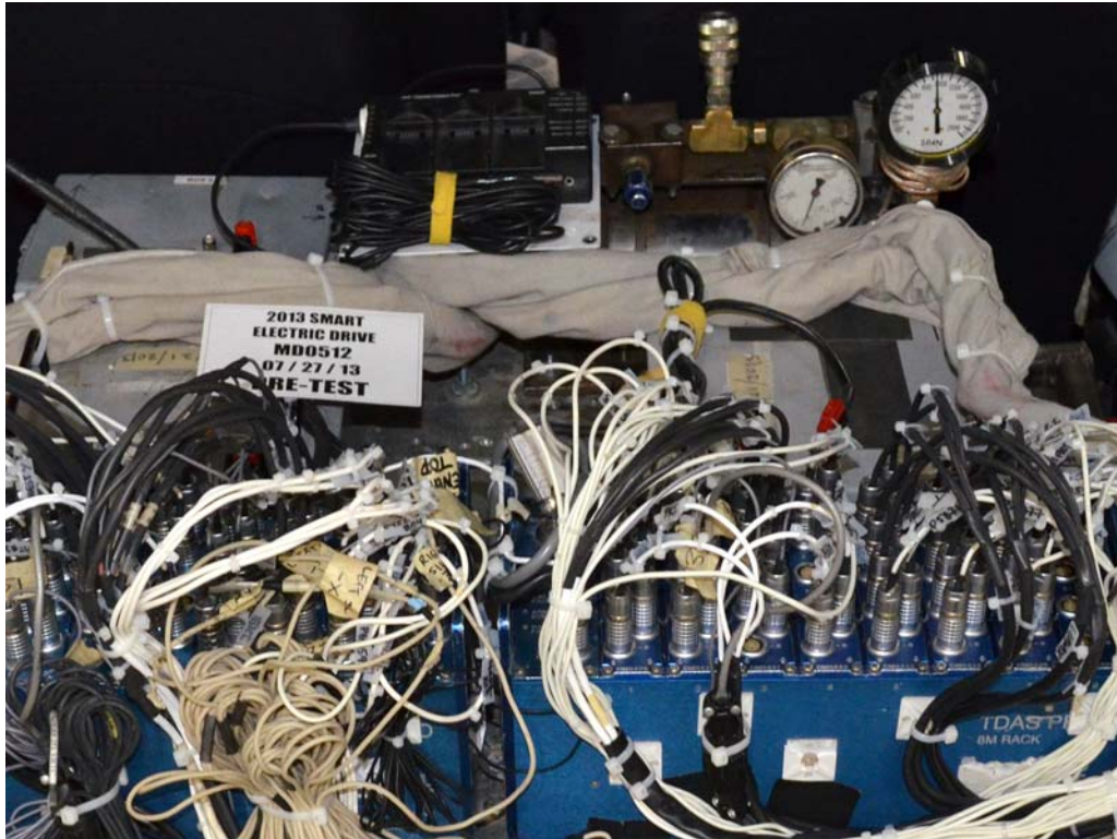
FIGURE 27. Pre-Test Dummy Cable Routing
