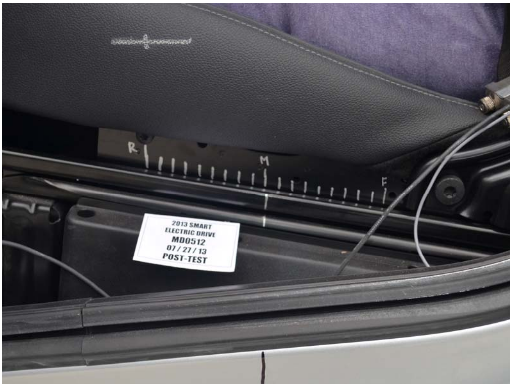
FIGURE 36. Post-Test Driver's Seat Fore-Aft Markings
