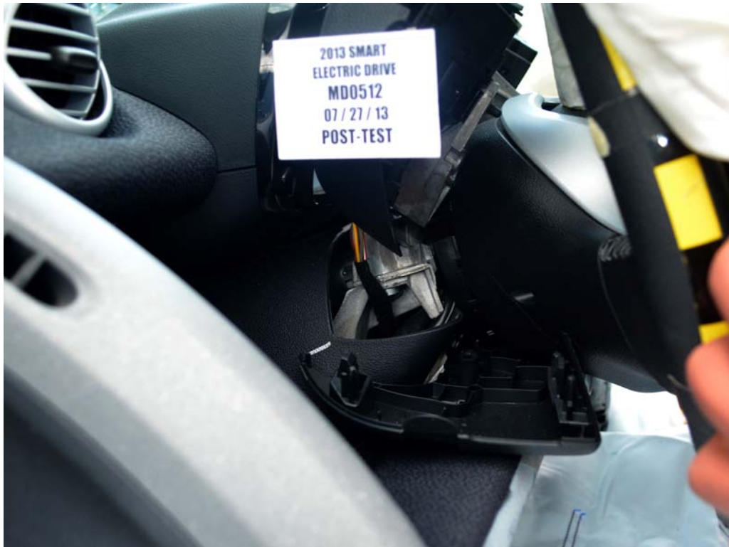
FIGURE 49. Post-Test View of the Steering Wheel
