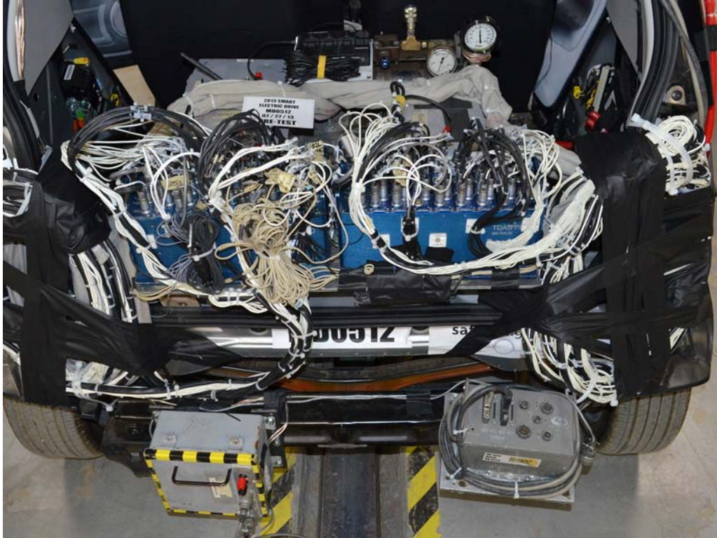
FIGURE 67. Photograph of Ballast Installed in Vehicle
