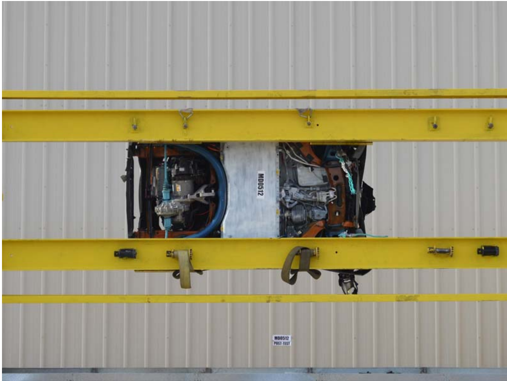
FIGURE 73. Vehicle at 270° on Static Rollover Device
