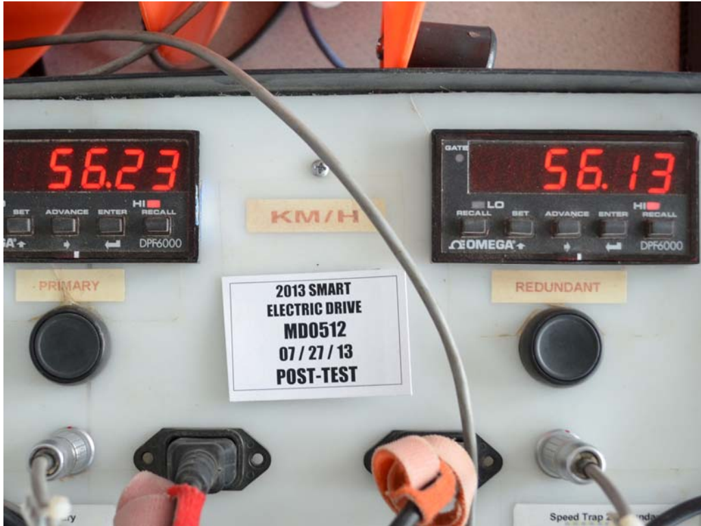
FIGURE 69. Post-Test Speed Trap Read-Out
