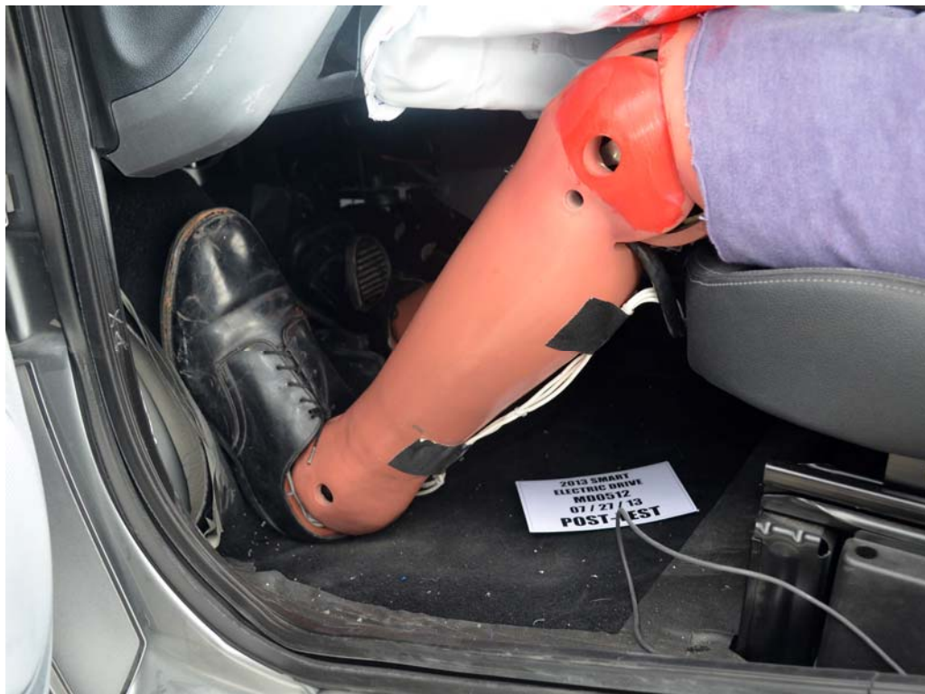
FIGURE 40. Post-Test Driver Dummy Feet
