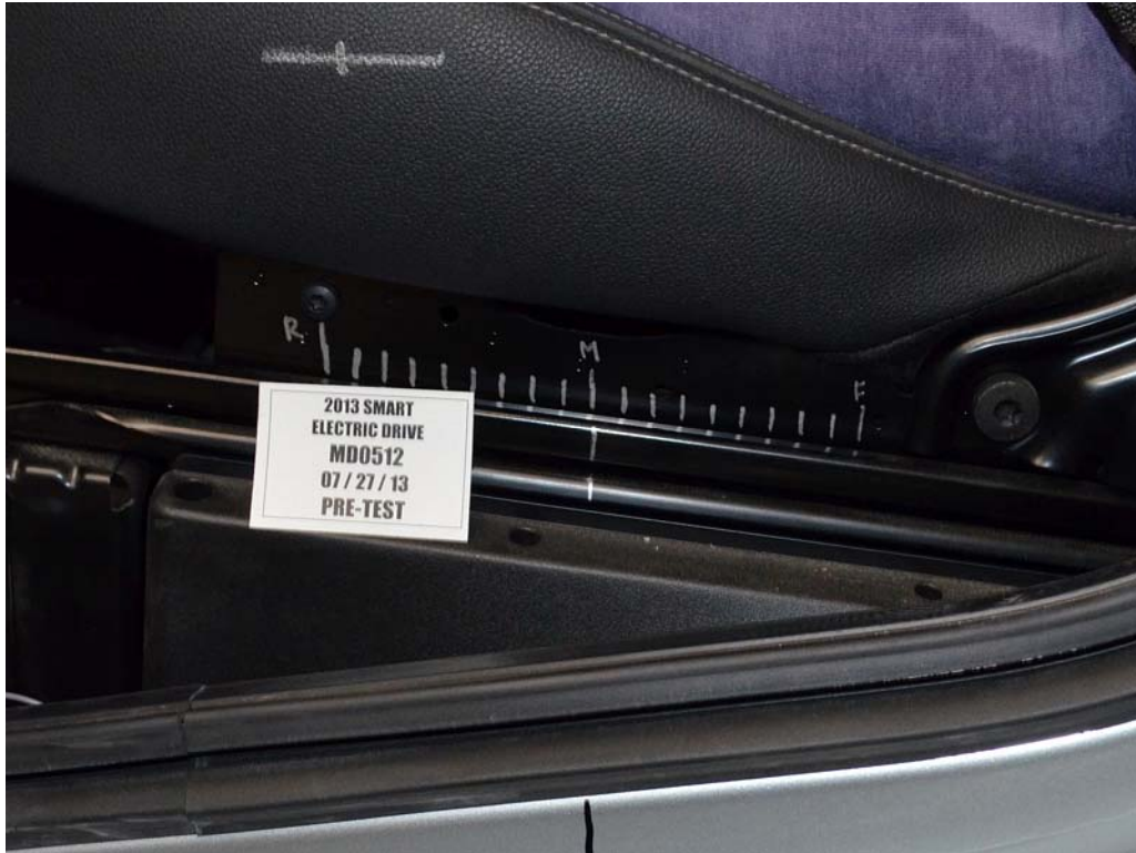
FIGURE 35. Pre-Test Driver's Seat Fore-Aft Markings
