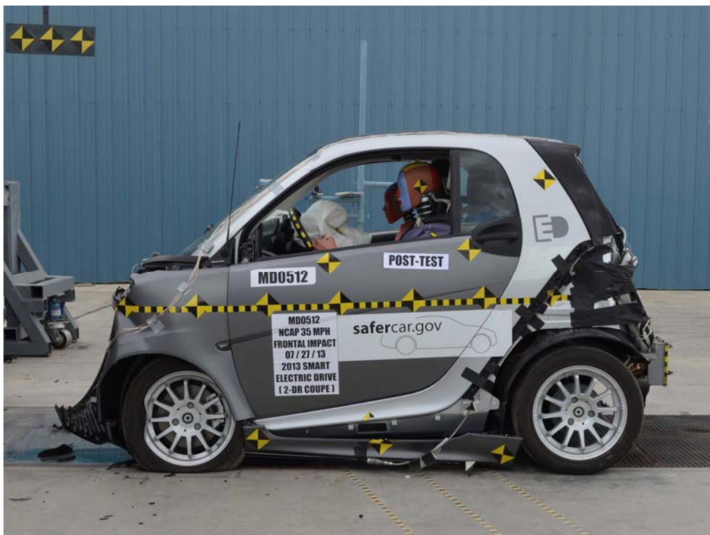
FIGURE 10. Post-Test Left View of Test Vehicle
