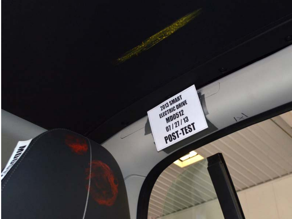
FIGURE 47. Post-Test Driver Dummy Contact with Headrest
