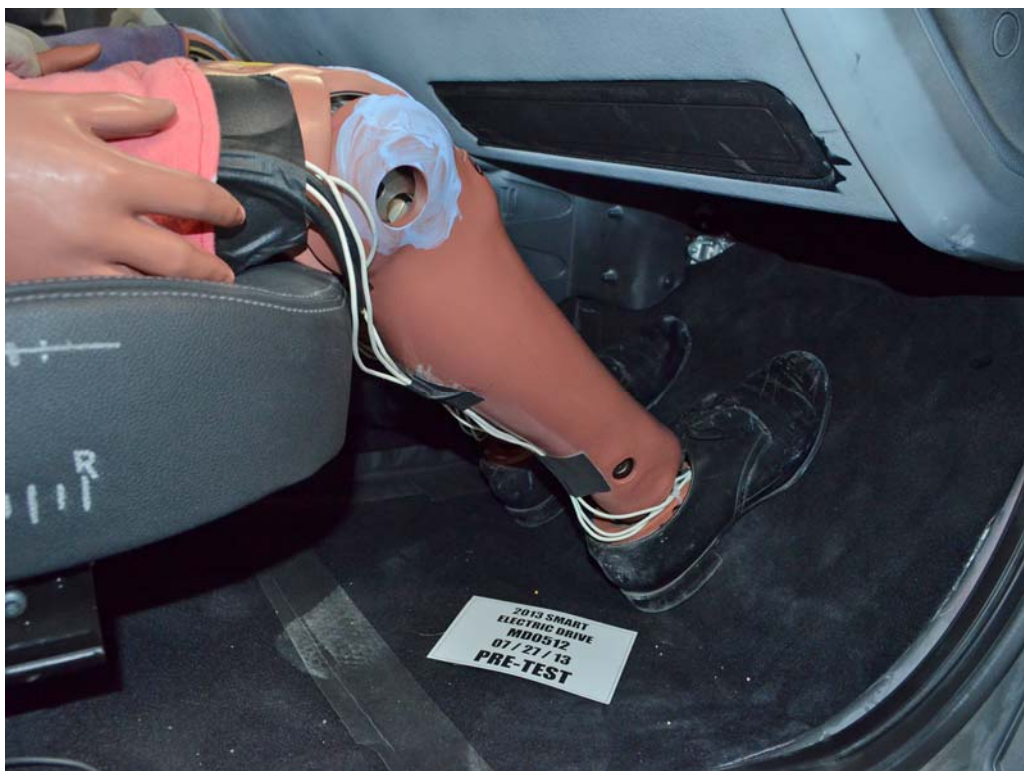
FIGURE 60. Pre-Test Passenger Dummy Feet
