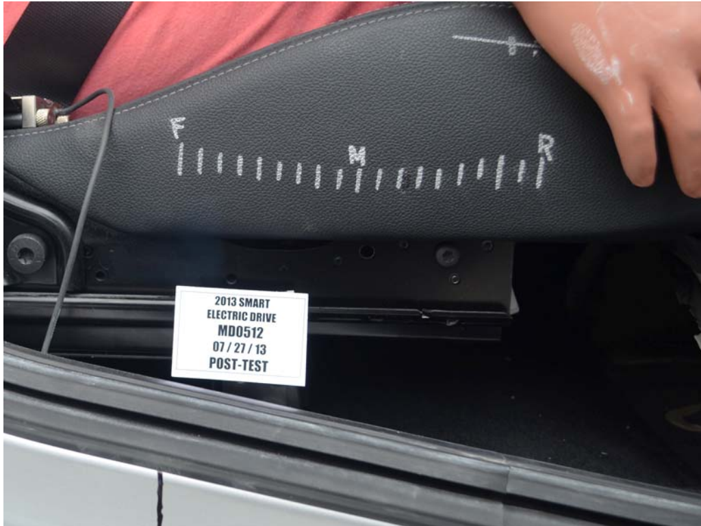
FIGURE 57. Post-Test Passenger's Seat Fore-Aft Markings
