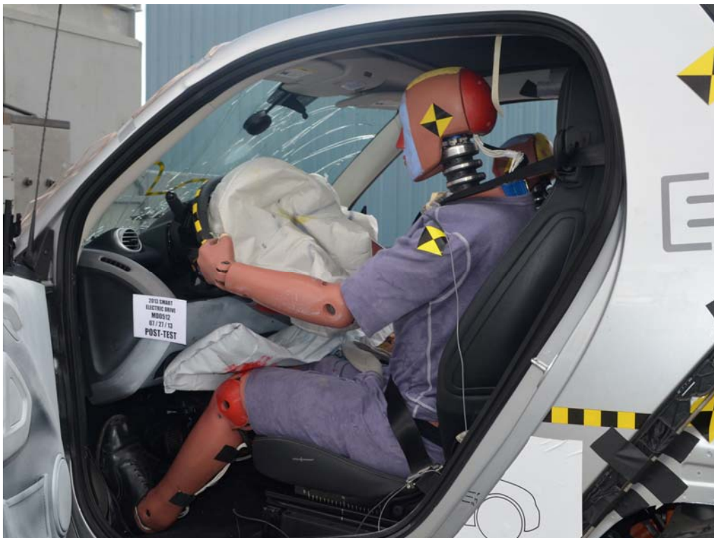
FIGURE 34. Post-Test Driver Dummy and Vehicle Interior View
