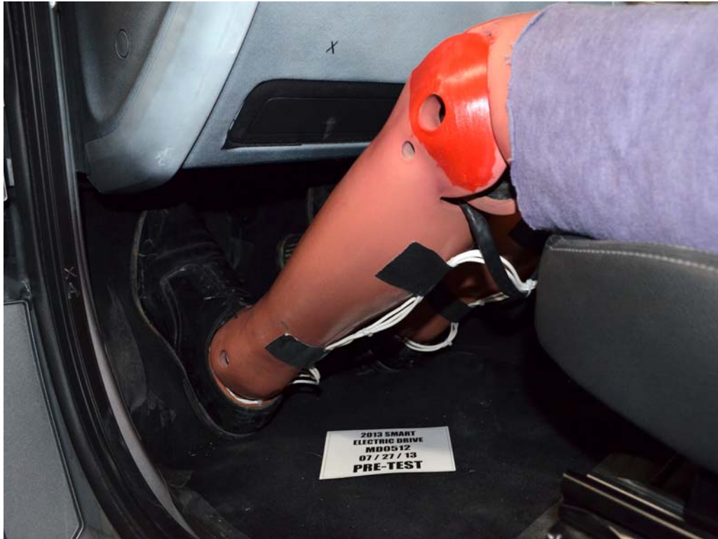
FIGURE 39. Pre-Test Driver Dummy Feet
