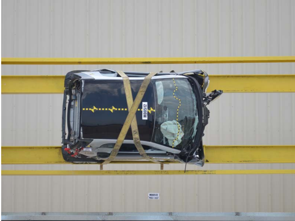
FIGURE 71. Vehicle at 90° on Static Rollover Device
