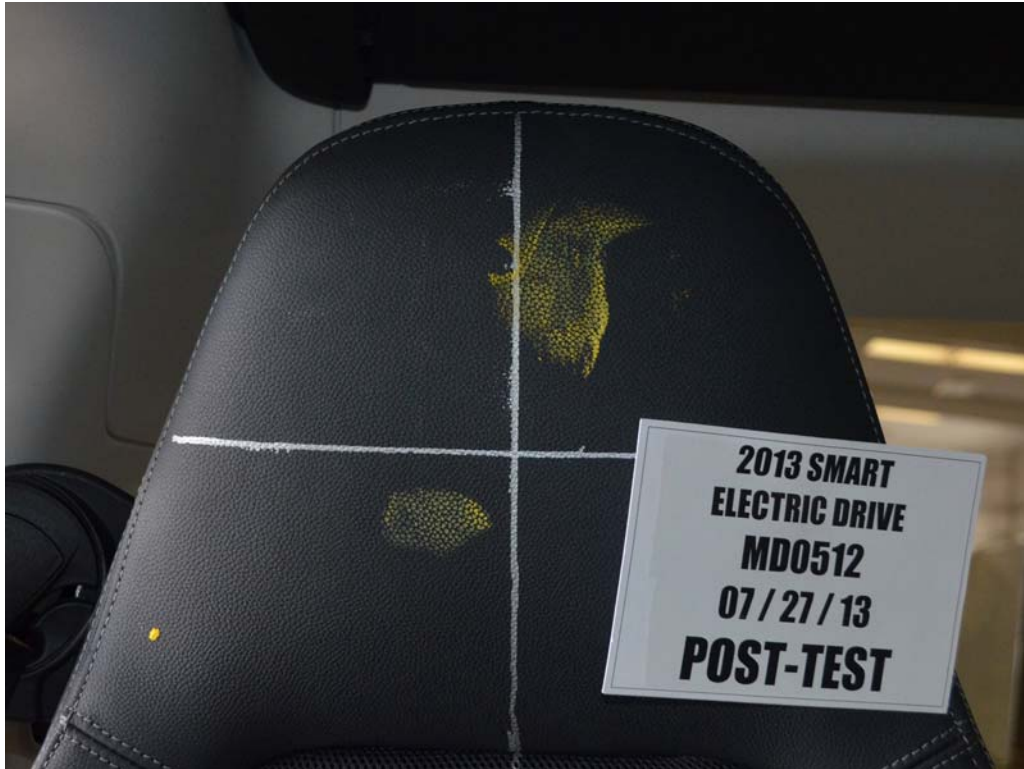
FIGURE 66a. Post-Test Passenger Dummy Contact with Headrest
