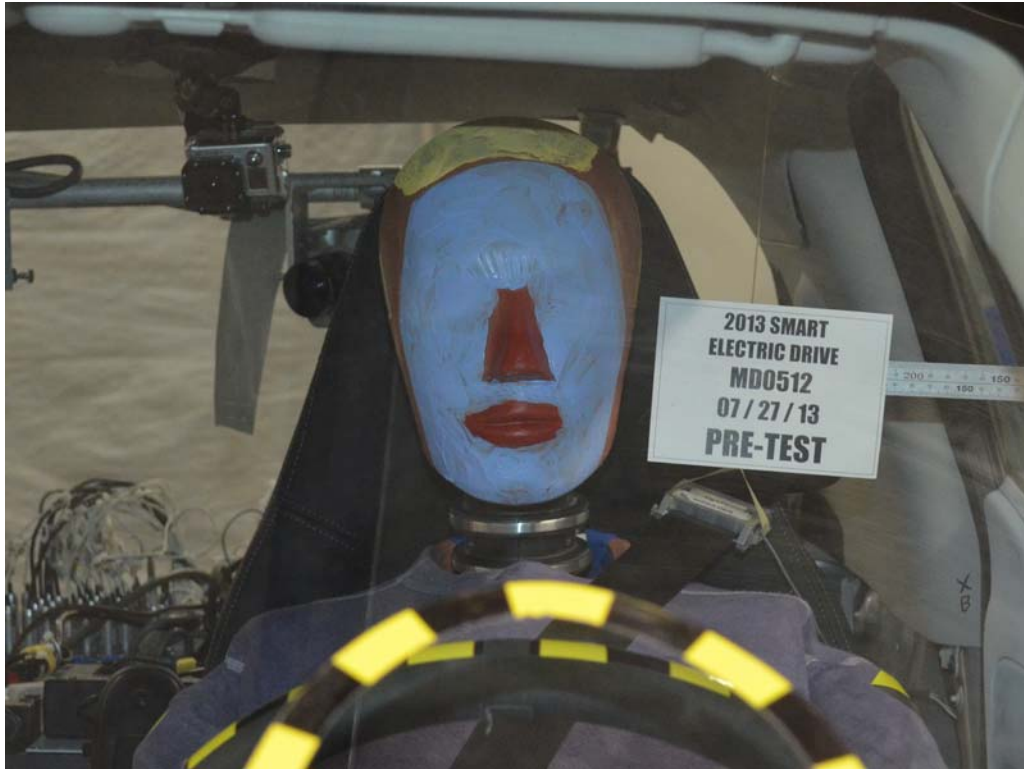
FIGURE 29. Pre-Test Driver Dummy Front View
