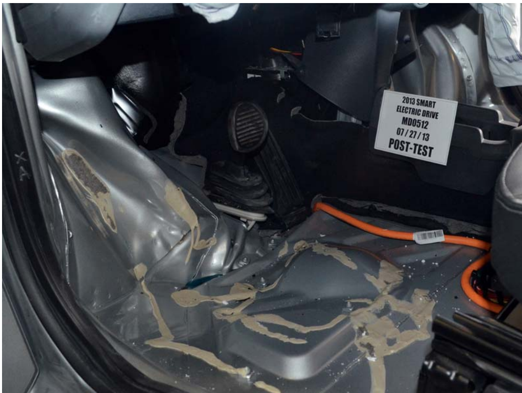
FIGURE 44. Post-Test Driver's Side Floorpan
