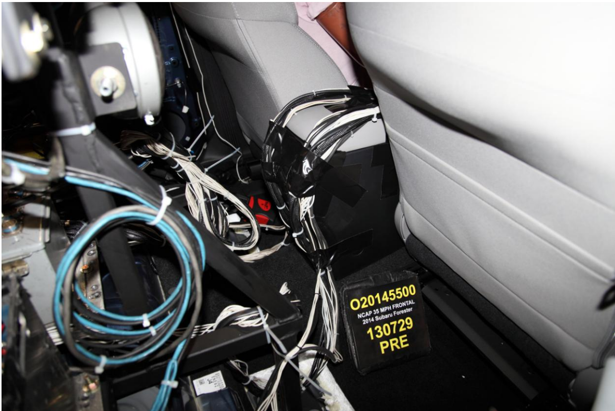
027 Pre-test Dummy Cable Routing
