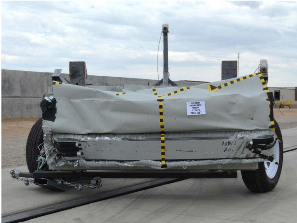
FIGURE 85. Post-Test Front View of MDB Impactor Face
