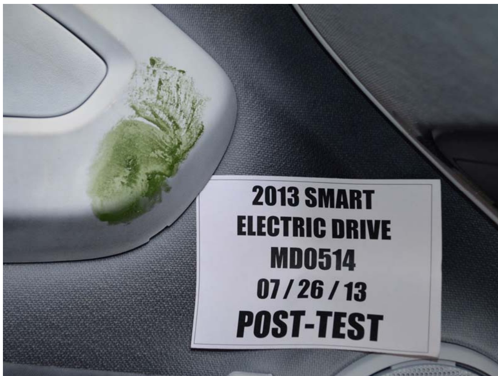
FIGURE 54. Post-Test Driver Dummy Close-Up Knee Contact View
