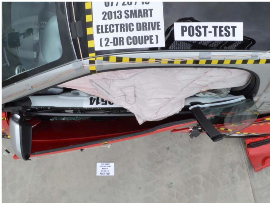
FIGURE 43. Post-Test Driver Dummy and Door Clearance View
