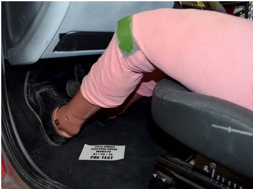
FIGURE 34. Pre-Test Placement of Driver Dummy's Feet
