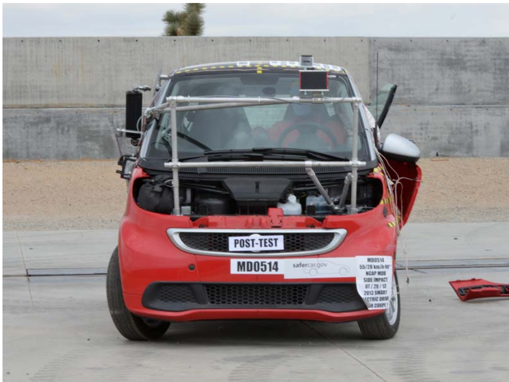
FIGURE 4. Post-Test Frontal View of Test Vehicle
