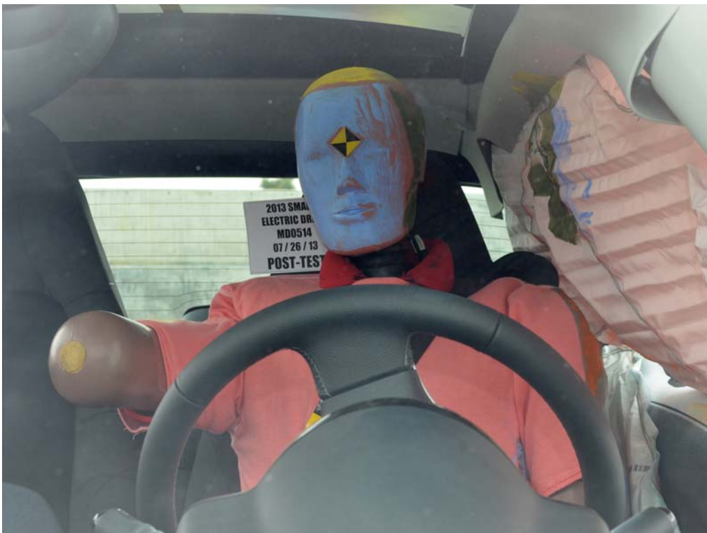
FIGURE 26. Post-Test Front Close-Up View of Driver Dummy
