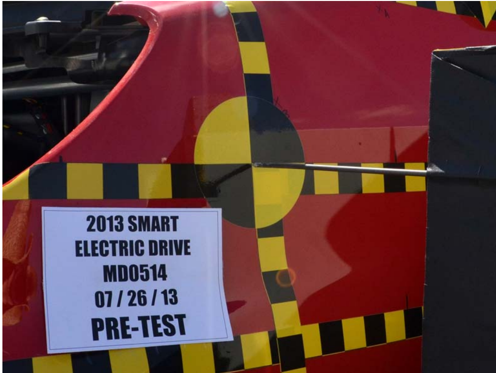
FIGURE 19. Pre-Test Close-Up View of Impact Point Target
