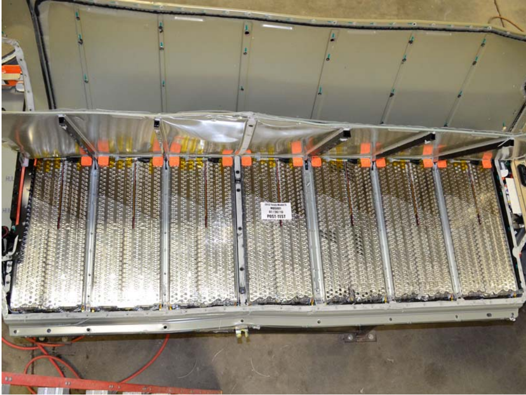
FIGURE 15. Post-Impact View of Propulsion Battery Module(s)
