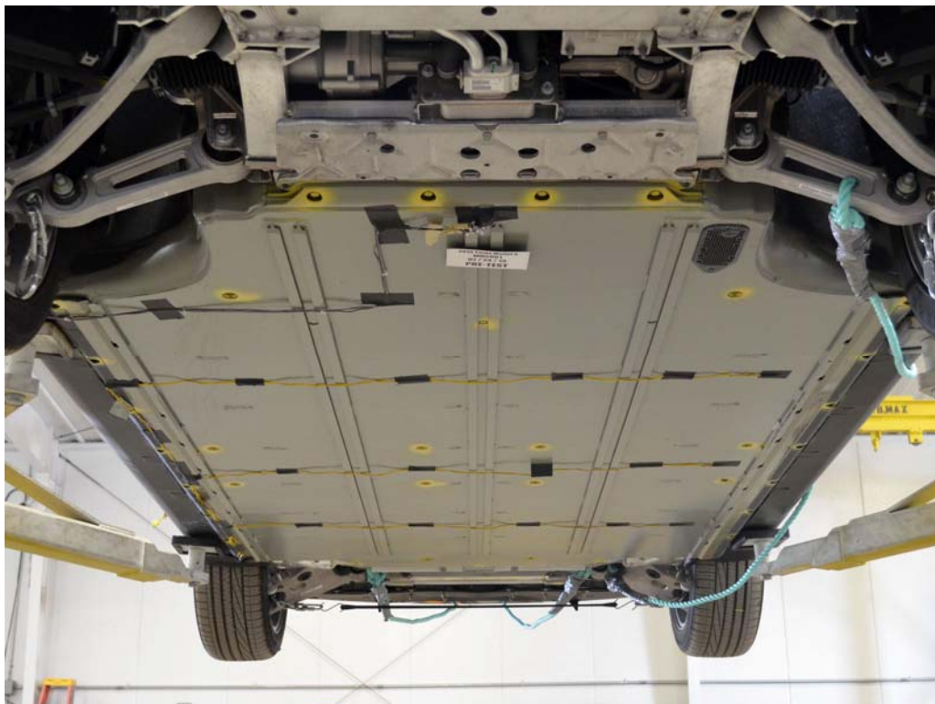
FIGURE 9a. Pre-Impact View of Propulsion Battery
