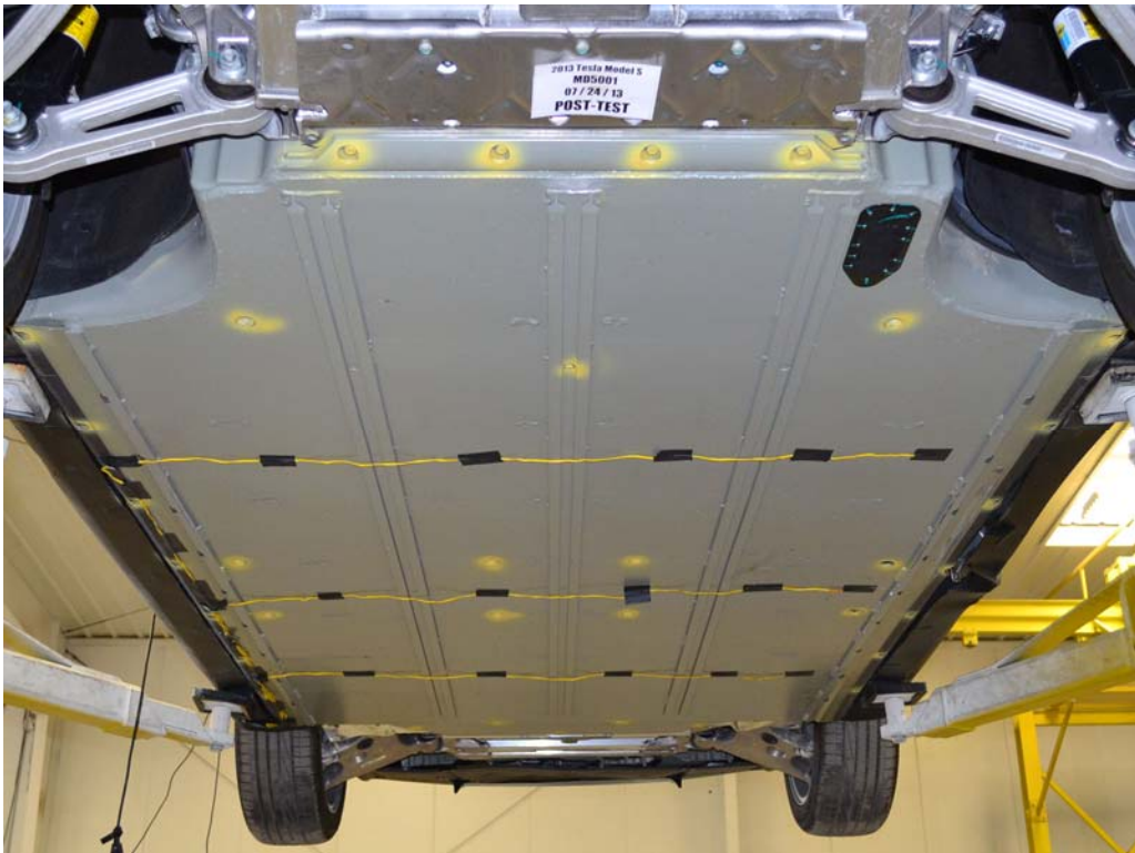
FIGURE 10. Post-Impact Front View of Propulsion Battery
