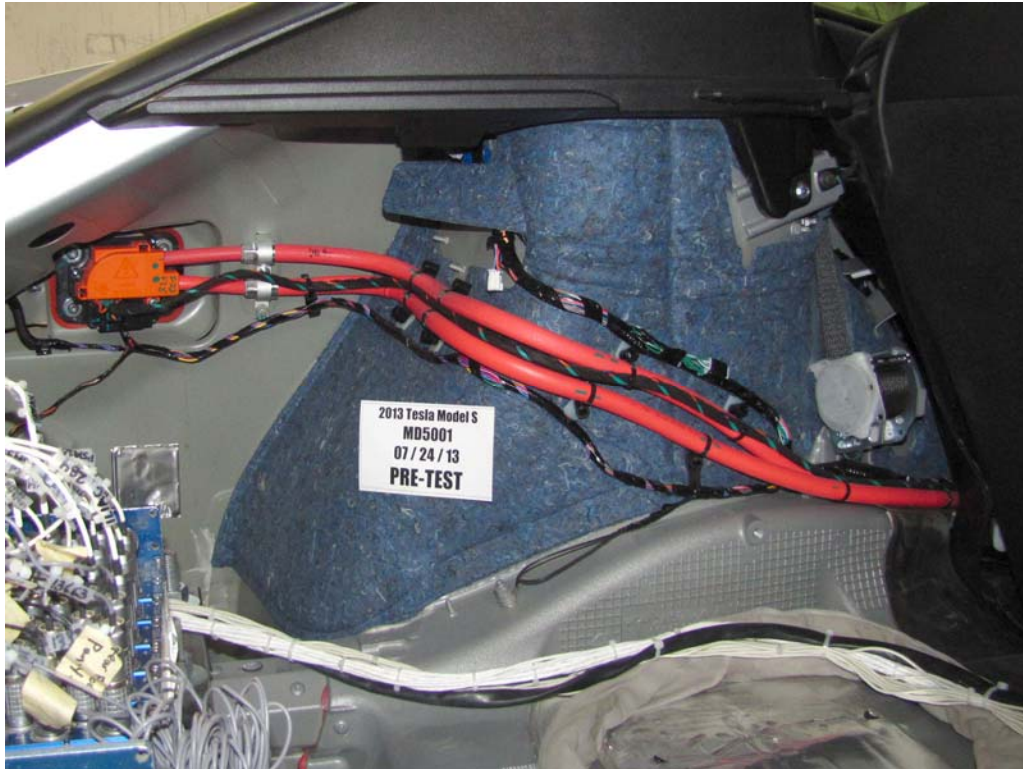
FIGURE 18h. Pre-Impact View of High Voltage Interconnect(s)
