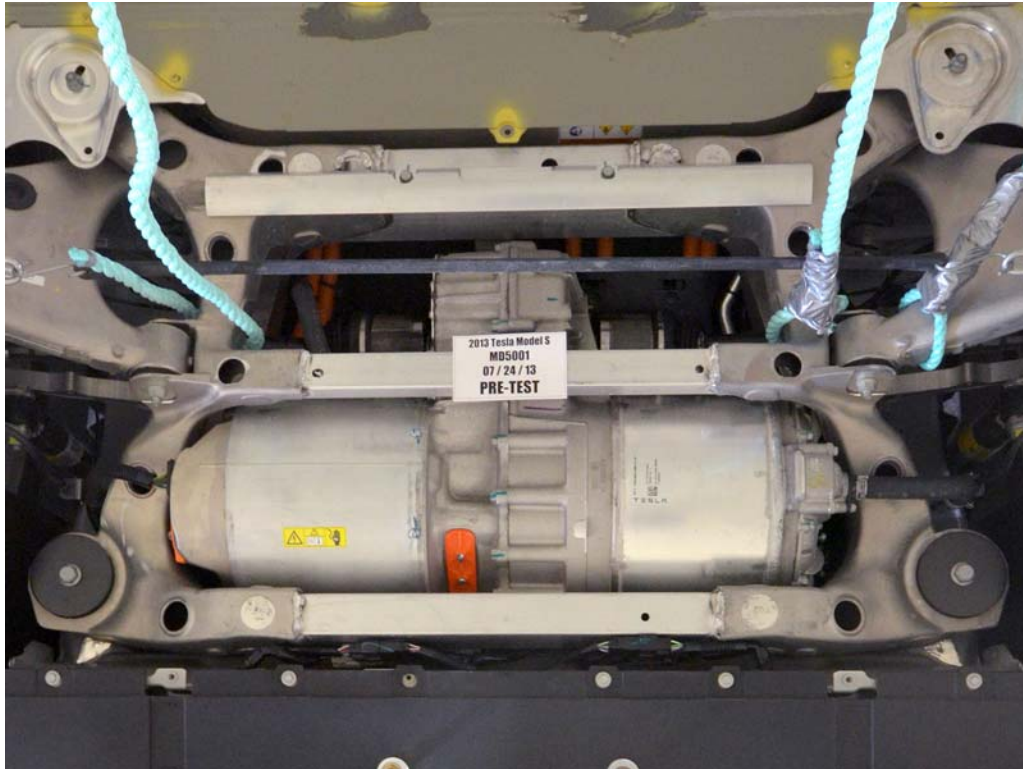
FIGURE 16. Pre-Impact View of Electric Propulsion Drive
