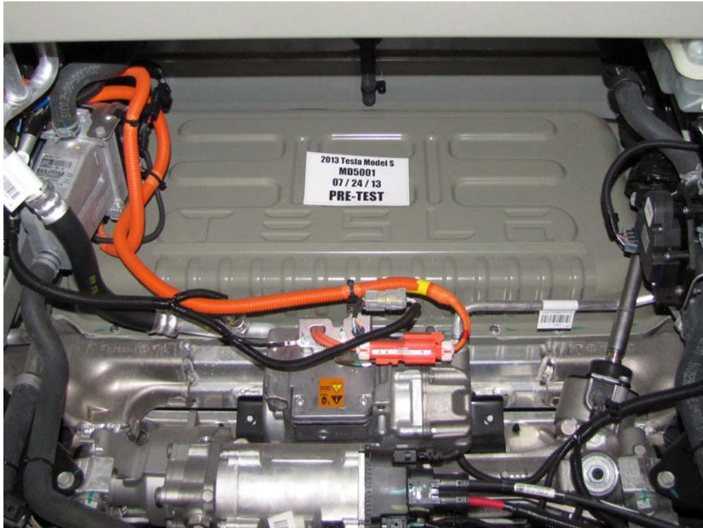
FIGURE 9. Pre-Impact View of Propulsion Battery
