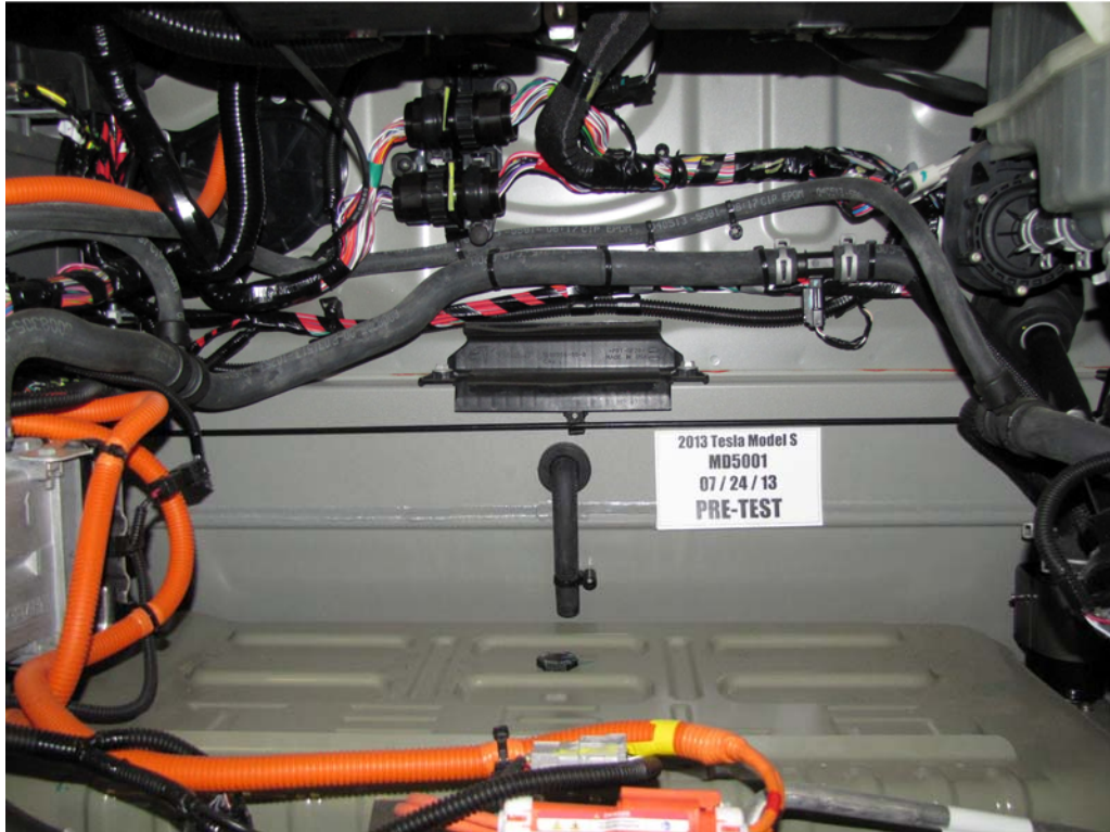
FIGURE19c. Pre-Impact View of Propulsion Battery Venting System(s)
