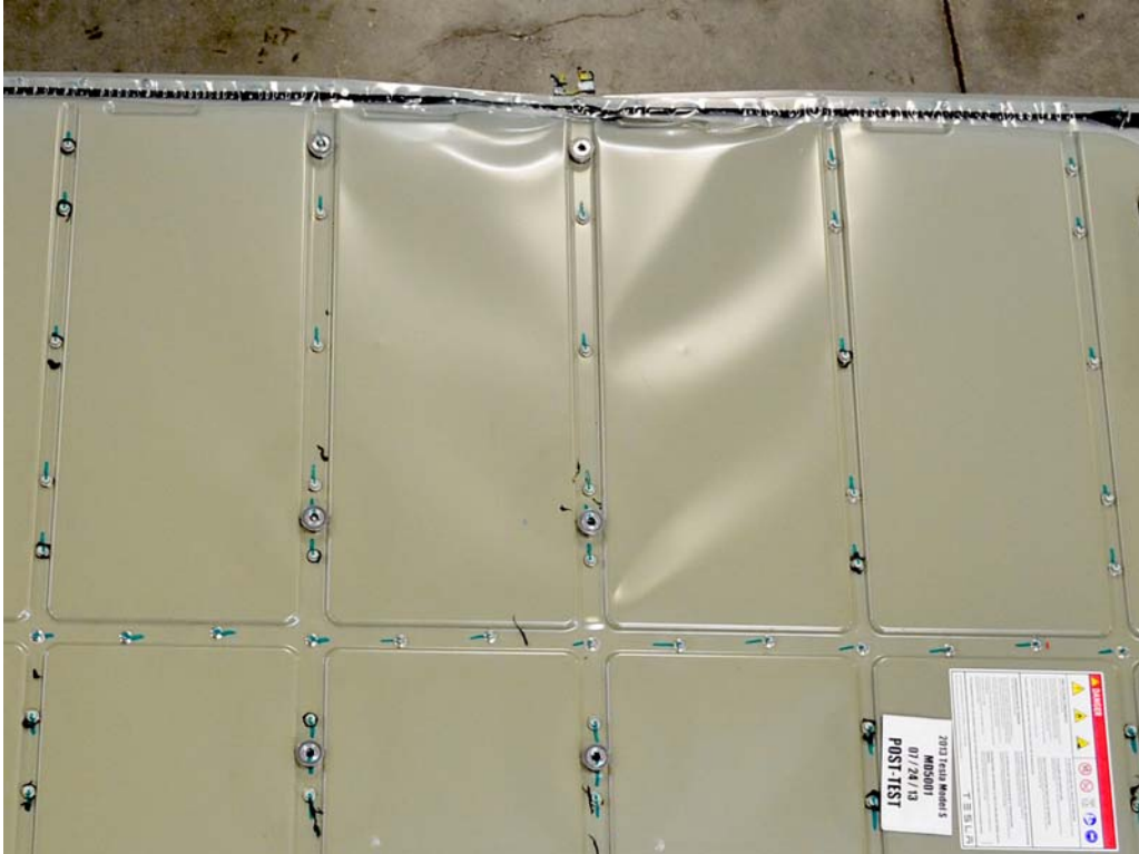
FIGURE 36. Post-Impact View of Propulsion Battery Component Intrusion
