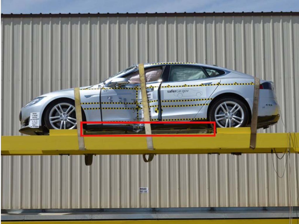
FIGURE 28. FMVSS No. 305 Static Rollover at 0°
