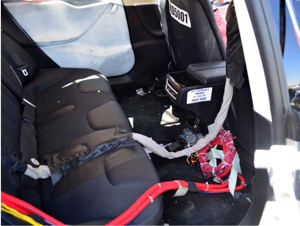
FIGURE 34. Post-Impact View of the Vehicle Passenger Compartment Adjacent to Propulsion Battery
