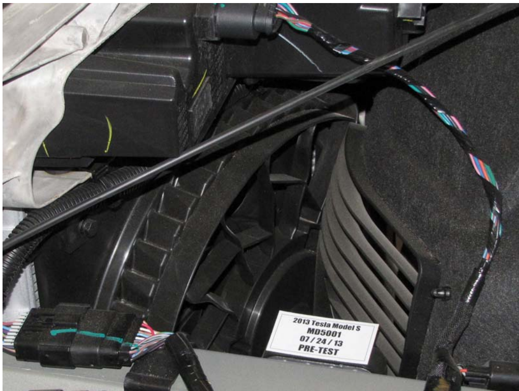
FIGURE 19. Pre-Impact View of Propulsion Battery Venting System(s)
