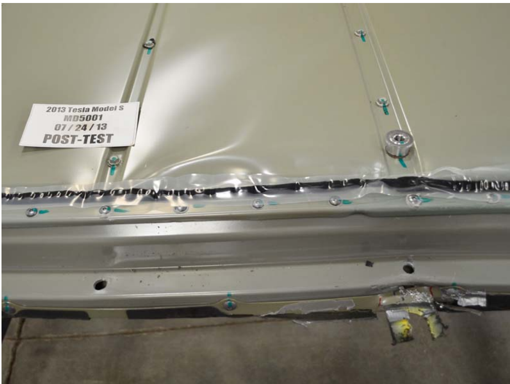
FIGURE 36a. Post-Impact View of Propulsion Battery Component Intrusion
