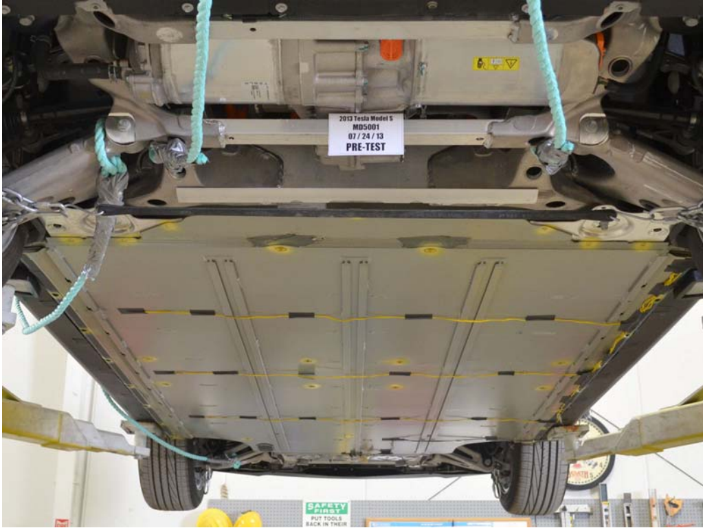
FIGURE 9b. Pre-Impact View of Propulsion Battery
