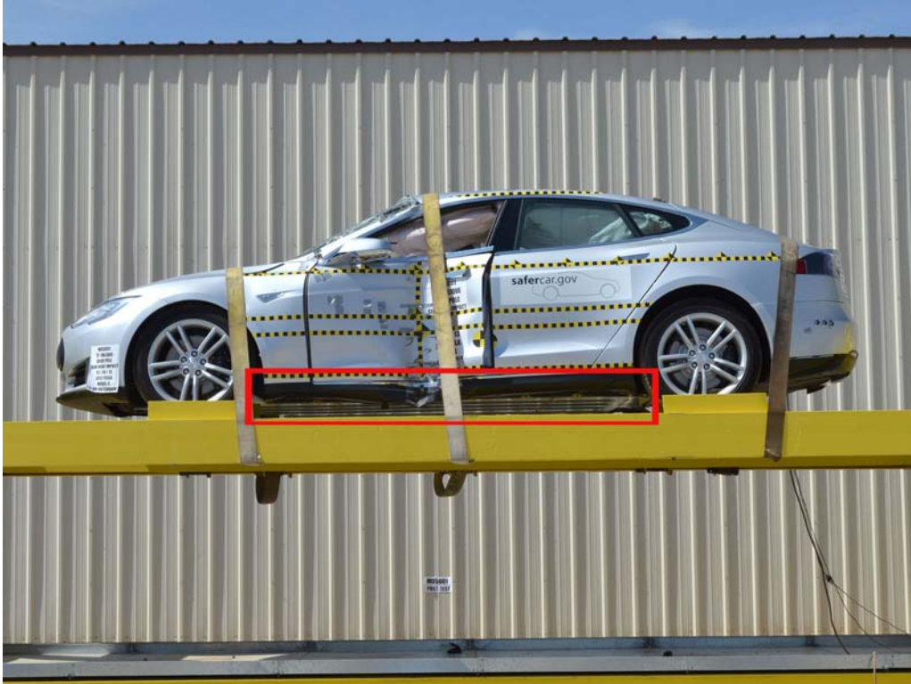
FIGURE 32. FMVSS No. 305 Static Rollover at 360°
