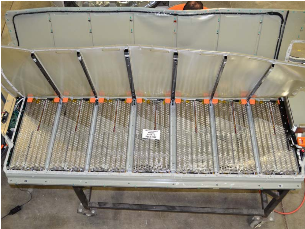
FIGURE 15a. Post-Impact View of Propulsion Battery Module(s)
