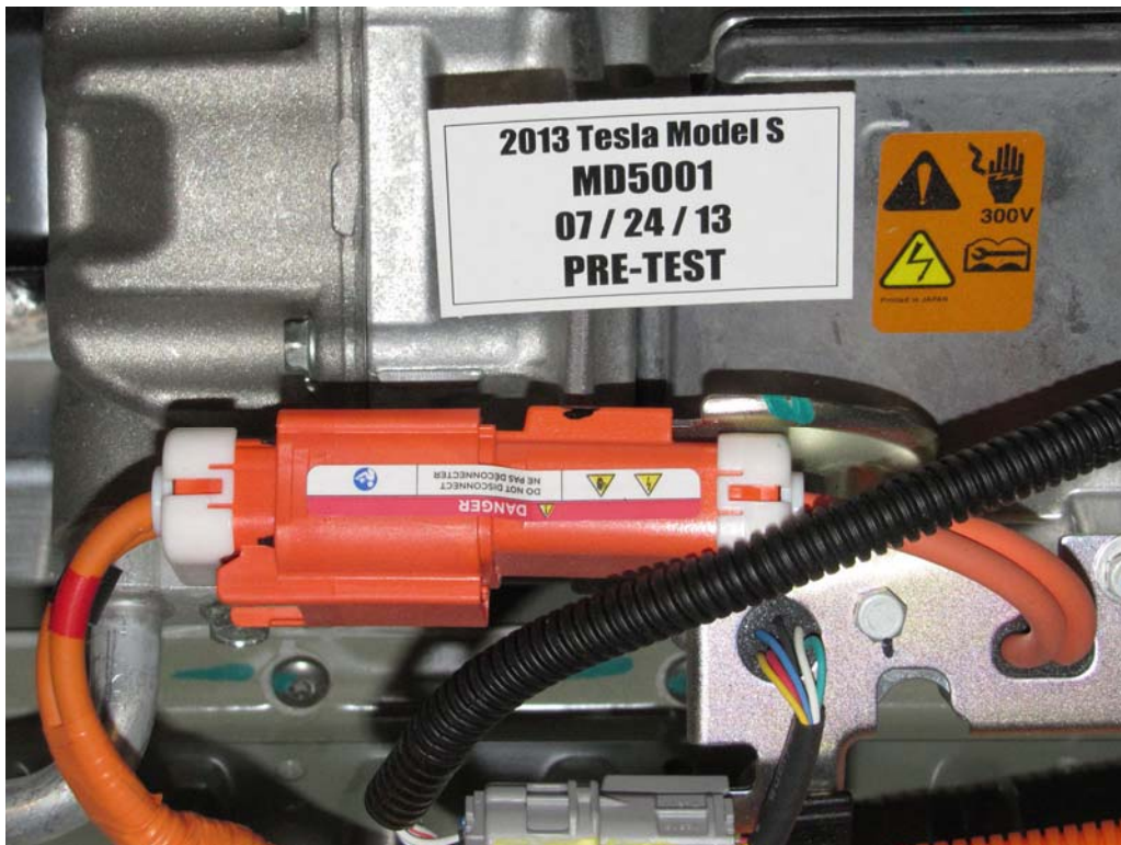
FIGURE 18a. Pre-Impact View of High Voltage Interconnect(s)
