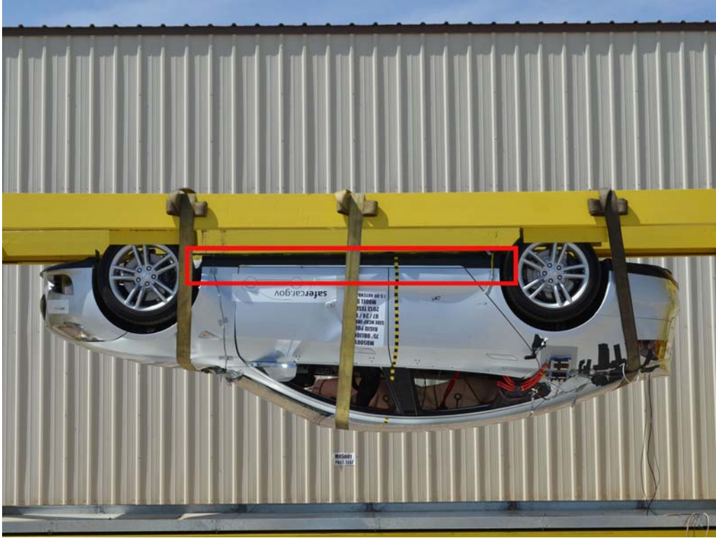
FIGURE 30. FMVSS No. 305 Static Rollover at 180°
