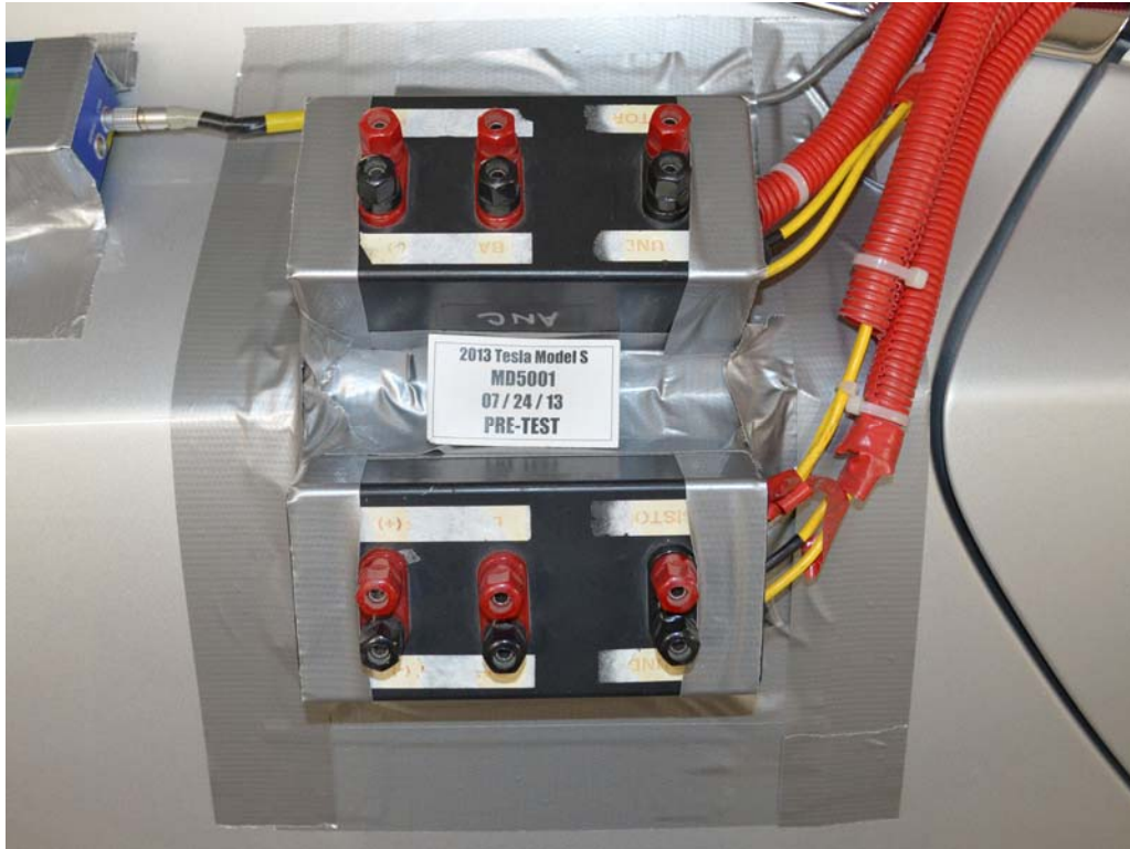
FIGURE 24. Pre-Impact View of Installed Test Interface Port
