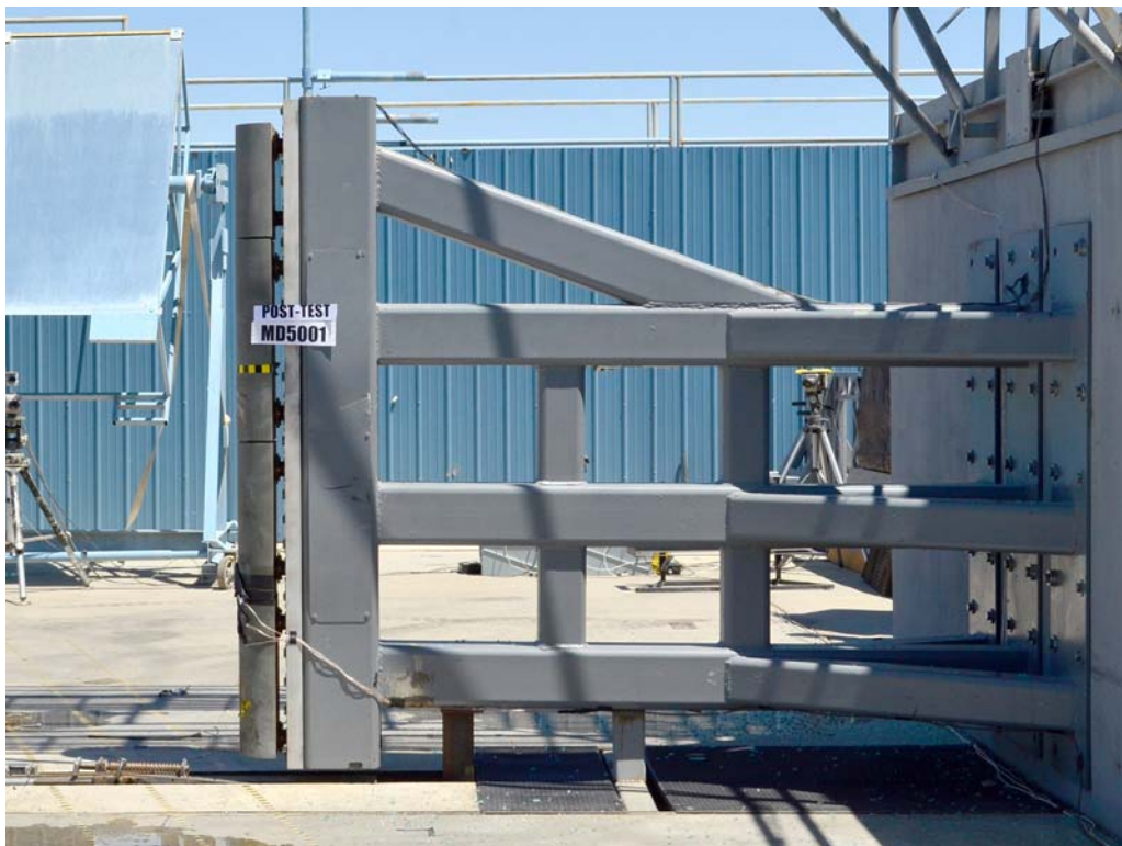
FIGURE 60. Post-Test Pole Barrier Side View
