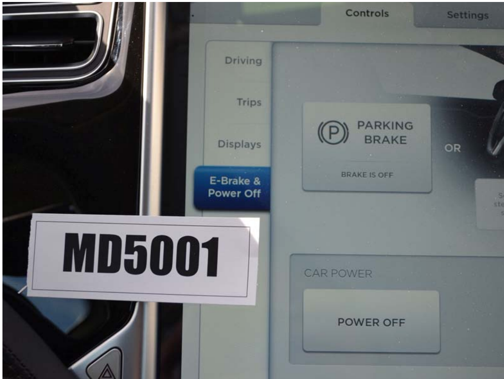
FIGURE 35. Pre-Test View of Disengaged Parking Brake
