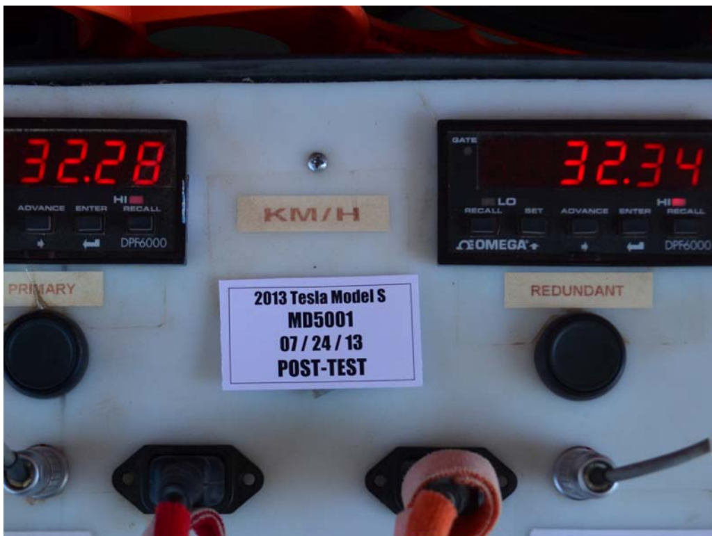
FIGURE 62. Post-Test Primary and Redundant Speed Trap Read-Out
