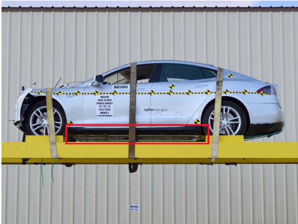
FIGURE 28. FMVSS No. 305 Static Rollover at 0°
