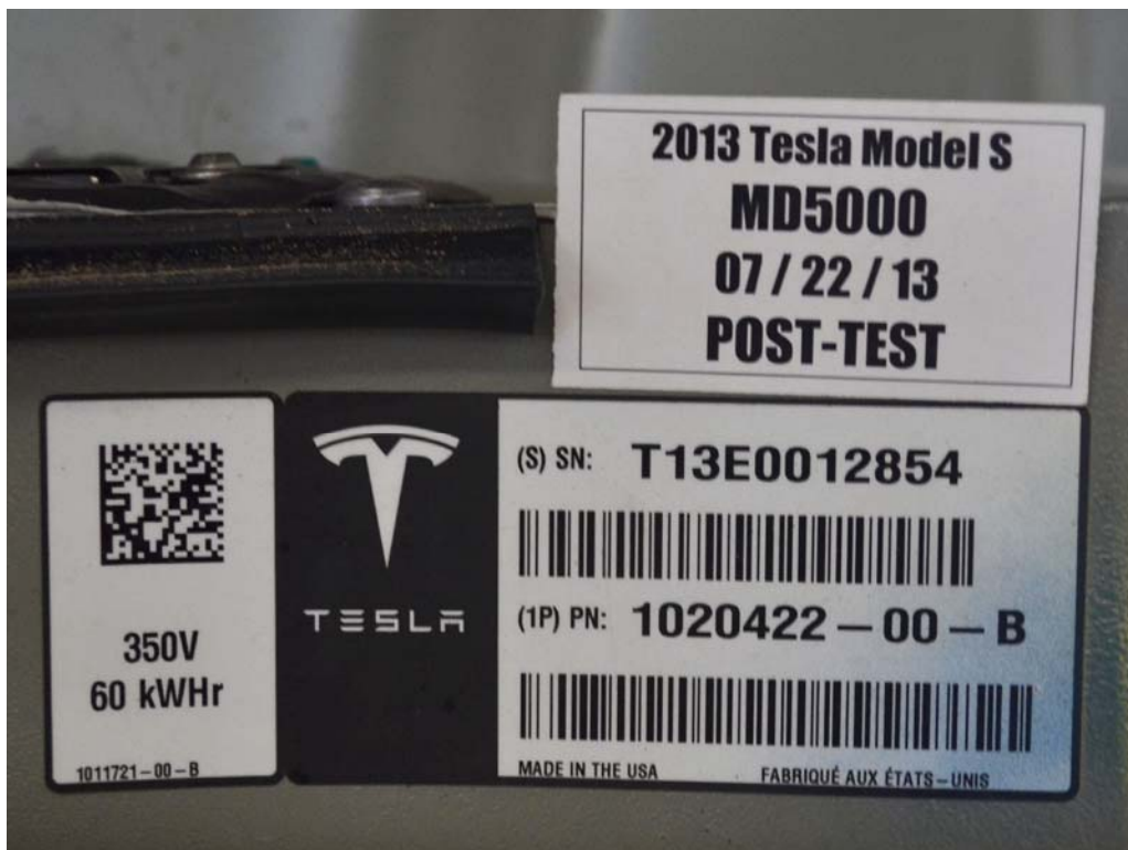
FIGURE 5e. Other Vehicle Label(s) Related to Electrical Propulsion System
