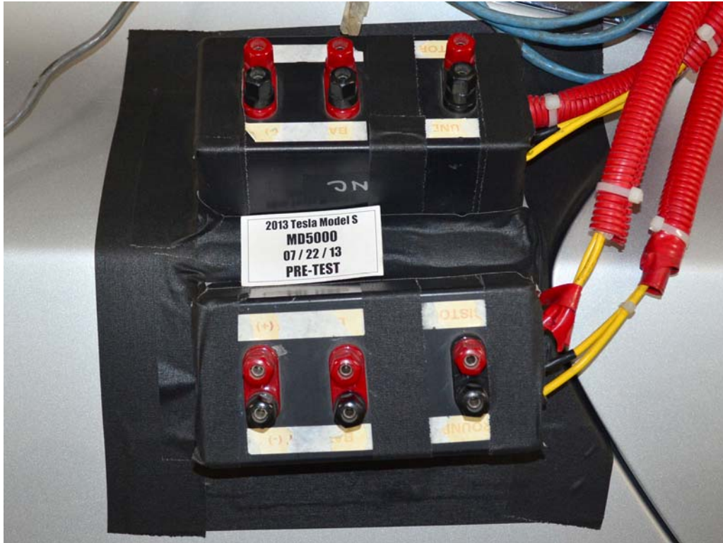
FIGURE 24. Pre-Impact View of Installed Test Interface Port
