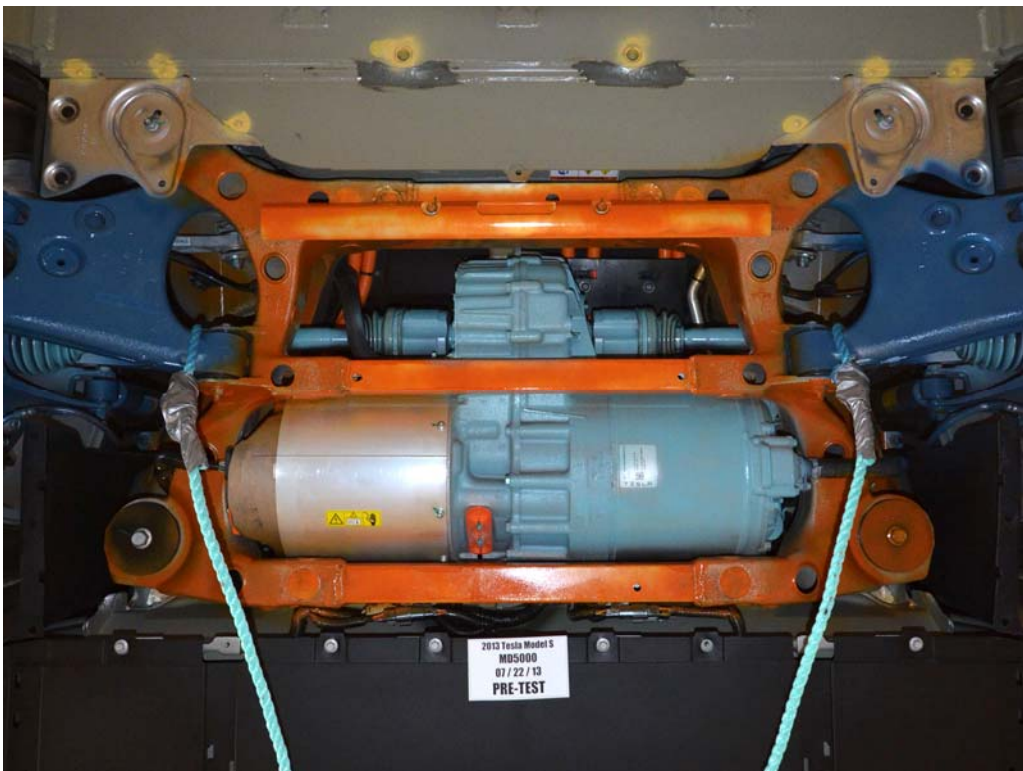
FIGURE 16. Pre-Impact View of Electric Propulsion Drive
