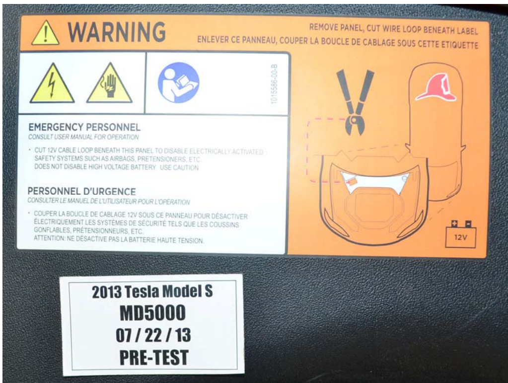
FIGURE 3. First Responder Warning Label
