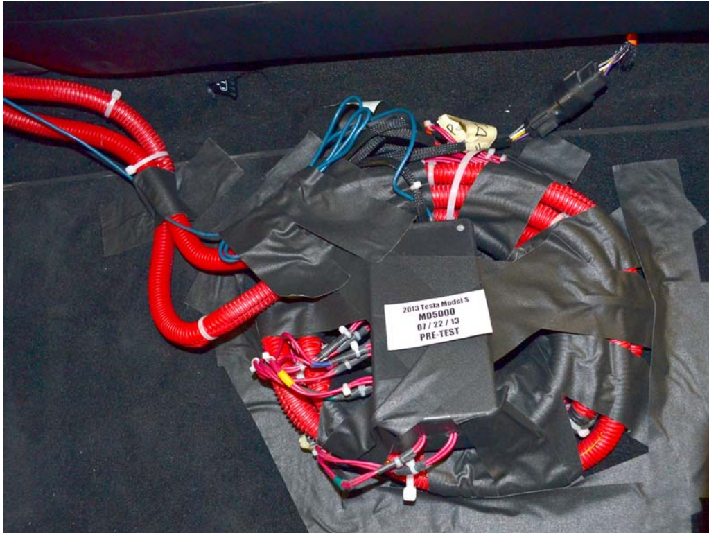
FIGURE 22. Pre-Impact View of High Voltage Leads Attached
