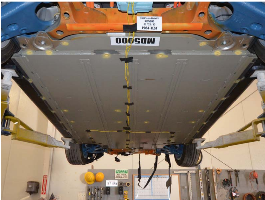
FIGURE 11. Post-Impact Rear View of Propulsion Battery
