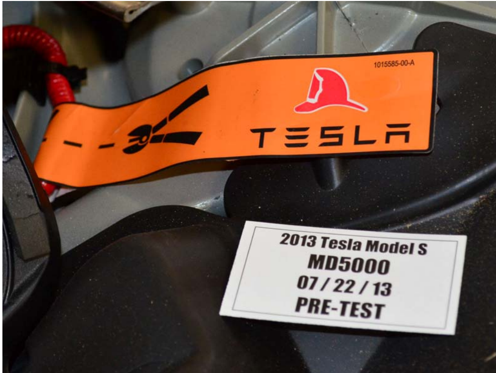
FIGURE 3a. First Responder Warning Label
