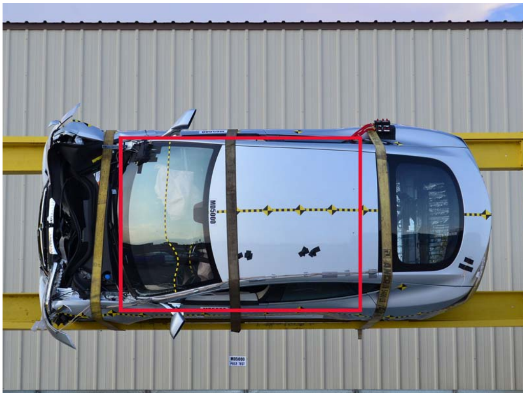
FIGURE 29. FMVSS No. 305 Static Rollover at 90°
