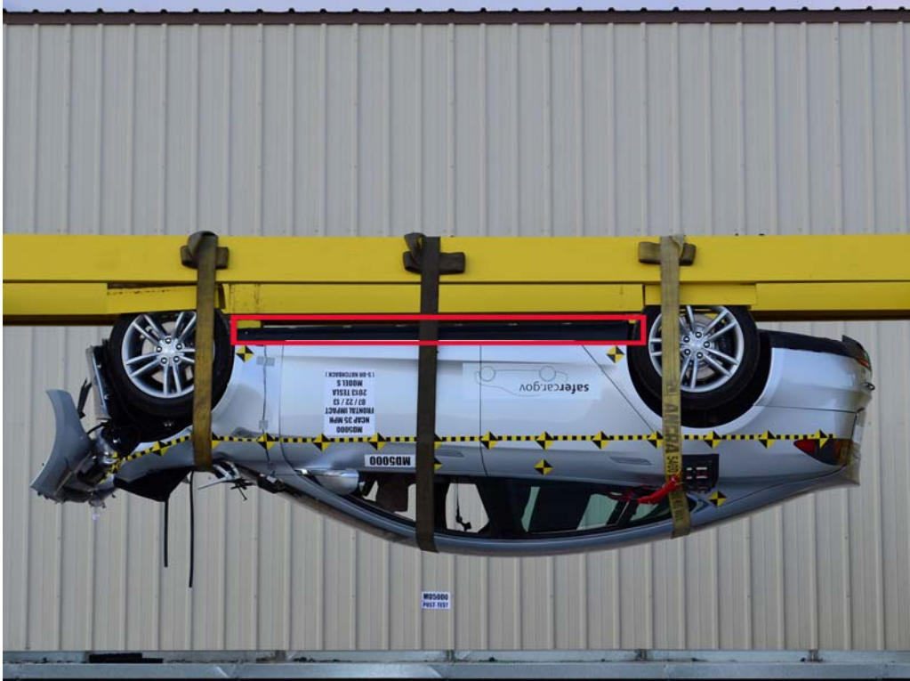
FIGURE 30. FMVSS No. 305 Static Rollover at 180°
