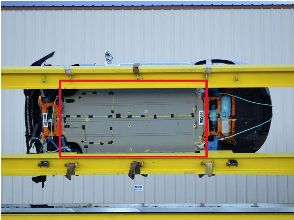
FIGURE 31. FMVSS No. 305 Static Rollover at 270°
