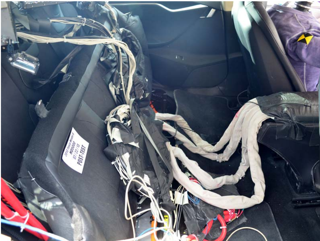
FIGURE 28. Post-Test Dummy Cable Routing
