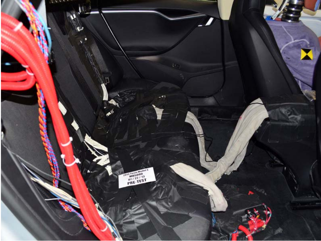
FIGURE 27. Pre-Test Dummy Cable Routing
