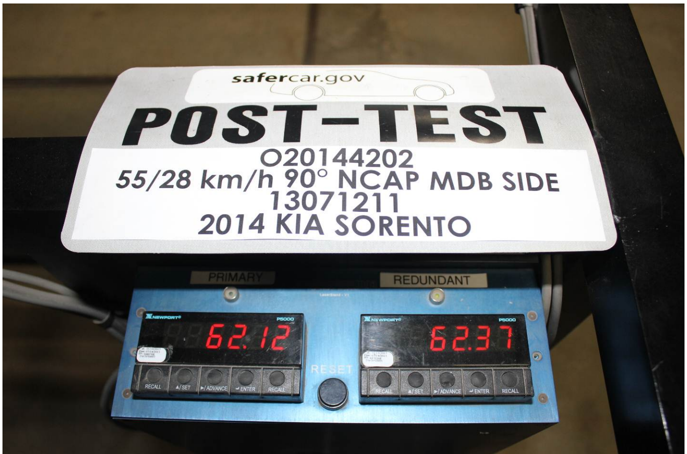
Post-Test Primary and Redundant Speed Trap Read-Out
