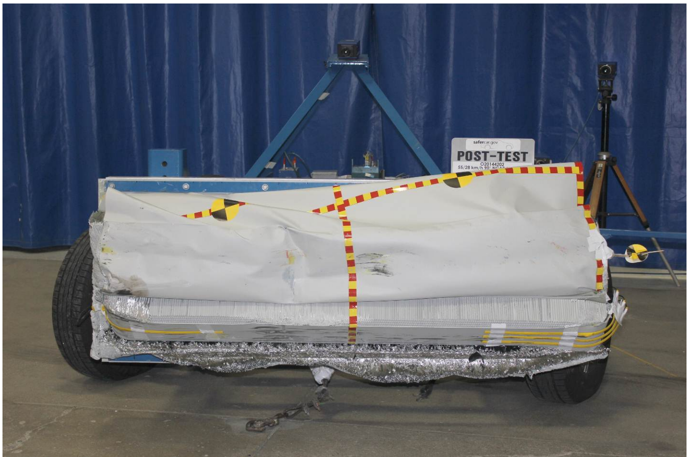
Post-Test Front View of MDB Impactor Face
