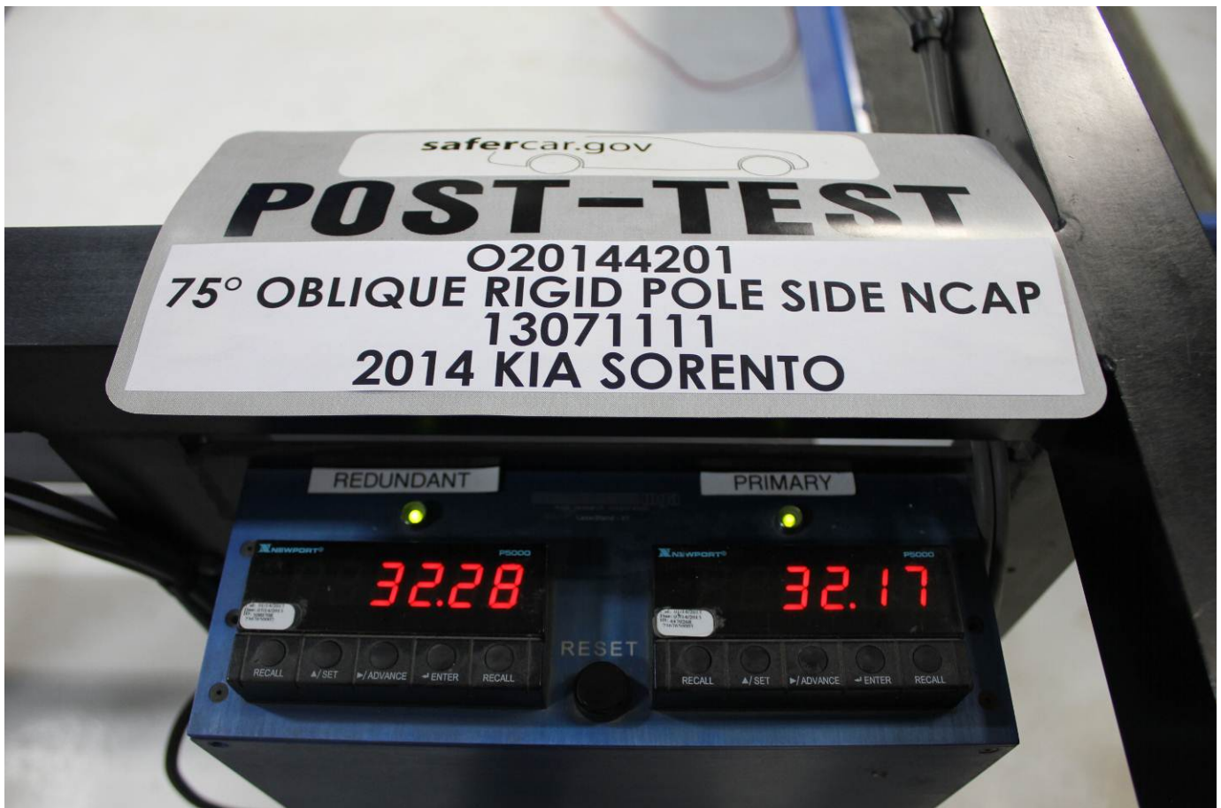
Post-Test Primary and Redundant Speed Trap Read-Out
