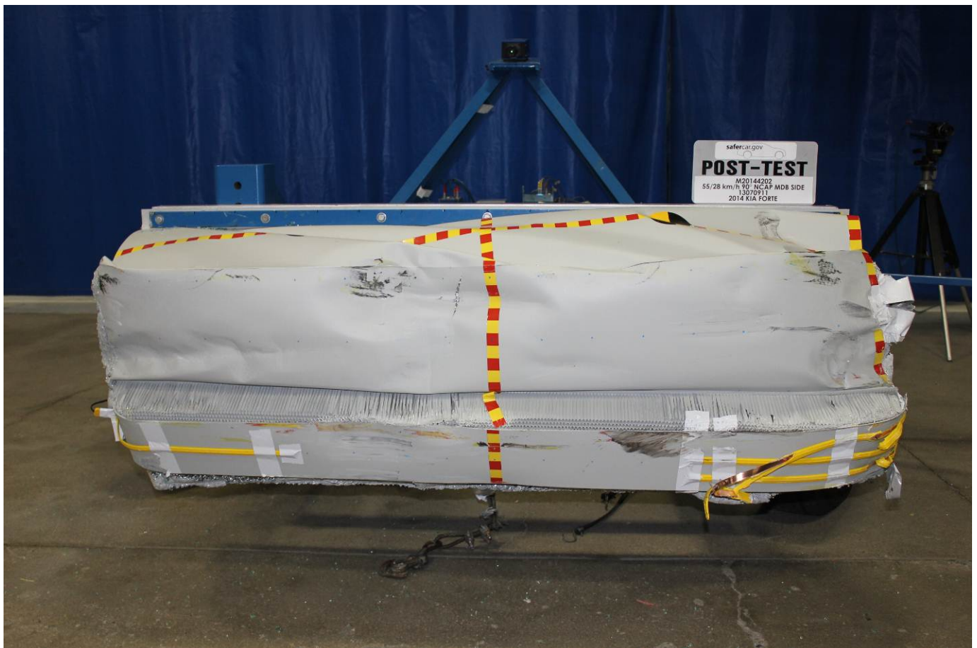
Post-Test Front View of MDB Impactor Face
