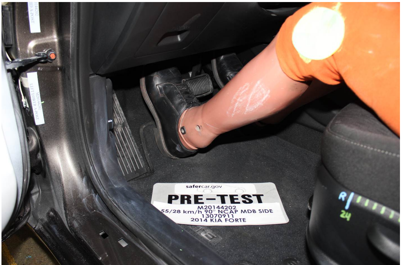
Pre-Test Placement of Driver Dummy's Feet
