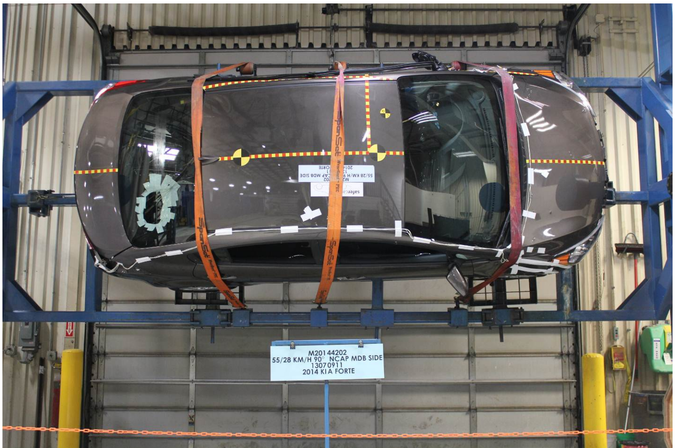
FMVSS No. 301 Static Rollover 270 Degrees
