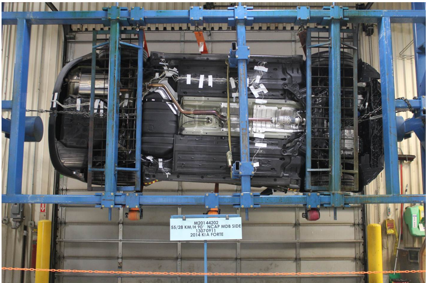
FMVSS No. 301 Static Rollover 90 Degrees
