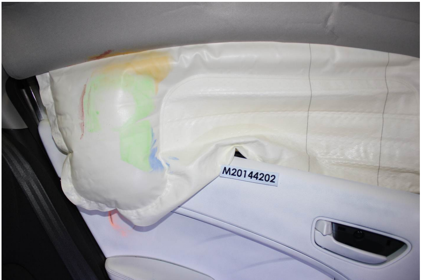
Post-Test Rear Passenger Dummy Close-up Head Contact with Side Airbag View
