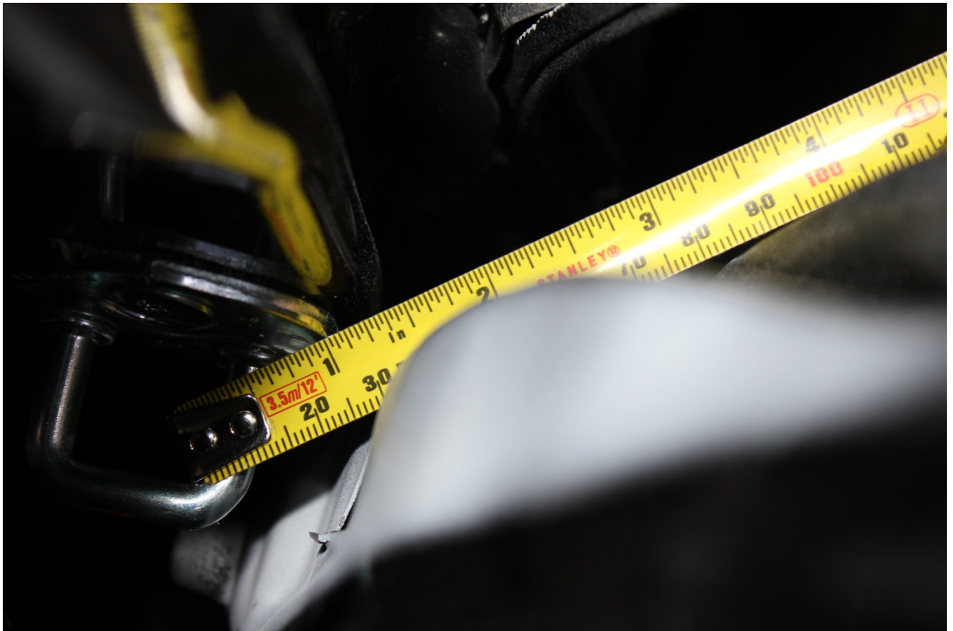
Post-Test Left Front Door Gap
