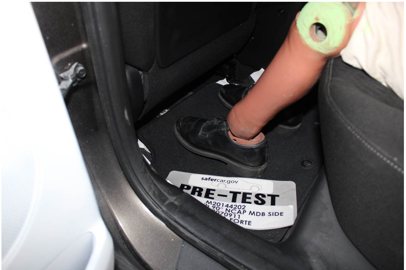
Pre-Test Placement of Rear Passenger Dummy's Feet
