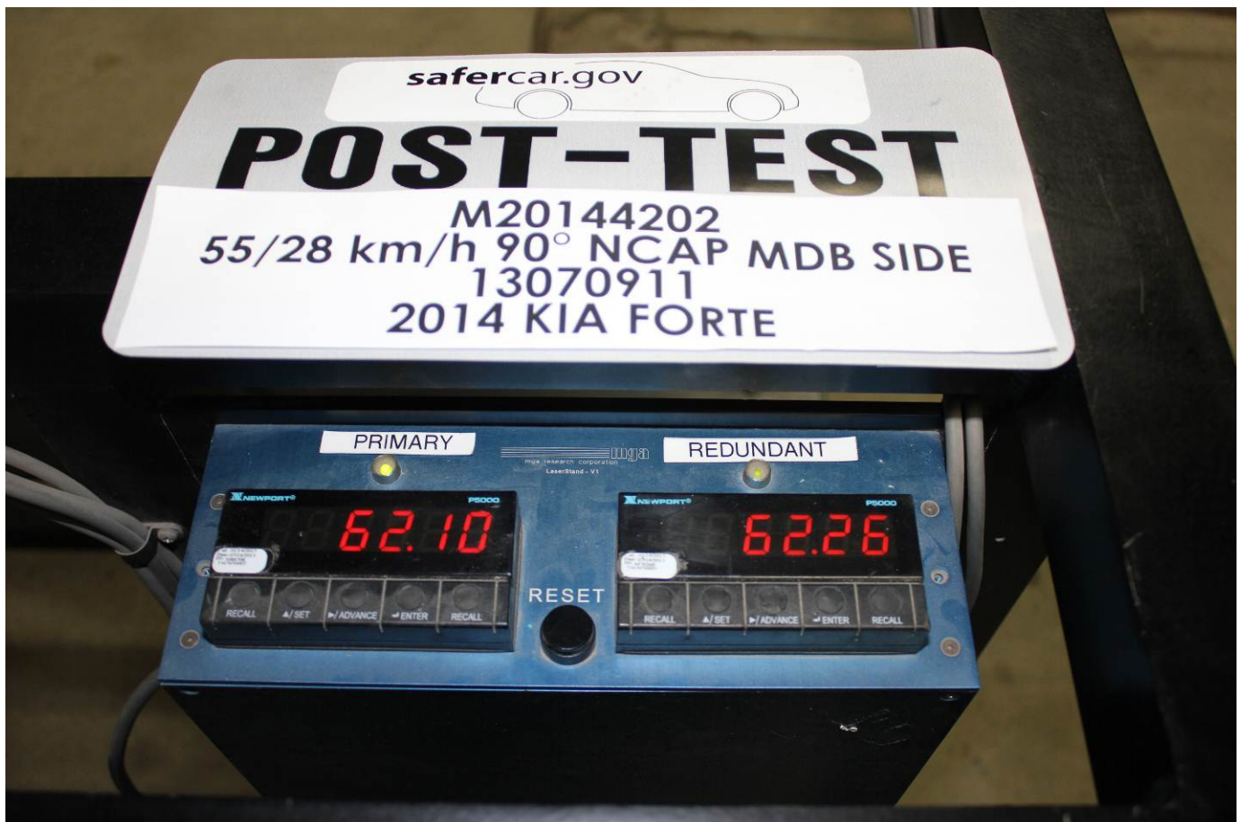
Post-Test Primary and Redundant Speed Trap Read-Out
