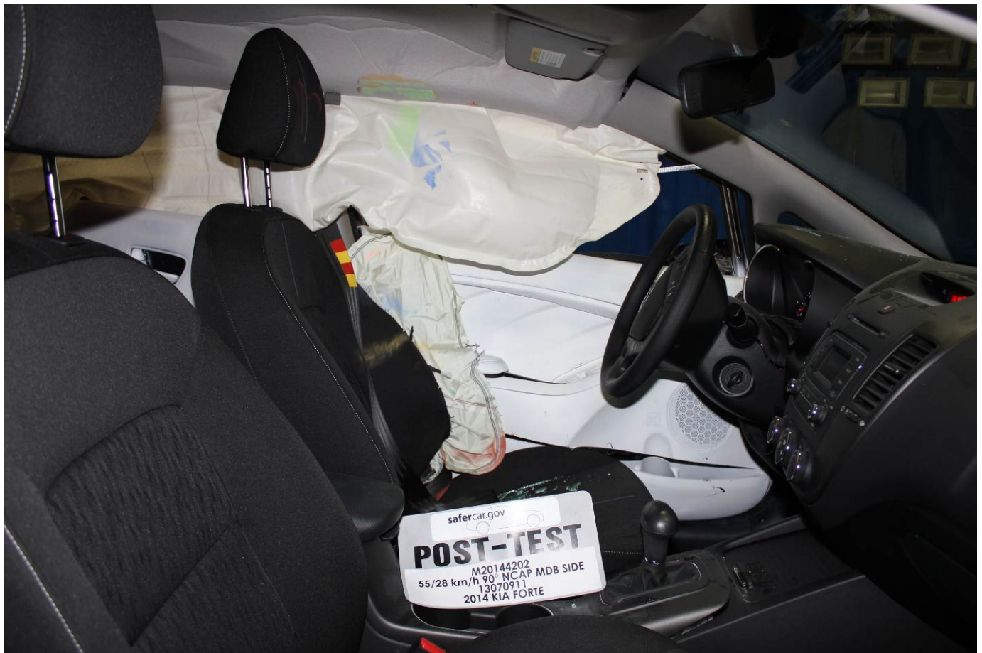
Post-Test Driver Inner Door Panel View
