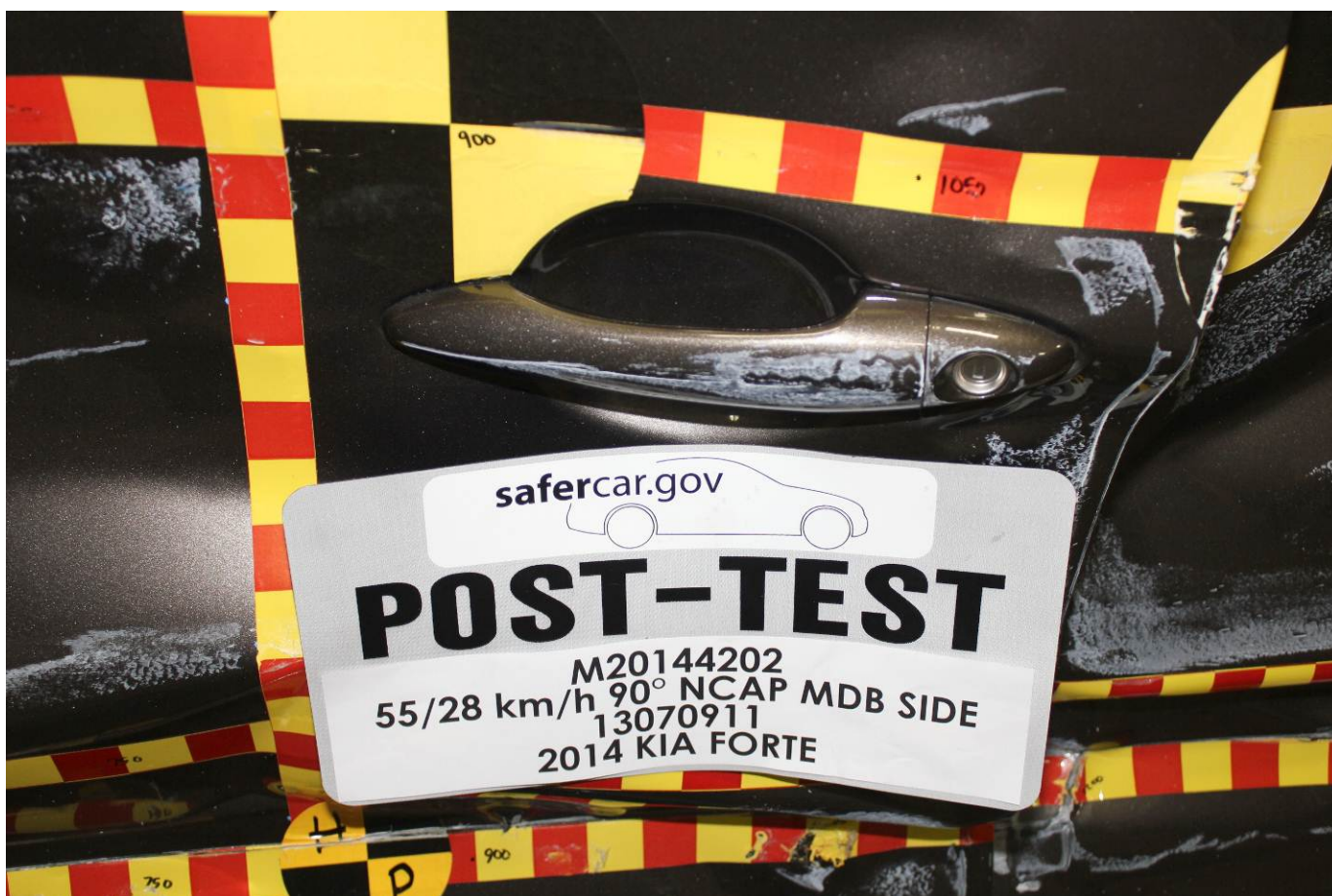
Post-Test Left Front Door Latch Close-Up
