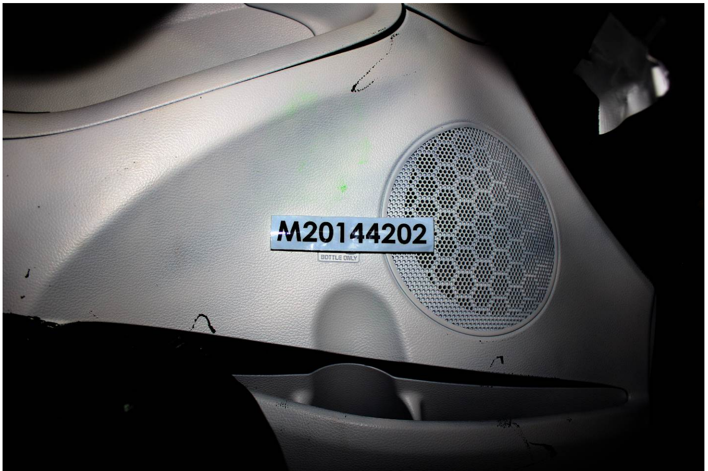
Post-Test Driver Dummy Close-up Knee Contact View
