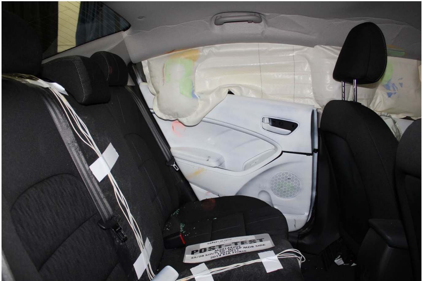
Post-Test Rear Passenger Inner Door Panel View
