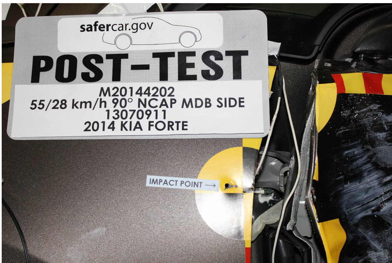
Post-Test Close-Up View of Impact Point Target
