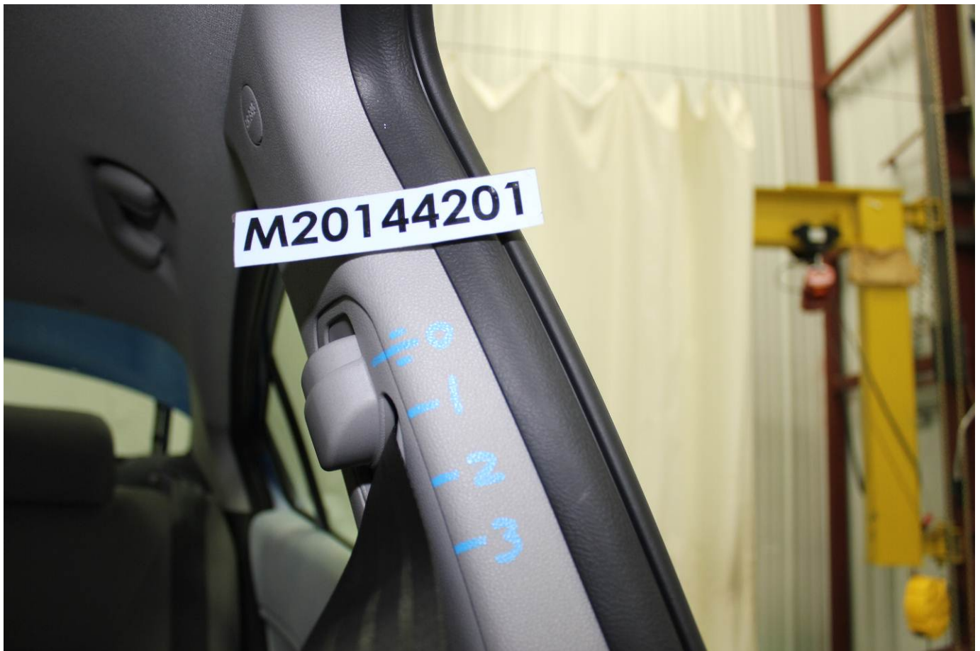
Pre-Test View of Belt Anchorage for Dummy
