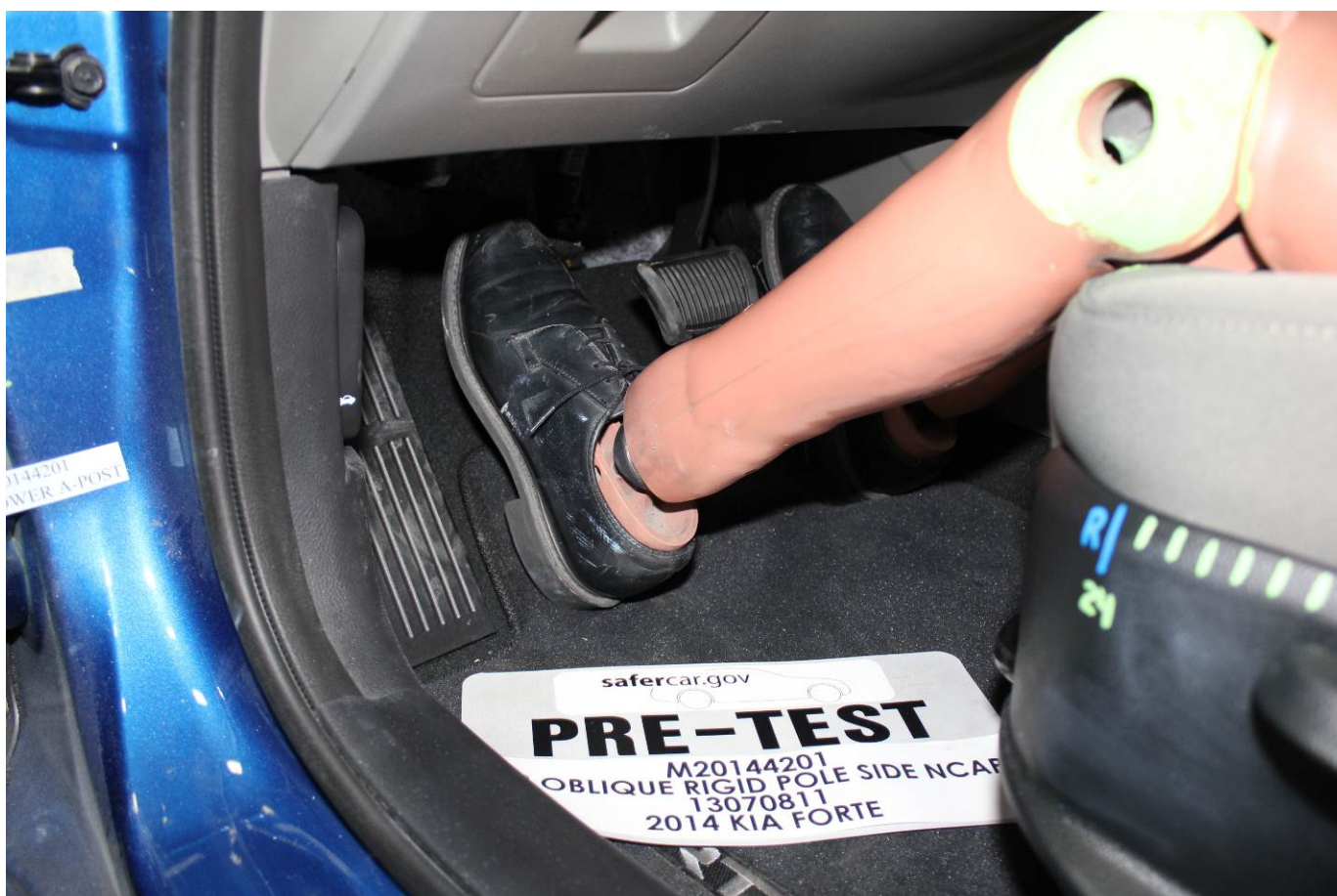
Pre-Test Placement of Dummy's Feet
