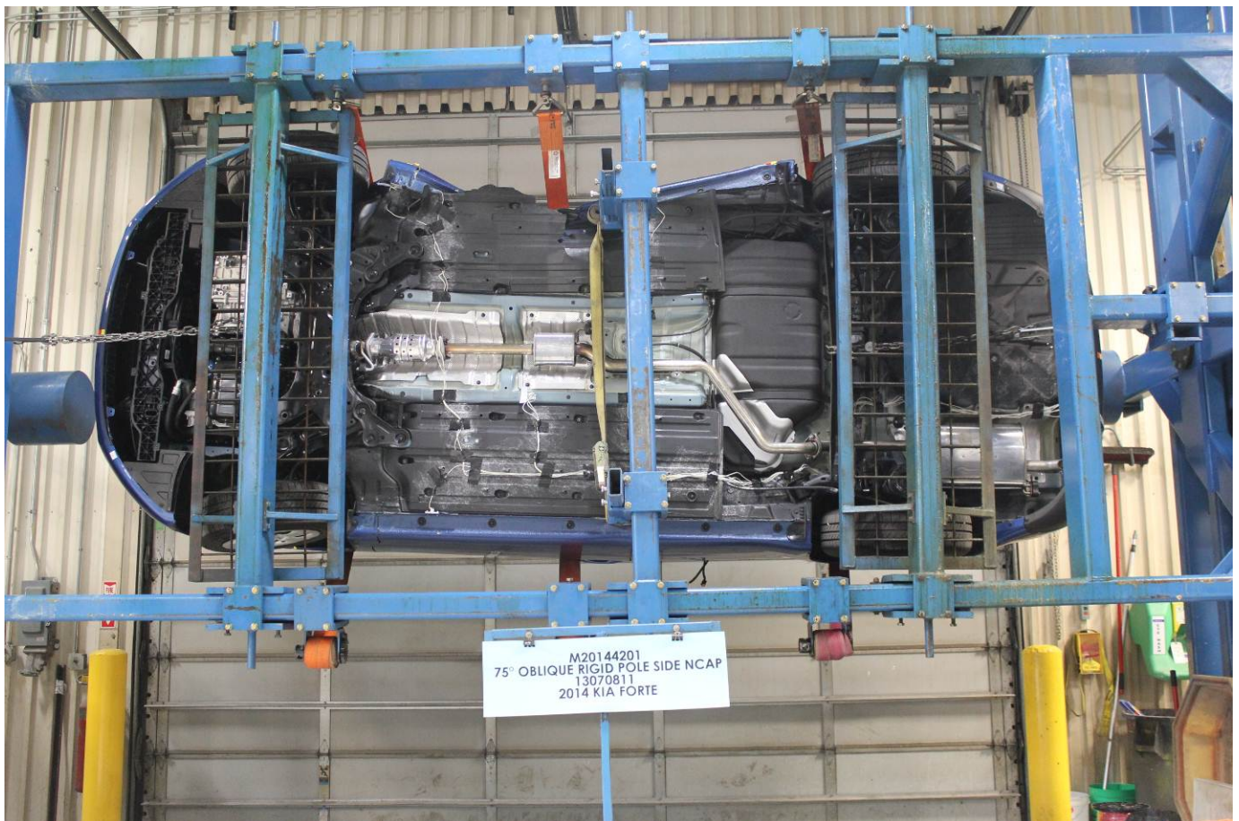
FMVSS No. 301 Static Rollover 270 Degrees
