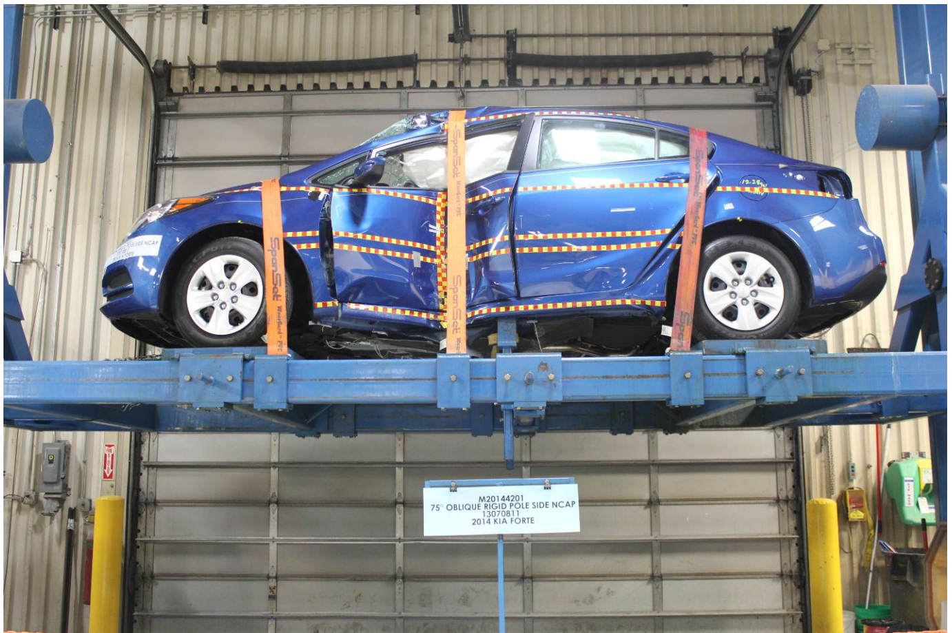
FMVSS No. 301 Static Rollover 0 Degrees
