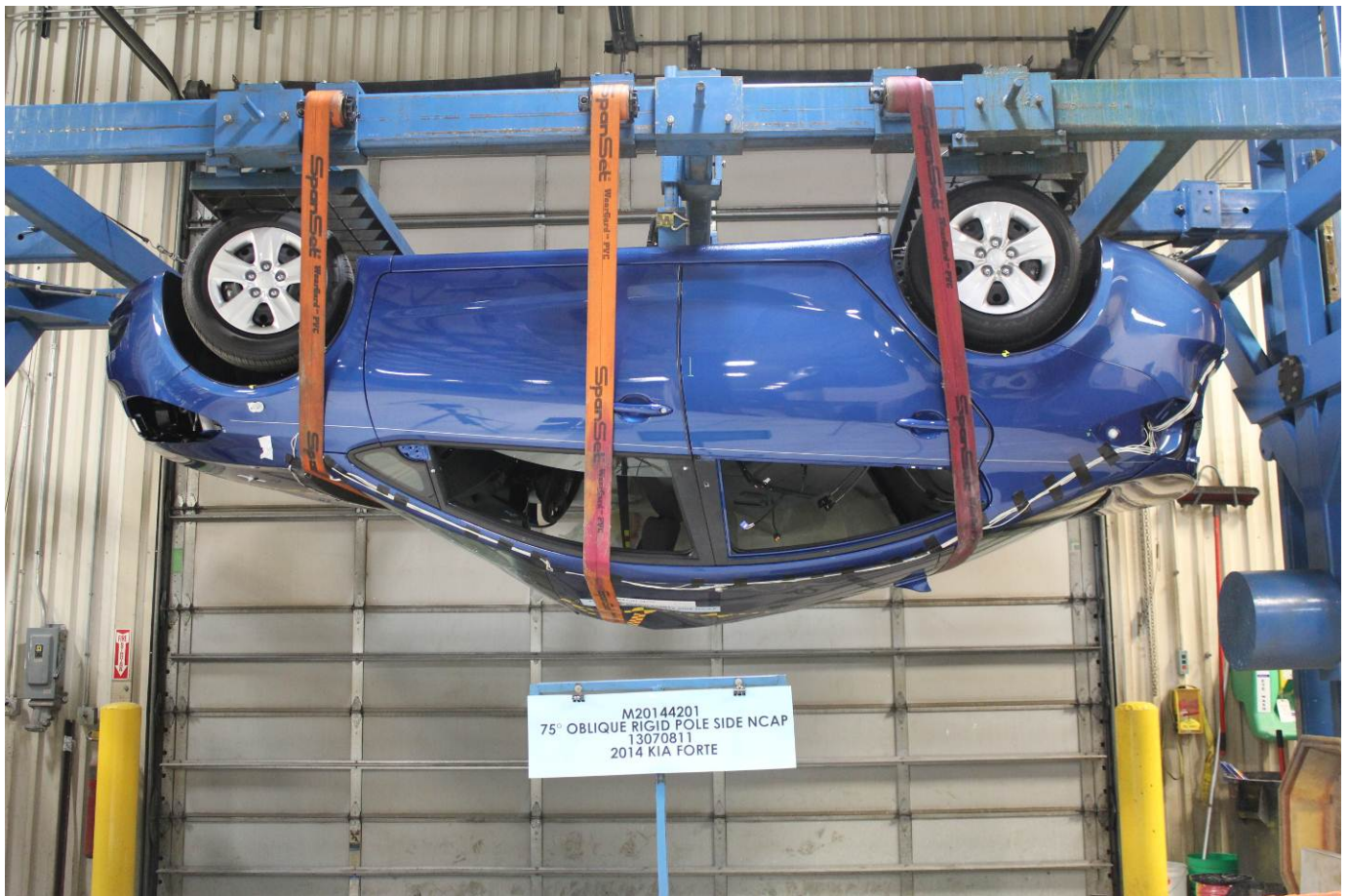
FMVSS No. 301 Static Rollover 180 Degrees
