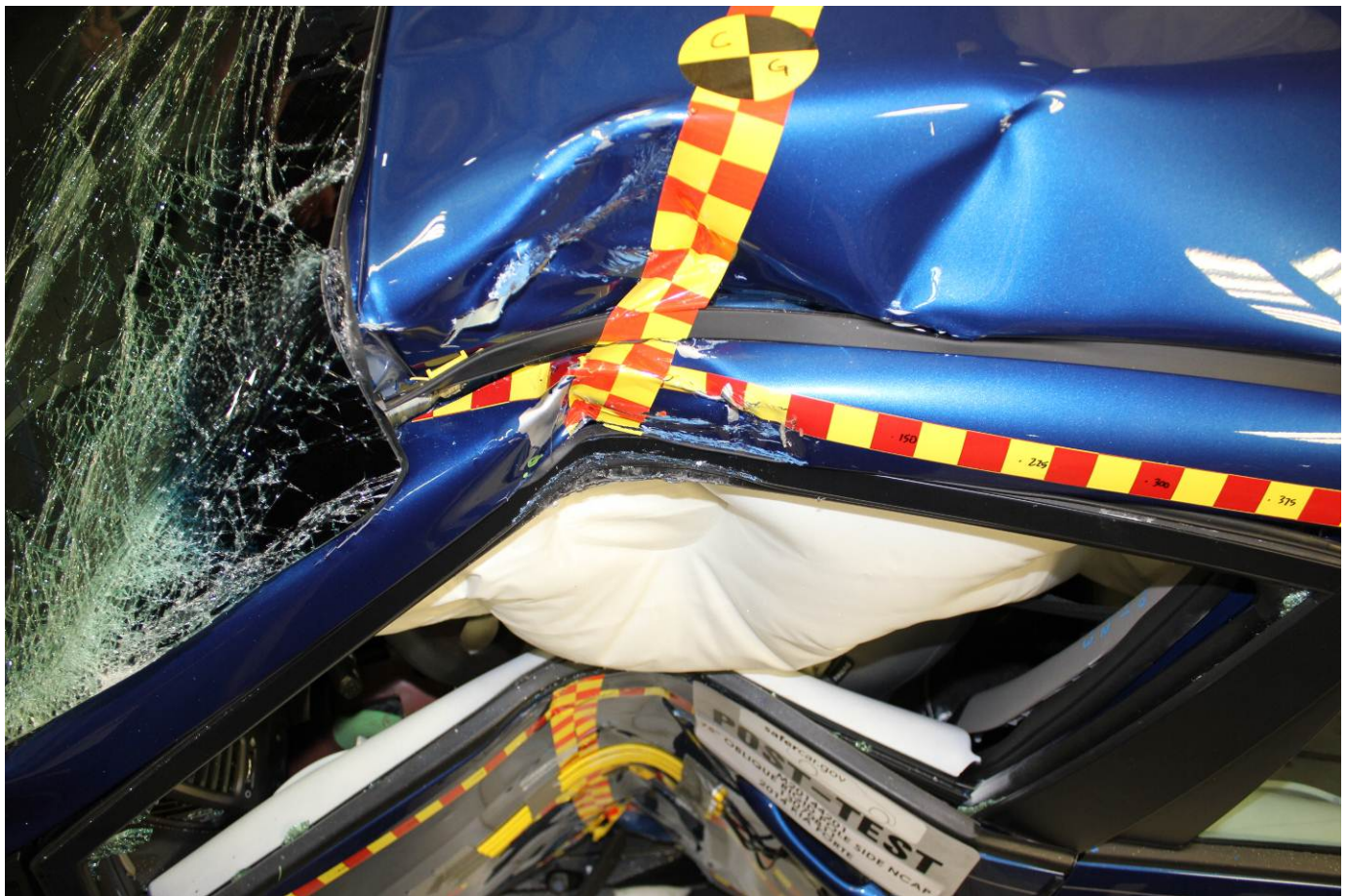
Post-Test Dummy and Door Clearance View
