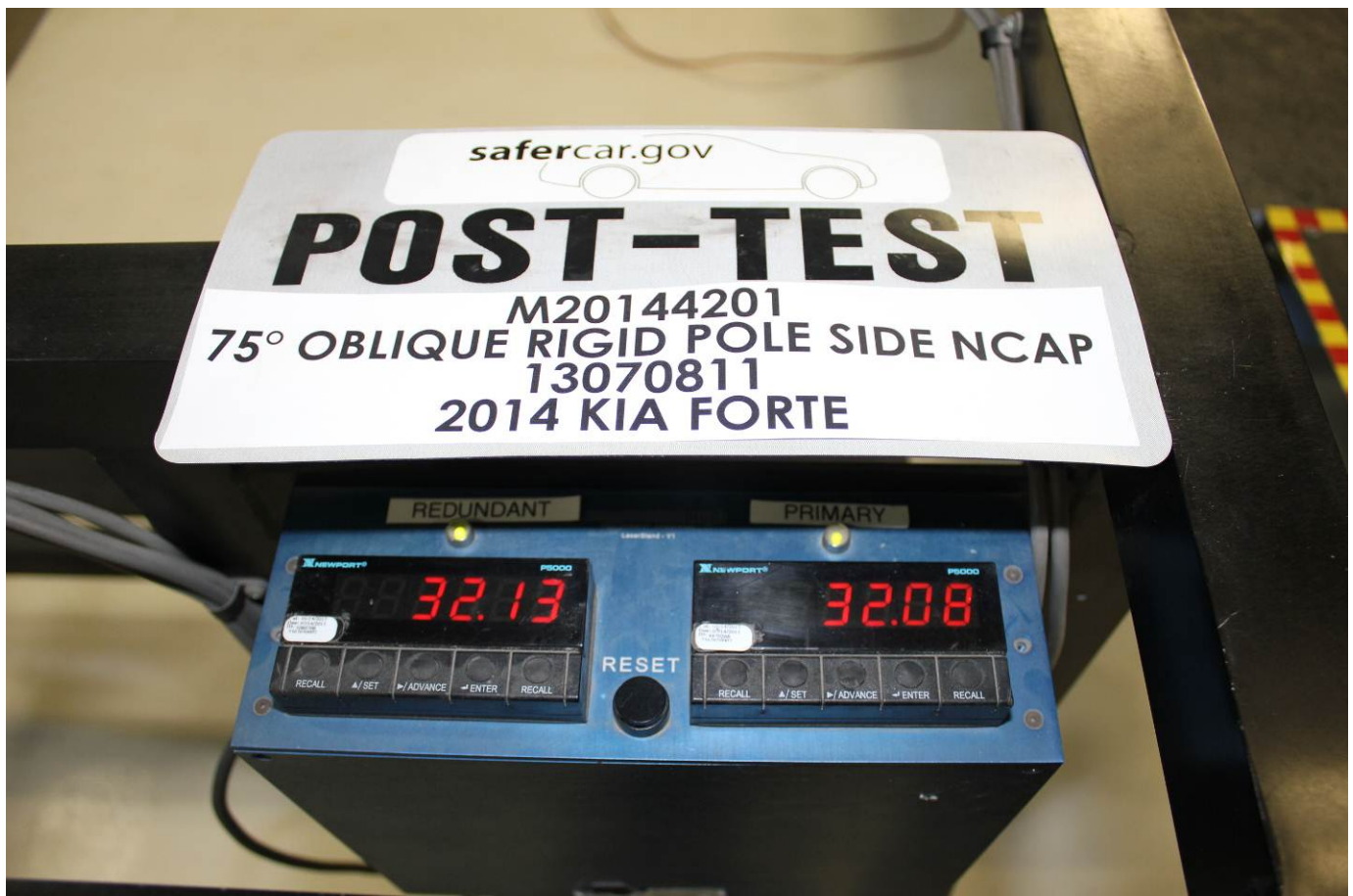
Post-Test Primary and Redundant Speed Trap Read-Out
