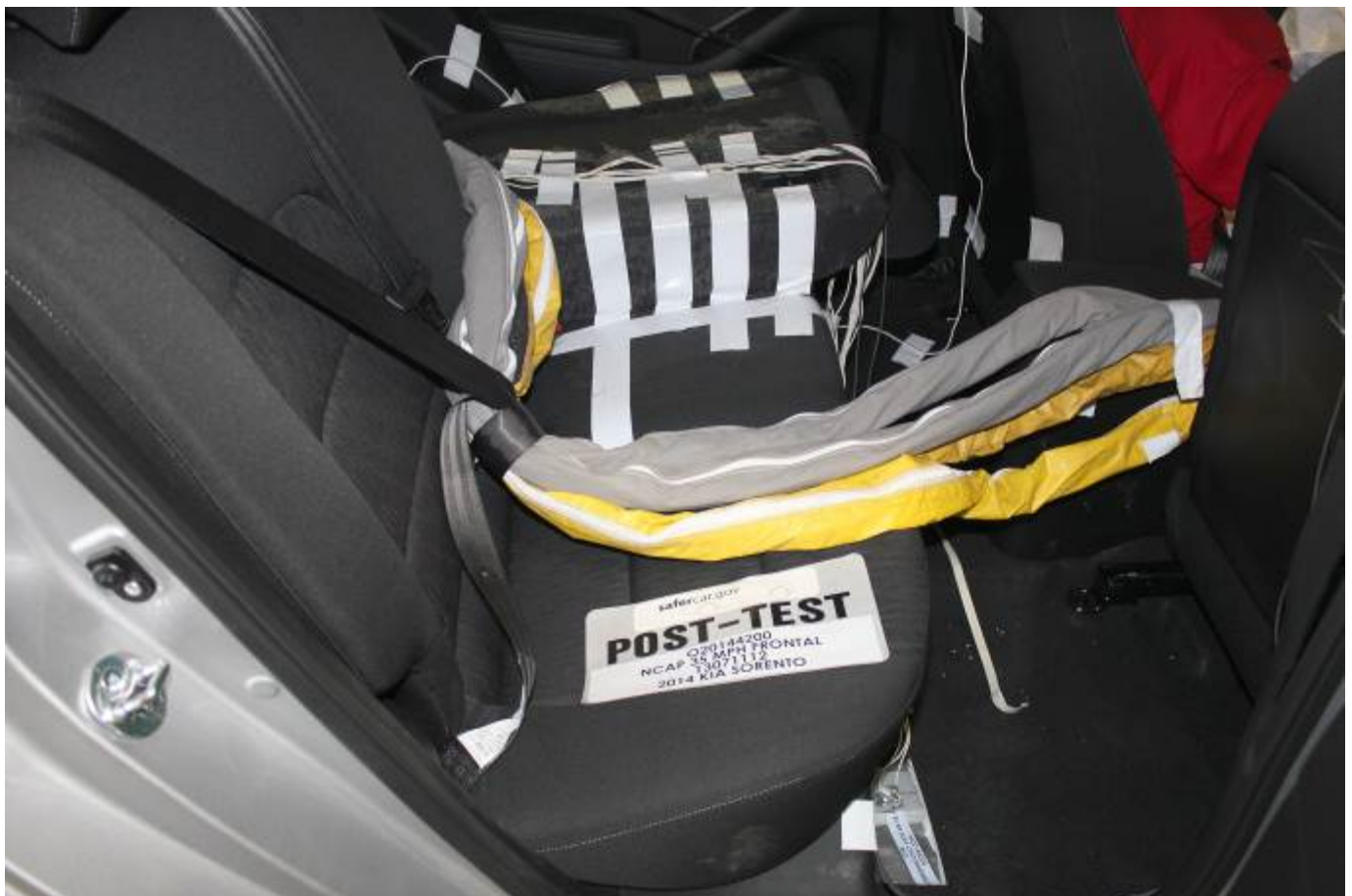
Post-Test Dummy Cable Routing
